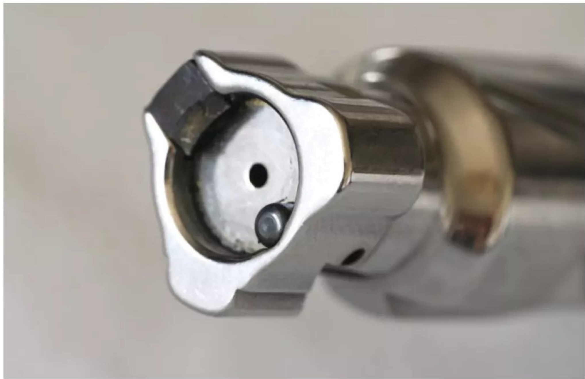
Franchi is hardly the first to utilize the tri-lug bolt design, but this design suits the MATE's functionality very well.
