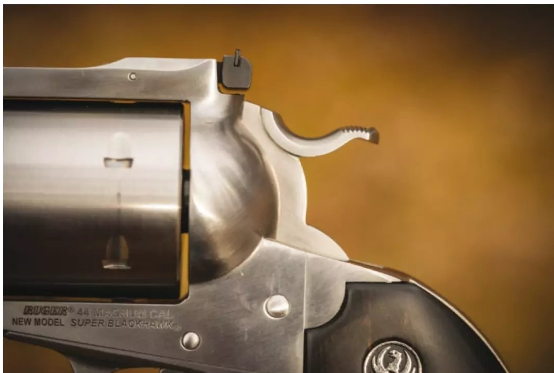
The Bisley hammer on this compact big-bore revolver is easier to manipulate than the standard hammer.
