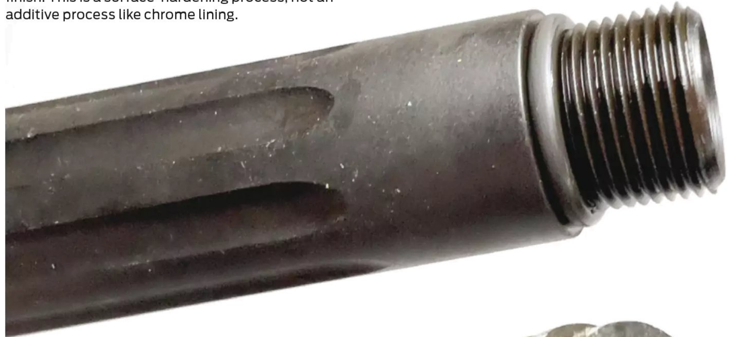
An original M1 Garand barrel showing lack of chrome lining.
