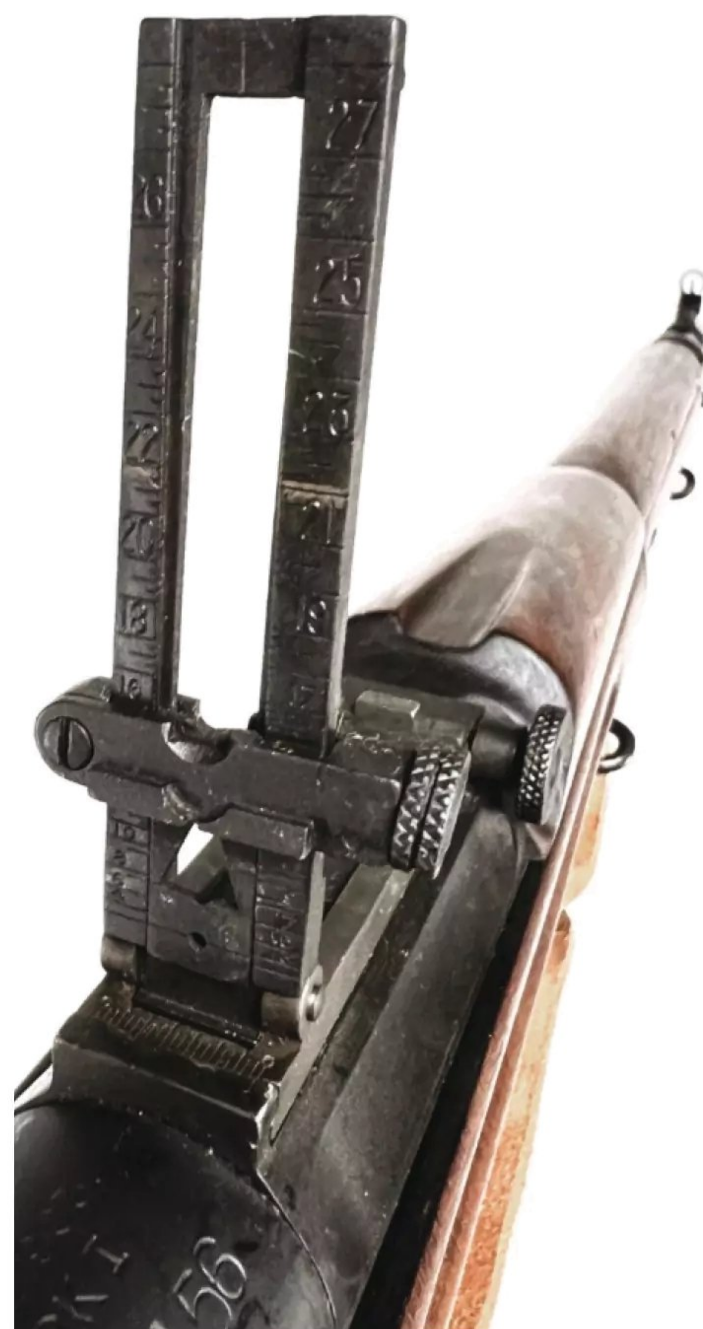
The Springfield rear sight is advanced yet simple, affording the shooter four aiming points either as U-notch or peep sight, and it even incorporated spin drift. Outside of an optical sight, this rear sight is about as good as it gets for the era.
