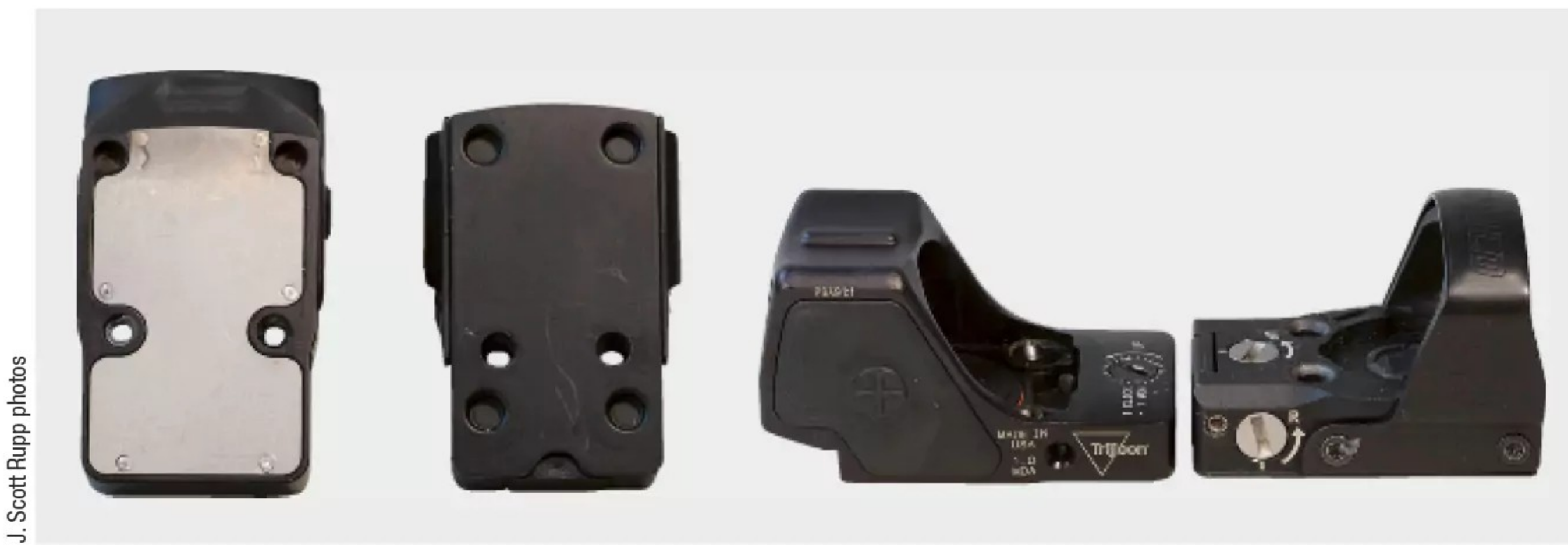
▲ The Trijicon RMR (l.) footprint has sockets only at the front, while the Leupold DeltaPoint Pro (r.) has them front and rear. Socket-to-hole and hole spacing are also different. The sights' deck heights and screw layouts dictate the types of screws necessary.
