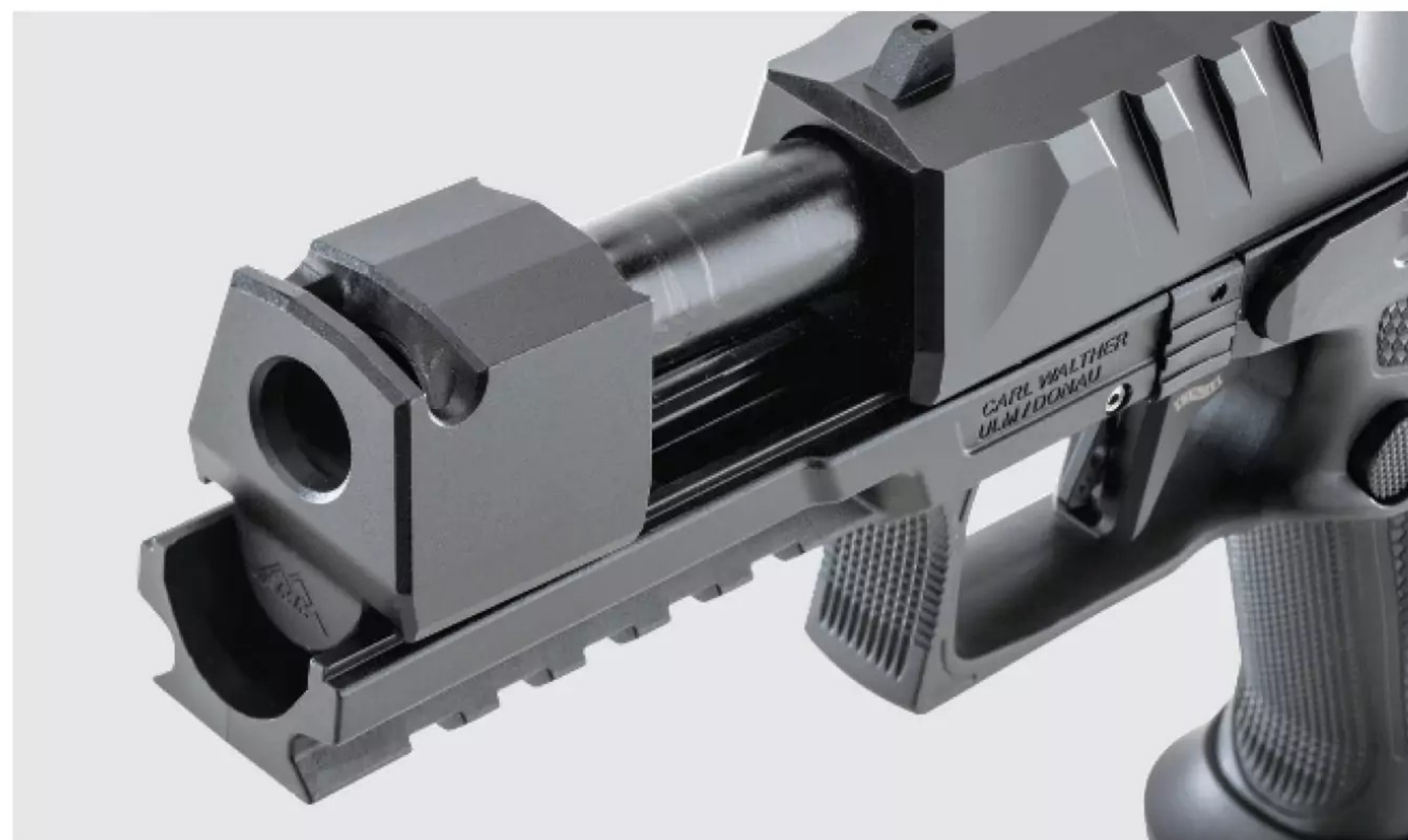
A The anodized aluminum compensator comes from Parker Mountain Machine. It's secured with Rocksett Engineering Adhesive and butts up against the slide for a solid fit.
