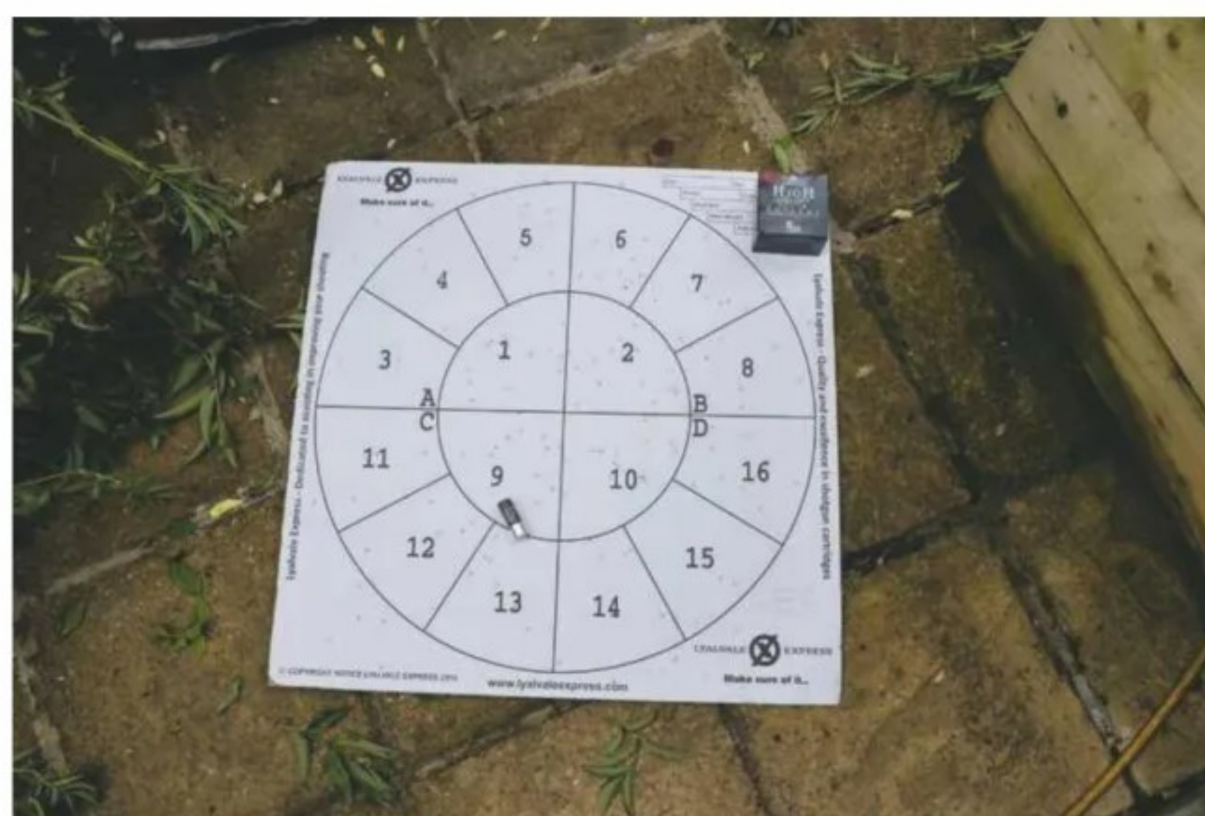
The larger No. 4 shot size (plastic wad) achieved a total of 155 pellet strikes within 30"
