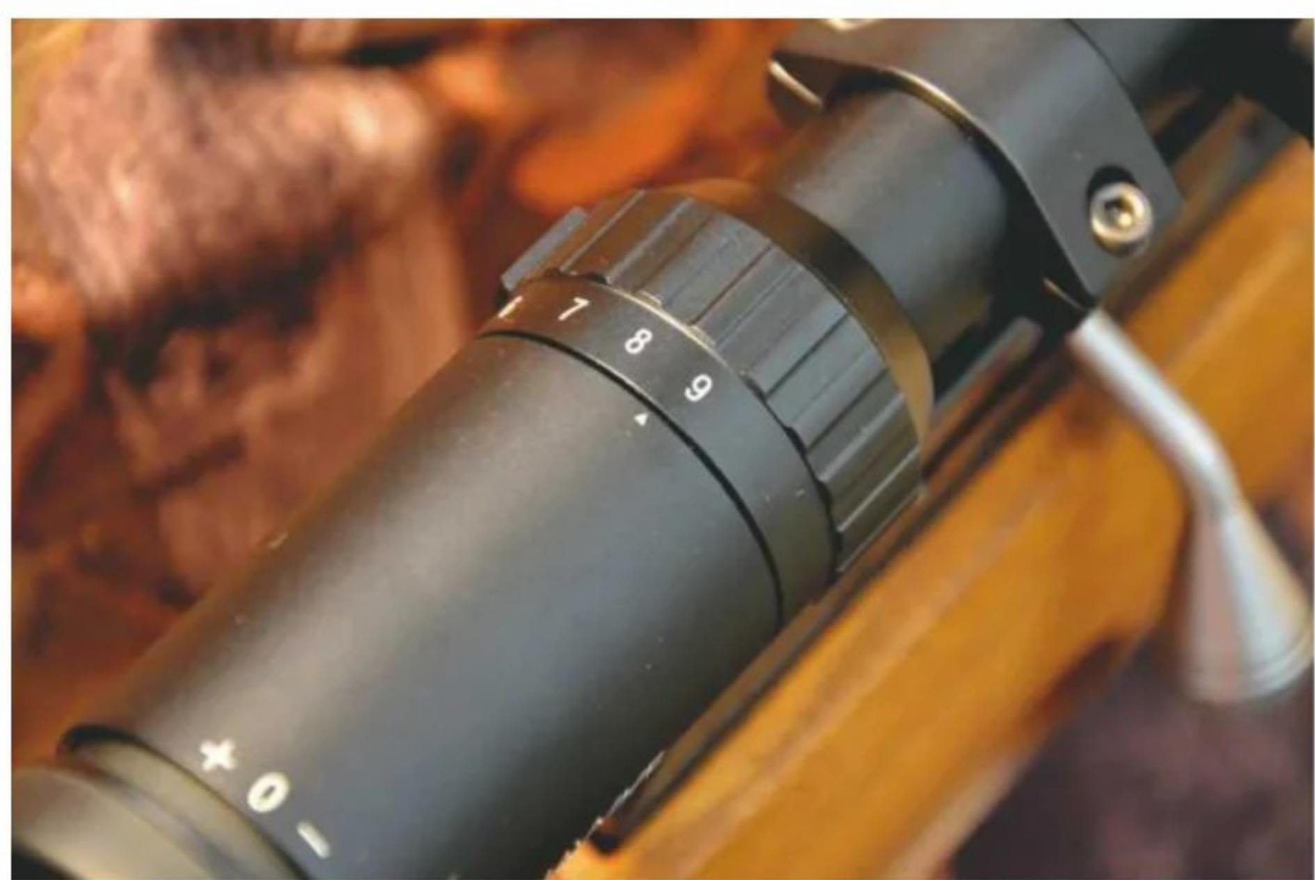
Note the knurled magnification collar
