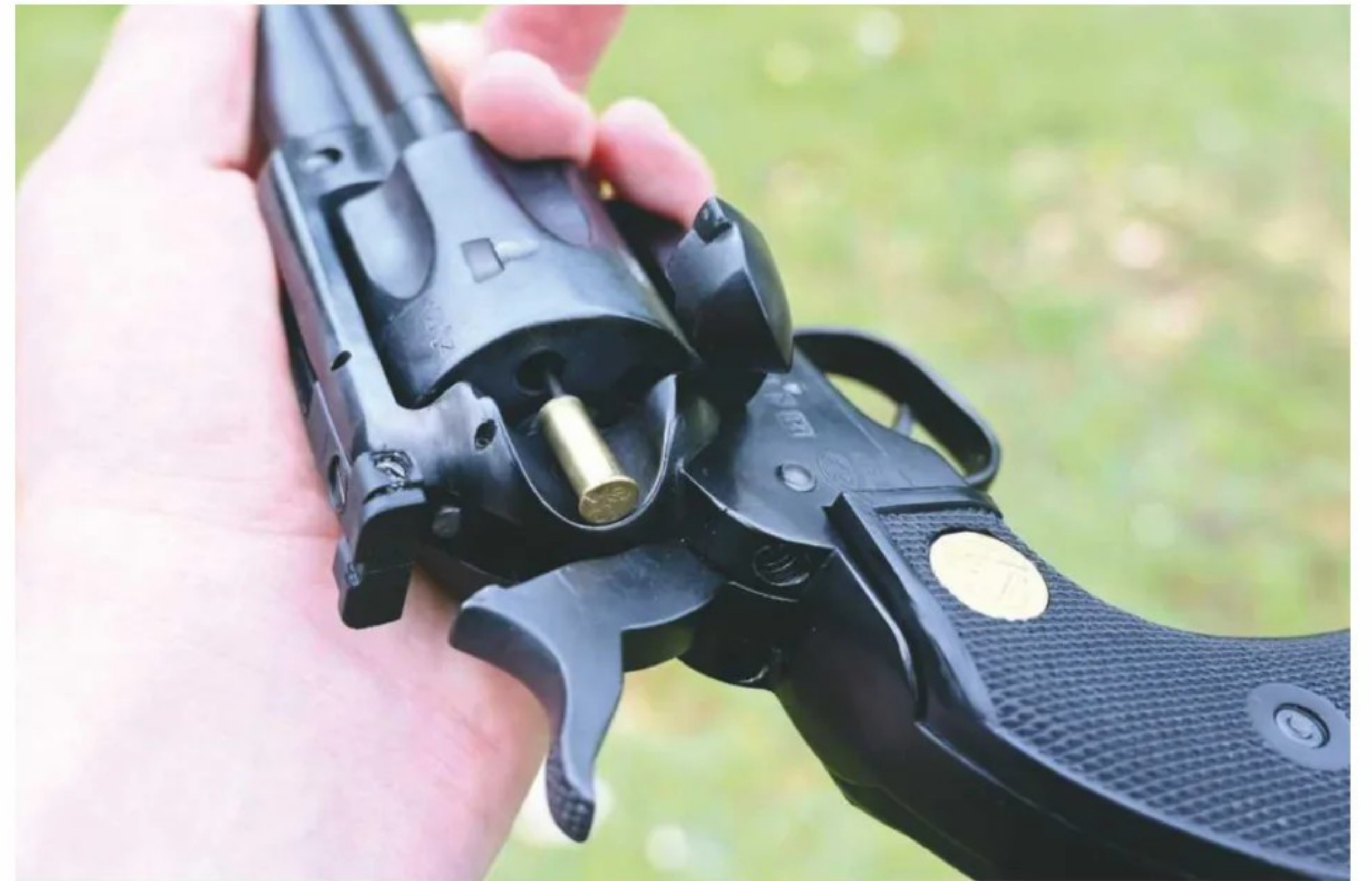
With all the rounds depleted, you can use the manually operated ejector rod to push the empties out. Note the protruding pin
