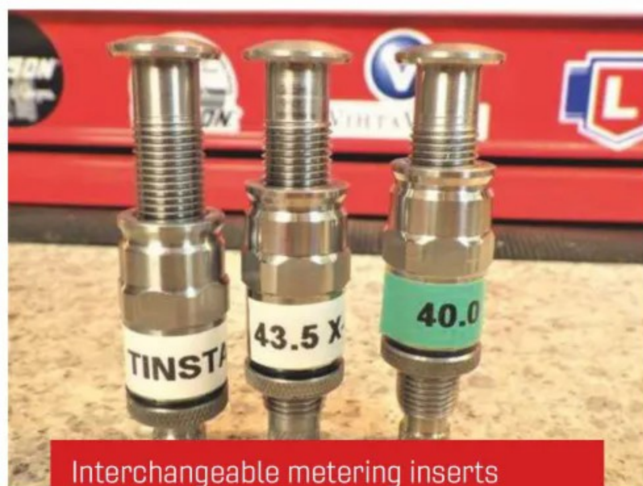
Interchangeable metering inserts labelled and set for different loads
