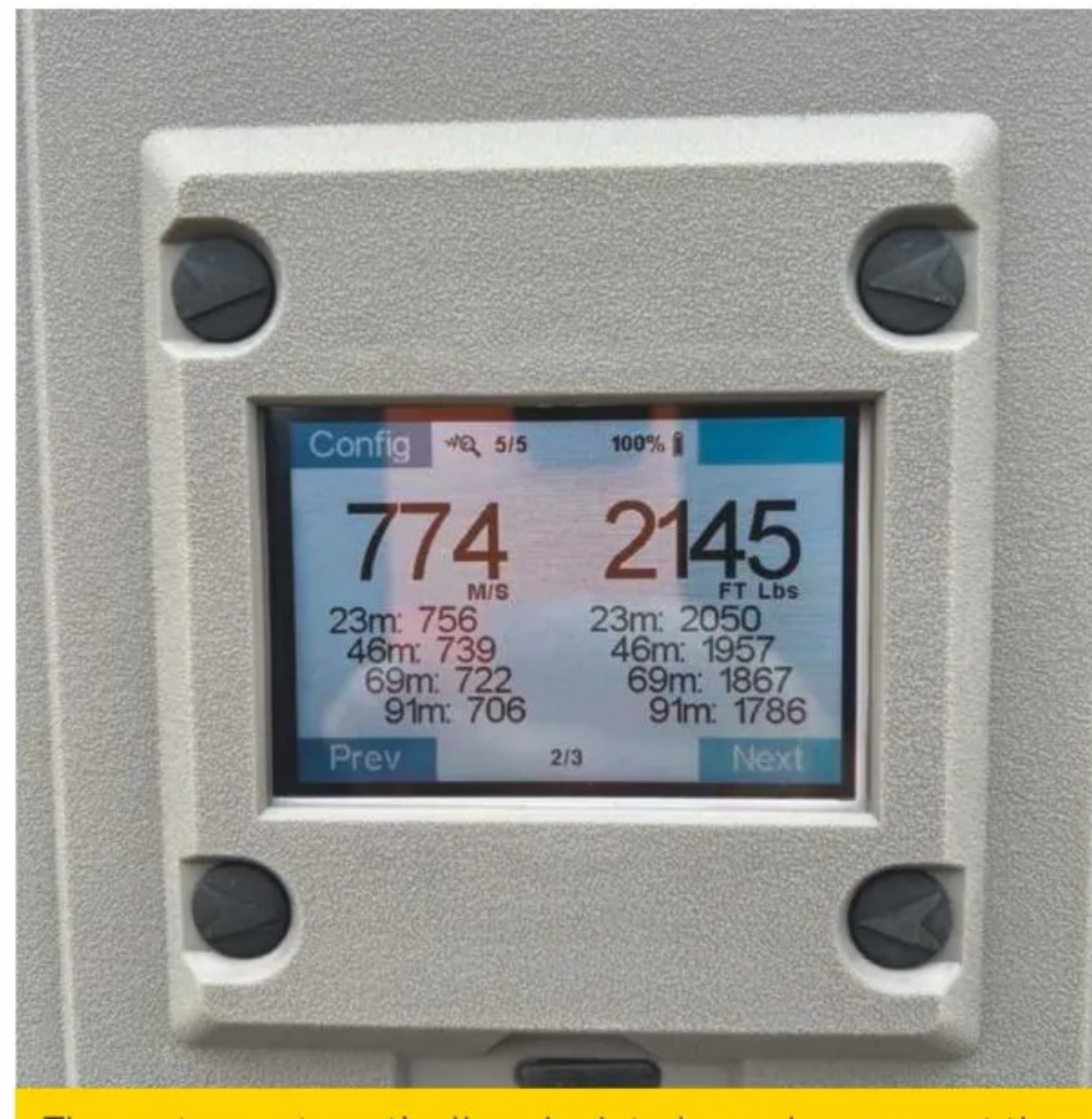
The system automatically calculated muzzle energy at the same intervals (remember to enter bullet weight!)
