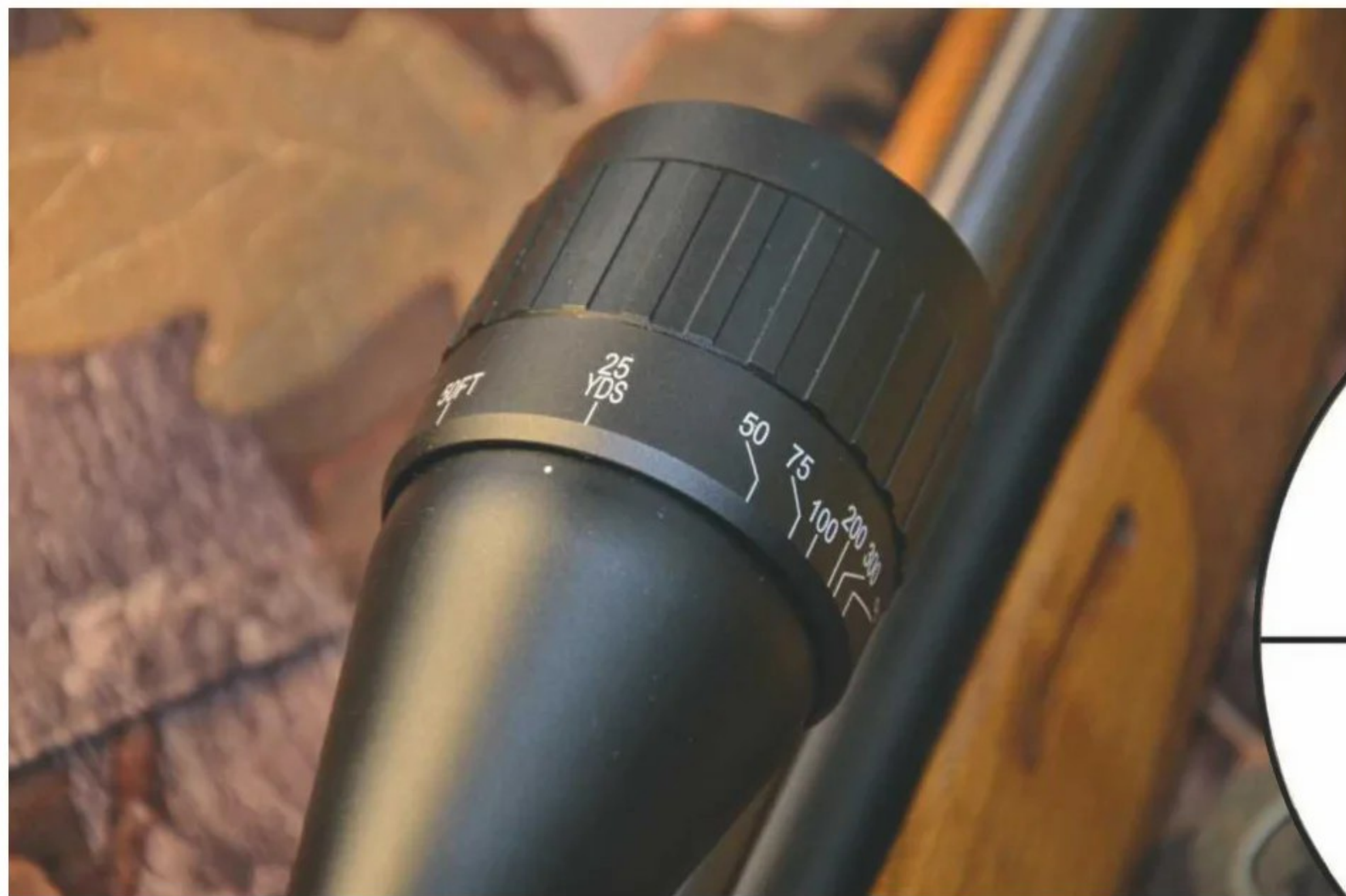
(Left) AO denotes 'Adjustable Objective' lens. Note the markings
