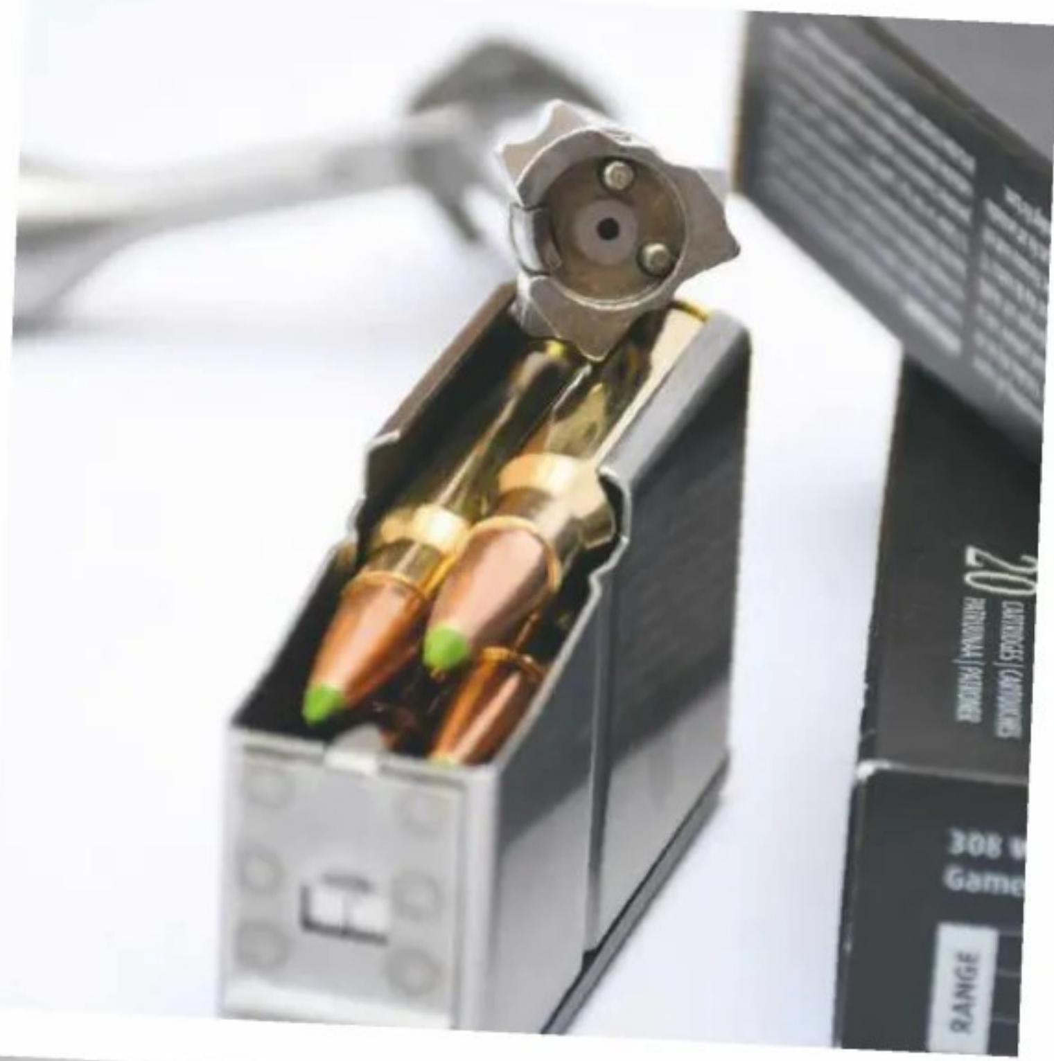
The recessed push feed bolt face has returned. Note the twin sprung plunger ejectors
