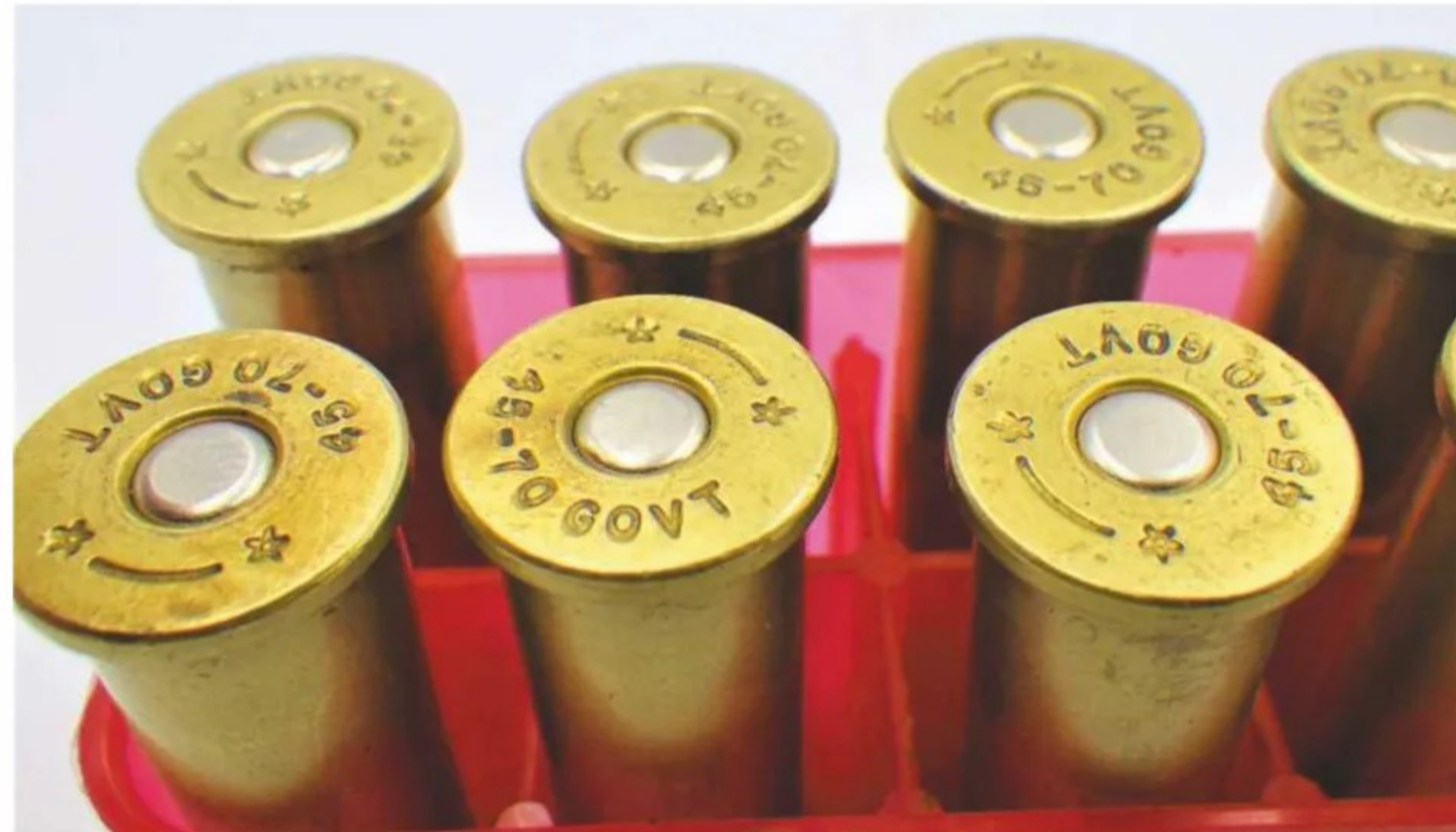
Perfectly seated primers for consistent ammunition make hand priming worthwhile
