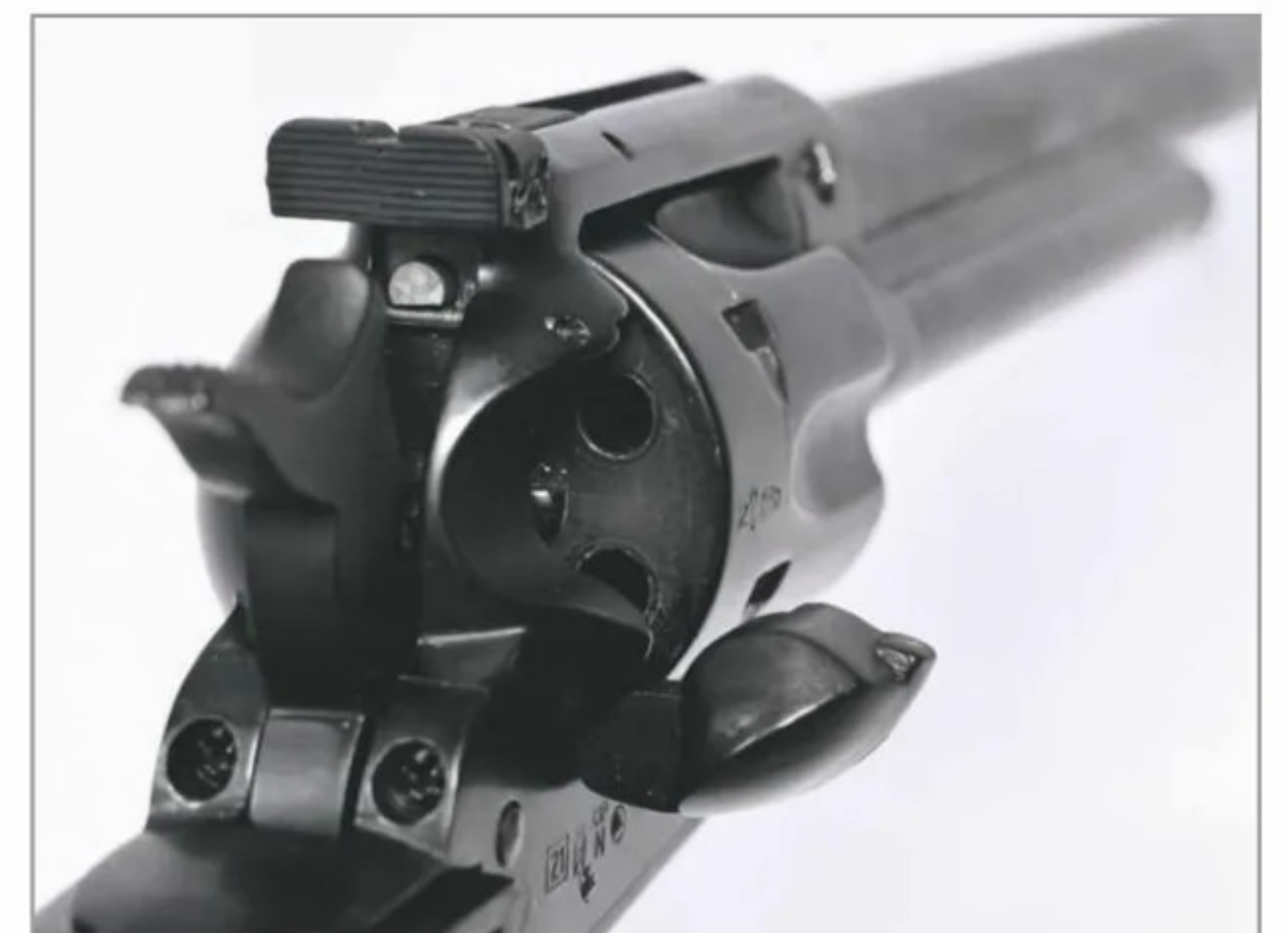
A closer look at the loading gate and the rear of the cylinder
