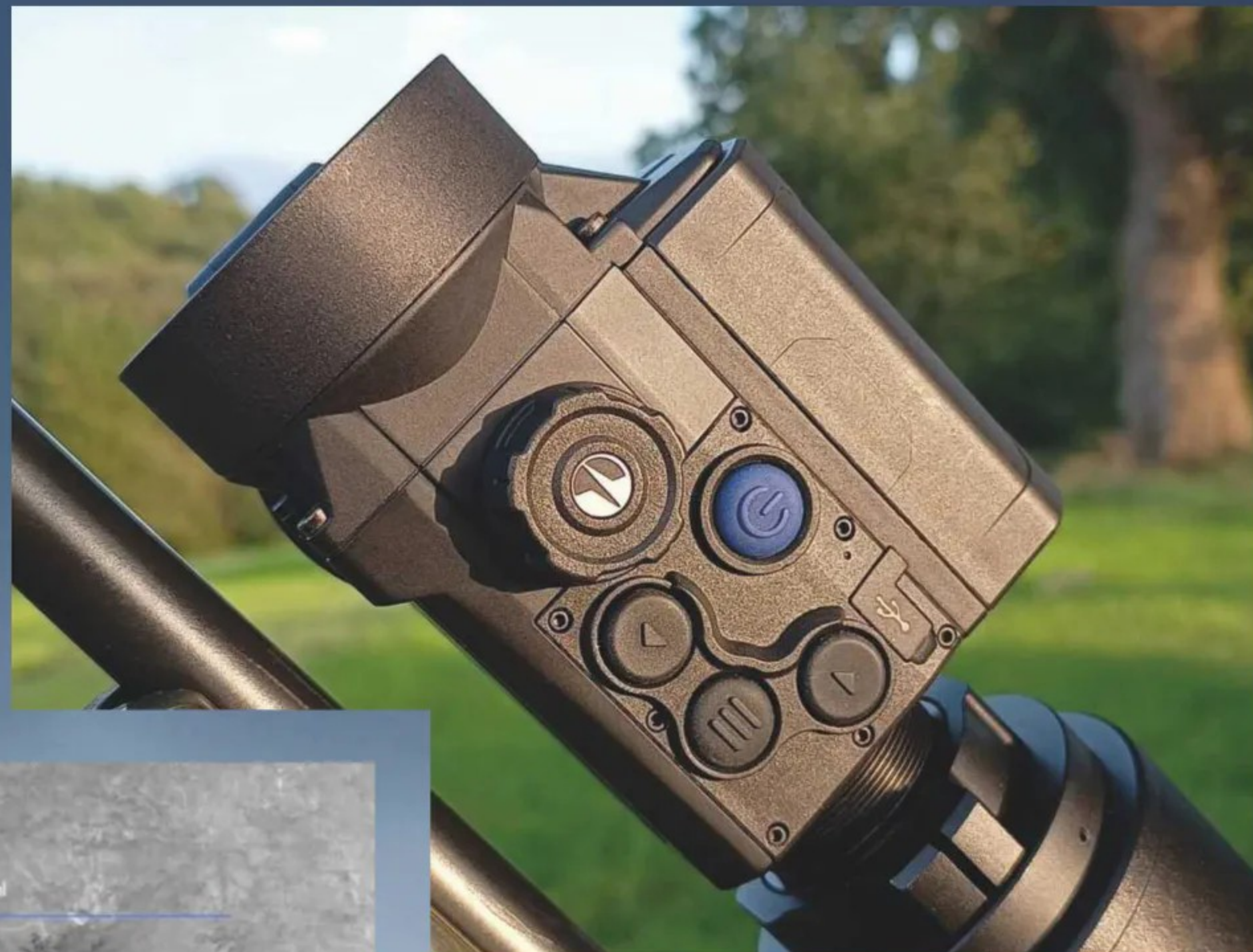
Personally, I'd have the UP and DOWN buttons next to each other! Note the neat cover to the USB-C port at the rear
