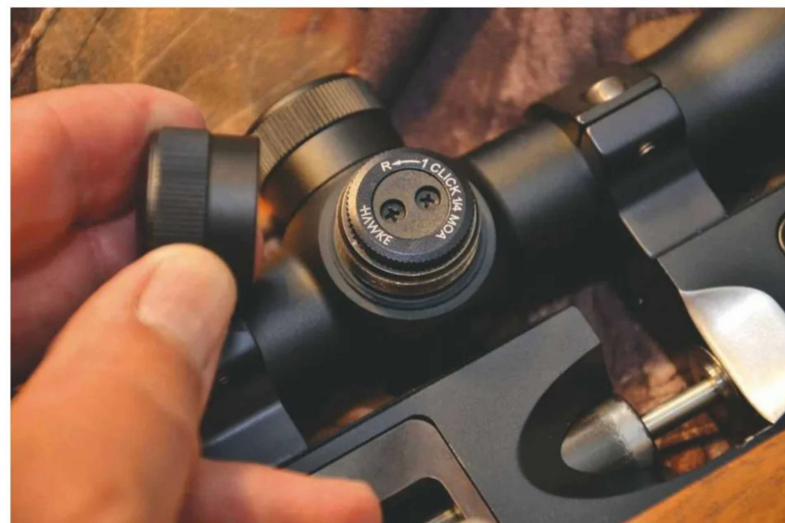
The clicks are positive. Note the low-profile turrets
