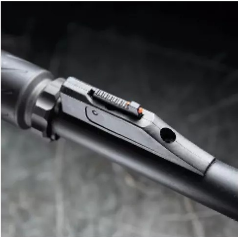
A fixed U-notch, two-dot sight is nestled inside the optic rail atop the receiver. The red fiber-optic front sight is height adjustable.
