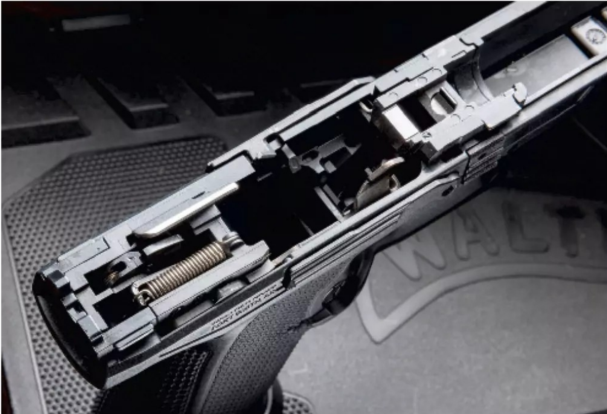
Internally, the action parts are identical to a standard F-Series PDP with a Dynamic Performance Trigger F-Series installed. This is as far as most users will disassemble the PDP.
