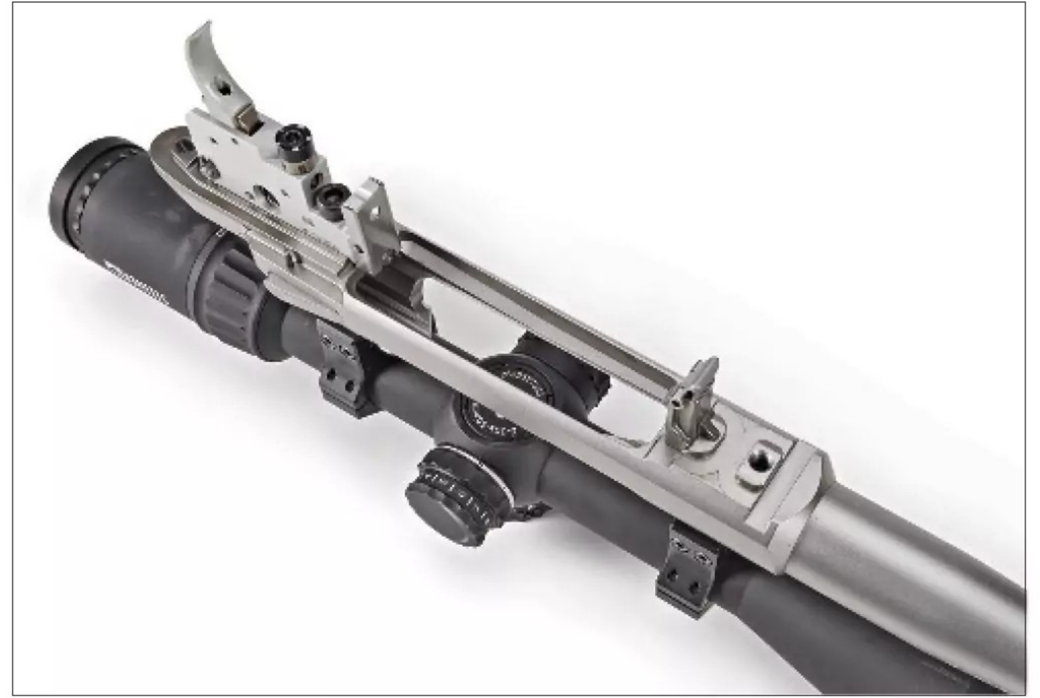
The recoil lug is integral to the SAKO 90 receiver. Both action screws thread deeply into the receiver. With the stock removed, the user has easy access to the trigger adjustment screws.
