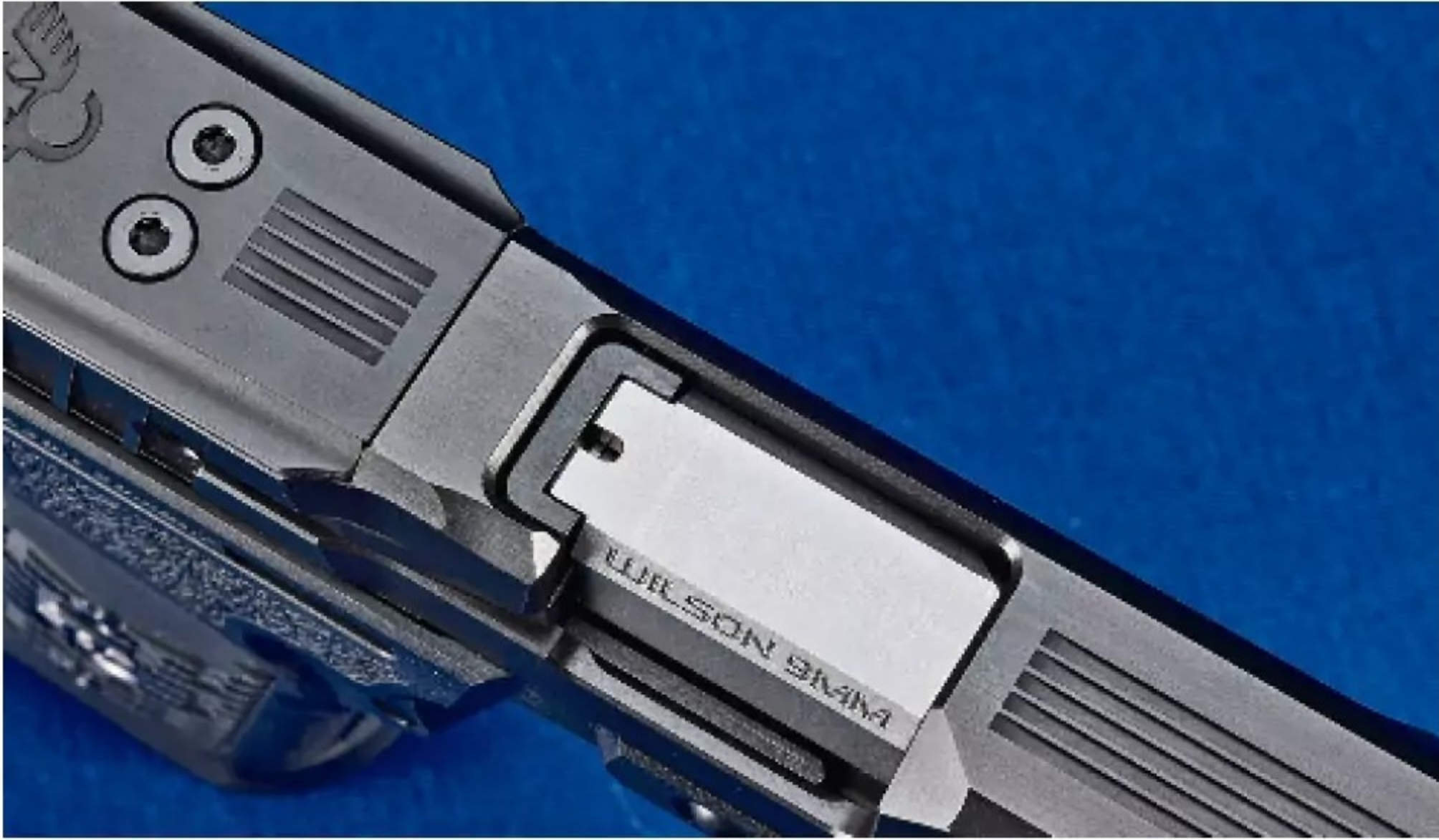
A loaded chamber indicator can be used to confirm a firearm's status at a glance. The top of the slide is serrated to prevent glare from interfering with sighting while also enhancing aesthetics.
