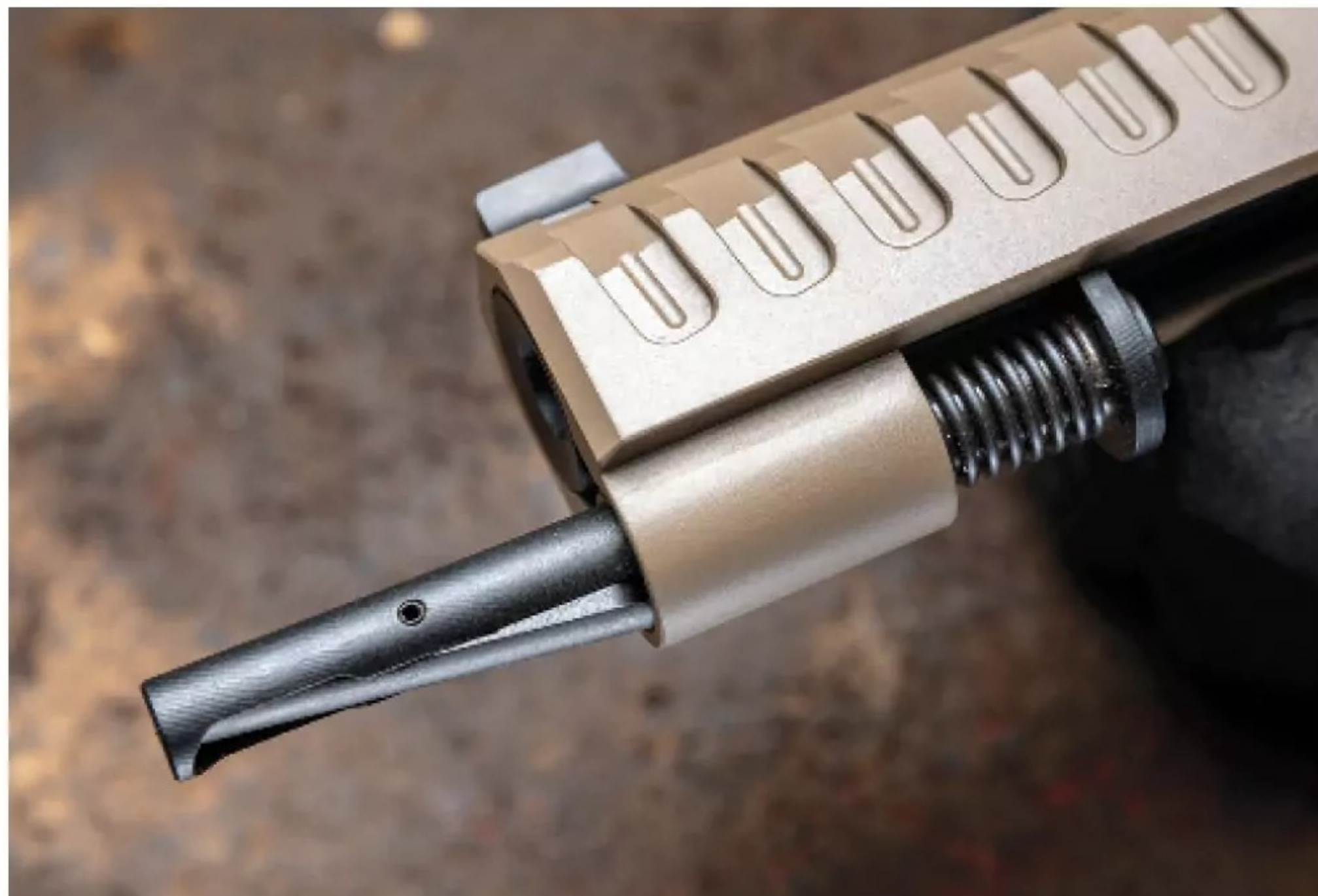
Bull barrels often require unique design approaches for disassembly. The Apache Commander's recoil spring has a lever that pivots out to capture the recoil spring to ease slide disassembly.
