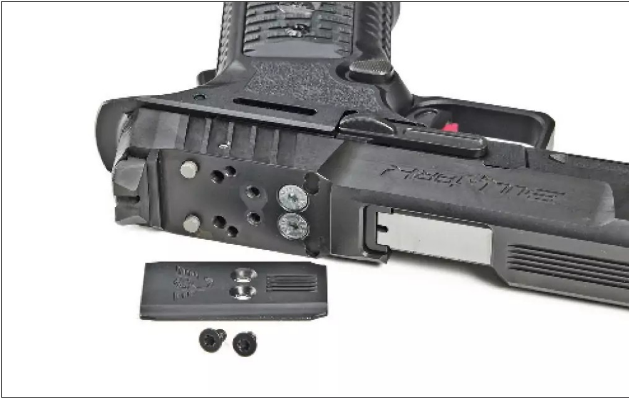
Cut for the Shield RMSc and Leupold DeltaPoint Pro optic footprint, reflex sights are supported with steel pins. These CPT pins bear the force of recoil so mounting screws don't have to.
