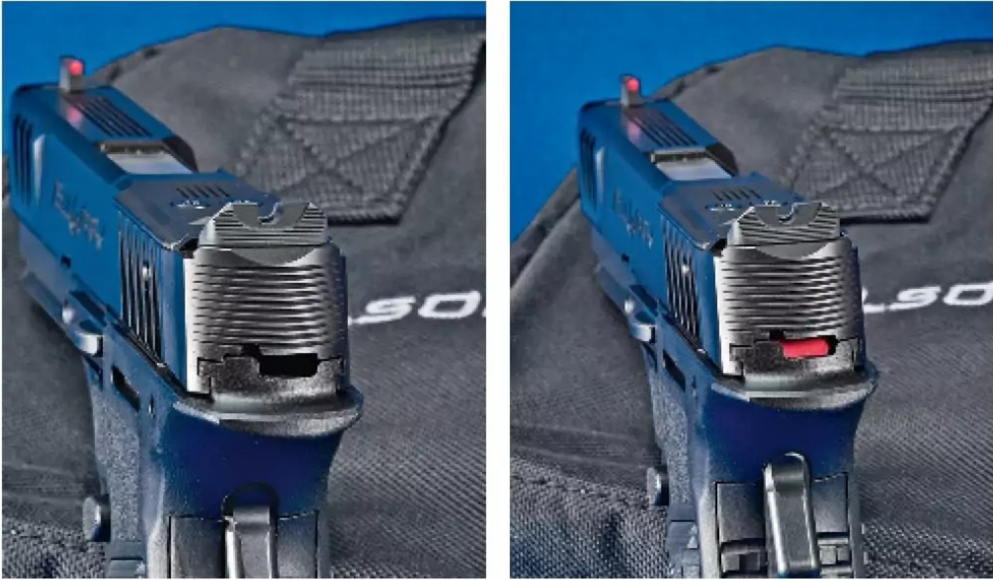
Even though the hammer is internal, a bright red portion of the hammer can be seen through the viewing port (above right), and it is not easily visible when uncocked (above left).
