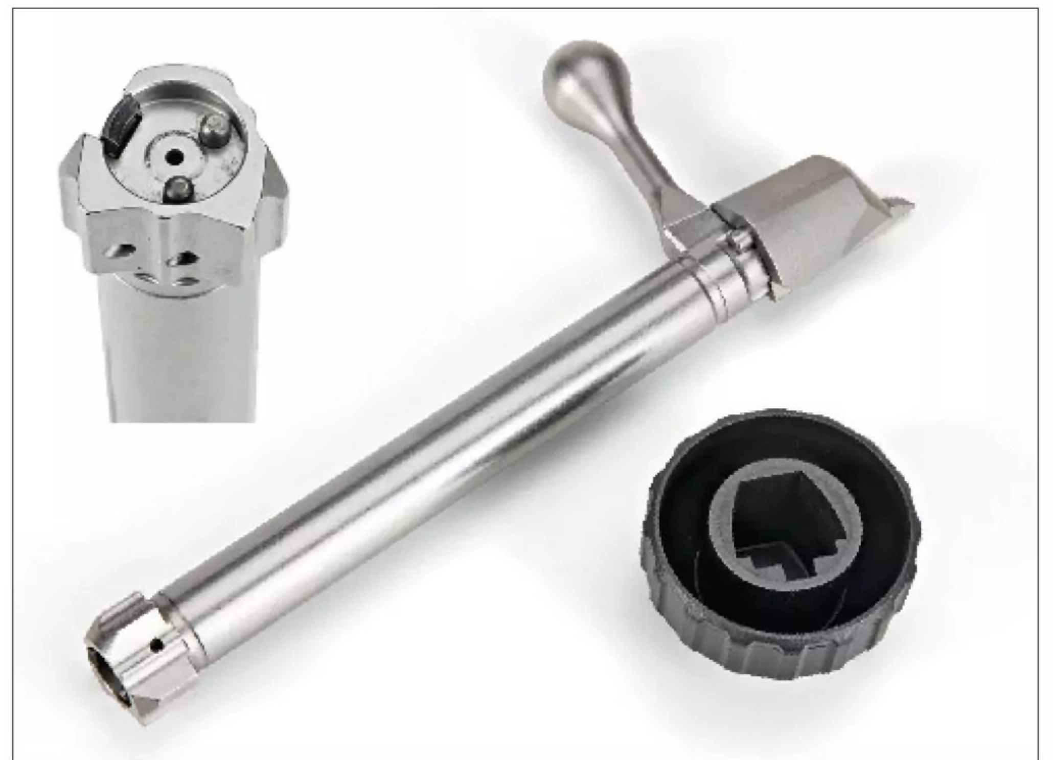
The bolt was designed for tool-less disassembly for easy field maintenance. The bolt face has two ears that drop down into the magazine for positive engagement and reliable feeding.
