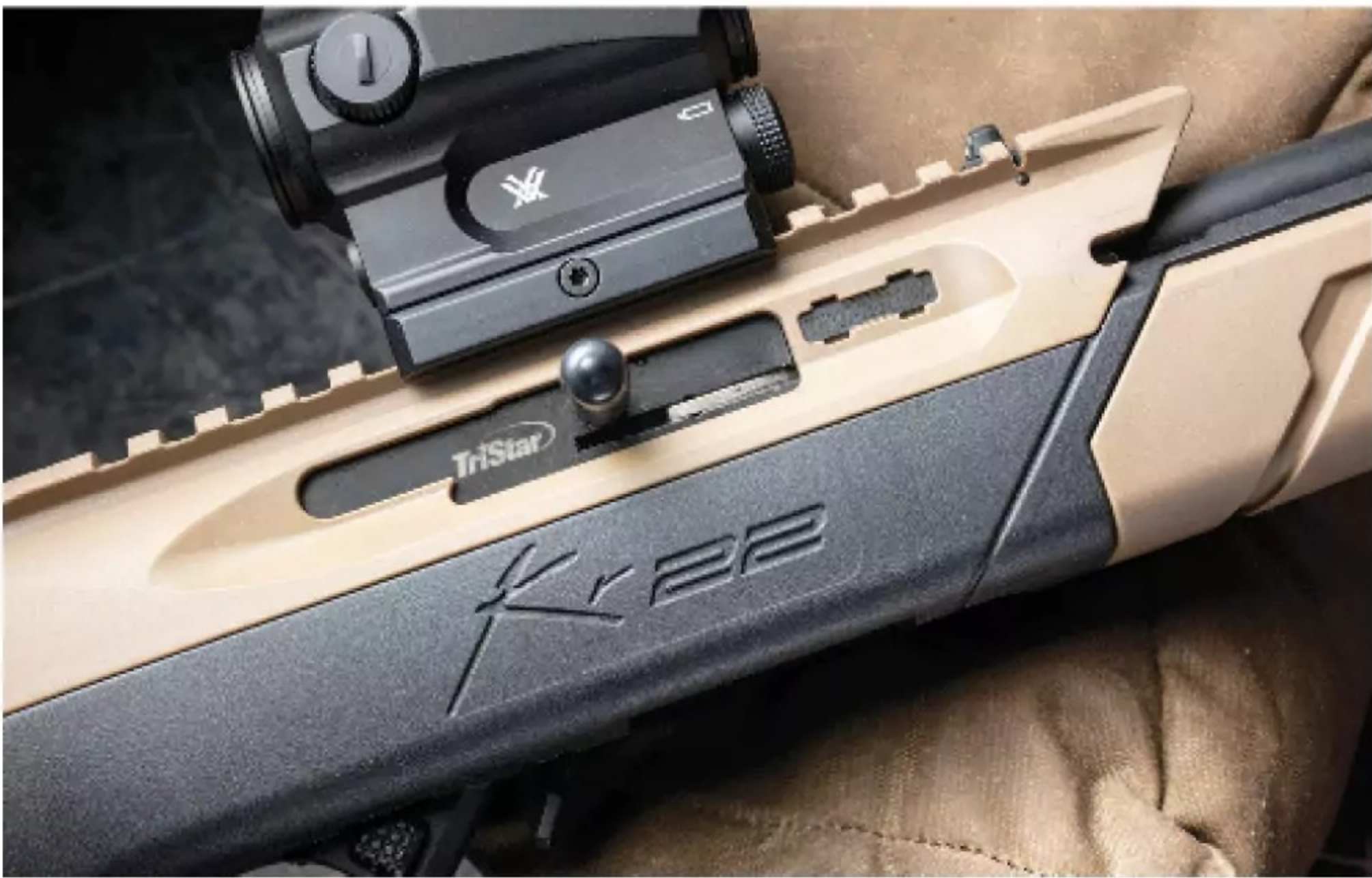
The charging handle can be unscrewed from one side of the bolt body and reattached to the opposite side. Great for lefties, a left-side charger is useful for right-handers behind the gun.
