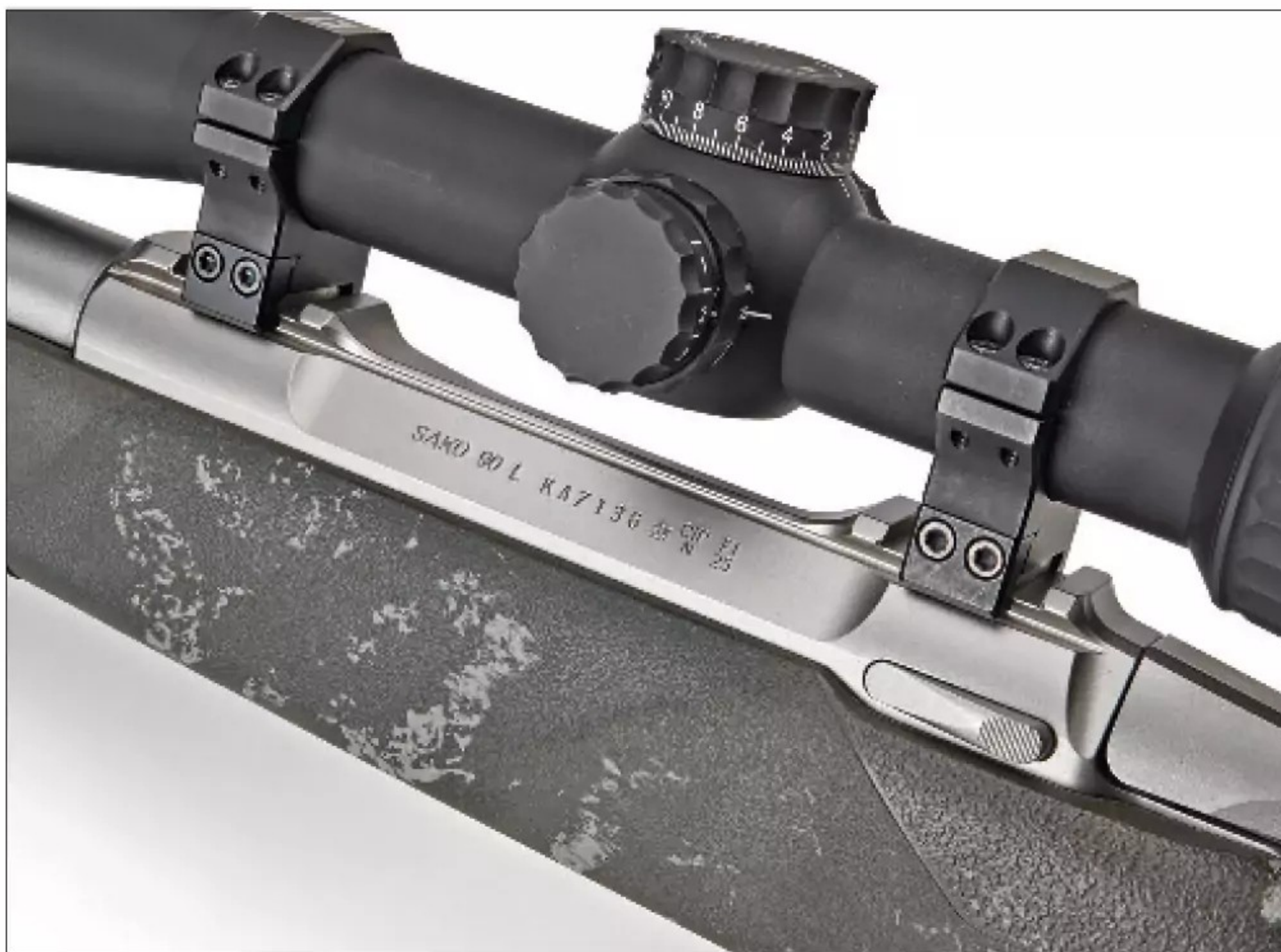
Also machined integrally on top of the receiver are scope-mounting rails. Integral rails never work loose and are low-profile, allowing a scope to sit close to the barrel.
