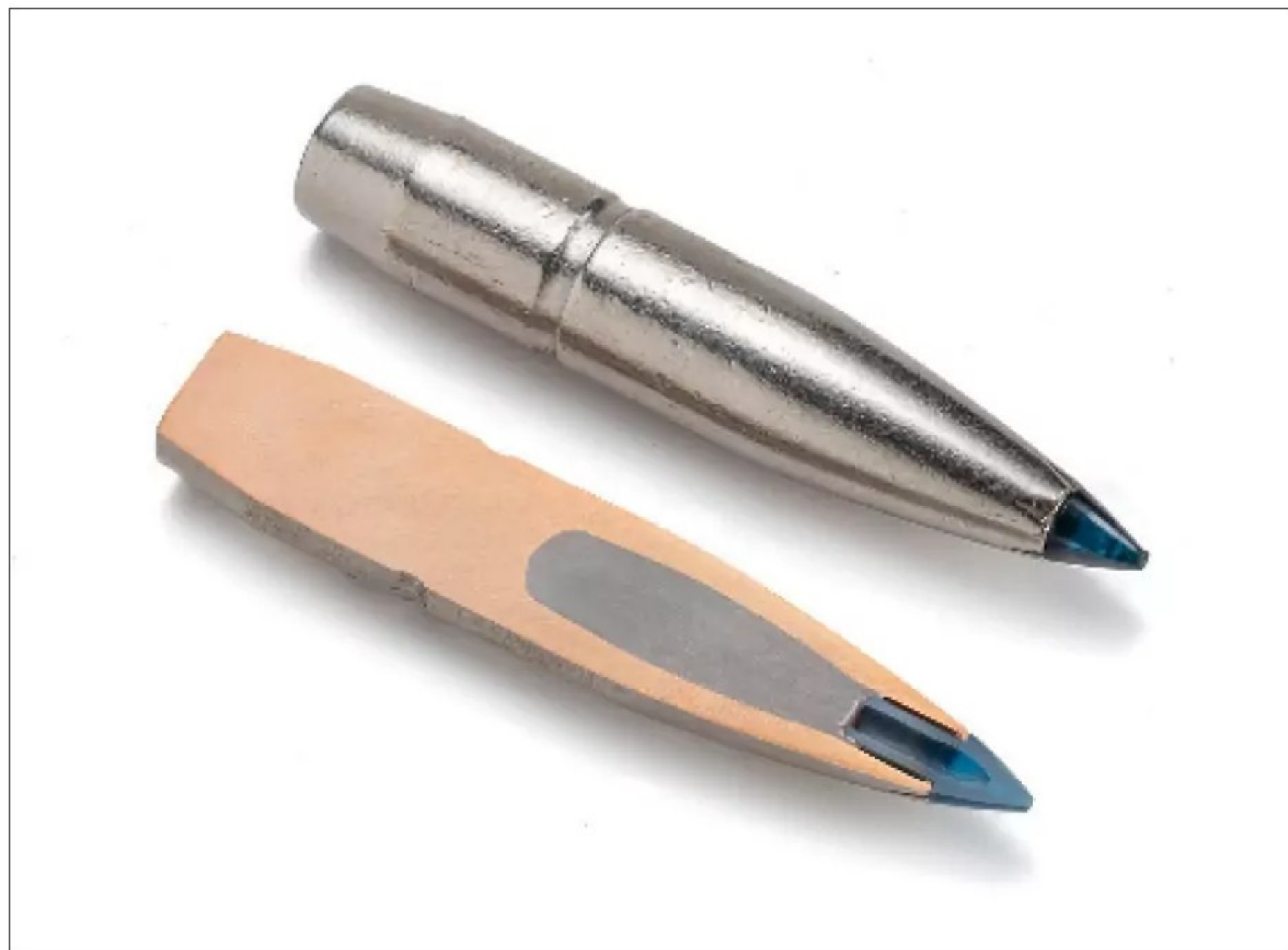
Federal's Terminal Ascent has an optimized boat-tail with AccuChannel on the nickel-plated bullet, and a Slipstream tip with a hollow core to initiate expansion at all distances.
