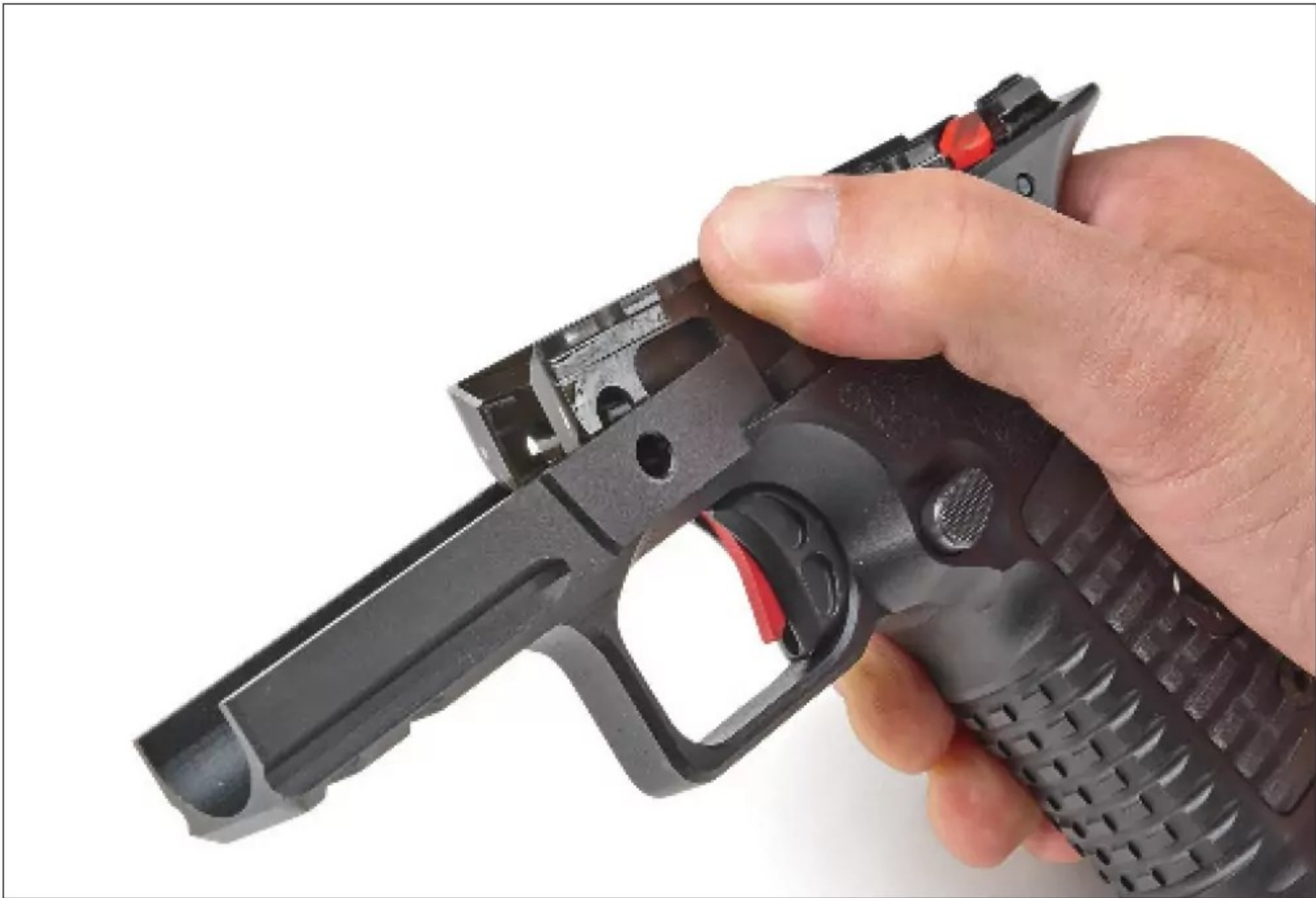
Inside the aluminum grip module, the stainless-steel fire control unit is the serialized component of the firearm. The number is viewable through a slot in the chassis on the top right side of the grip.
