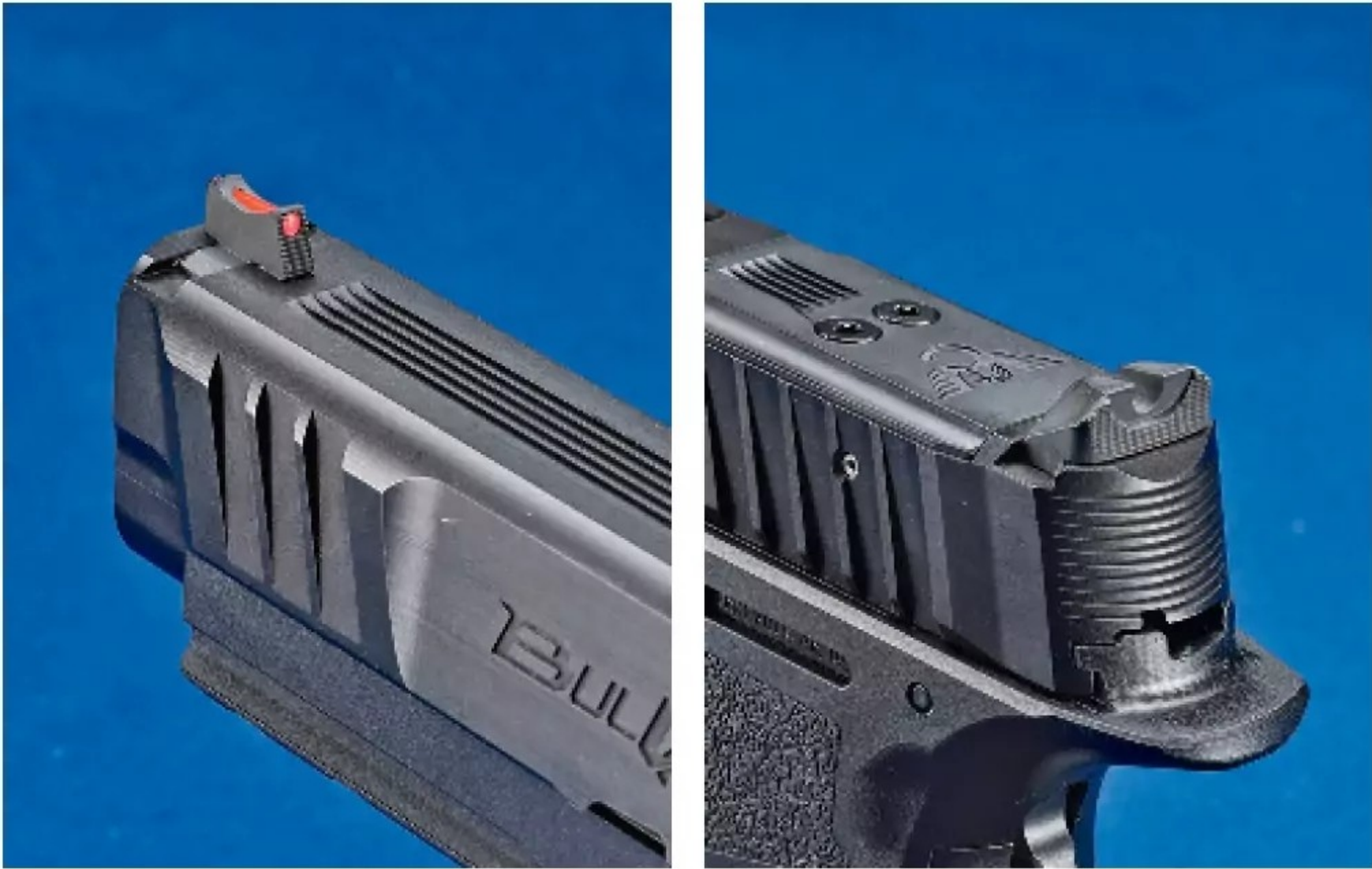
Sights are made by Wilson Combat and are tall enough to co-witness through many optics. The front includes a red fiber-optic insert, and the black rear sits far back to accommodate an optic.
