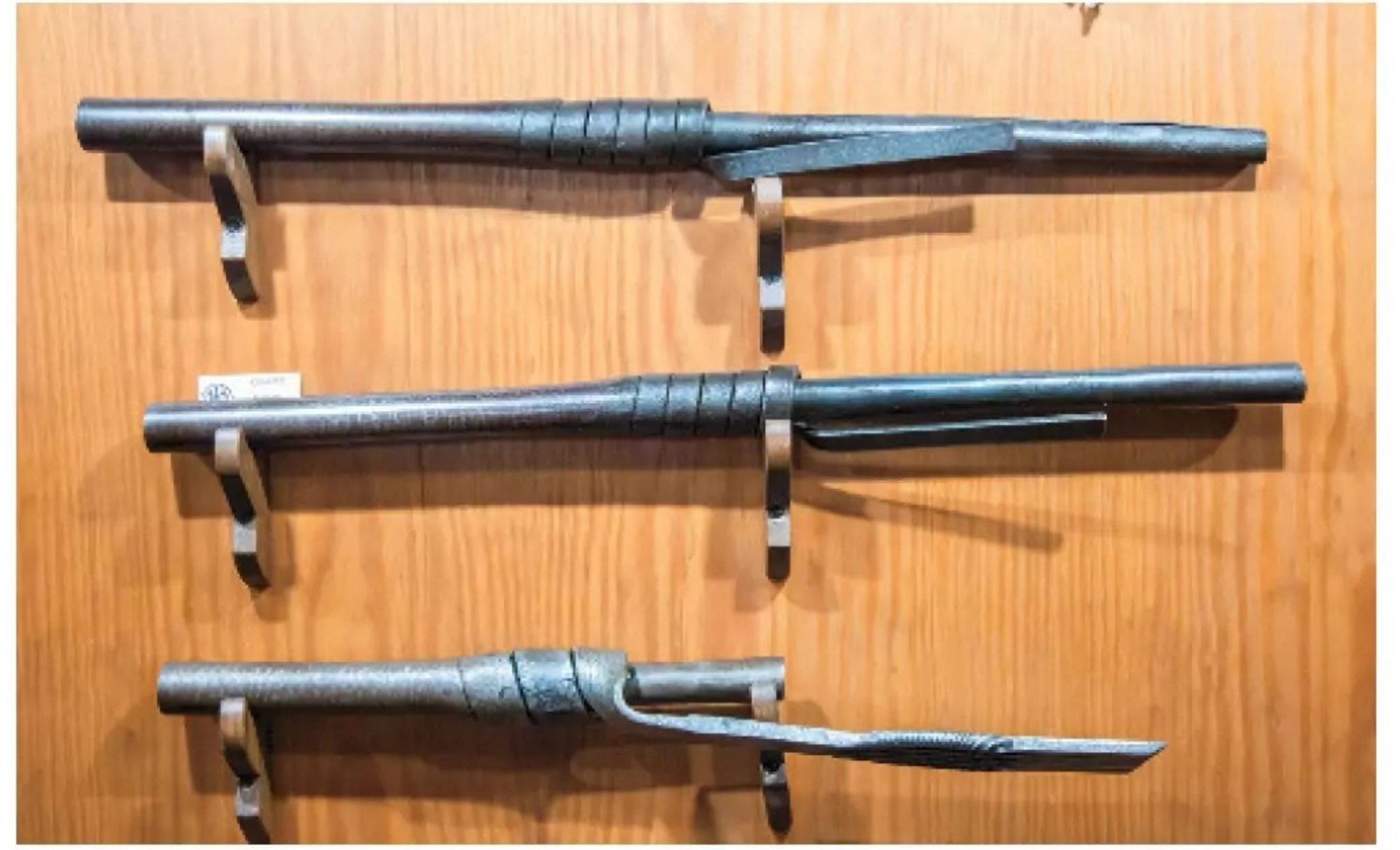
Samples of Damascus steel barrels were on display to illustrate a barrel making method during the blackpowder era.
