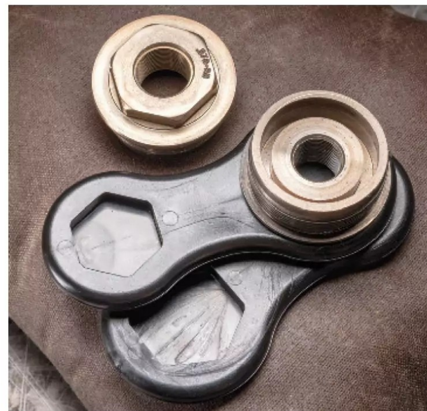
Each molded polymer wrench features sockets to accommodate two endcap sizes, 13/16 and 1-inch.
