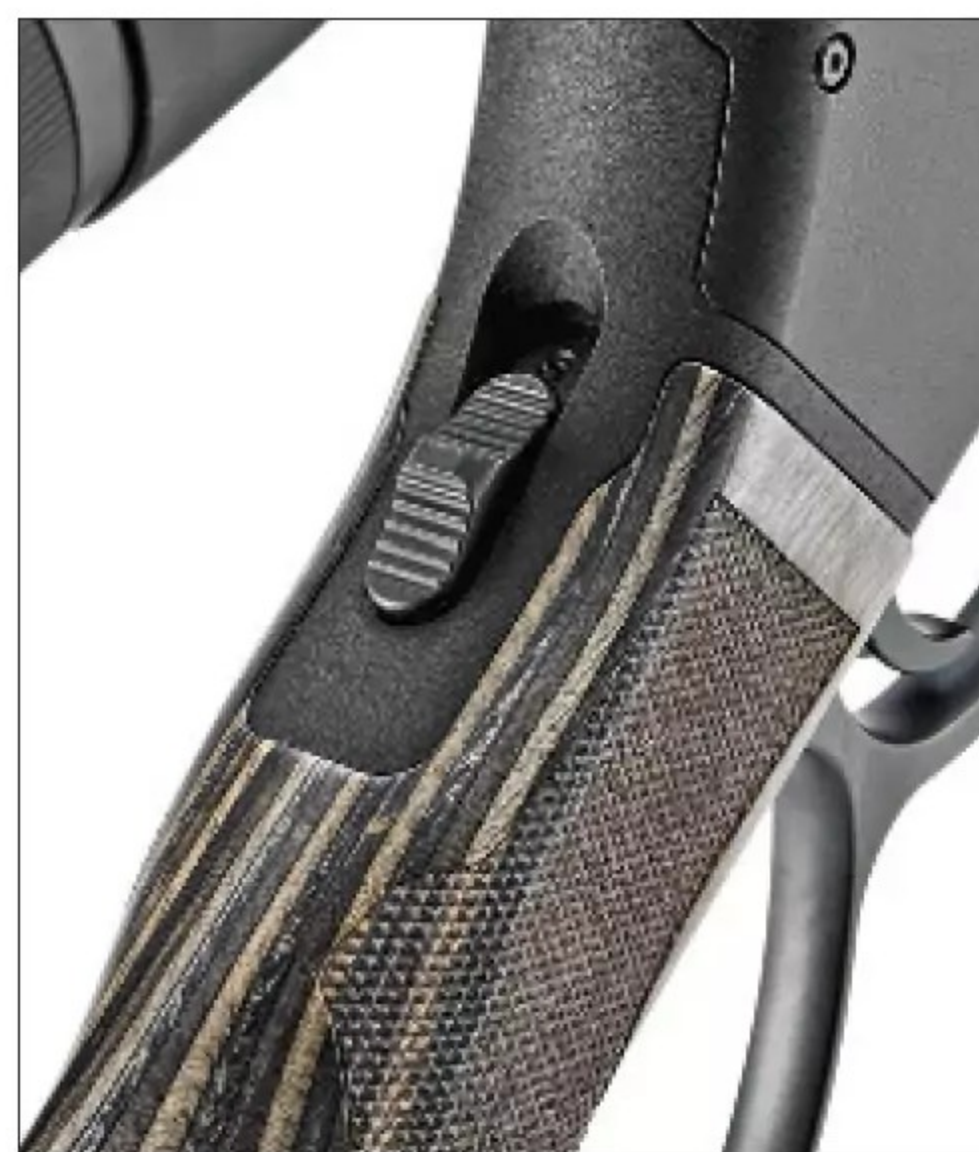
Push the tang-mounted thumb safety switch forward to fire, revealing a red-dot indicator. It is serrated to be used in both directions.
