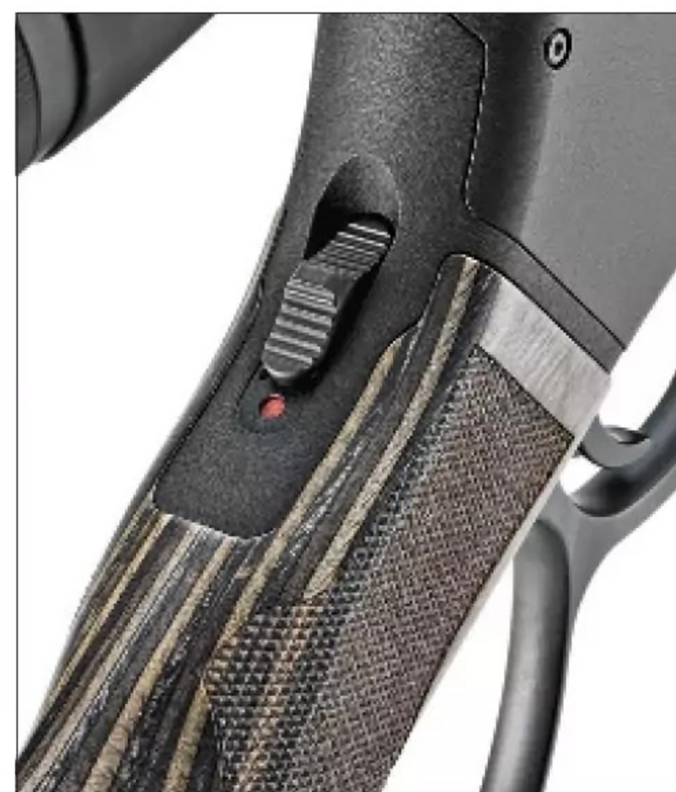
Push the tang-mounted thumb safety switch forward to fire, revealing a red-dot indicator. It is serrated to be used in both directions.
