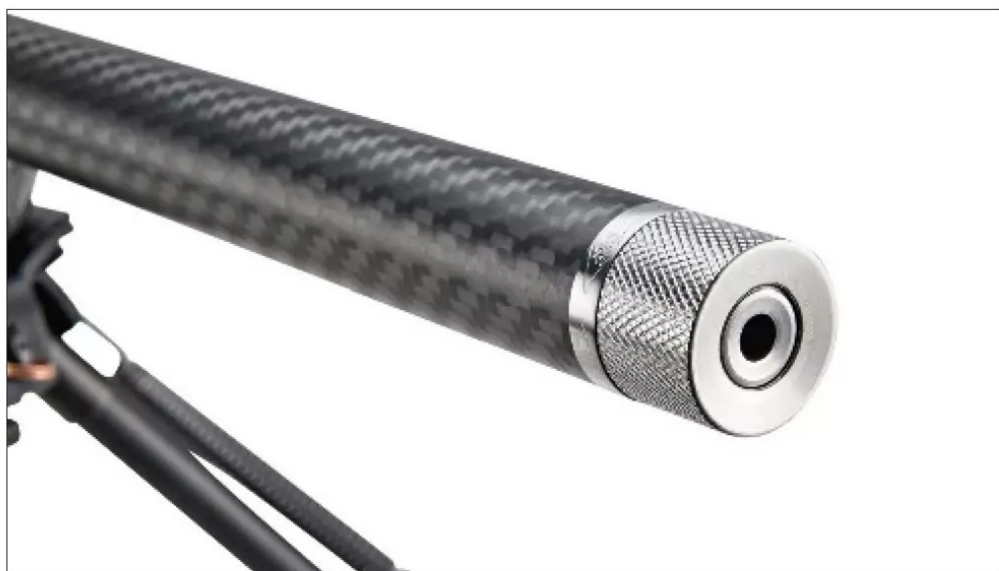
Under the knurled cap is a 1/2x28 threaded barrel that accepts muzzle devices, and lever actions are excellent suppressor hosts.
