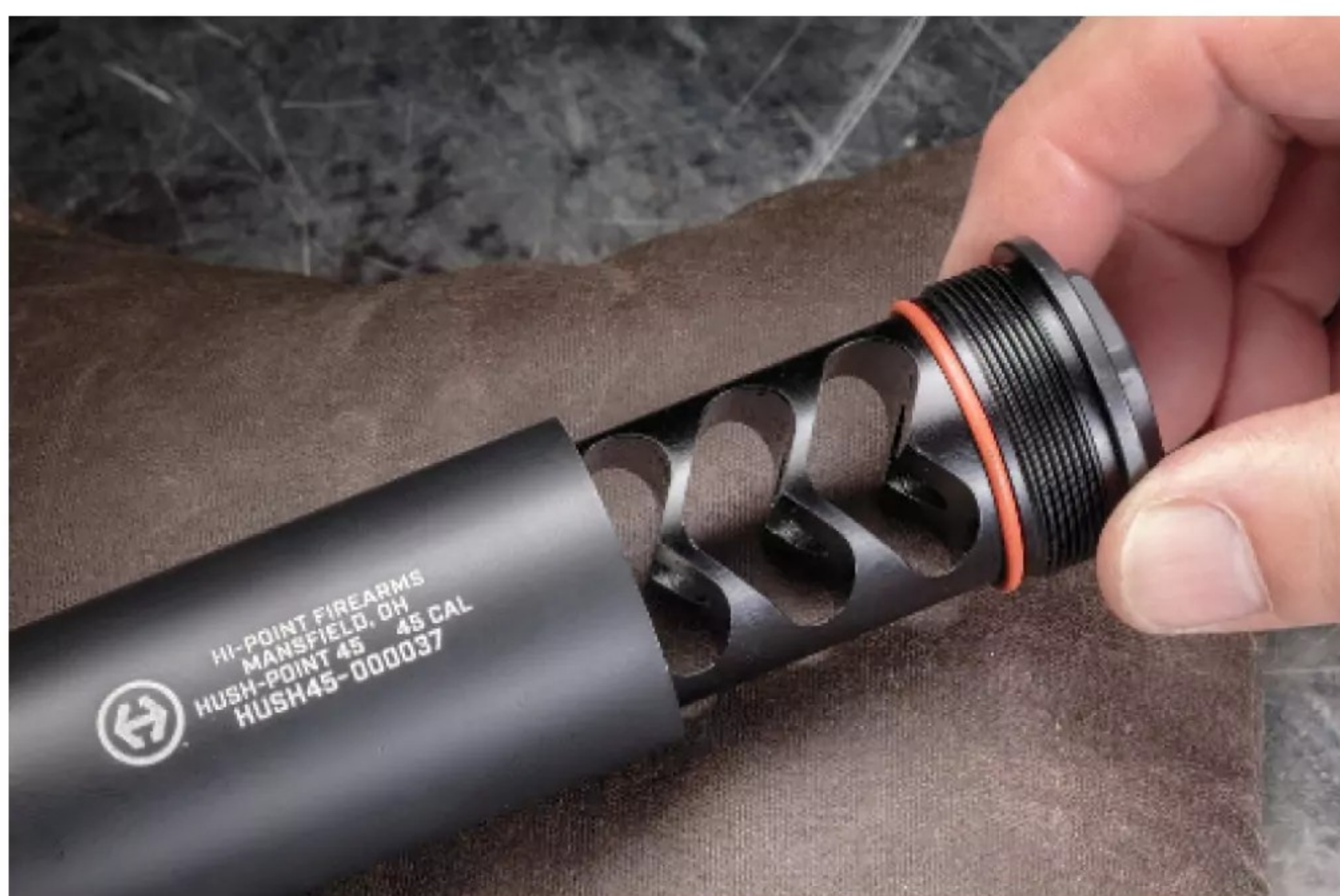
Unscrewing the muzzle allows the monocoire baffle design to be removed, providing access to the ports for maintenance or replacement of the orange O-ring.
