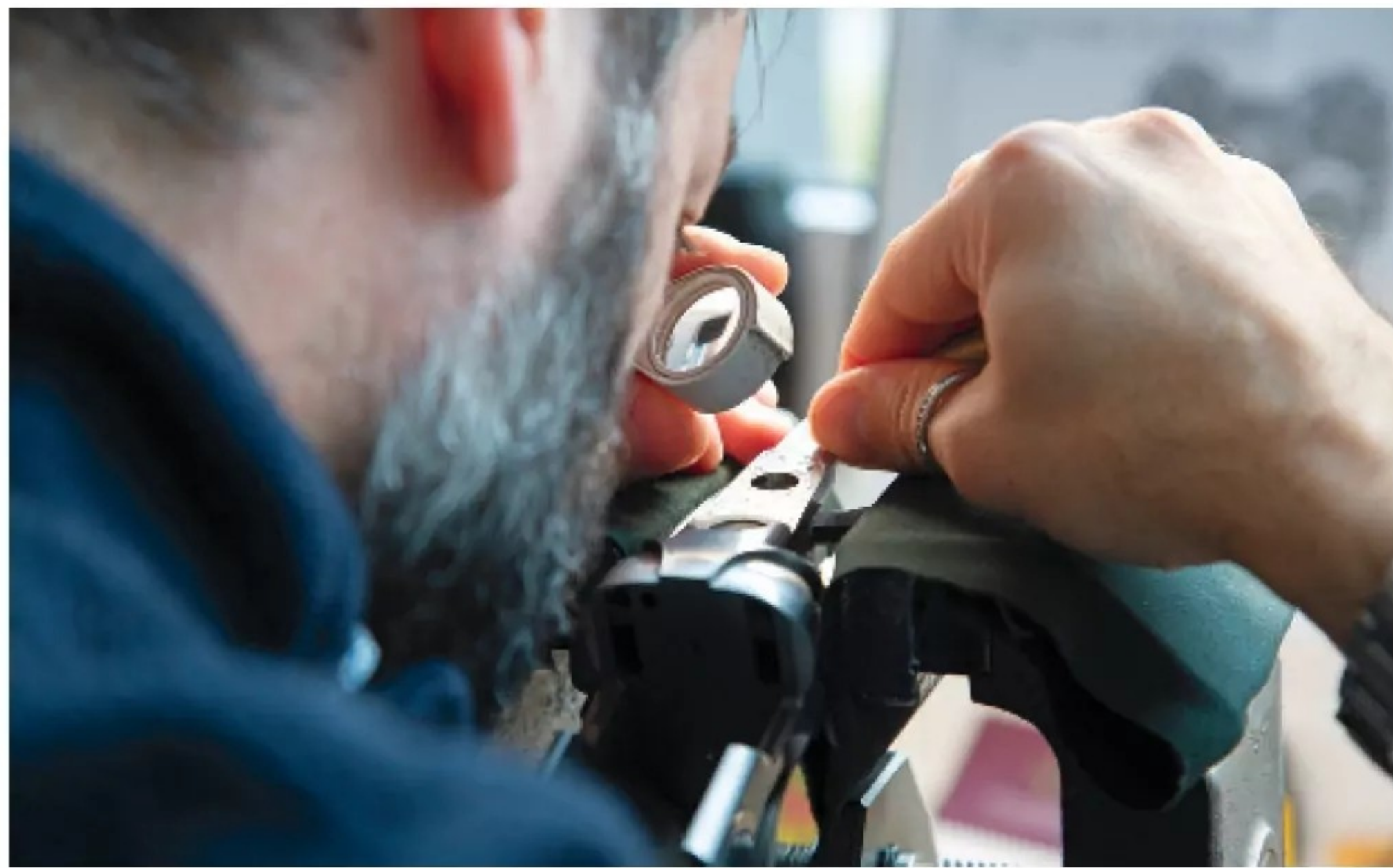
An artisan engraves the tang of a Beretta shotgun under the magnification of a handheld loop.
