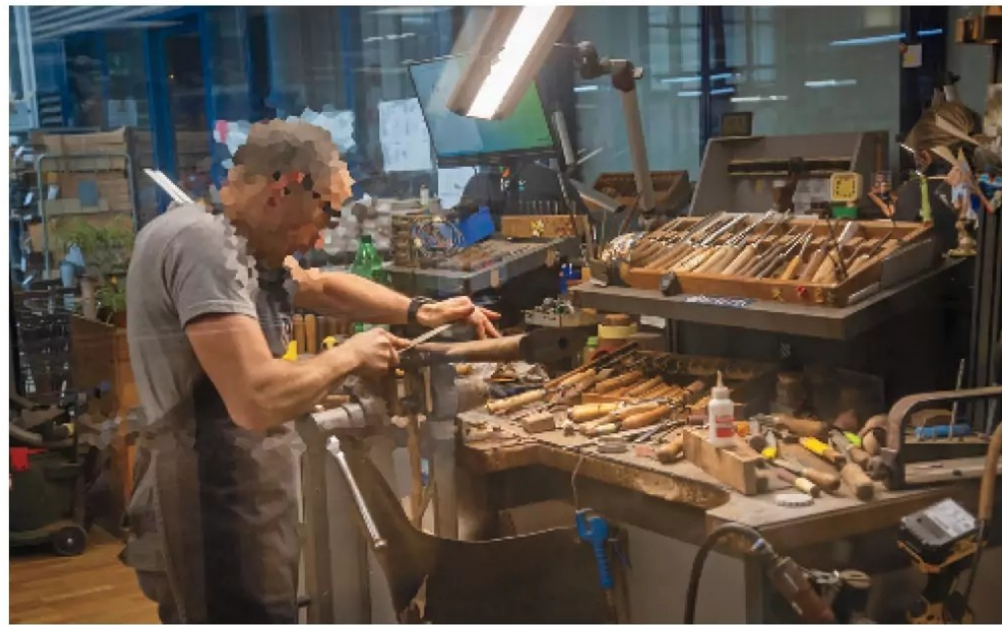
A Beretta Custom Shop craftsman uses a file to blend a high-grade walnut stock to a shotgun receiver.
