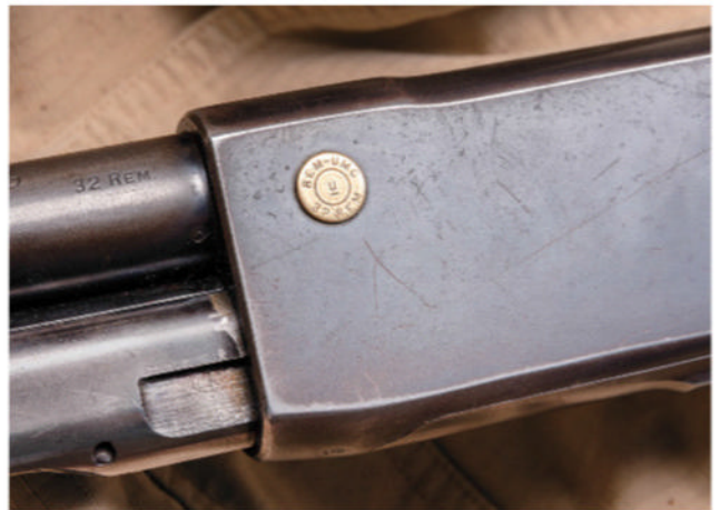
A simulated cartridge case head pressed into the side of the receiver served as an attractive, visual aid to identify the chamber.
