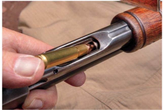
Blunt flat-point bullets did not turn the corner and load into G&A's Model 14 magazine tube. Only the Speer .321-inch, 170-grain flat-point would feed into the tubular magazine of the test rifle.
