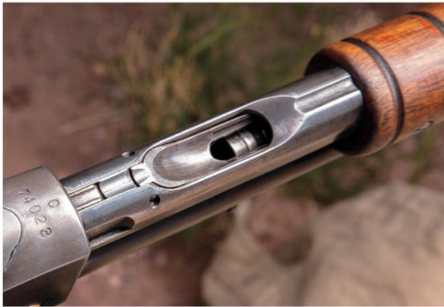
Like a shotgun, the Model 14 loading gate is underneath the magazine tube. The follower is visible through the port on the gate. Feeding the first is tricky, but subsequent rounds are easy to load.
