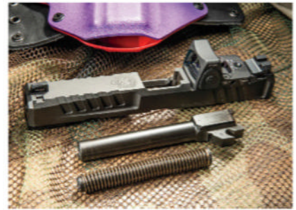
Fieldstripping the Echelon doesn't require pressing the trigger.
