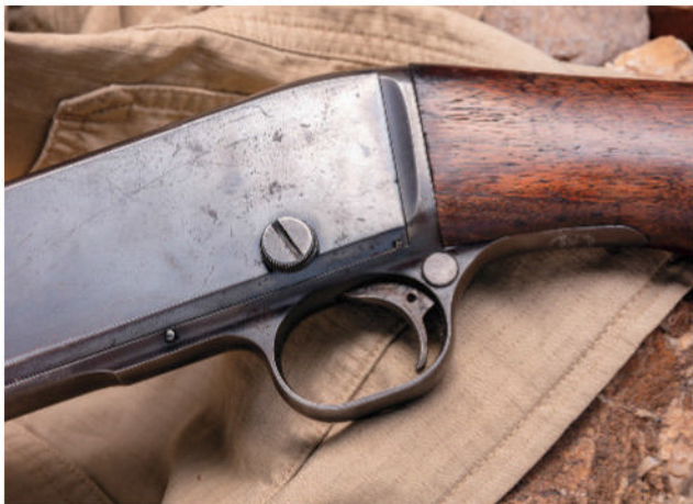
The knurled and slotted takedown screw is on the left side of the receiver. A safety filler plug is visible on the triggerguard.
