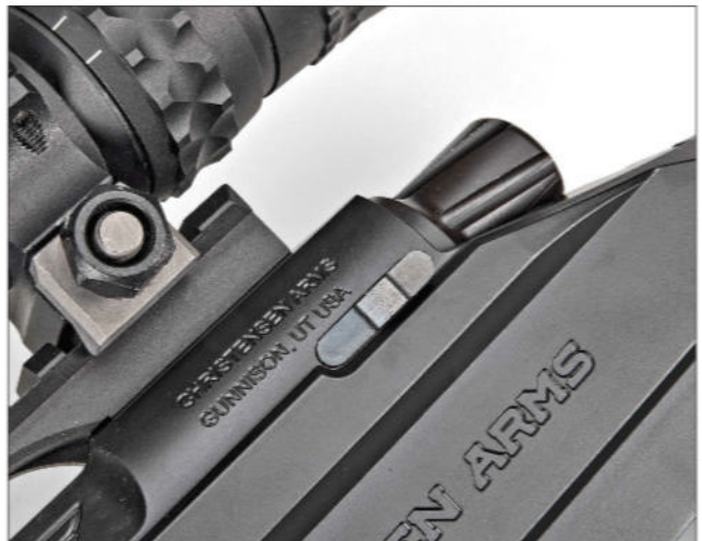
As with most Model 700-pattern actions, the bolt-release button lever is located at the left-rear of the action. It is low profile and easy to operate with the bolt to the rear.
