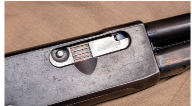
The button behind the safety unlocks the action, allowing the gun to be unloaded. The receiver was scalloped to ease safety access.
