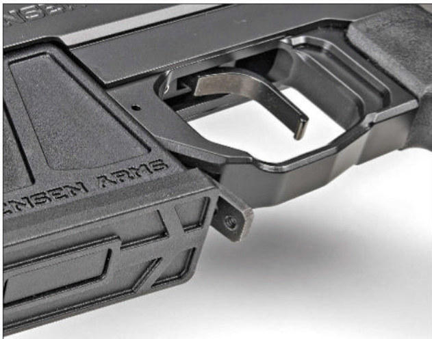
The ambidextrous magazine release lever is at the front of the triggerguard, just behind the rear of the magazine's basepad. Push the lever forward to release the AICS-pattern magazine.
