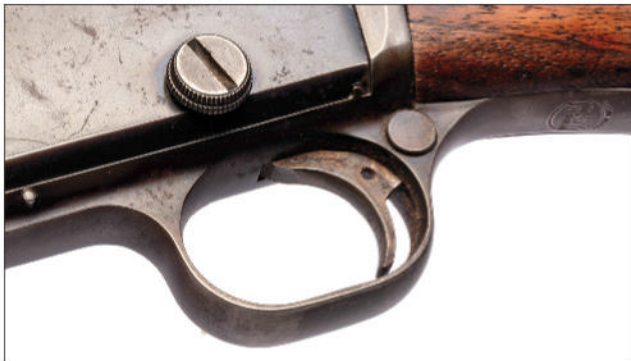
The steel triggerguard was blued, while the trigger was case hardened. The trigger on G&A's rifle averaged 6 pounds, 10 ounces.
