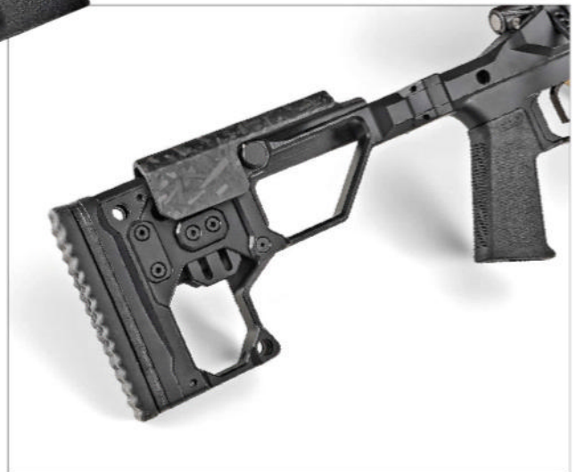
The folding stock is convenient for storage and travel. Length of pull and comb height are adjustable, and the stock features QD mounting points for slings. The flat toe rides rear bags for stability.
