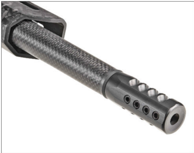
The hand-lapped, button-rifled, carbon-fiber-wrapped barrel is free floating. The MPR includes a stainless-steel muzzlebrake. Removing any combination of hex screws can further tune the device.
