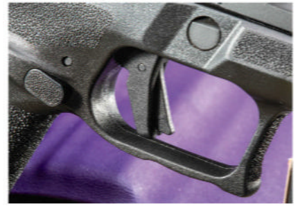
The trigger safety lever bisects the flat-face polymer trigger.
