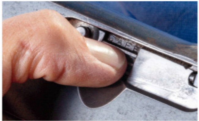
The sliding bolt safety switch on a Model 14 bolt is a less-common feature. A shooter can use their right-hand thumb to push it down to engage the safety, revealing the word “SAFE” (above, right). The switch blocked both the firing pin and trigger.
