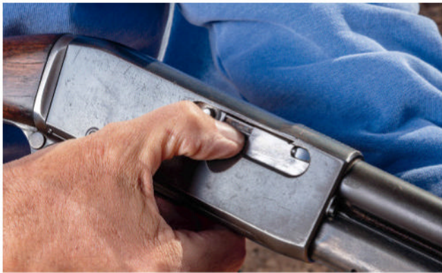
The sliding bolt safety switch on a Model 14 bolt is a less-common feature. A shooter can use their right-hand thumb to push it down to engage the safety, revealing the word “SAFE” (above, right). The switch blocked both the firing pin and trigger.
