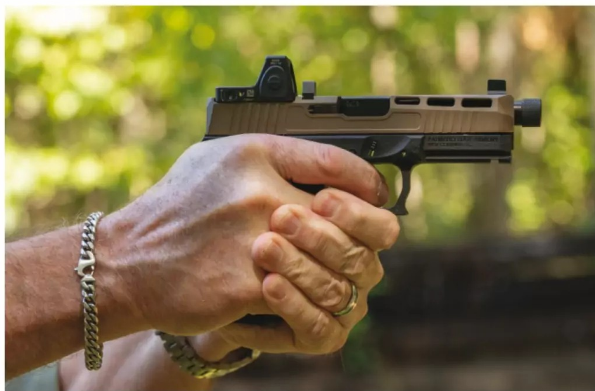
The version of the PSA Dagger that was tested comes with a capped and threaded muzzle—1/2x28—for suppressor use.
