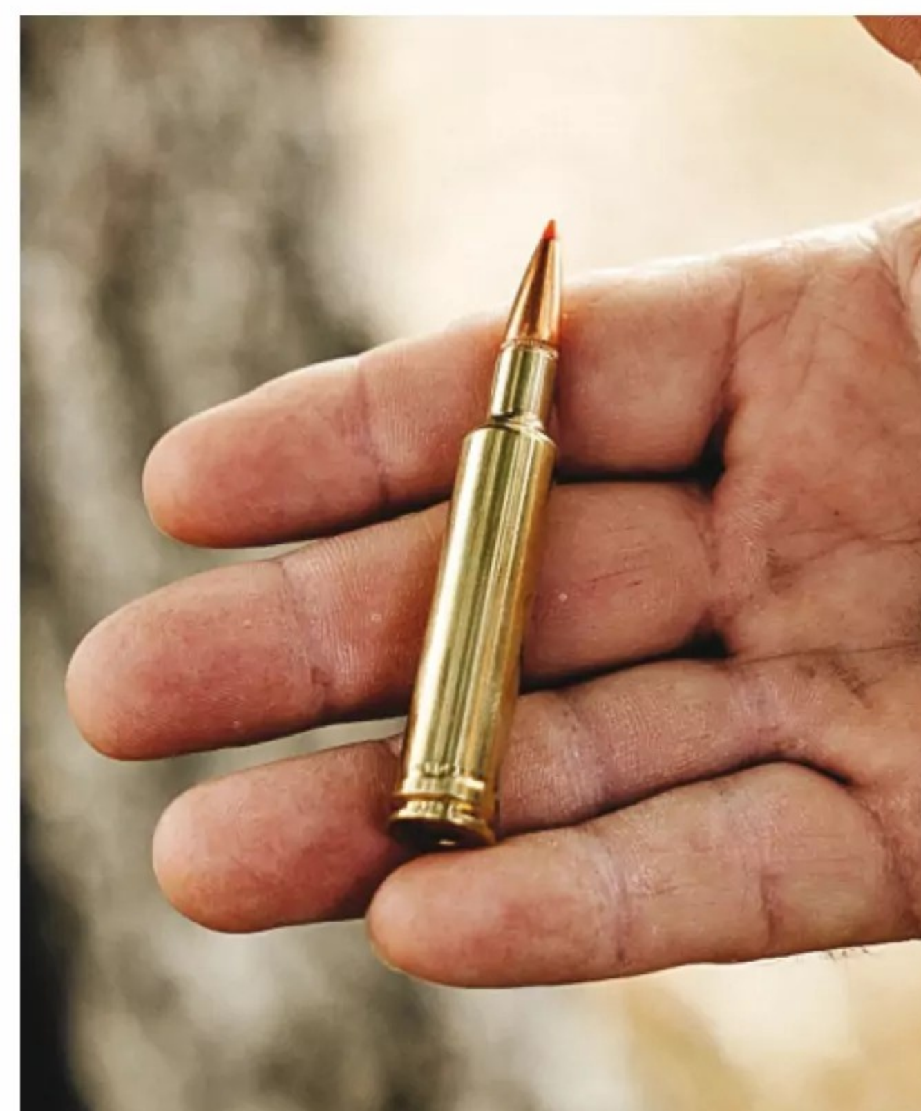
7mm Weatherby cartridge the author reloaded with Hornady brass, Hornady 154-grain SST bullet and IMR 4350 powder ignited by a Remington 9½ M primer.
