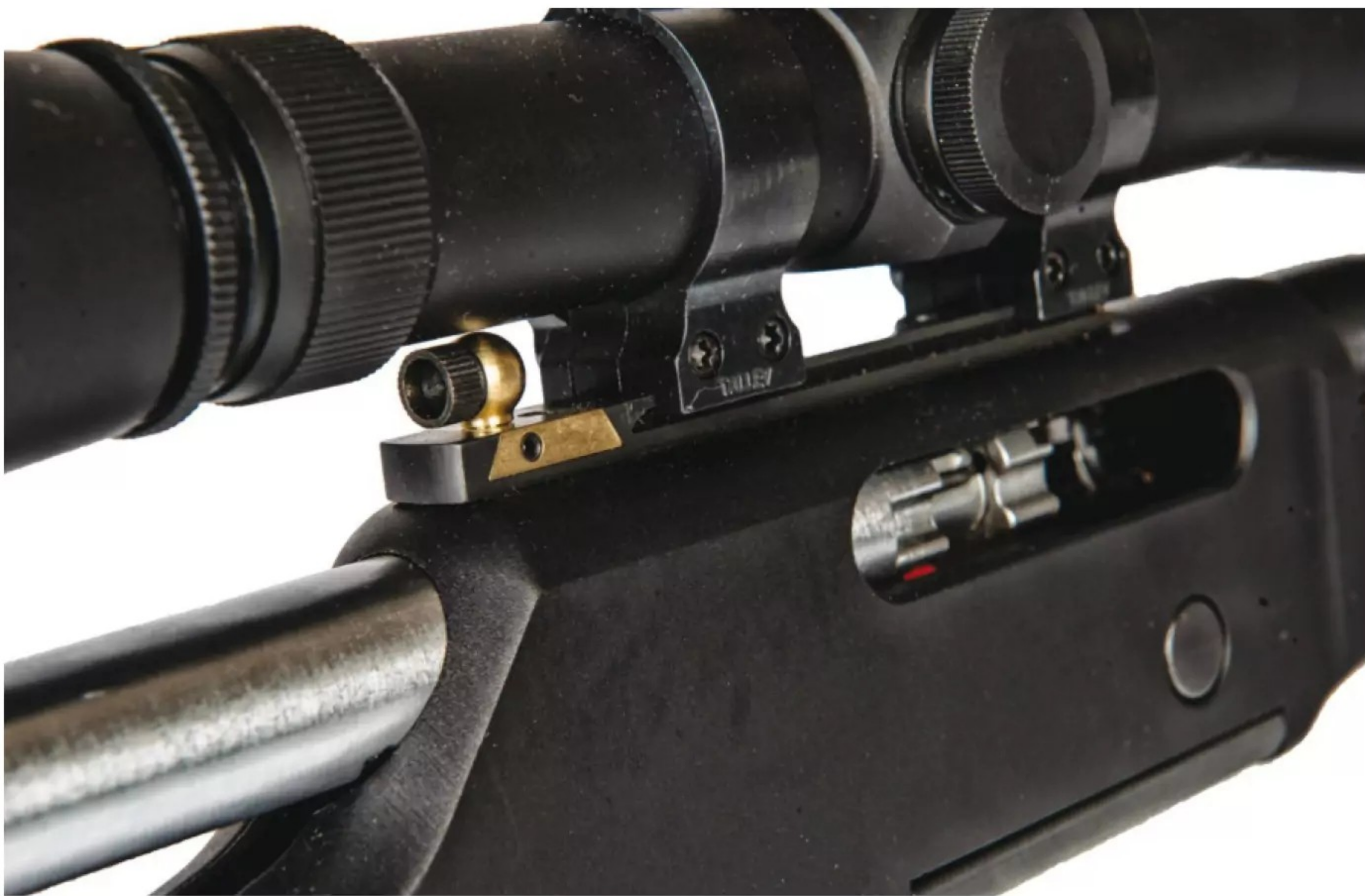
The author's Henry Long Ranger uses Talley Quick-Detach Rings, which enabled him to choose either the Skinner Sights peep system or the Leupold VX3i 4.5-14x40mm riflescope.
