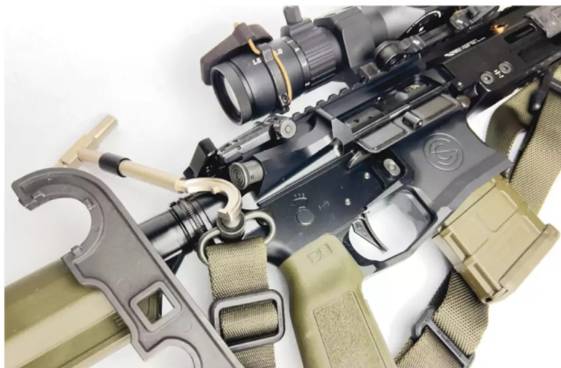
Tightening castle nuts can be done with small tools as well as big ones ... although it is far easier to damage parts with more leverage.
