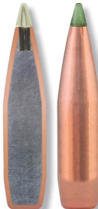
The Speer Impact's jacket is chemically fused to the lead core to prevent separation on impact, while the Slipstream tip promotes expansion.
