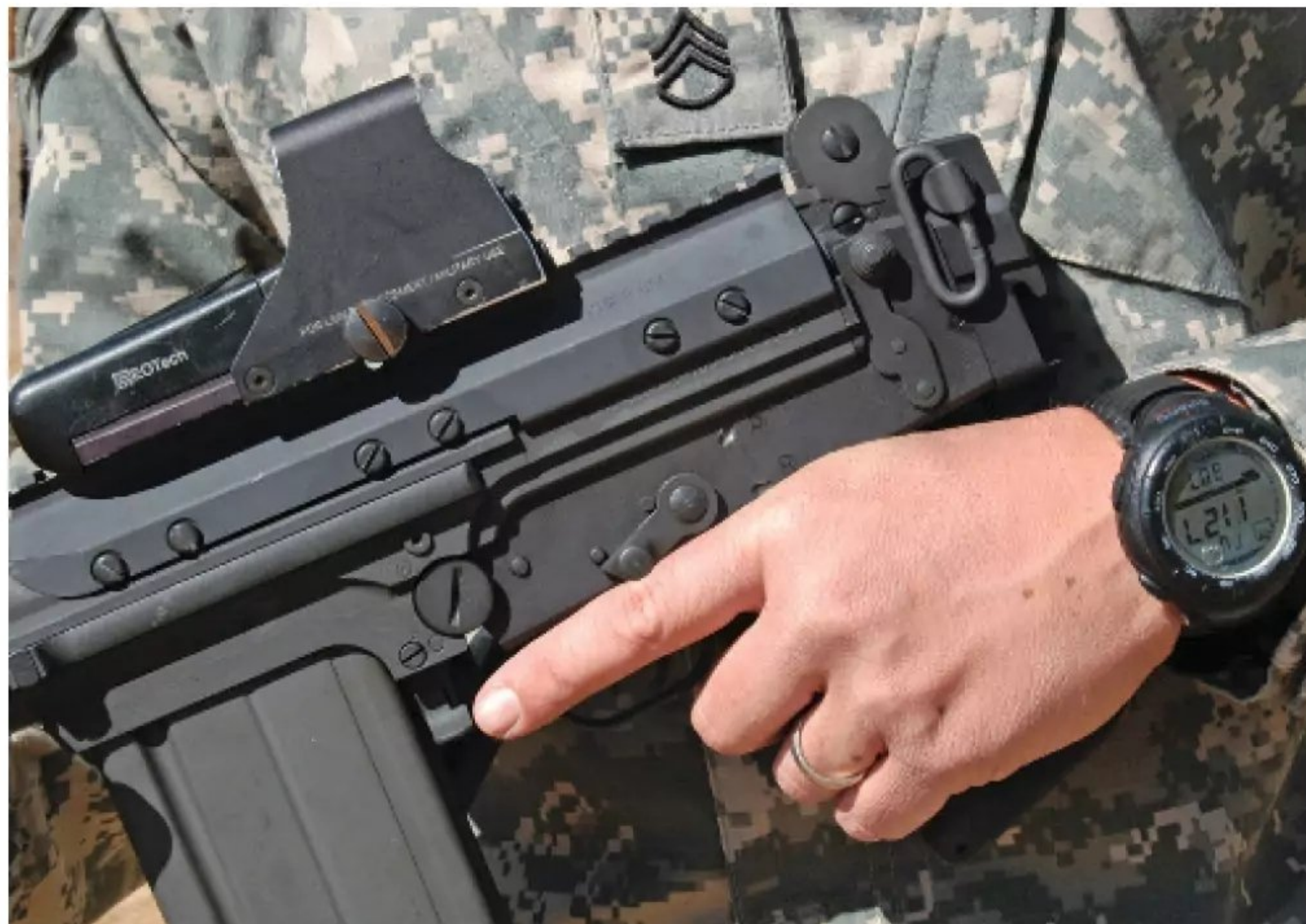
Controls are straight FAL and easy to manipulate. Note it takes a conscious decision to rotate the selector to the full auto position as seen here.
