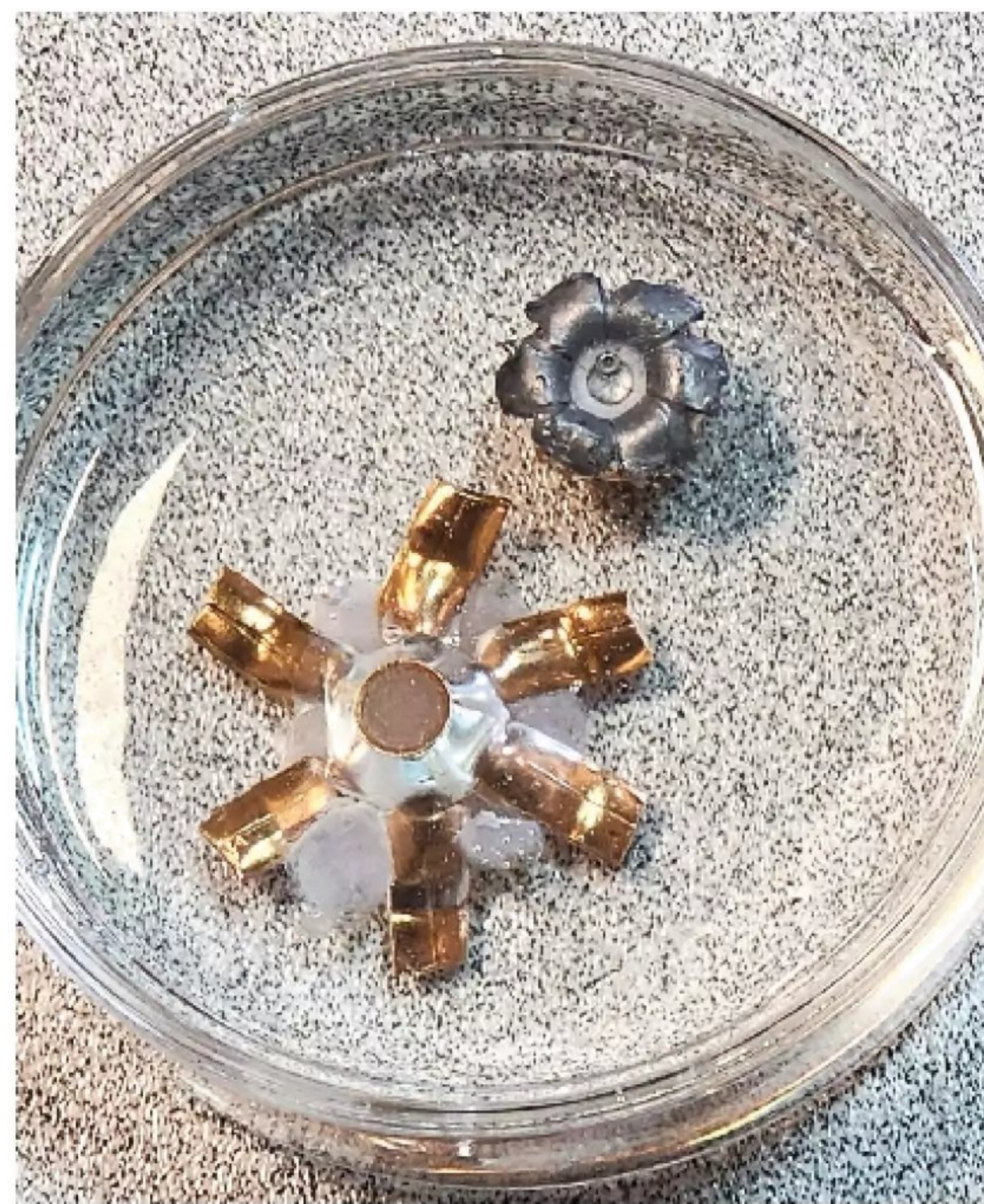
An expanded SIM-X DefenseCore bullet on the bottom, compared to a traditional JHP with a lead core. They perform very differently upon impact.
