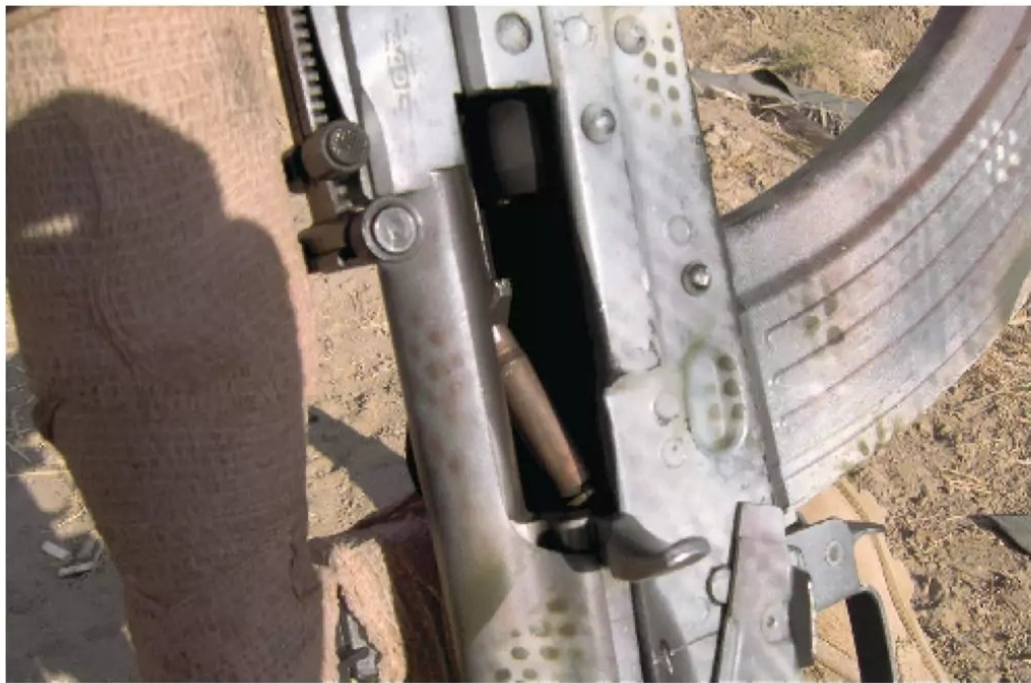
Reliability was not 100% during testing probably due to the poor quality of available ammunition. Also note the RPK style rear sight. (Photo by LTC Kendrick McCormick)
