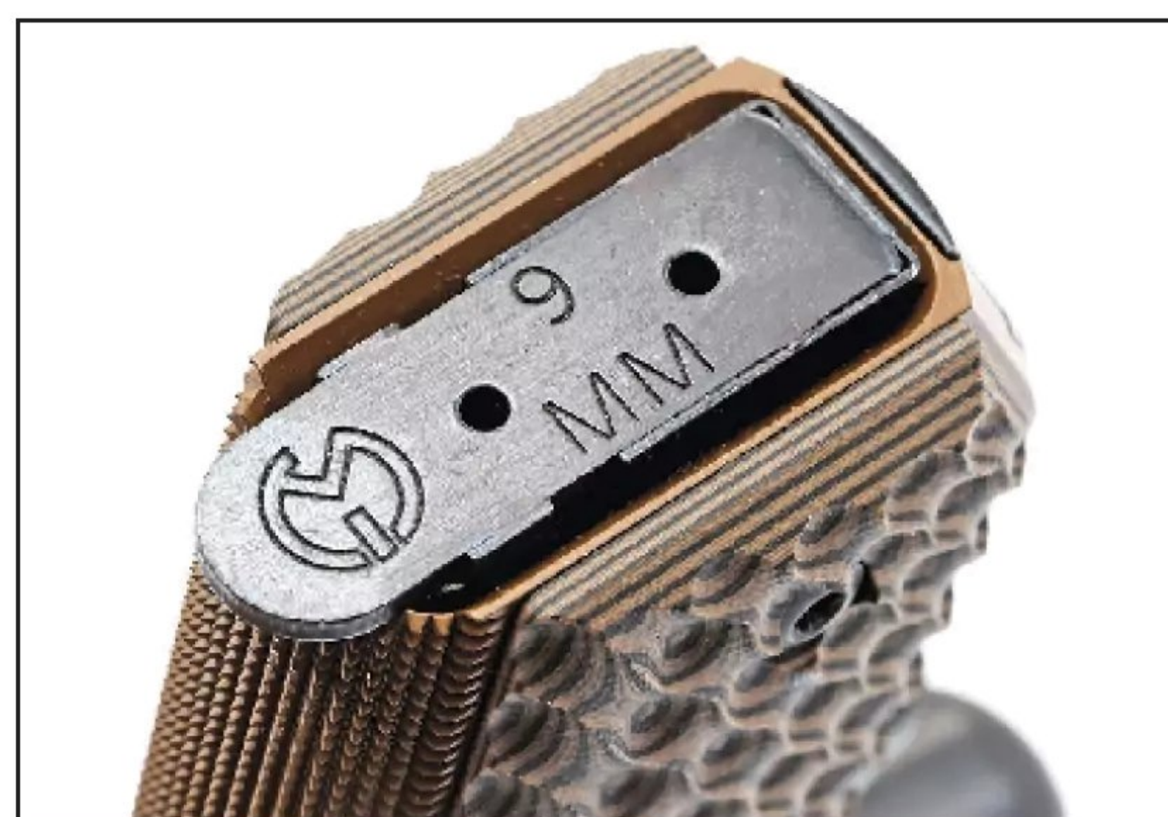
The TRP CC has the magazine well beveled a bit, as much as it can be. It comes with three magazines, and they are already drilled for bolting on a magazine base.
