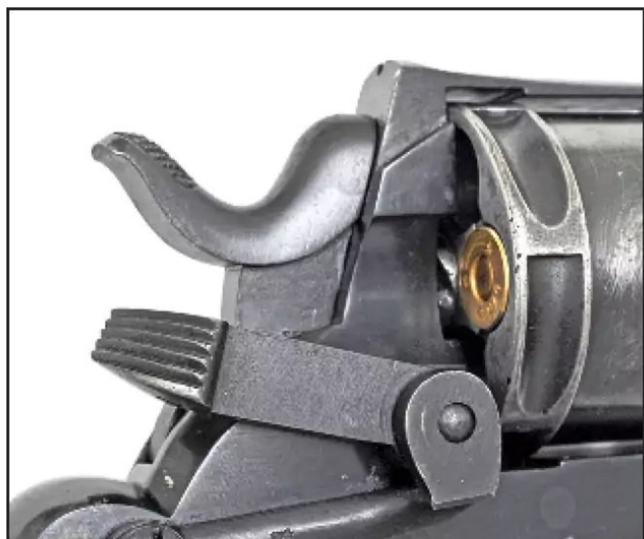
The loading gate was rotated to the rear to load or unload the revolver.
