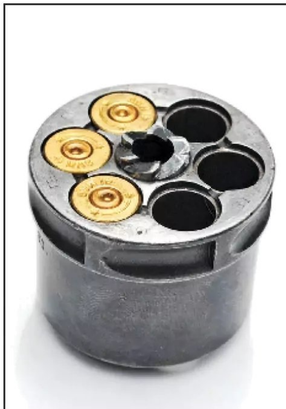
The cylinder had thick walls and recessed chamber mouths for full support of the cartridge head.
