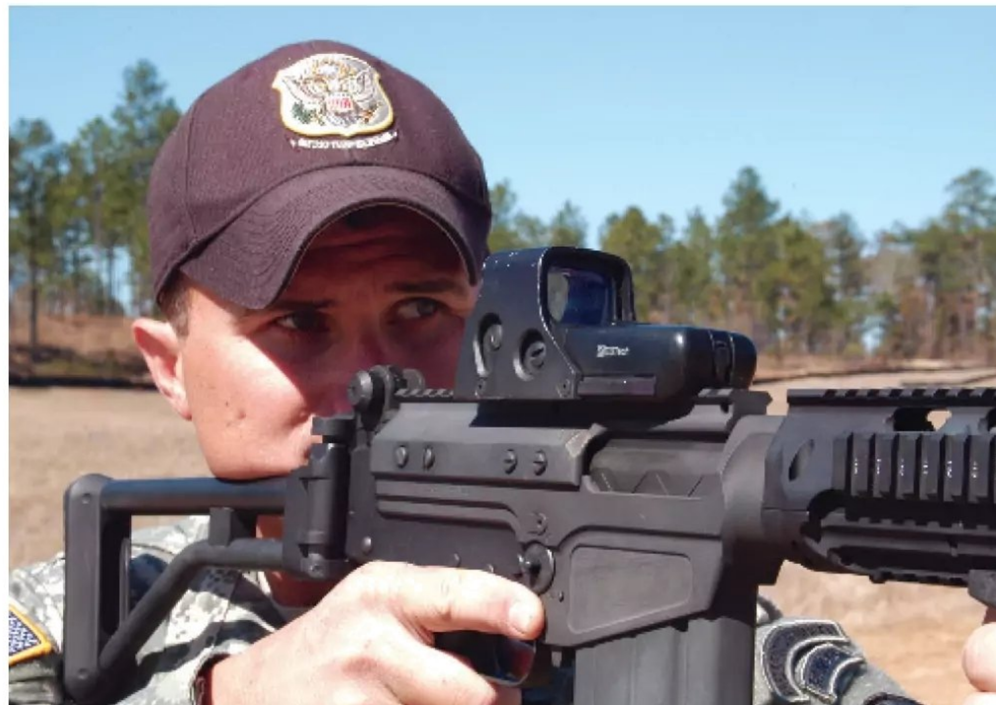
The OSW's top cover sports a MIL-STD 1913 rail to allow a variety of optical sights, such as this EOTech, to be easily mounted.
