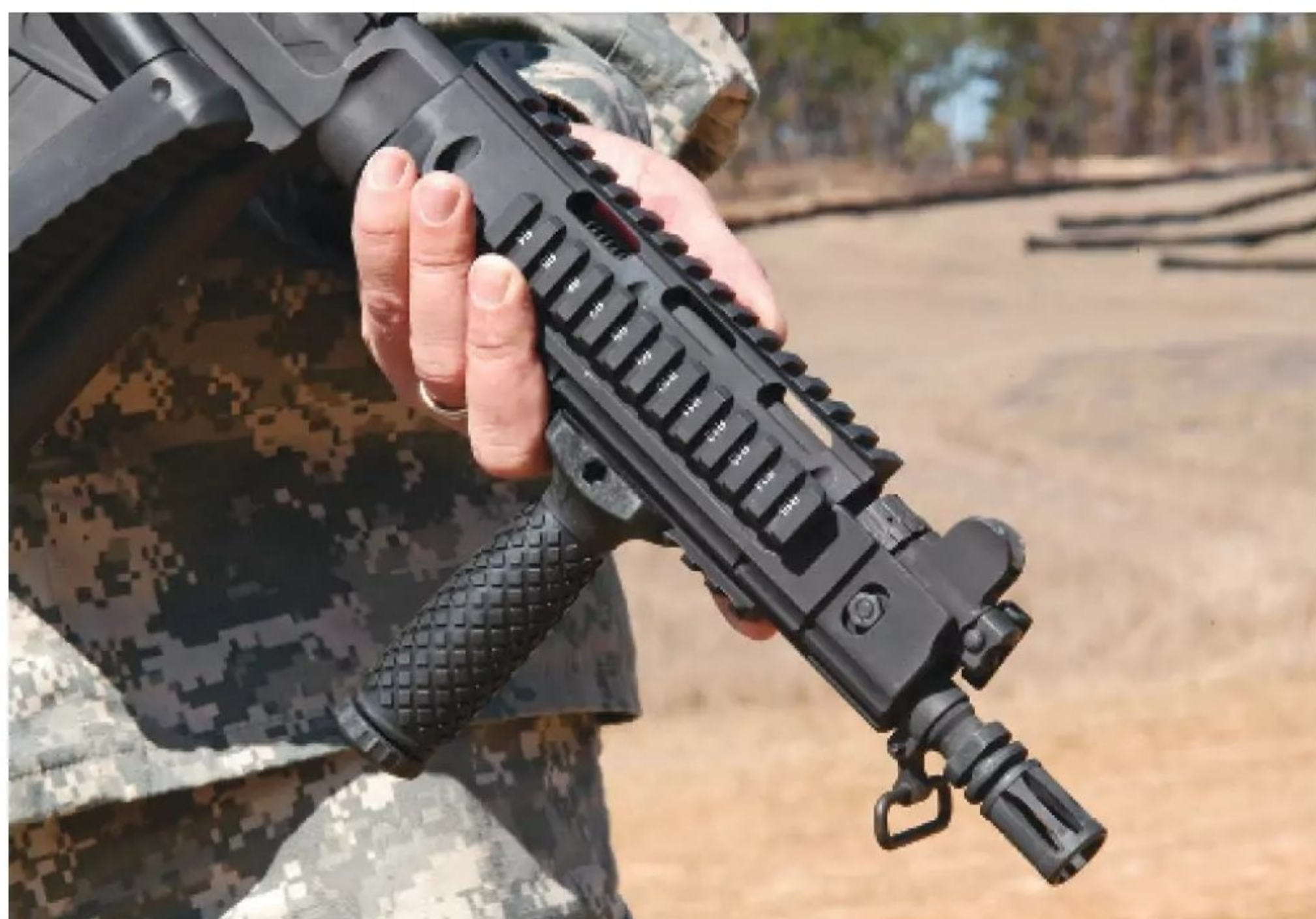
To allow accessories to be easily mounted to the weapon the aluminum fore-end features MIL-STD 1913 rails.
