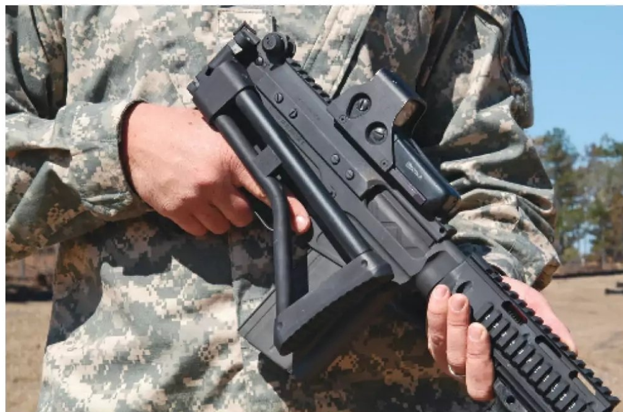
The OSW's stock folds neatly out of the way for storage drastically reducing the weapon's overall length. Downside? Length of pull is long for use with body armor.
