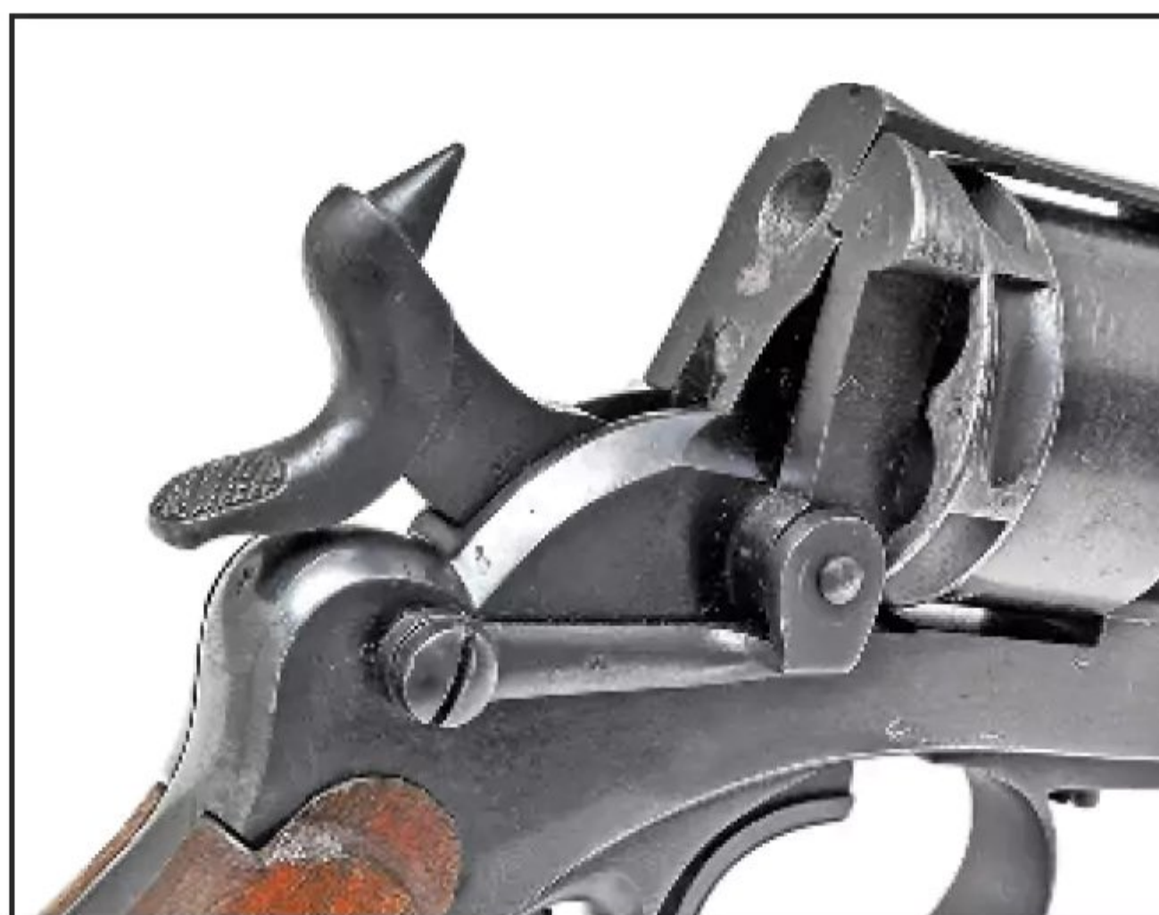
A rather massive hammer and heavy mainspring insured reliable cartridge ignition. Note the U notch rear sight.
