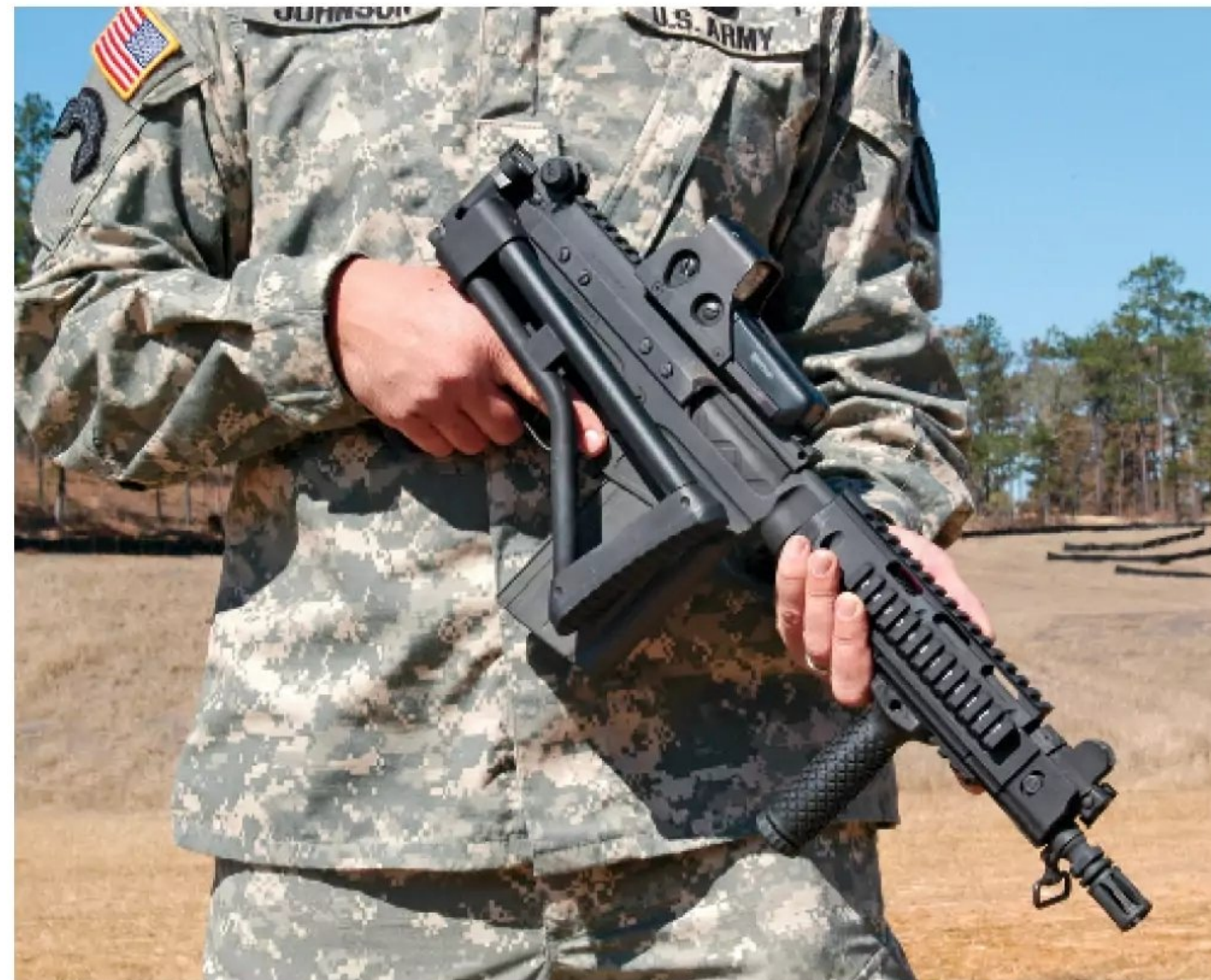
DSA's OSW is a very compact 7.62x51mm NATO carbine thanks to a stubby 11-inch barrel.
