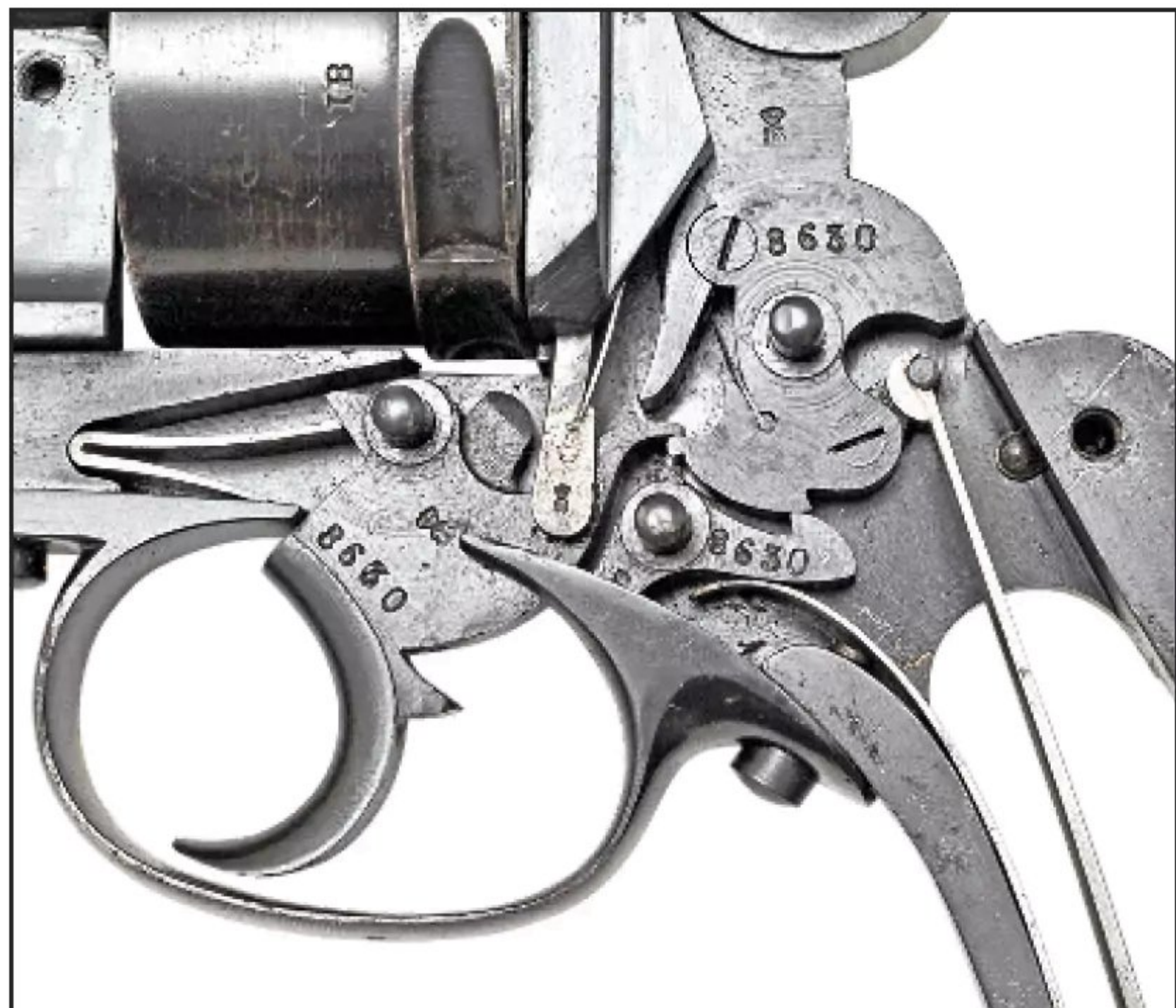
The left-hand side plate could be removed for cleaning or repairs. Note how just about every part is marked with the serial number.
