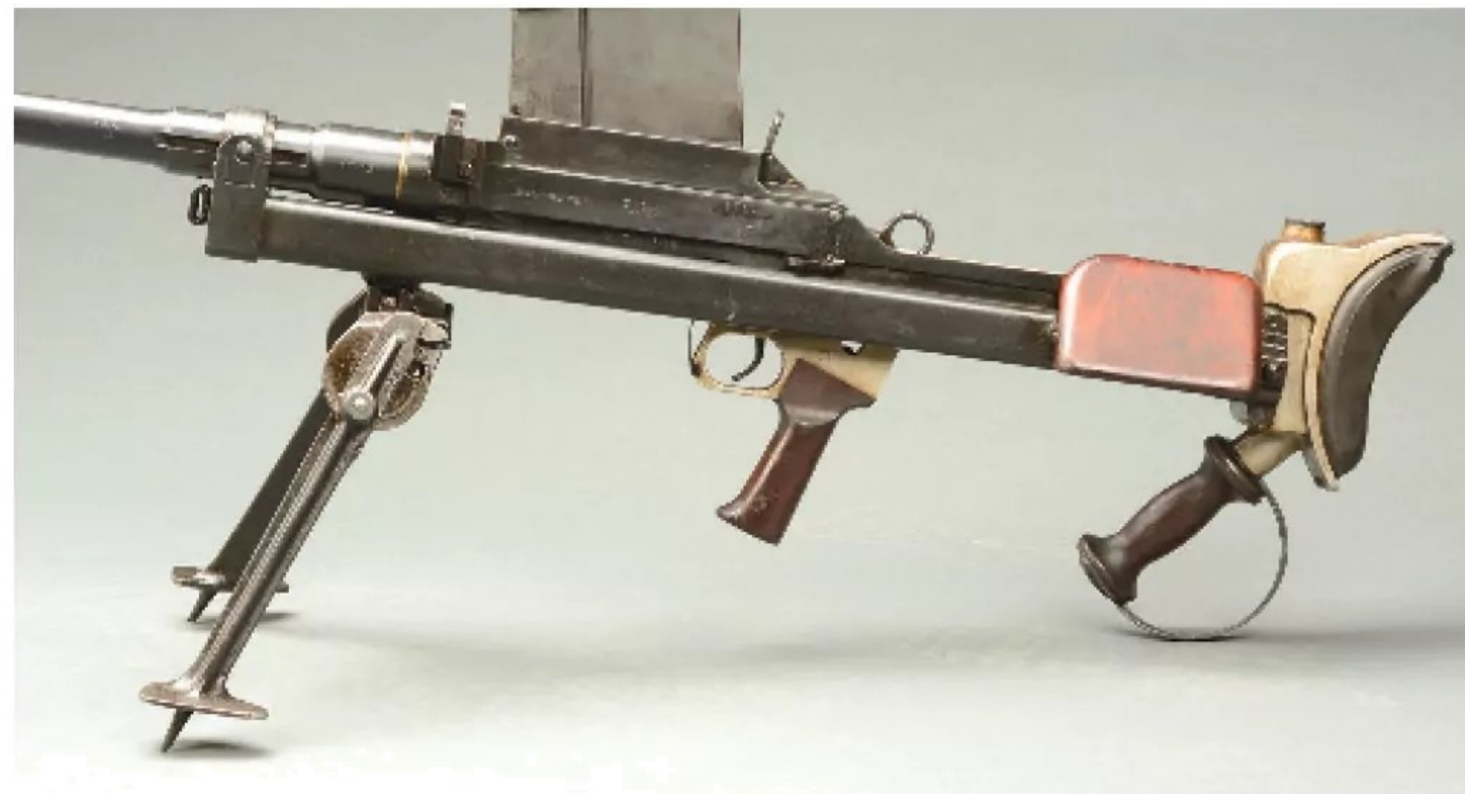
An Inglis-made Boys Mark I* rifle. Note the bipod, muzzle and rear sight. (Rock Island Auction Co.)
