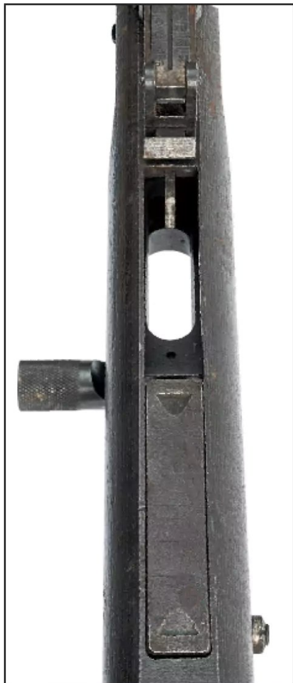
Centrally-located fixed ejector over the wide ejection port. (Oleg Volk)
