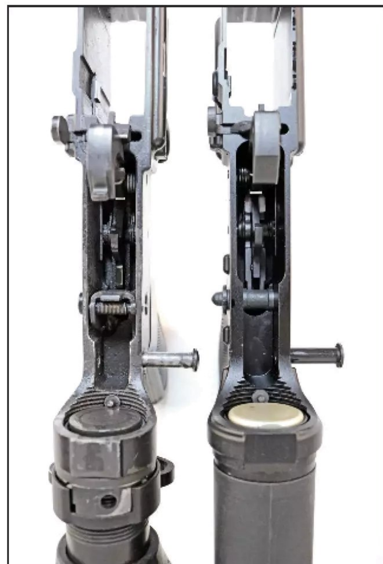
The M16 receiver (left) sports enough space in the rear for a GI auto sear along with the corresponding hole for the pin. Early AR-15s had space here, but manufacturers later added more material to block the insertion of full-auto sears in order to make ATF happy.
