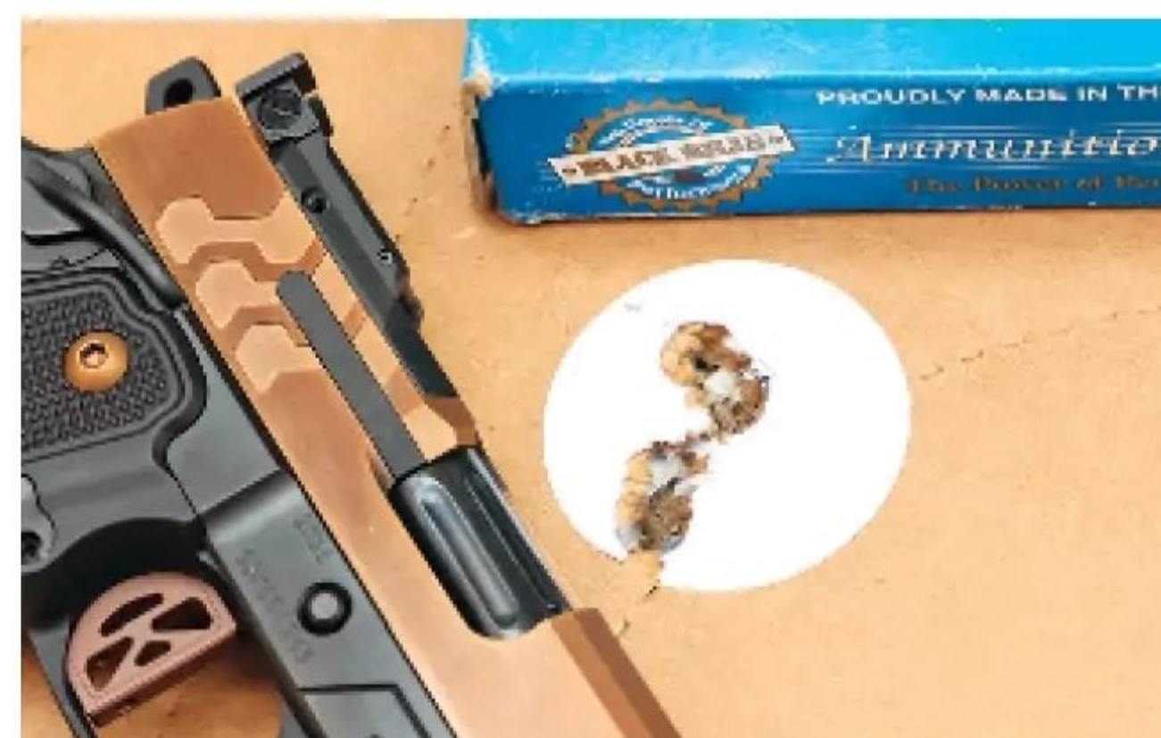
The rear sight is on the cover plate for the optics installation. Remove it to install the optics and you lose the rear sight.
