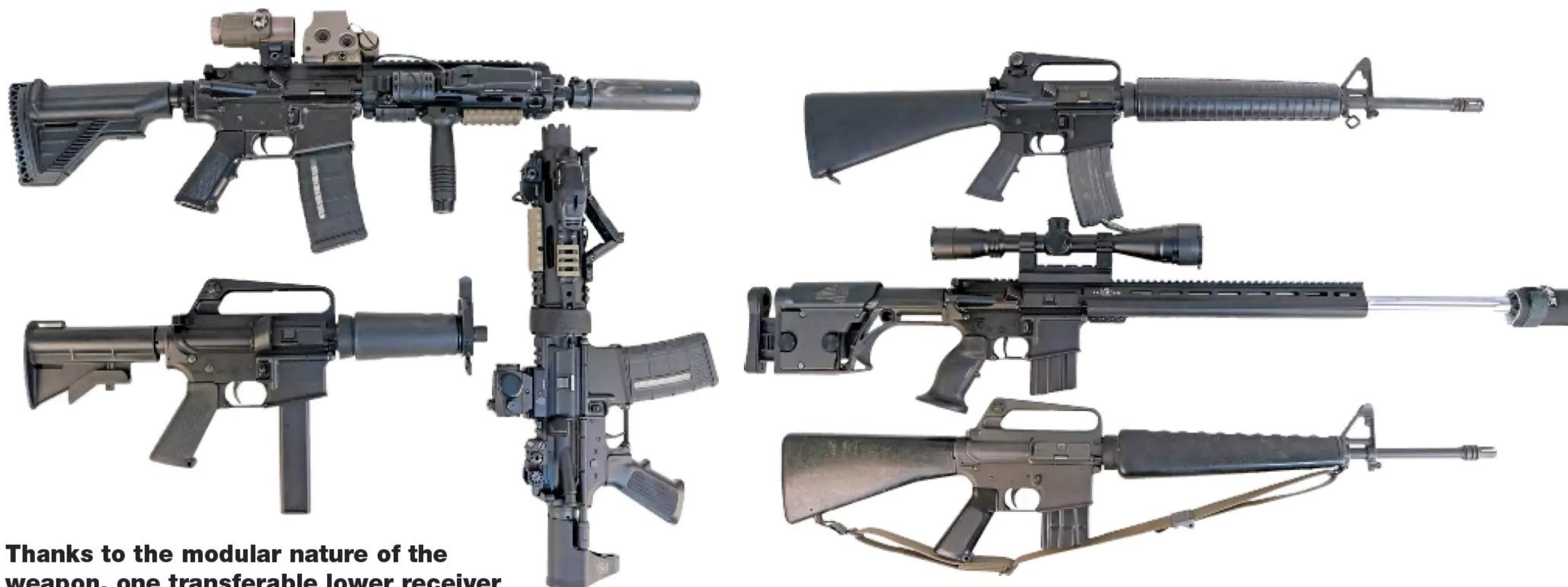
This HK416 parts kit rides on a transferable Wilson Arms M16 receiver Dabbs bought back in 1987. With the AR-15/M16 design, it is the lower receiver that is the actual gun. Everything else is fluff.
