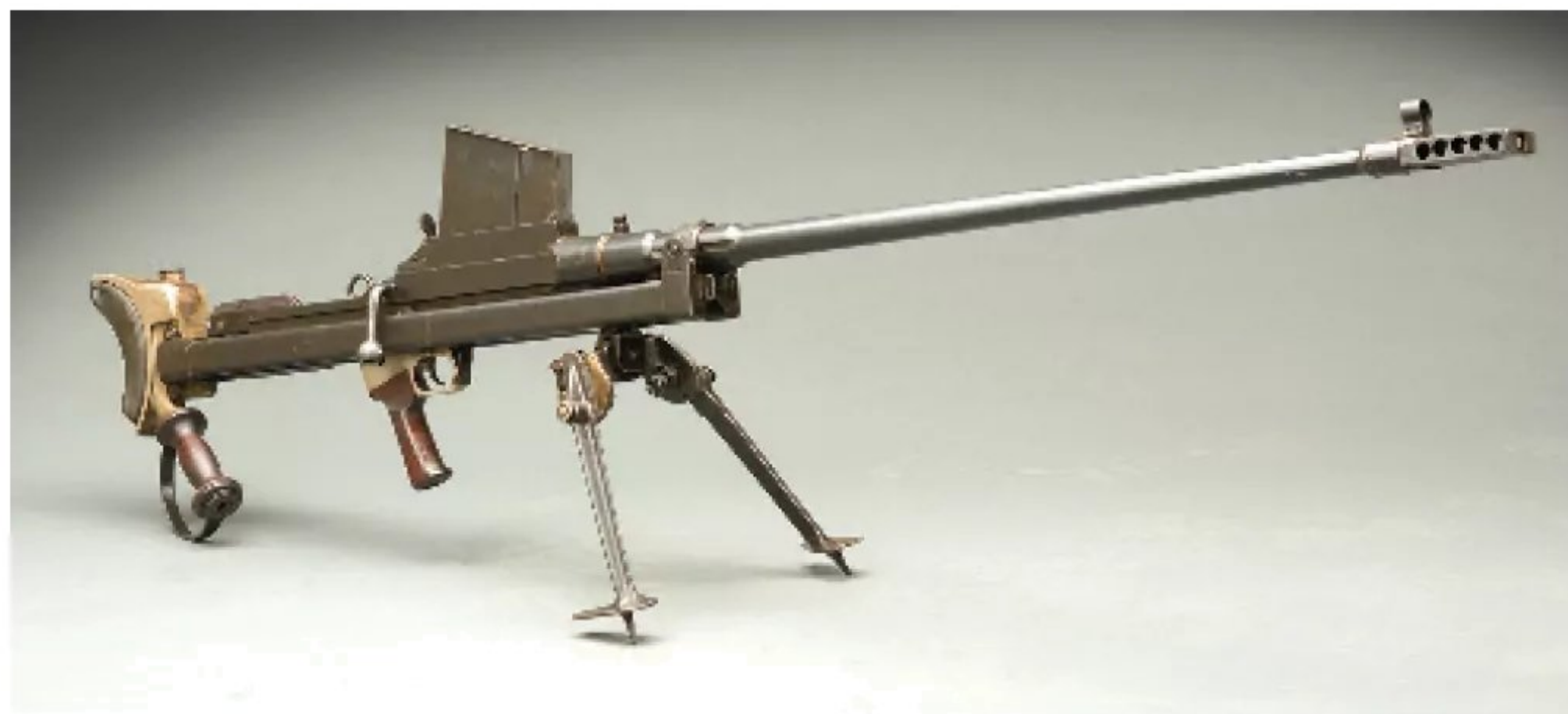
An Inglis-made Boys Mark I* rifle. Note the bipod, muzzle and rear sight. (Rock Island Auction Co.)
