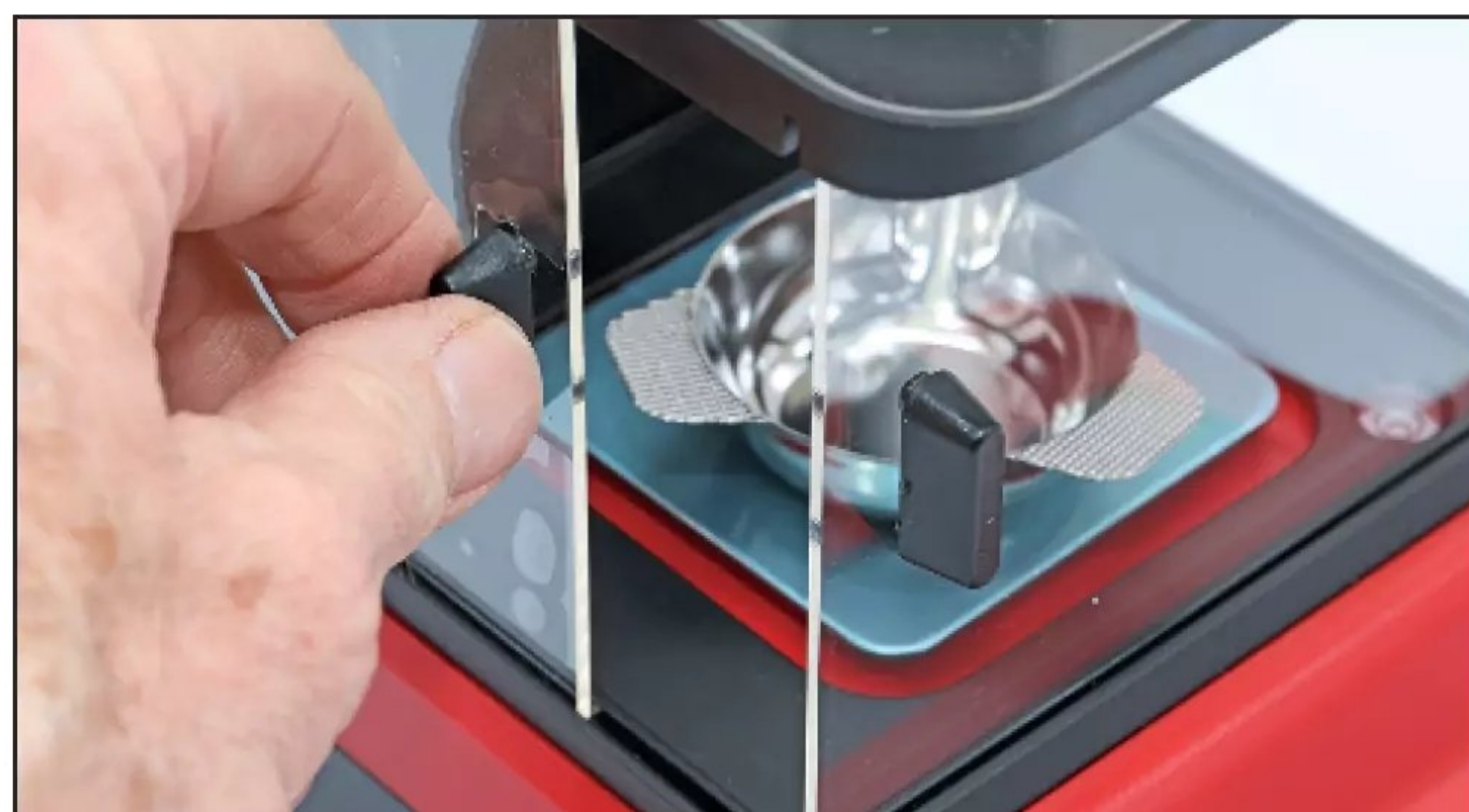
The enclosure has sliding doors so you can control breezes and keep dust out of the system.
