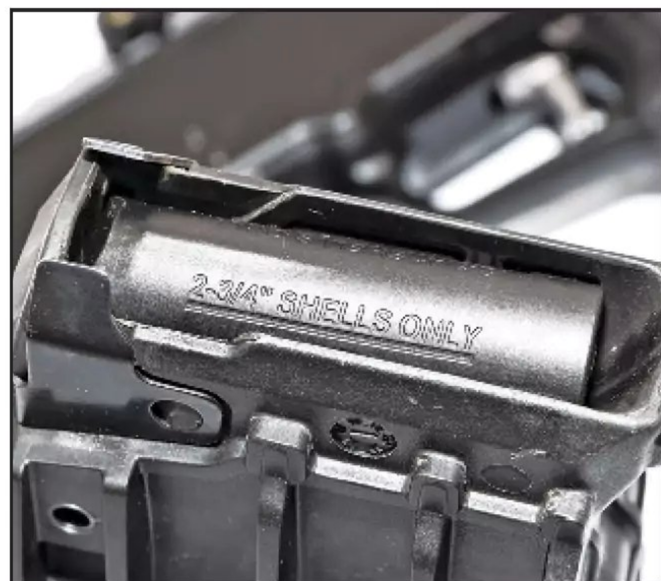
The magazine (and the 590RM) only accepts regular 12-gauge shells, not the magnums. Fine by me, I don't need three-inch magnums.
