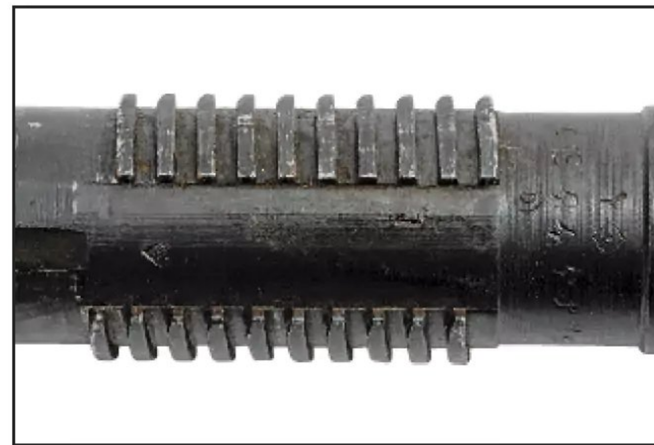
A long interrupted thread ensures consistent barrel positioning. (Oleg Volk)
