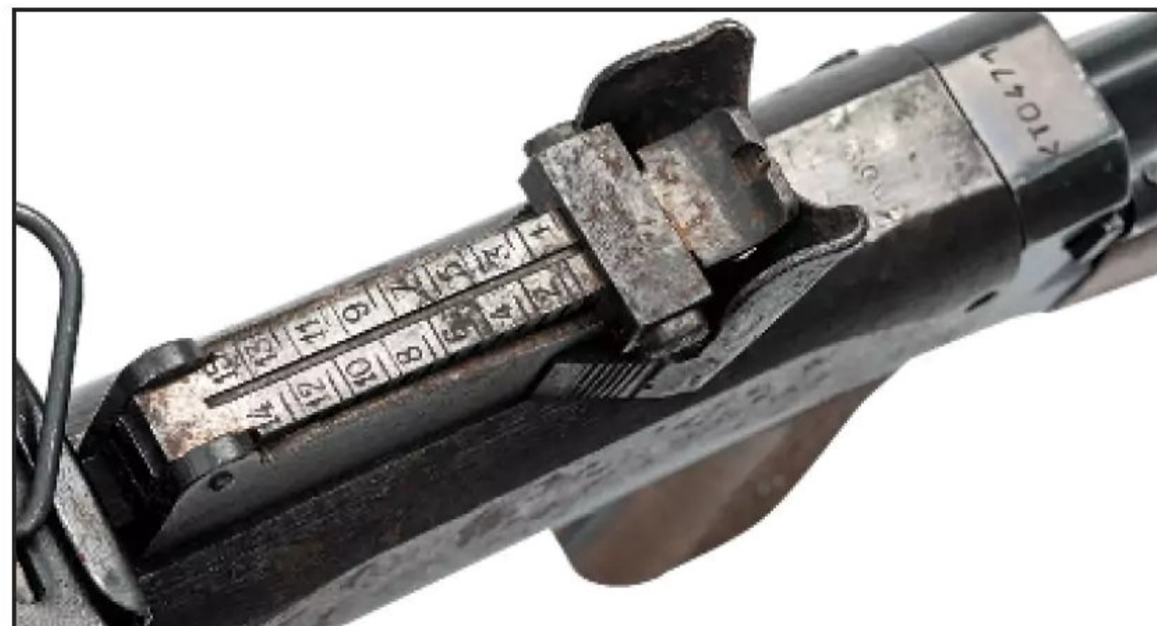
Long sight radius maximized the accuracy potential of this weapon. (Oleg Volk)
