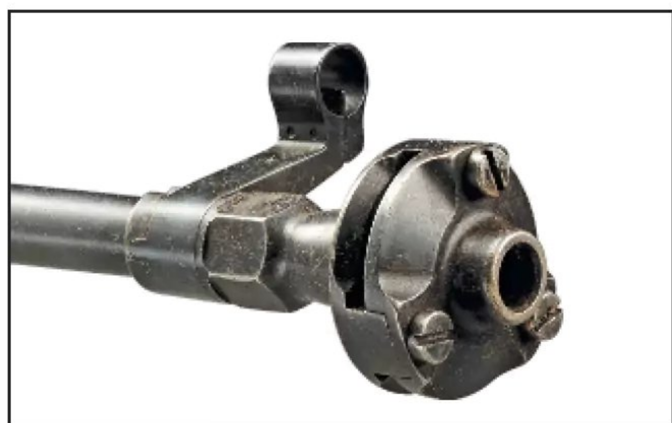
The Mark I* Boys used a slotted, circular muzzle brake. (Morphy Auctions)
