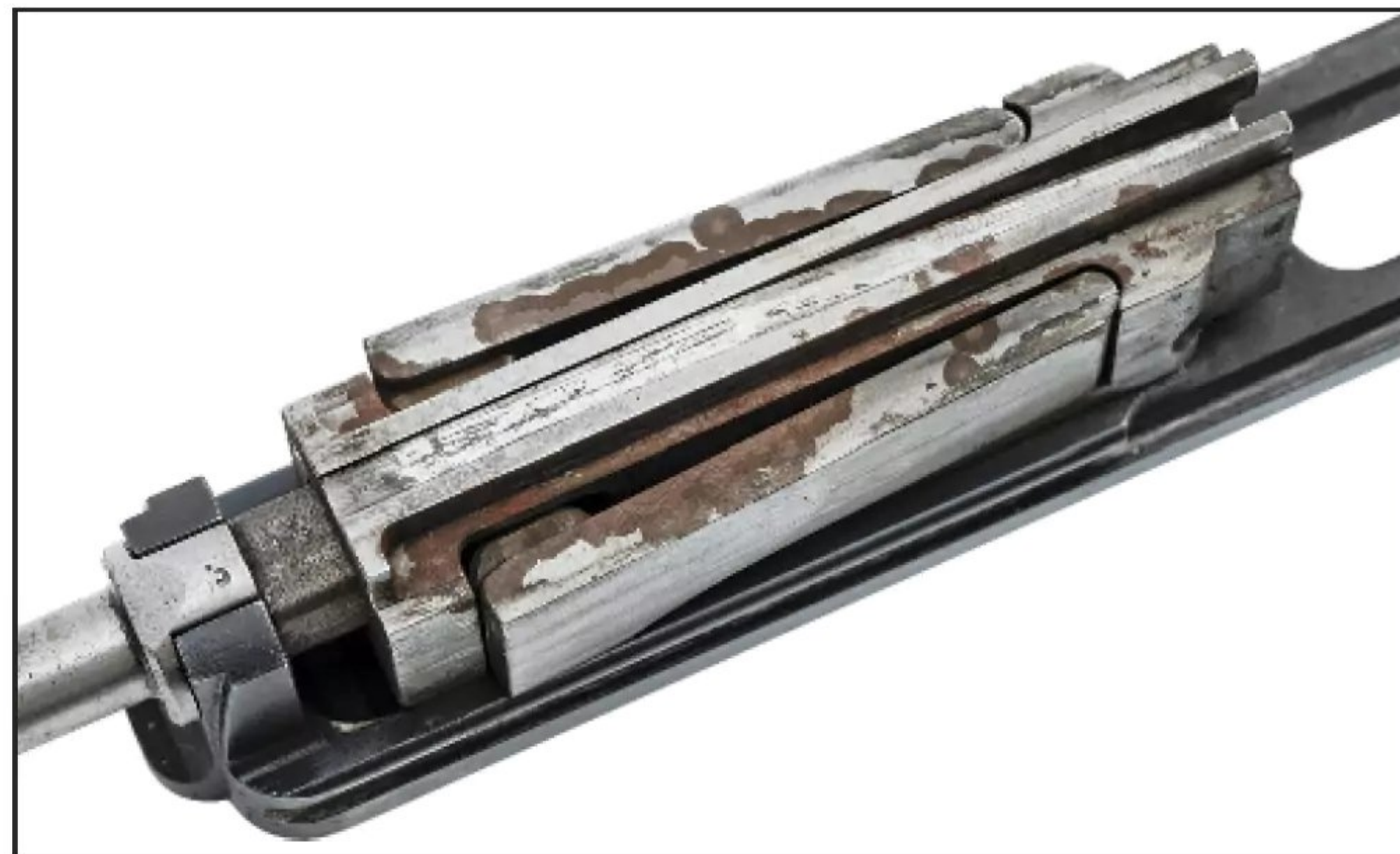
DP28 bolt with flaps in the spread, locked position. (Oleg Volk)
