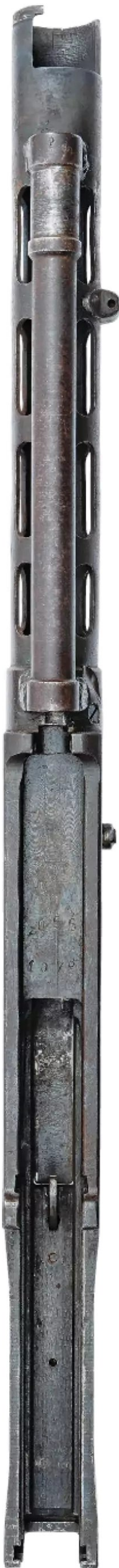
◀ Forged receiver of the DP28. (Oleg Volk)
