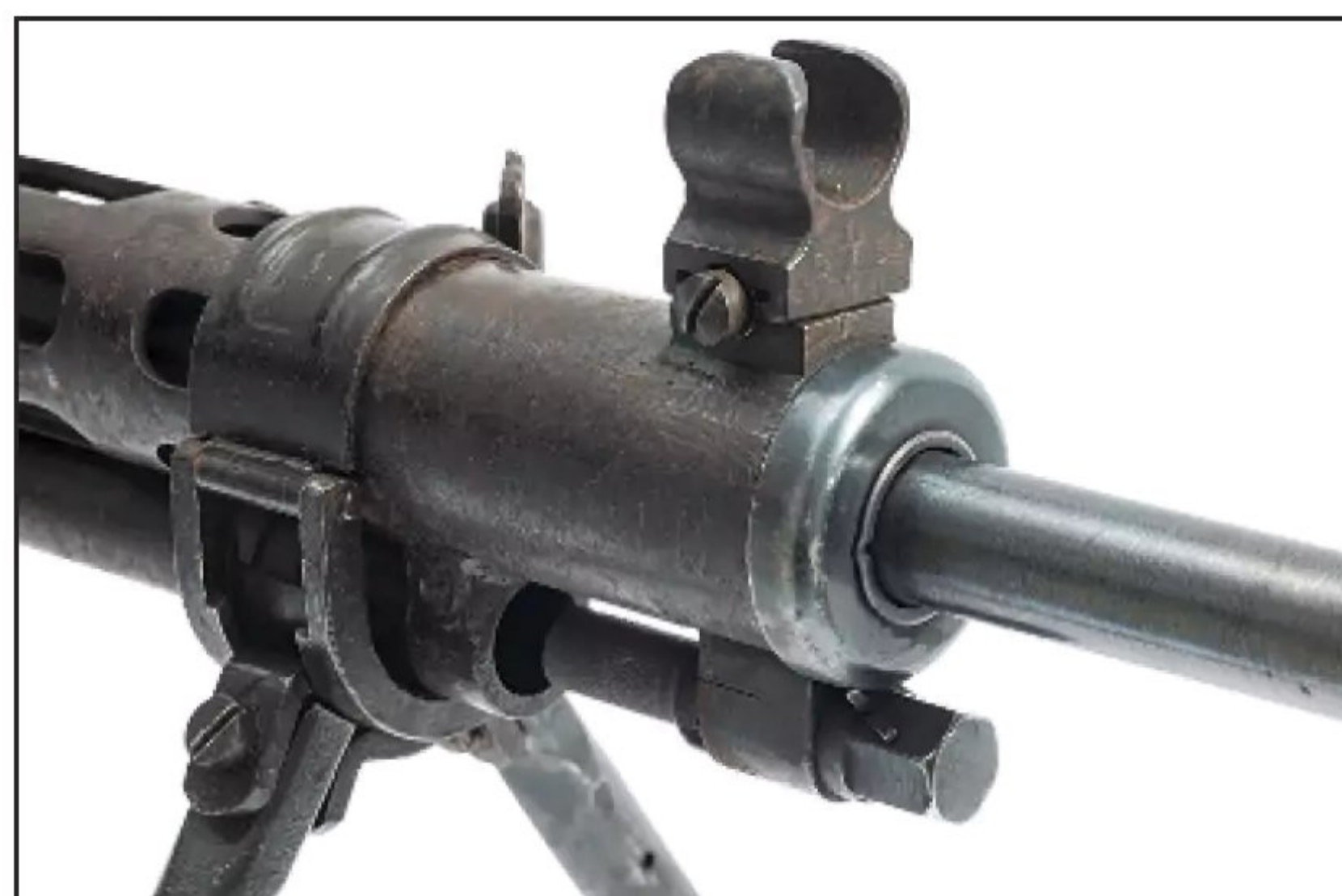
The front sight, and its base, sport hashmarks for repeatable adjustments. (Oleg Volk)
