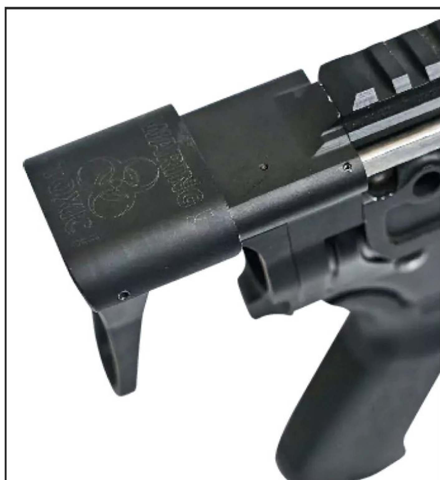
◀ The interface for J&C Armament's PDW-type stock plugs on to the rear of the upper and lower receiver and does not require modification to the lower; the stock must be fully extended for field-stripping, which is otherwise identical to a typical AR-15.
