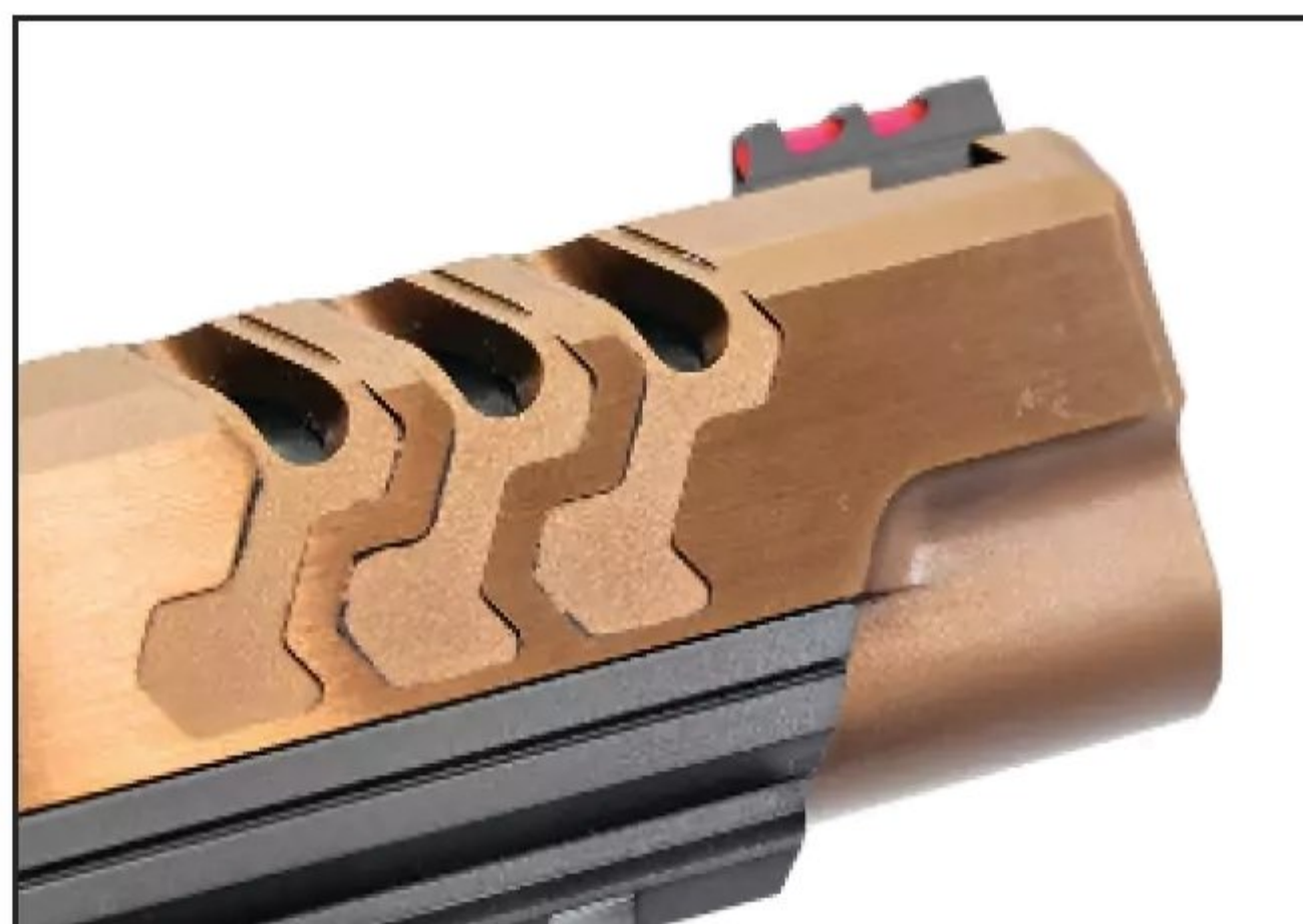
The slide has both cocking serrations and through-cuts to adjust mass and balance.
