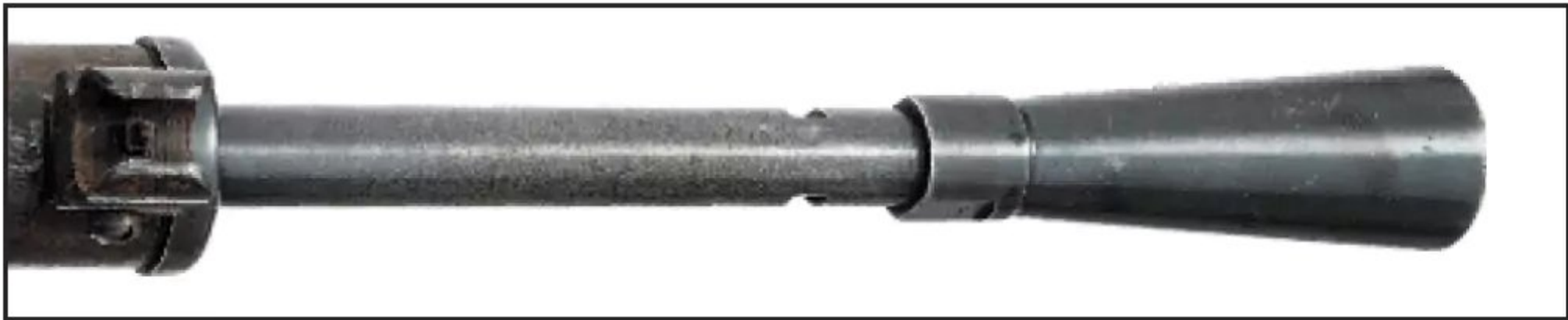
Cone-shaped flash hider, removable for transport. (Oleg Volk)
