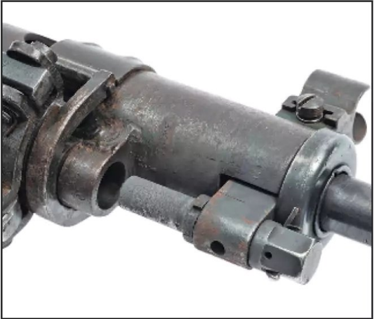
The gas regulator is easily adjustable, allowing reliability with less reciprocating mass. (Oleg Volk)
