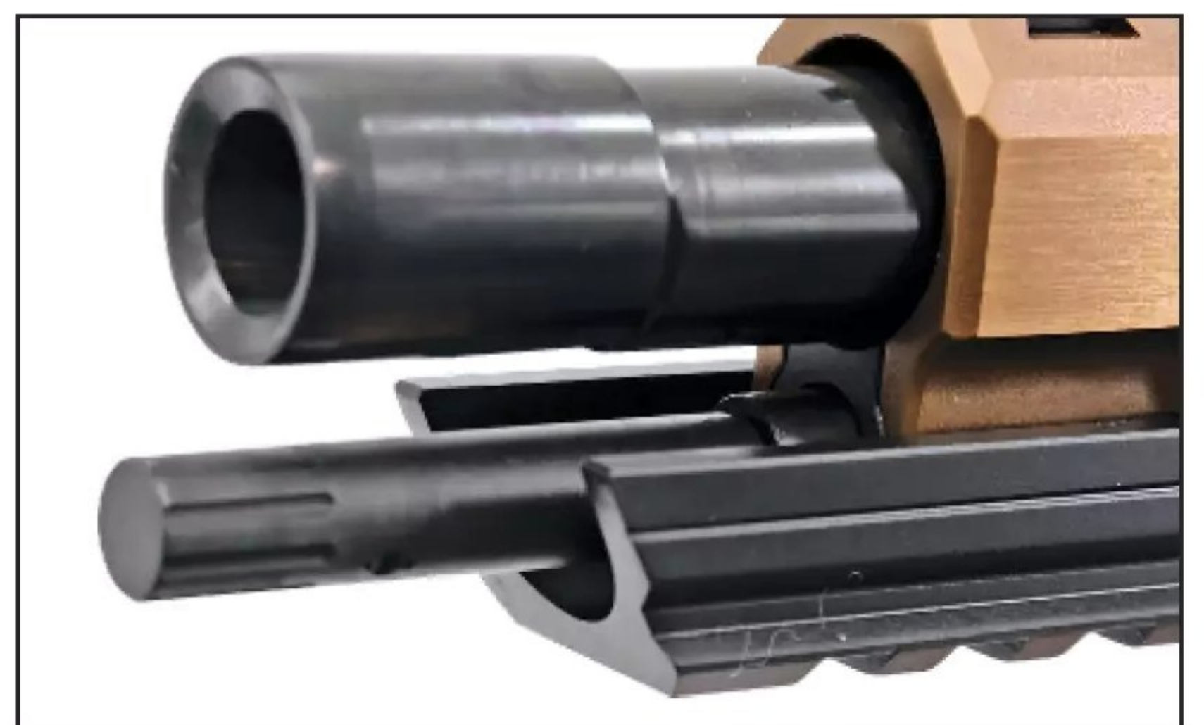
The guide rod is built as a two-piece rod, with an eccentric connection. Rotate it and you lock the spring and retainer for disassembly.
