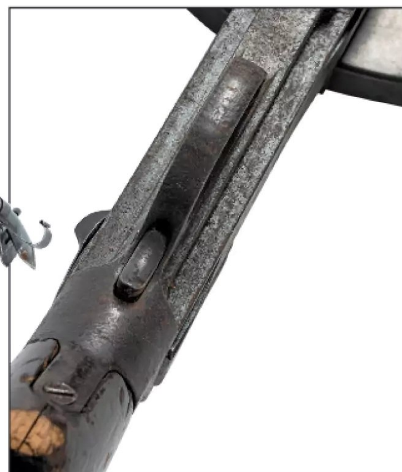
► The grip safety was deleted in later models. (Oleg Volk)
