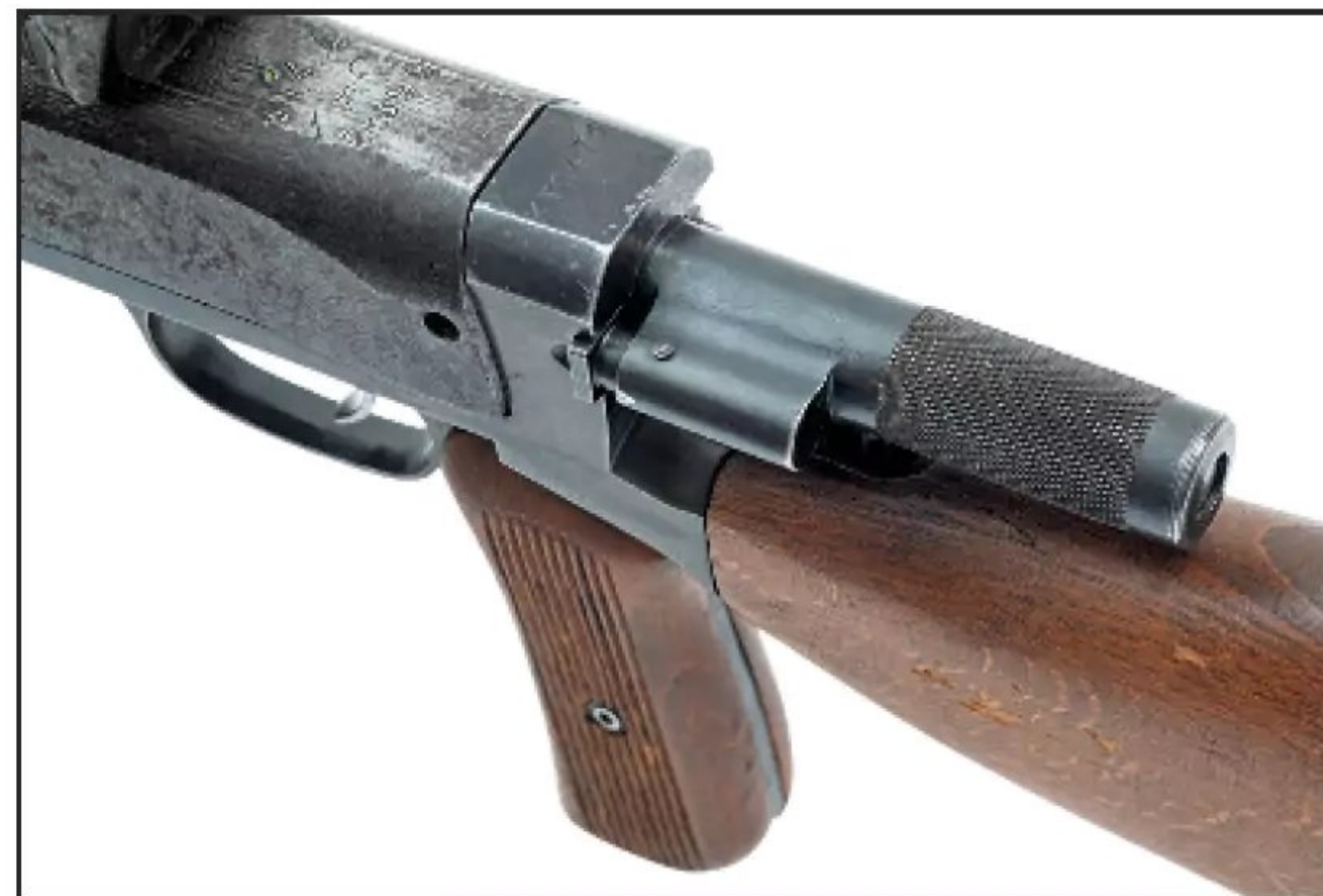
▶ The recoil spring housing: scary-looking but not actually problematic. (Oleg Volk)
