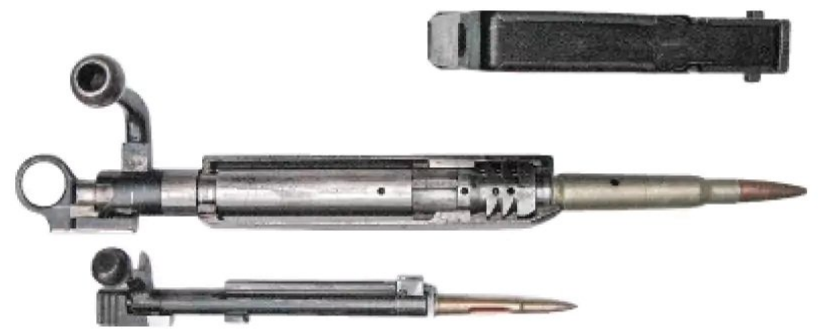
The bolt used six interrupted tread locking lugs, dual extractors, and a large ring-shaped cocking piece. (Morphy Auctions)
