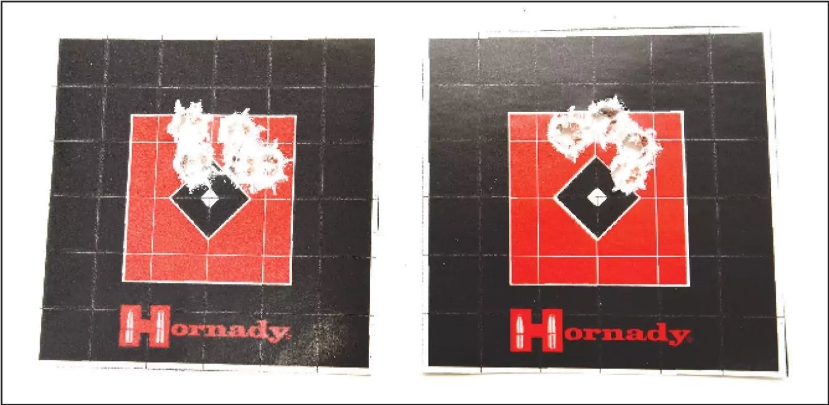
100-yard accuracy of the 6.5mm PRC Hawkeye Long-Range Target was quite acceptable with the target on the left shot with 143-grain ELD-X and on the right with 147-grain ELD Match.
