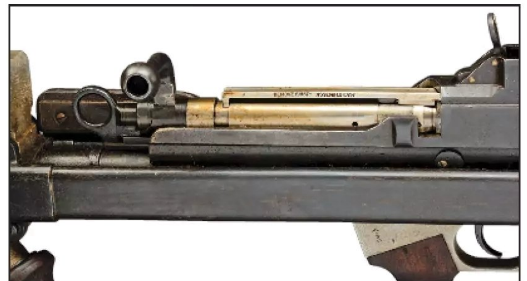
Close up of the Mark I receiver with the bolt open. (Morphy Auctions)
