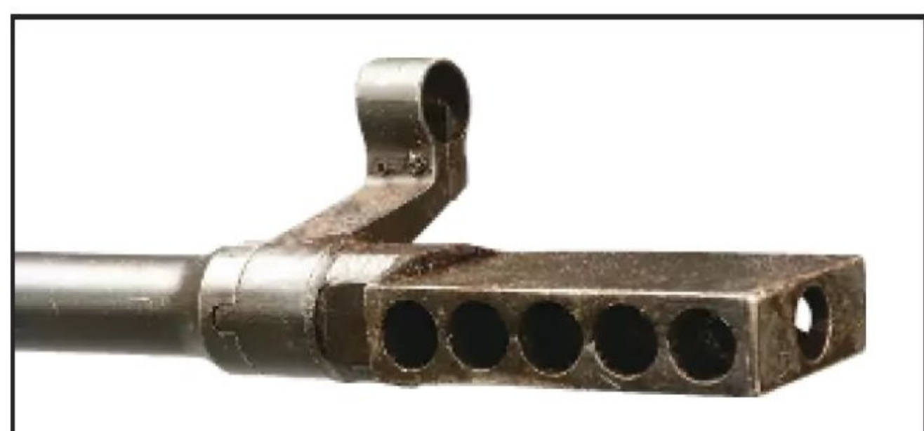
The Mark I* guns used a muzzle brake with 10 vents.
