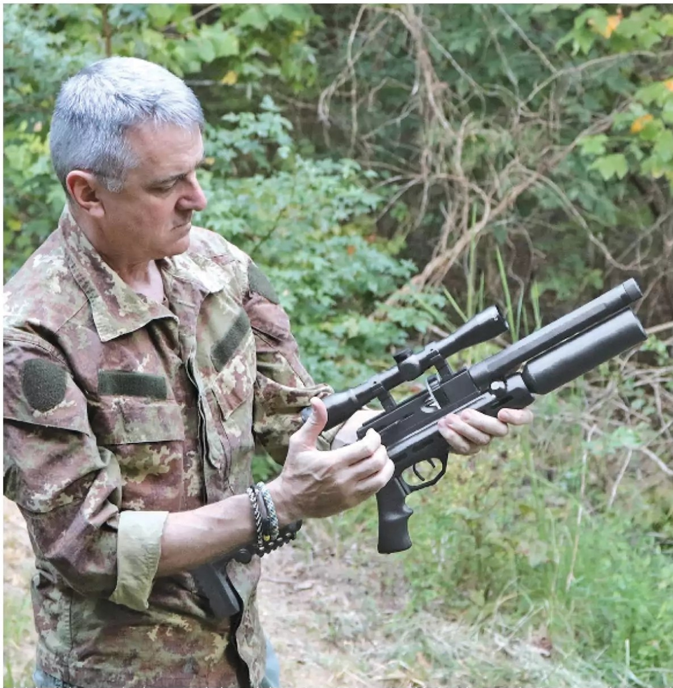
The right-sided action lever manually cycles the rifle.
