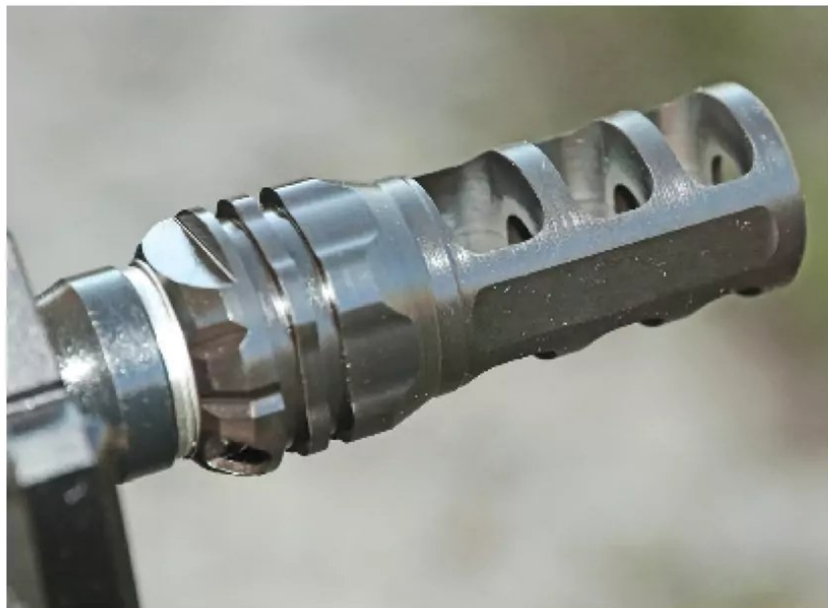
The ETM, the Elite Taper Mount, is the Gemtech QD muzzle device for mounting the Abyss. It is a muzzle brake, and it is also a very quick QD mount design.
