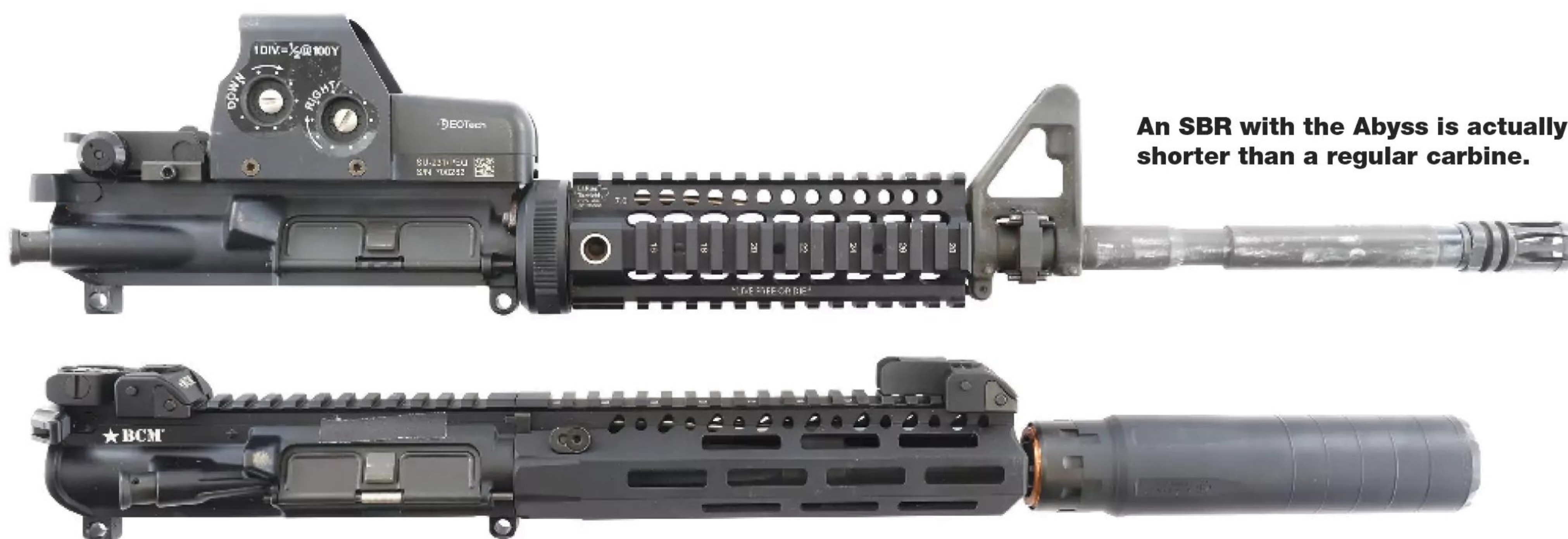
The ETM, the Elite Taper Mount, is the Gemtech QD muzzle device for mounting the Abyss. It is a muzzle brake, and it is also a very quick QD mount design.
