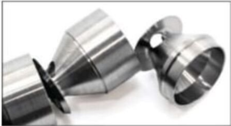
The baffles are the same except for the front-most one. That one nestles into the front cap, to maintain the stack seal.
