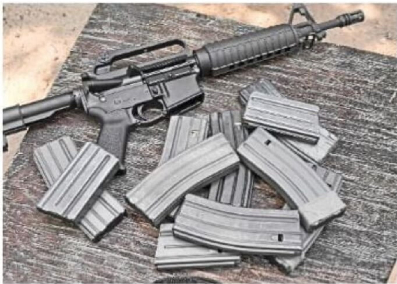
Tarr has 520 rounds through the Brownells upper without a single malfunction, using all GI-type aluminum magazines, including authentic pre-ban Colt 20-rounders.
