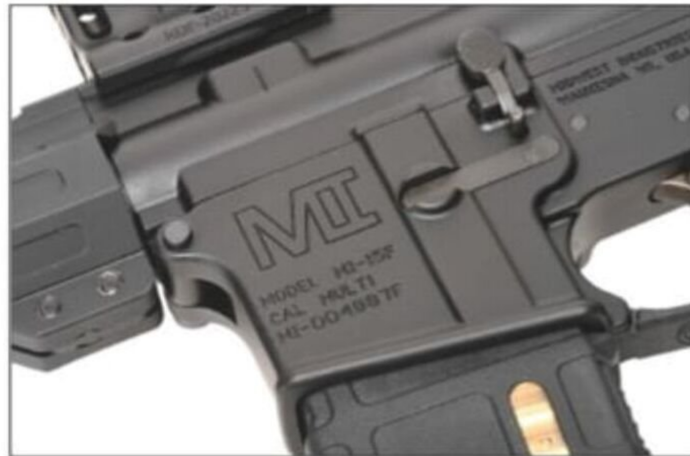
Midwest Industries uses forged upper and lower receivers machined from 7075-T6 aluminum and hard coat anodized per Mil-Spec/TDP Mil-A-8625F, Class 2, Type 3.
