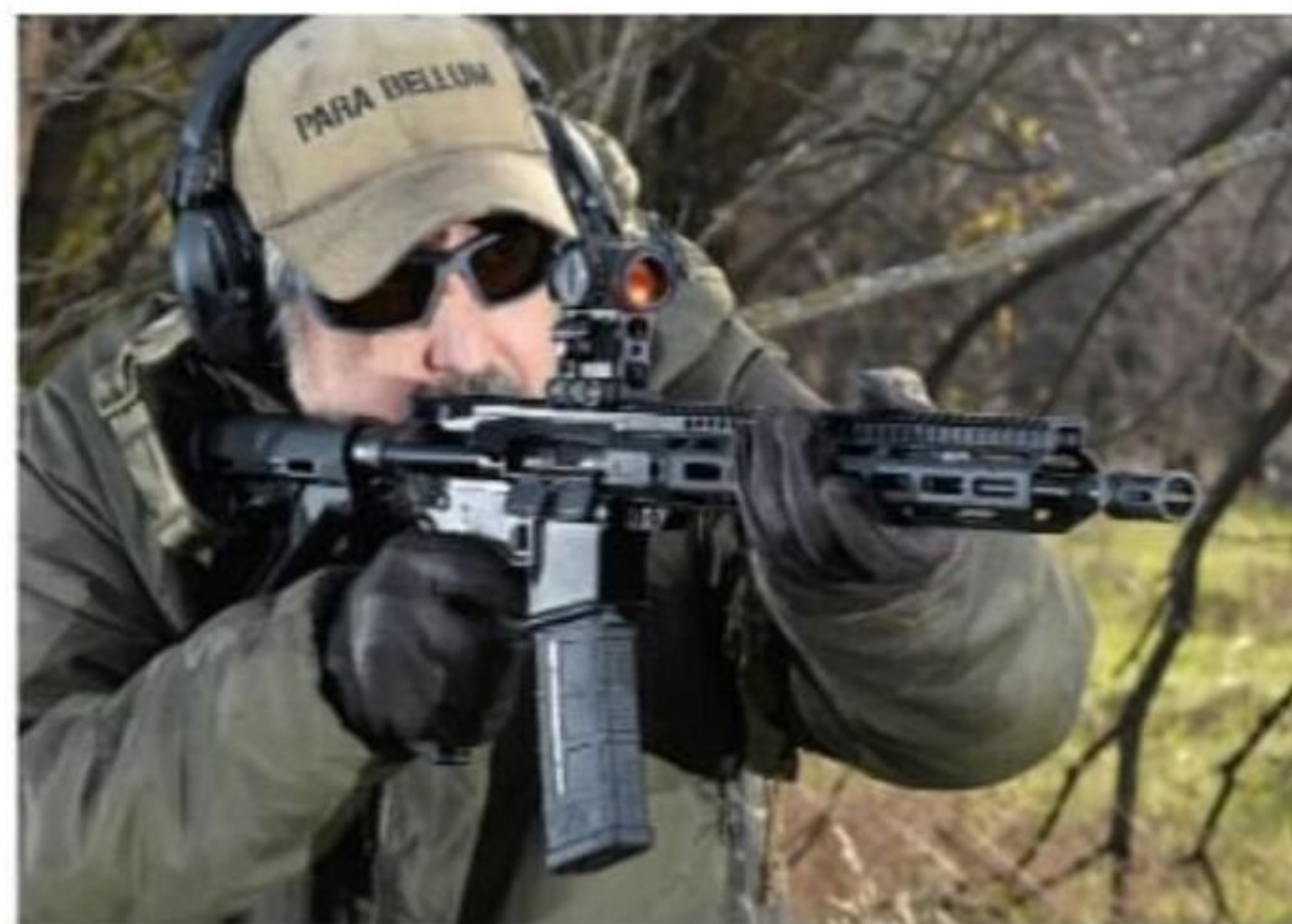
Midwest Industries chose to use a .223 Wylde chamber which offers the best of both the 5.56x45mm NATO and commercial .223 Remington chamber designs.
