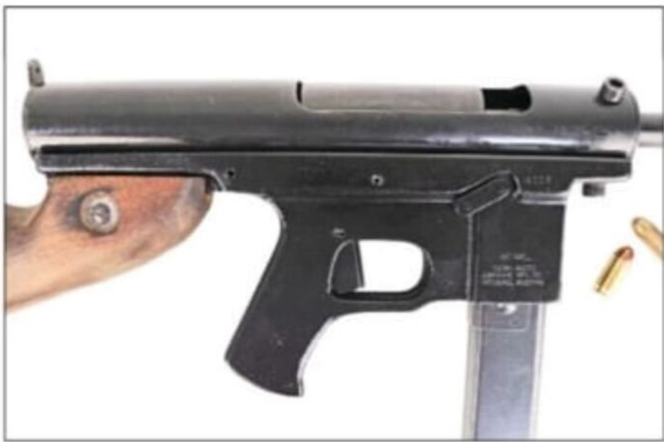
The fire control unit on the Spitfire is a rough aluminum casting. This is the only piece of the gun that bears any markings.
