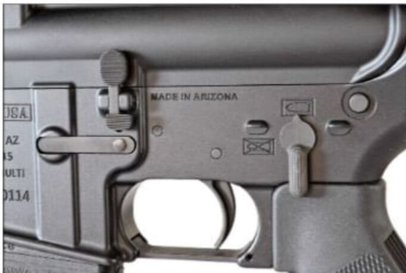
The bolt catch has an enlarged lower section to more easily lock the bolt back. Tarr likes the pictograph markings on the receiver.
