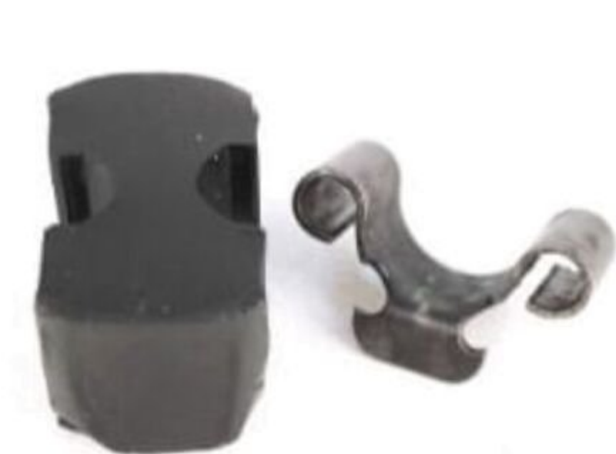
My gun has this rubber buffer in the back that speeds up the cyclic rate. The pressed steel piece on the right is the original feed ramp. Many Spitfire owners will replace this part with a more robust machined steel component.
