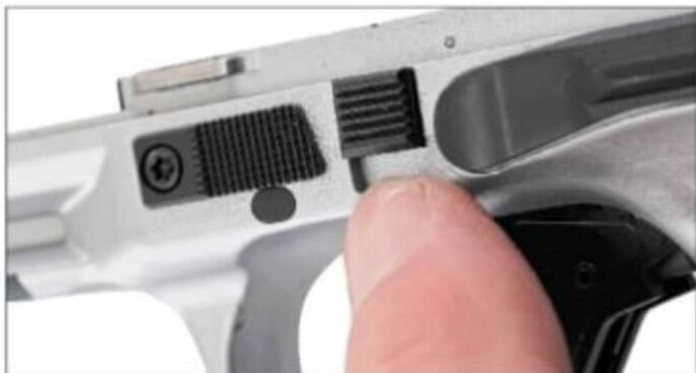
The takedown tabs, one on each side, for disassembly.
