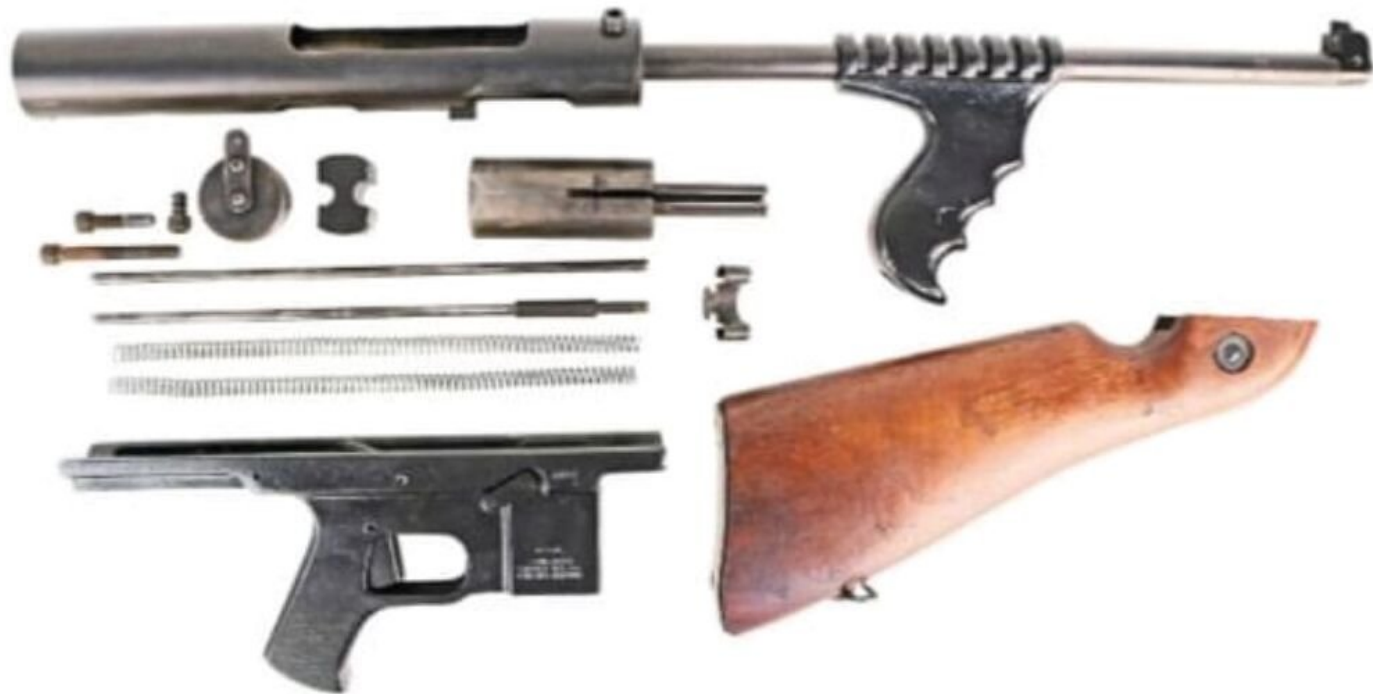
"No kidding, it took me an hour to get the Spitfire reassembled after a basic field-stripping." The gun is held together with big Allen screws. It is clearly not meant to be maintained in the field.
