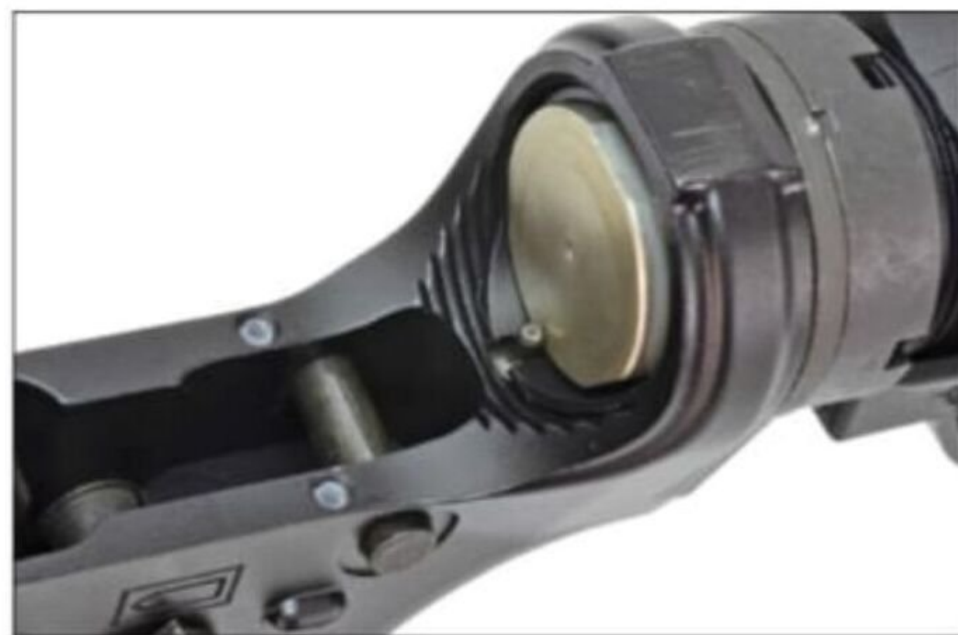
POF's buffer tube extends forward further than standard, so the rear of the bolt carrier is cradled at all times. Note the polymer screws in the lower receiver which can be utilized to tension the lower and upper receivers.
