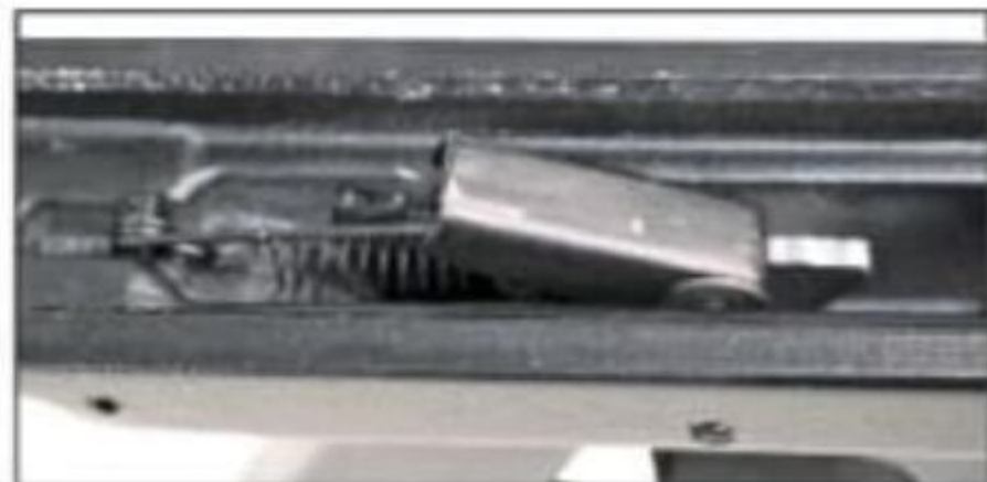
The entrails of the Spitfire are ridiculously simple. A very basic design flaw made the gun inadvertently selective fire right from the factory. By trimming back the tab on the right with a Dremel (or whatever tool was popular in the 1960s), the gun was easily rendered full auto-only.
