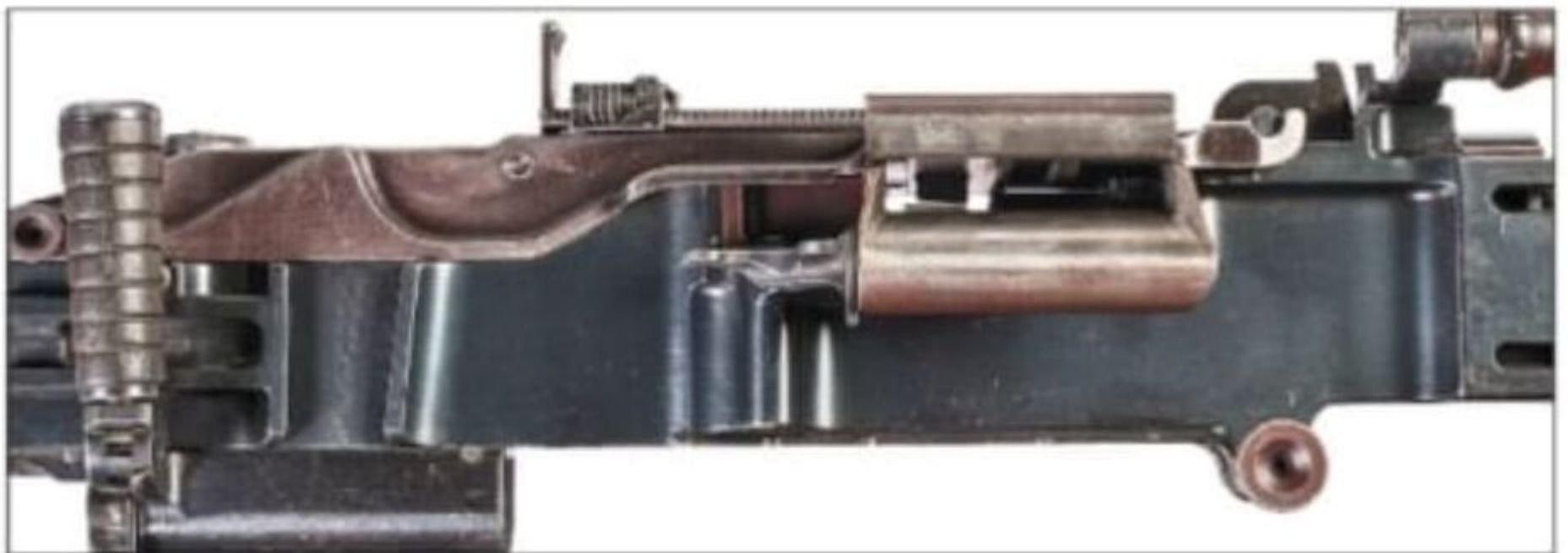
The feed ramp was located on the right side of the receiver. Note the knurled adjustment screw of the rear sight. (Rock Island Auction Co.)
