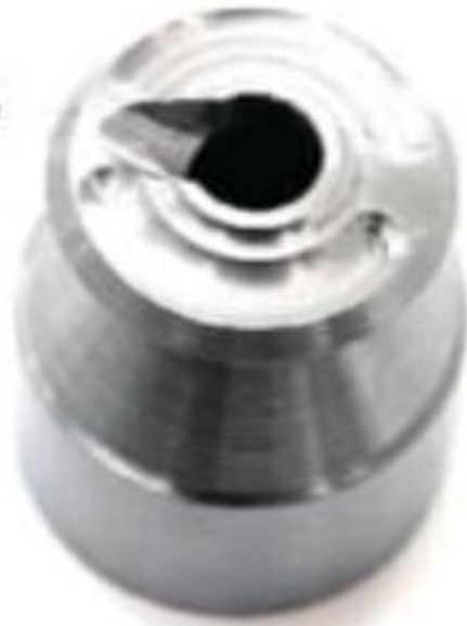
Here, you can see the turbulence-inducing notch machined on the entry port of the baffle.
