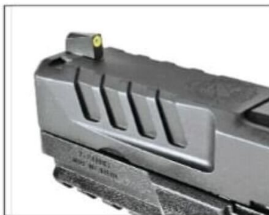
The day/night front sight of the Echelon has a bright ring of light green photo-luminescent paint around a tritium insert.
