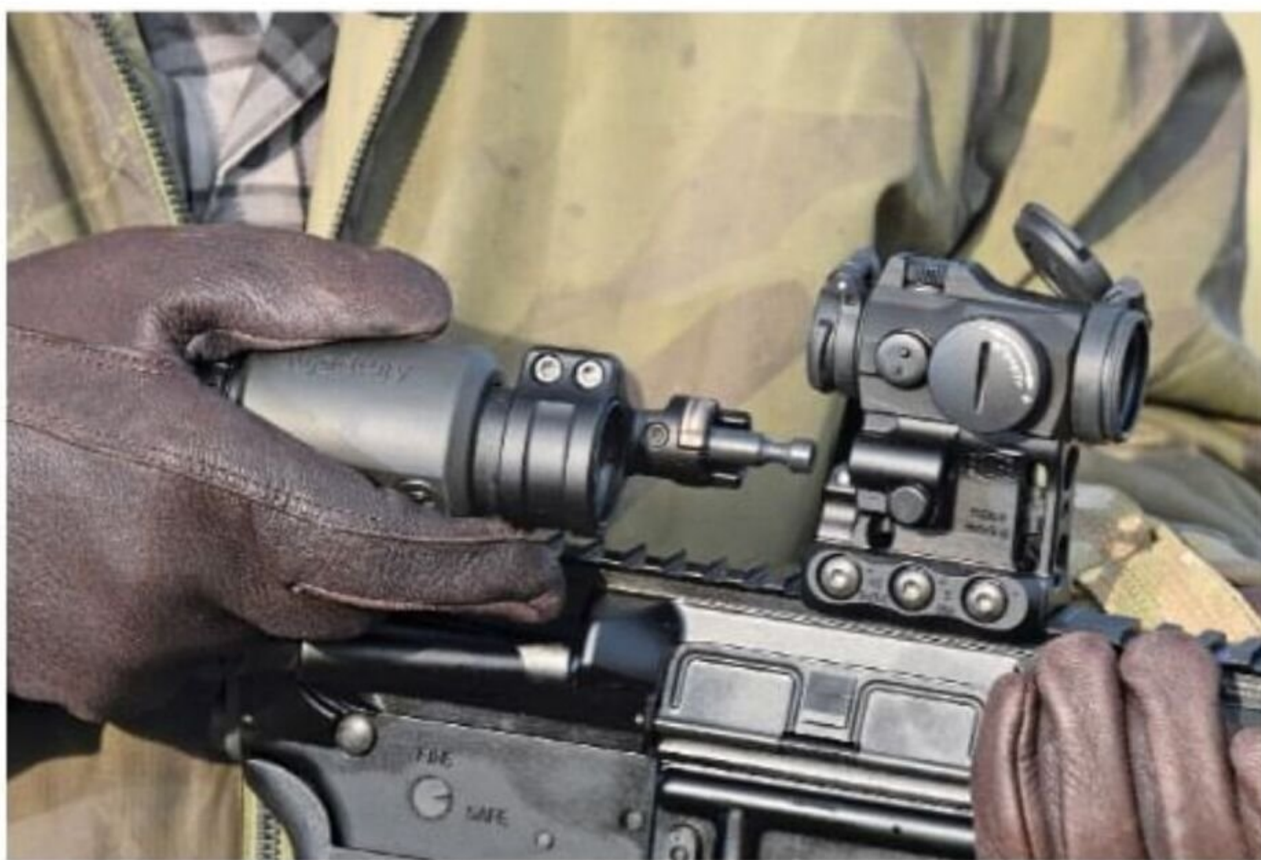
If not needed the magnifier is easily removed, not the robust mounting spigot. (Photo by Ashley Jaderborg)
