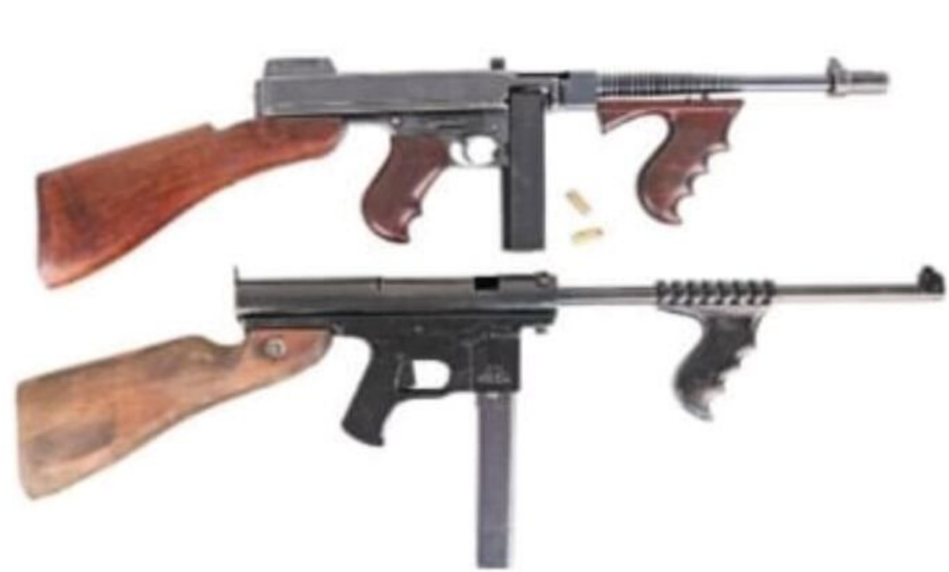
The Spitfire wanted so badly to be a Thompson, but it's just not. Aside from the chamberings and general layout of the thing, the two guns have little to nothing in common. Although Dabbs has the vertical grip mounted rather forward, typically, these were bolted on toward the rear.
