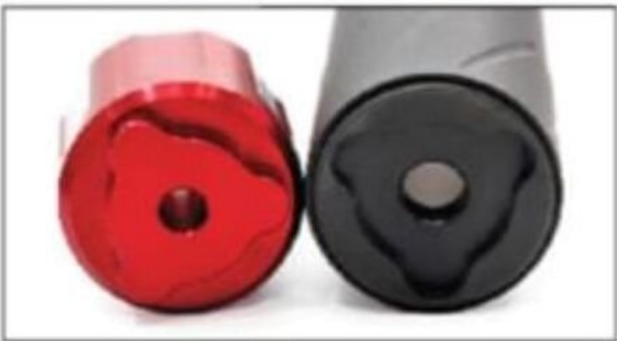
The disassembly tool is machined to fit the front cap, and this lets you unscrew the front cap.
