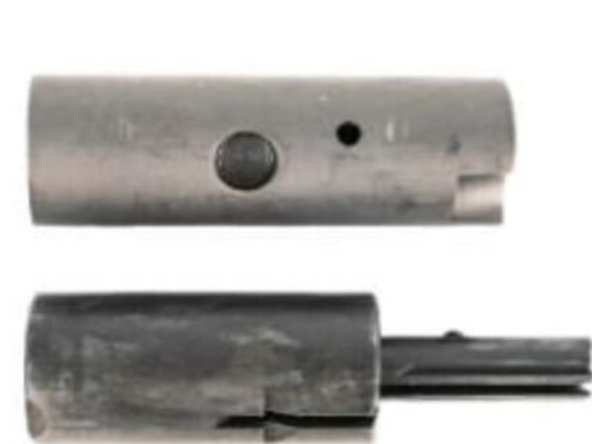
The Spitfire bolt (bottom) is shown alongside that of an M3 Grease Gun. The concept is identical, and both components are the same diameter.
