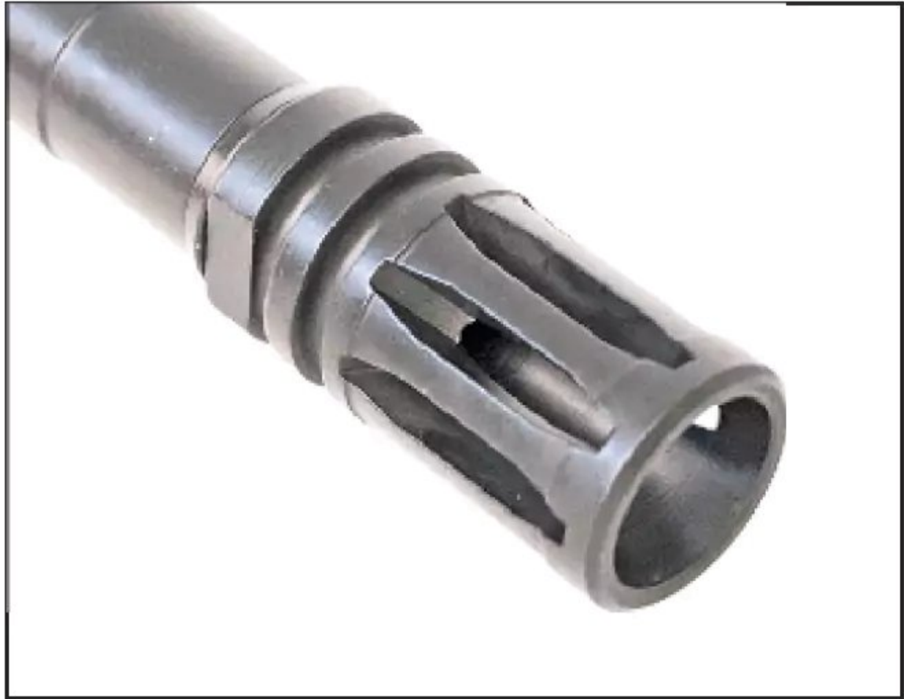
The flash suppressor is left closed on the bottom to minimize firing signature in dusty environments.
