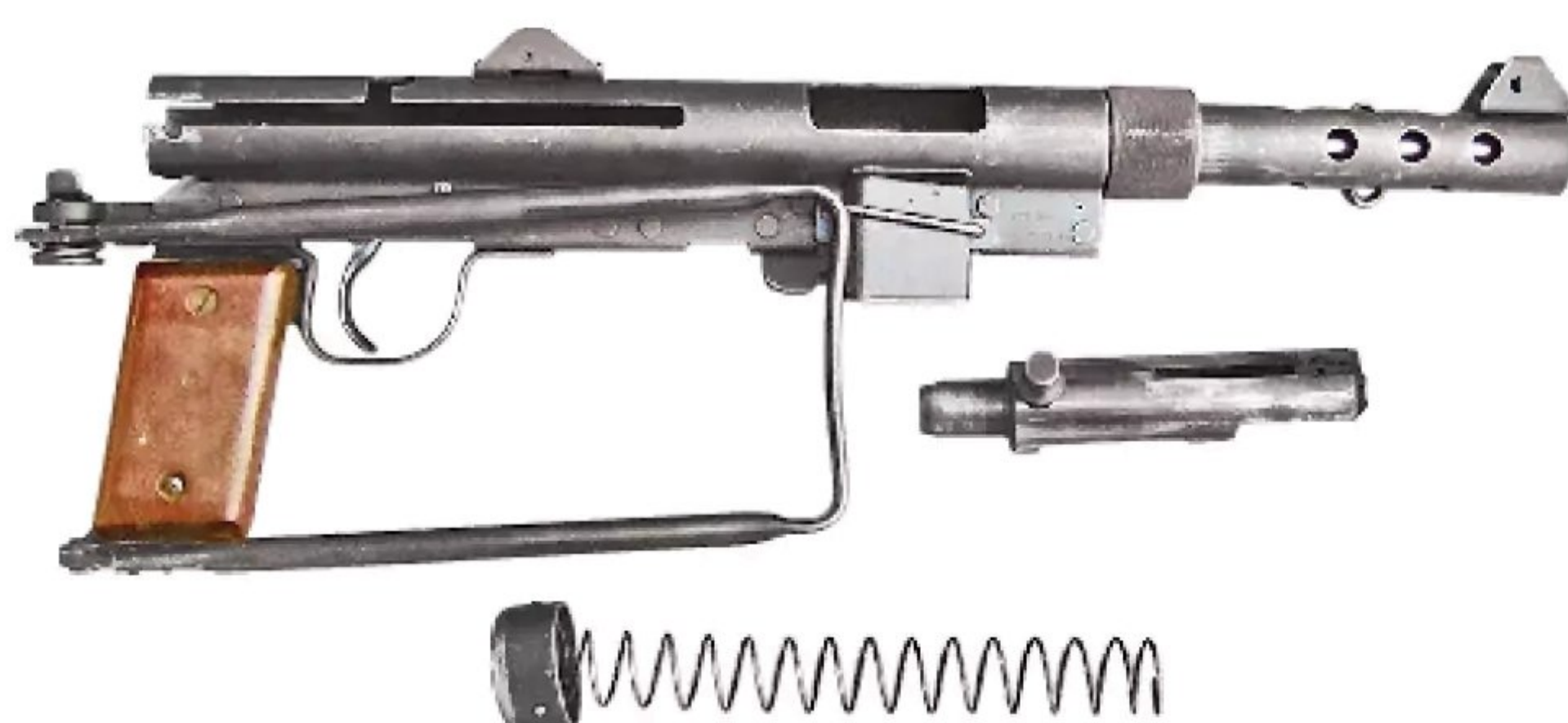
An m/45 with bolt and mainspring removed; note the detachable mag well indicating an older model m/45 or a Port Said.
