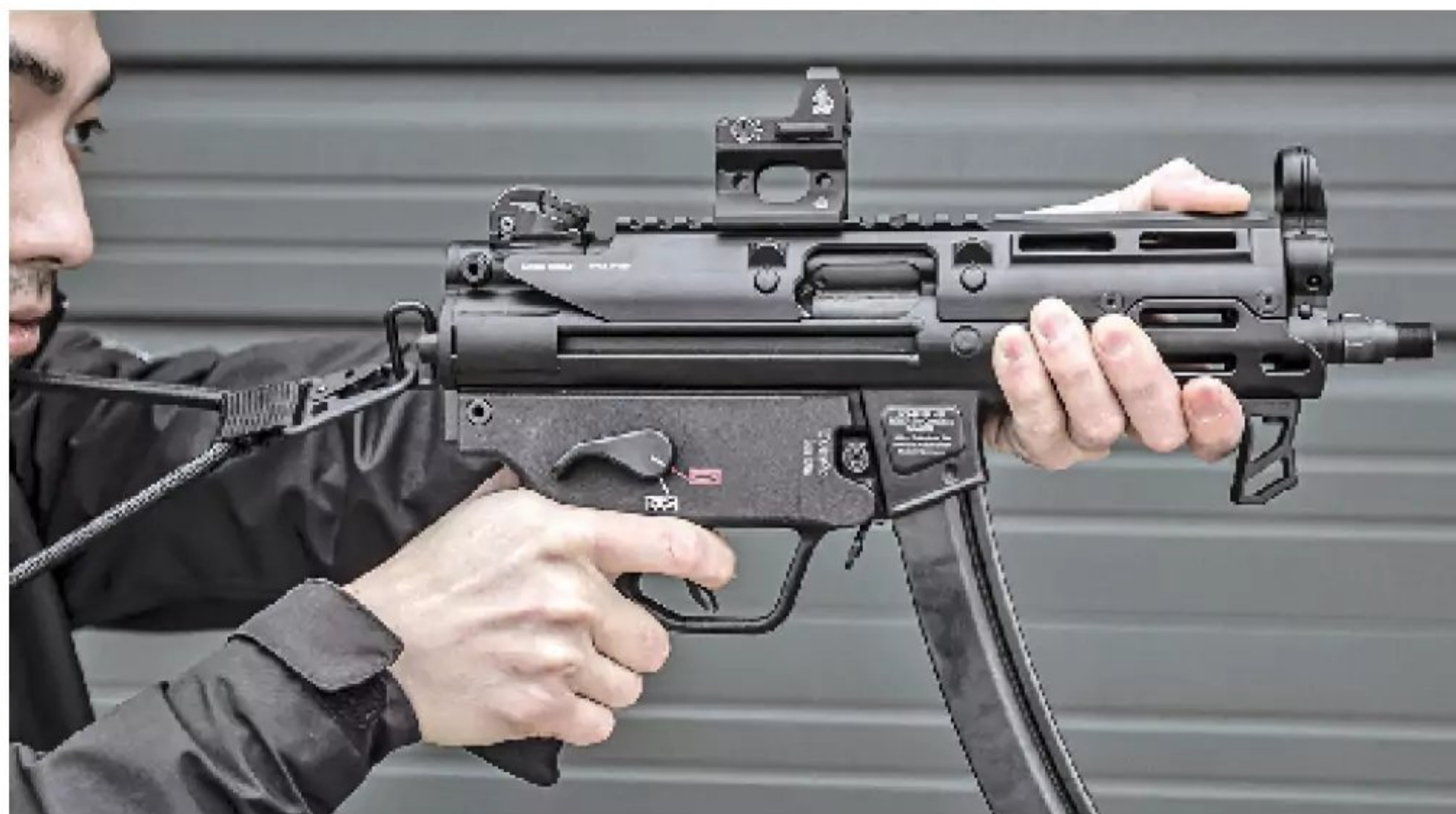
Leapers' UTG Pro monolithic mount for the MP5/MP5K clamps to the receiver, offers a lot of rail space for optics, and has M-LOK slots in the handguard.
