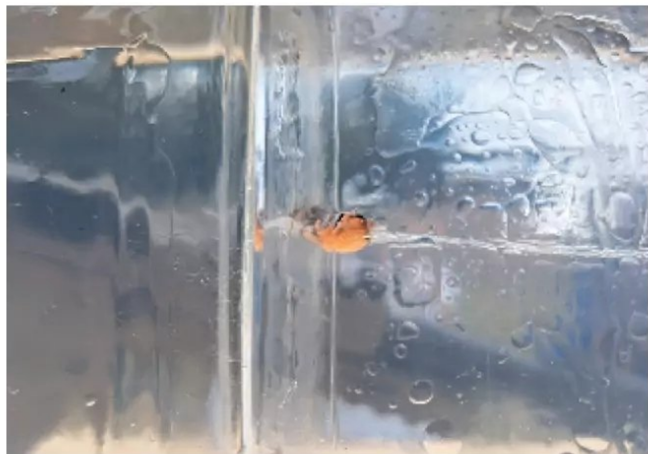
They did a lot of gel testing using Clear Ballistics' polymer blocks. Here's a Hornady 40-grain Critical Defense FTX JHP, which penetrated the block 16 inches.
