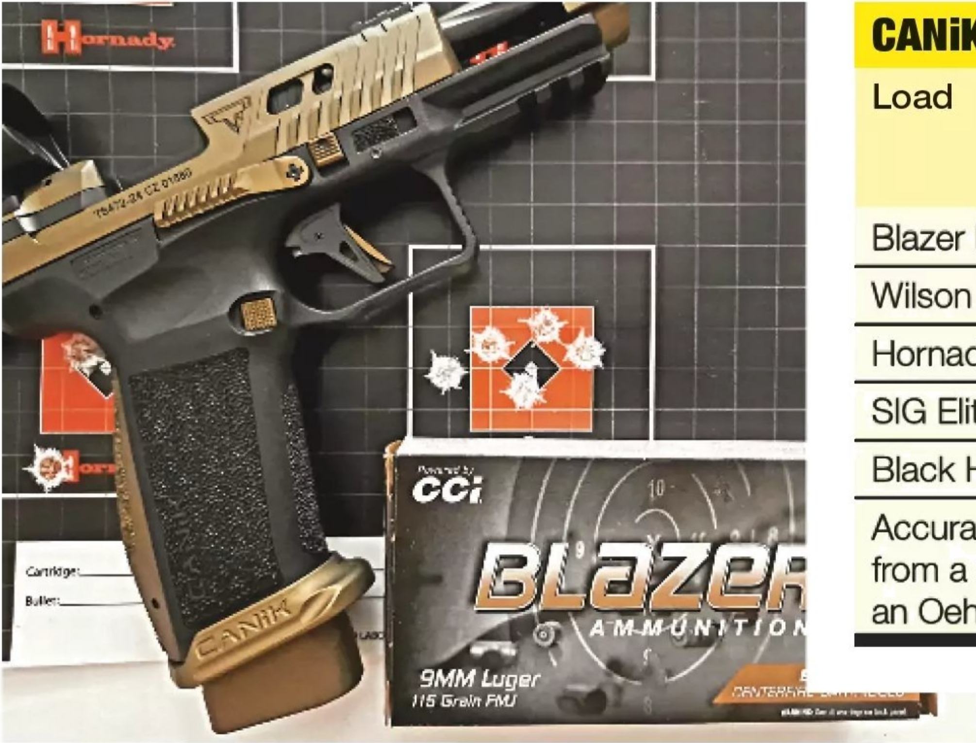
The most accurate group in Tarr’s testing was this sub-two-incher with Blazer FMJ.
