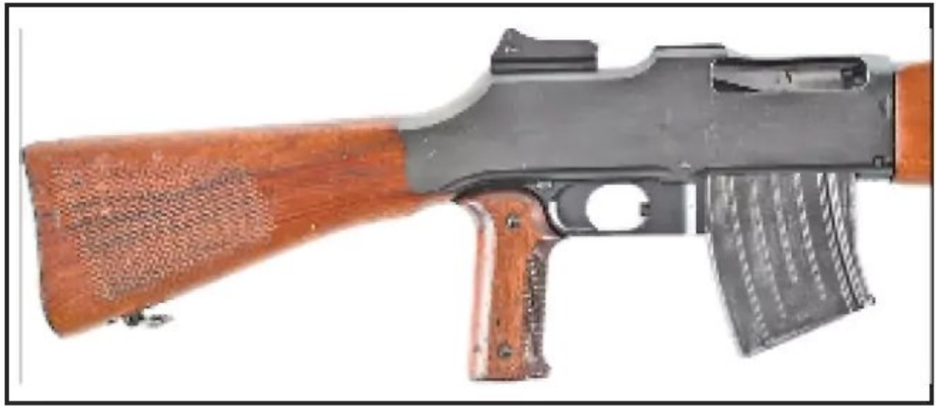
This right-hand view of the m/21's receiver shows the checkered buttstock and pistol grip, magazine release inside the trigger guard and rear sight. (Morphy Auctioneers)
