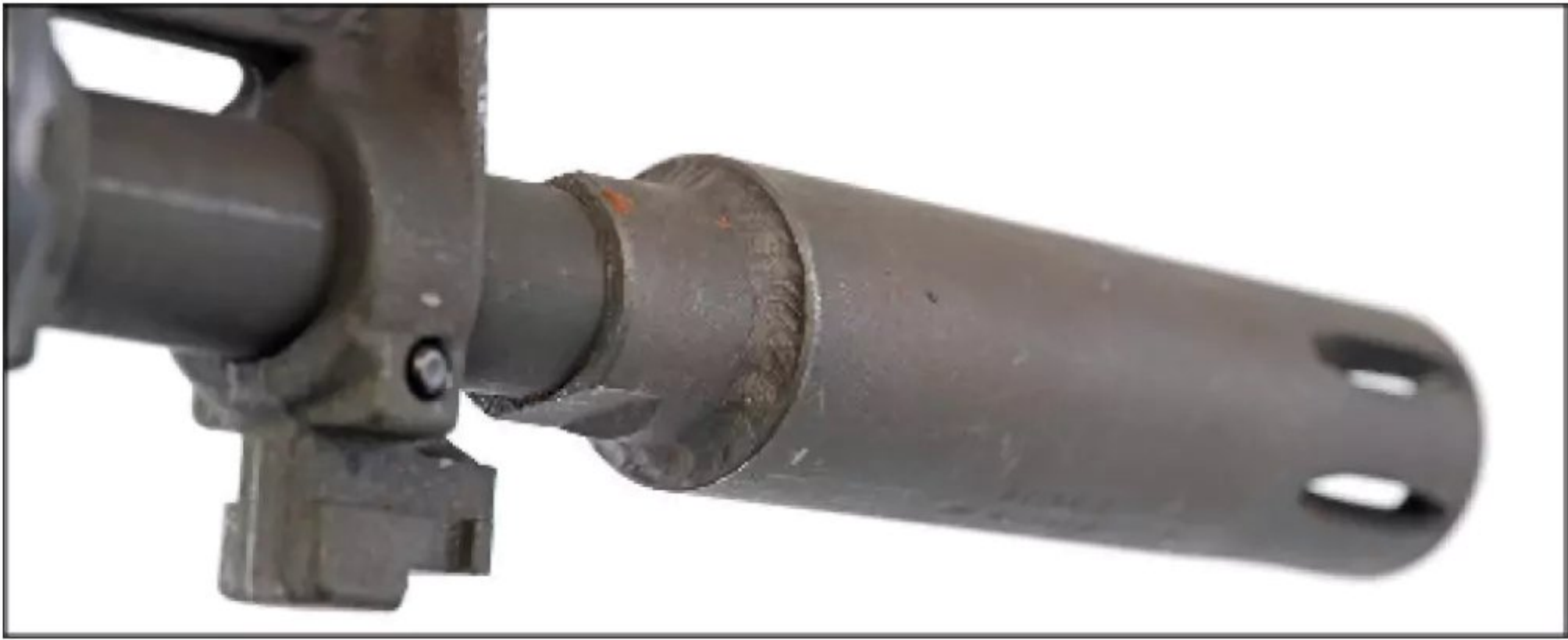
The external sleeve is welded to the baffle stack, which might be described as an early monocoire.
