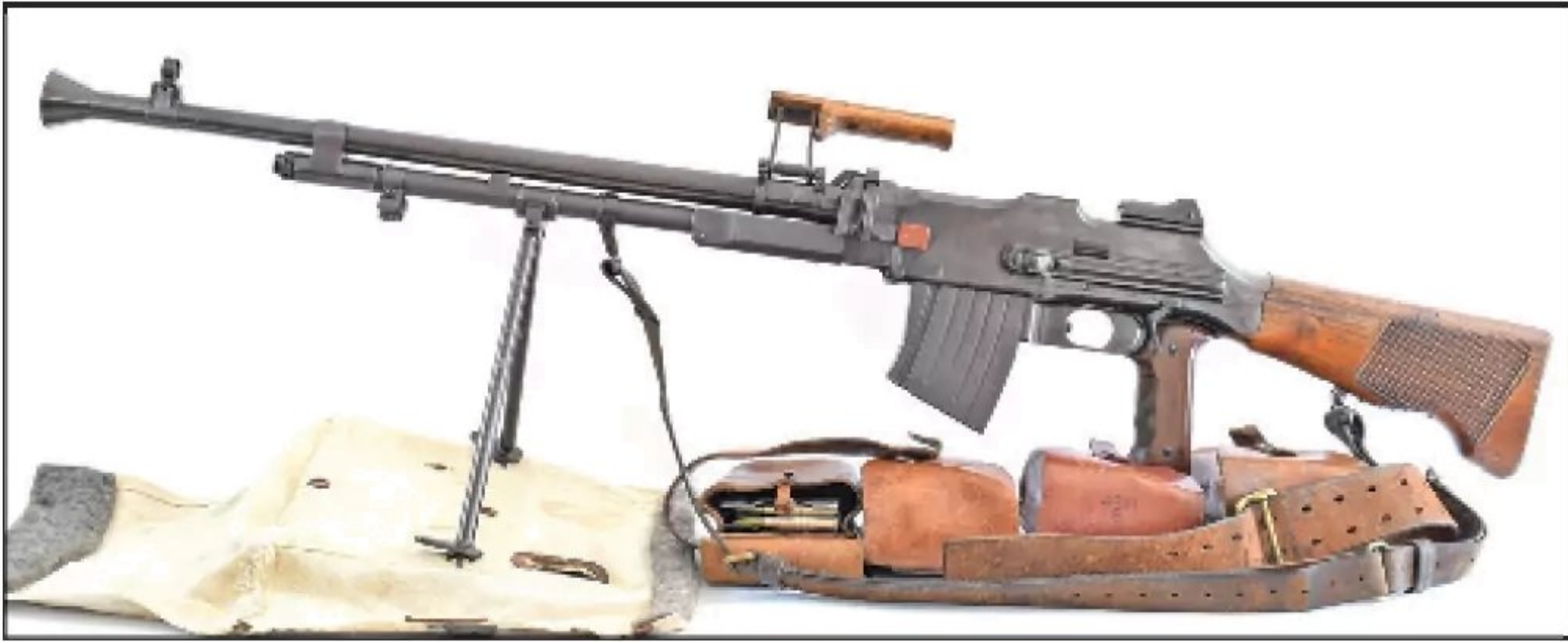
The Kulsprutegevär m/37 featured a heavier, quick change barrel system, a gas regulator, flash hider and a strengthened bipod. (Rock Island Auction Co.)
