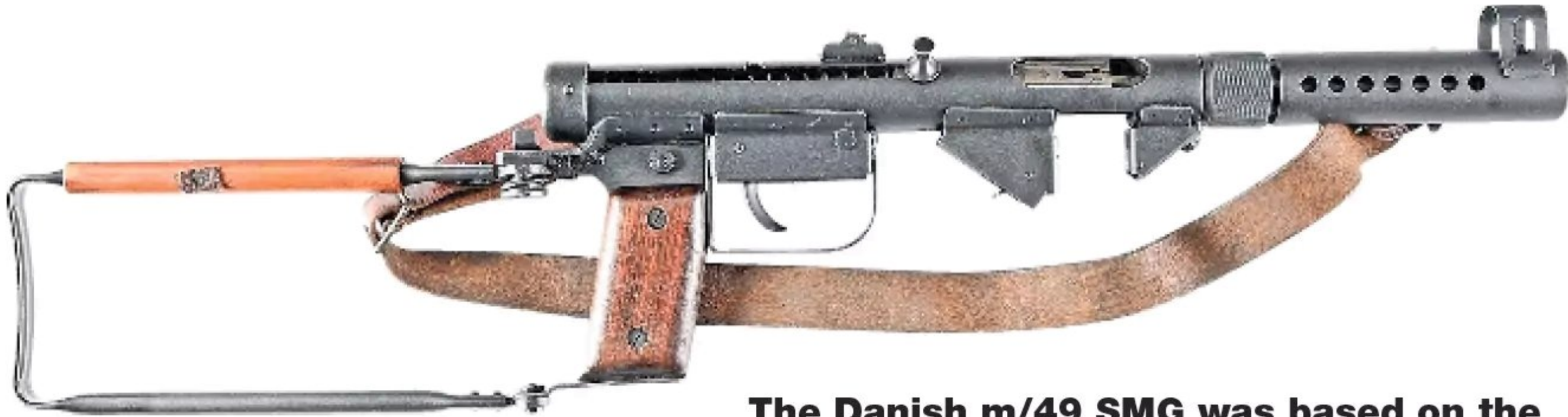
The Danish m/49 SMG was based on the Hovea m/49 designed for the Swedish SMG trials. Note the magazine well to take Suomi “coffin” magazines. (Courtesy of Morphy Auction Service)
