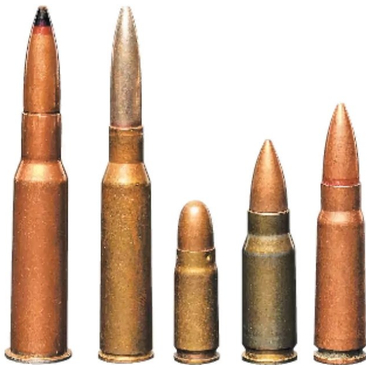
Cartridge comparison showing L to R: 7.62x54mmR, 6.5x50mmSR Arisaka as used in Fedorov Avtomat M1916, 7.62x25mm used in Soviet submachine guns, 7.92x33mm Kurz and 7.62x39mm. (Photo by David M. Fortier)
