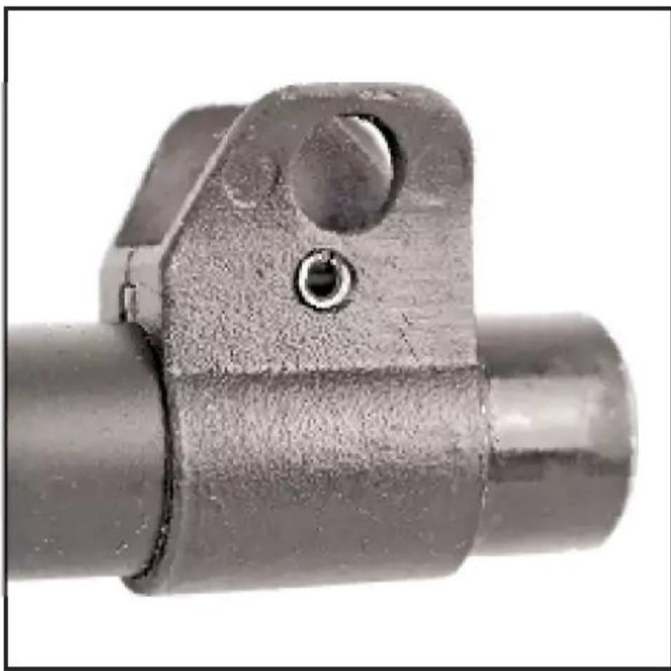
Removing the front sight involves pushing out this small roll pin. There's really not much to that.
