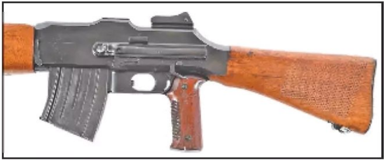
This left-hand view of the receiver shows the non-reciprocating cocking handle, safety and fire selector levers. (Morphy Auctioneers)
