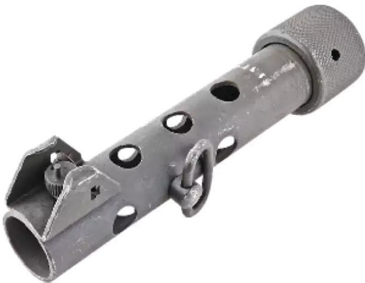
The barrel shroud of an m/45 removed and showing the cooling holes and the post front sight.
