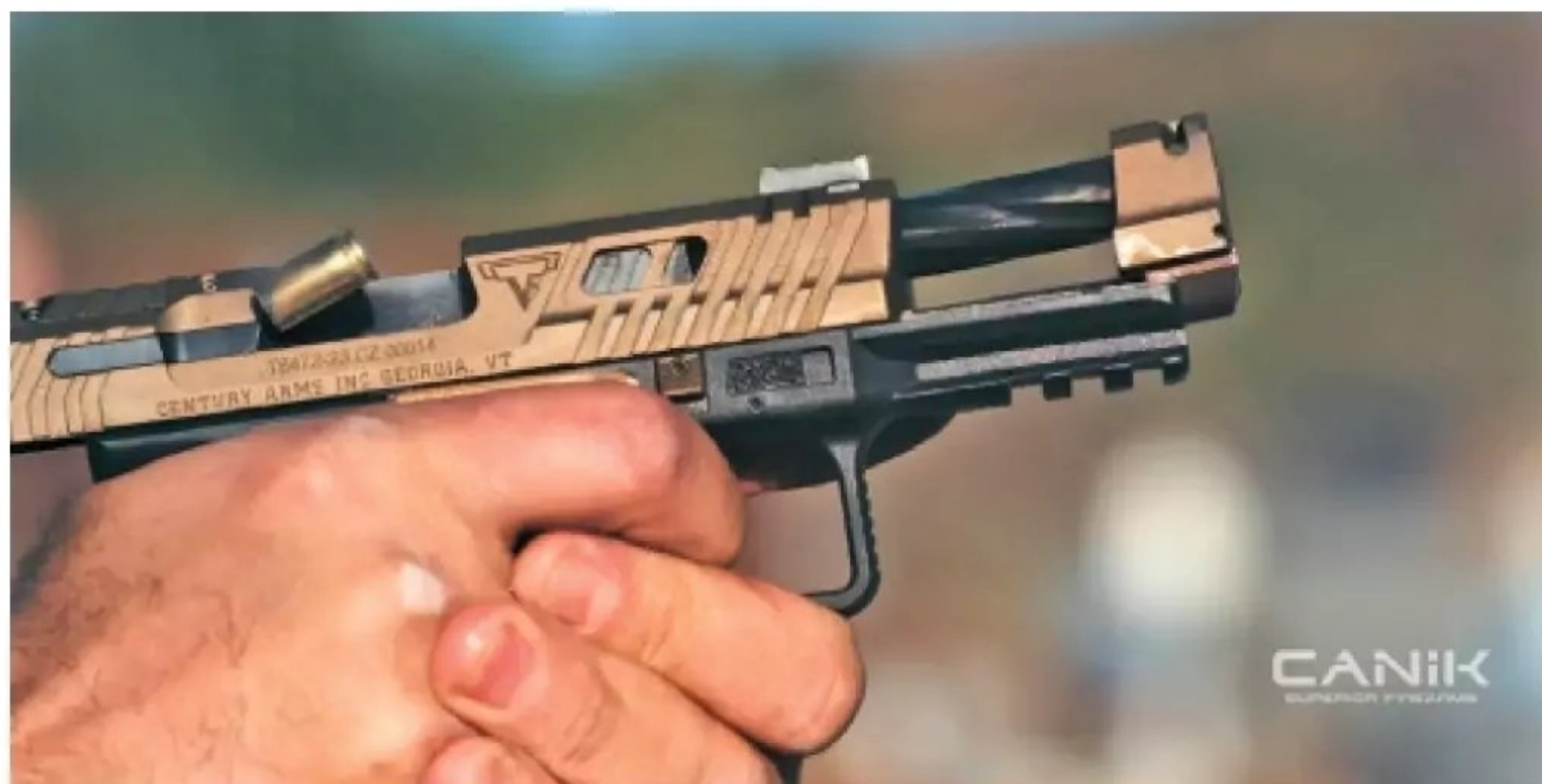
A still from Taran Butler shooting the TTI Combat, the gun in full recoil. Between the aggressive texturing and the compensator muzzle rise is reduced about 20%. (Taran Butler)
