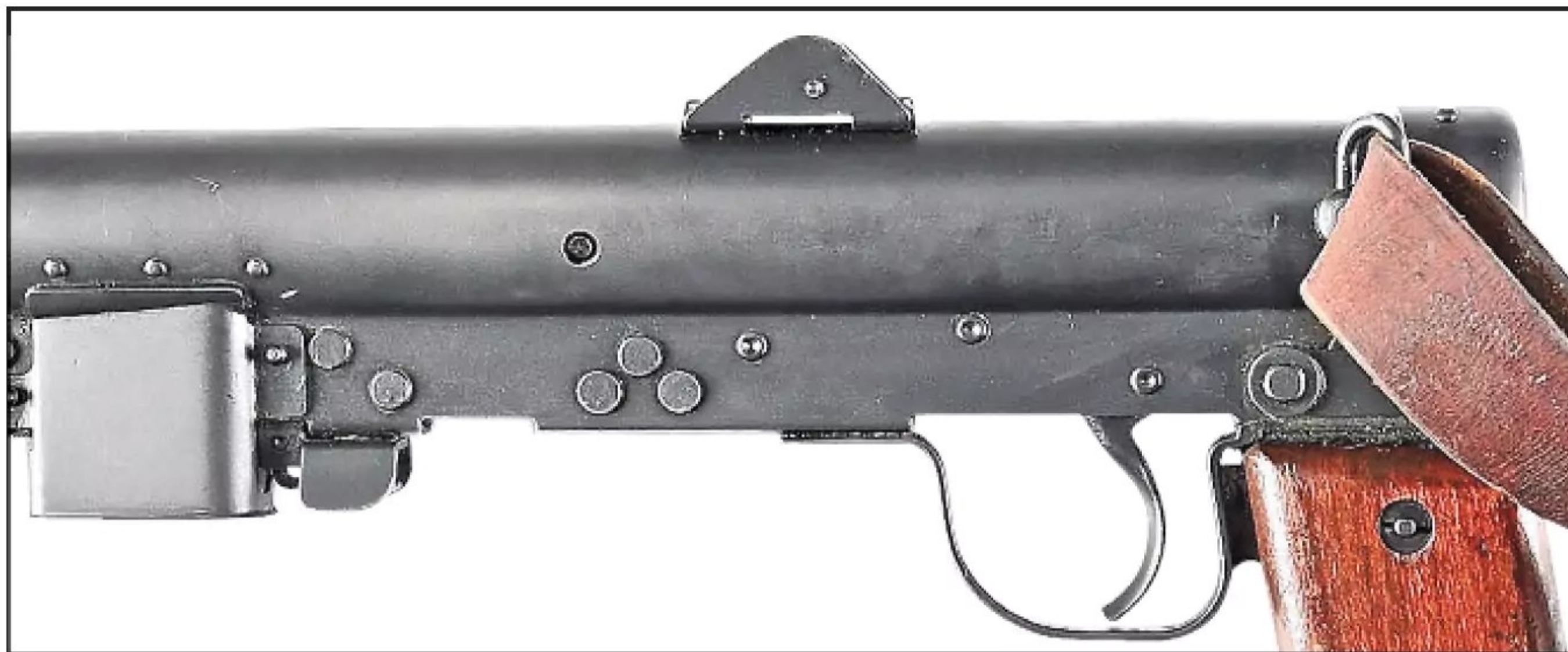
Left-side view of the m/45Bs receiver; note the shield for the magazine release behind the magazine well for the 36-round magazine. Note also on the receiver in front of the rear sight, the recess through which the bolt knob is pressed to lock the bolt forward.
