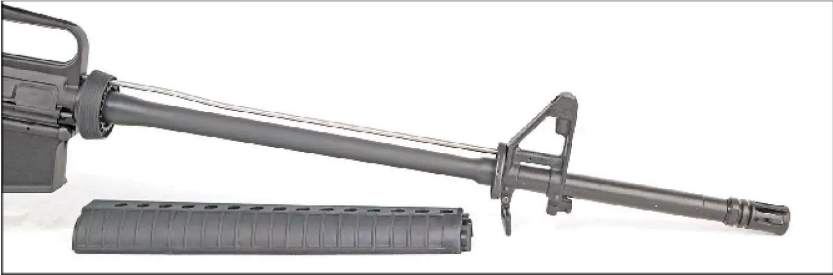
The barrel on the SA-16A2 is heavy ahead of the front sight base but thinner behind, just like those of the original M16A2 service rifles.
