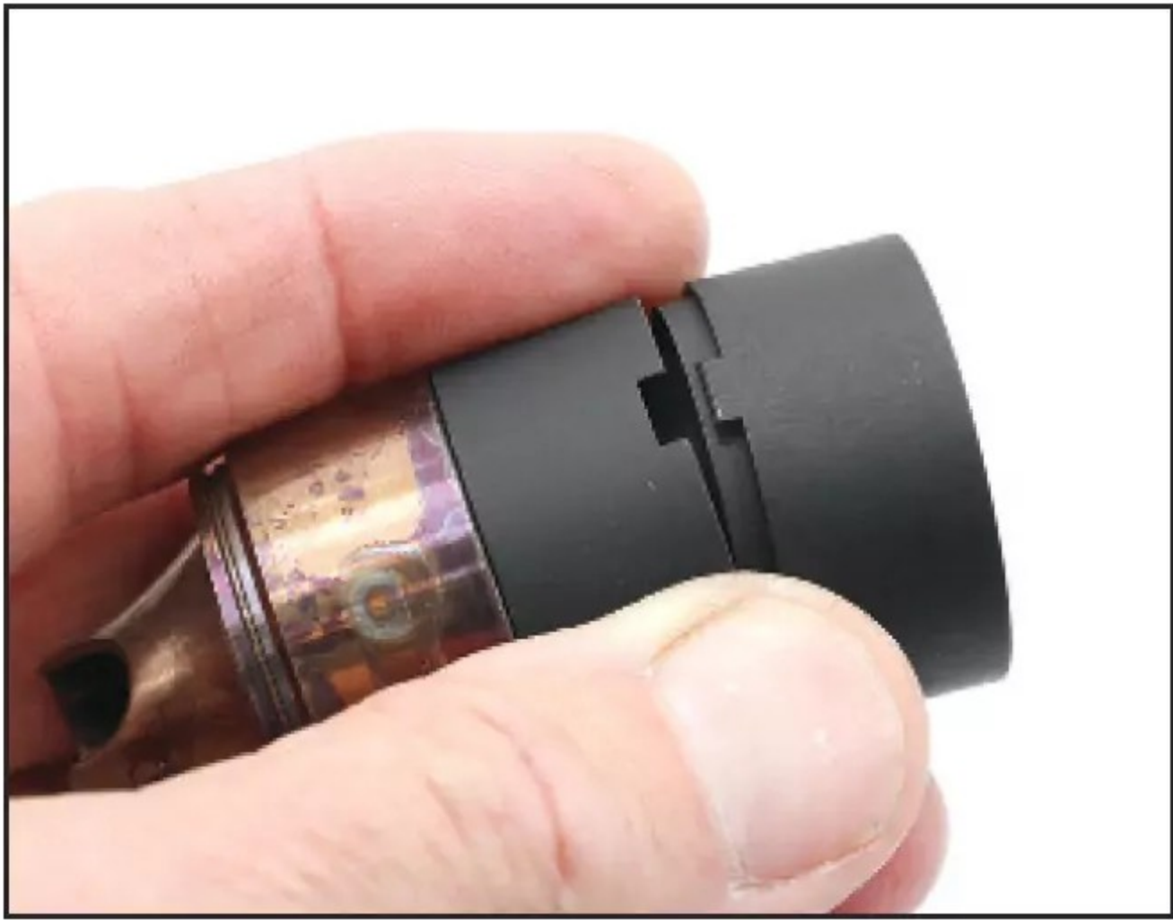
Each baffle is lugged and notched so you can only fit them together properly, and still screw on the front cap.
