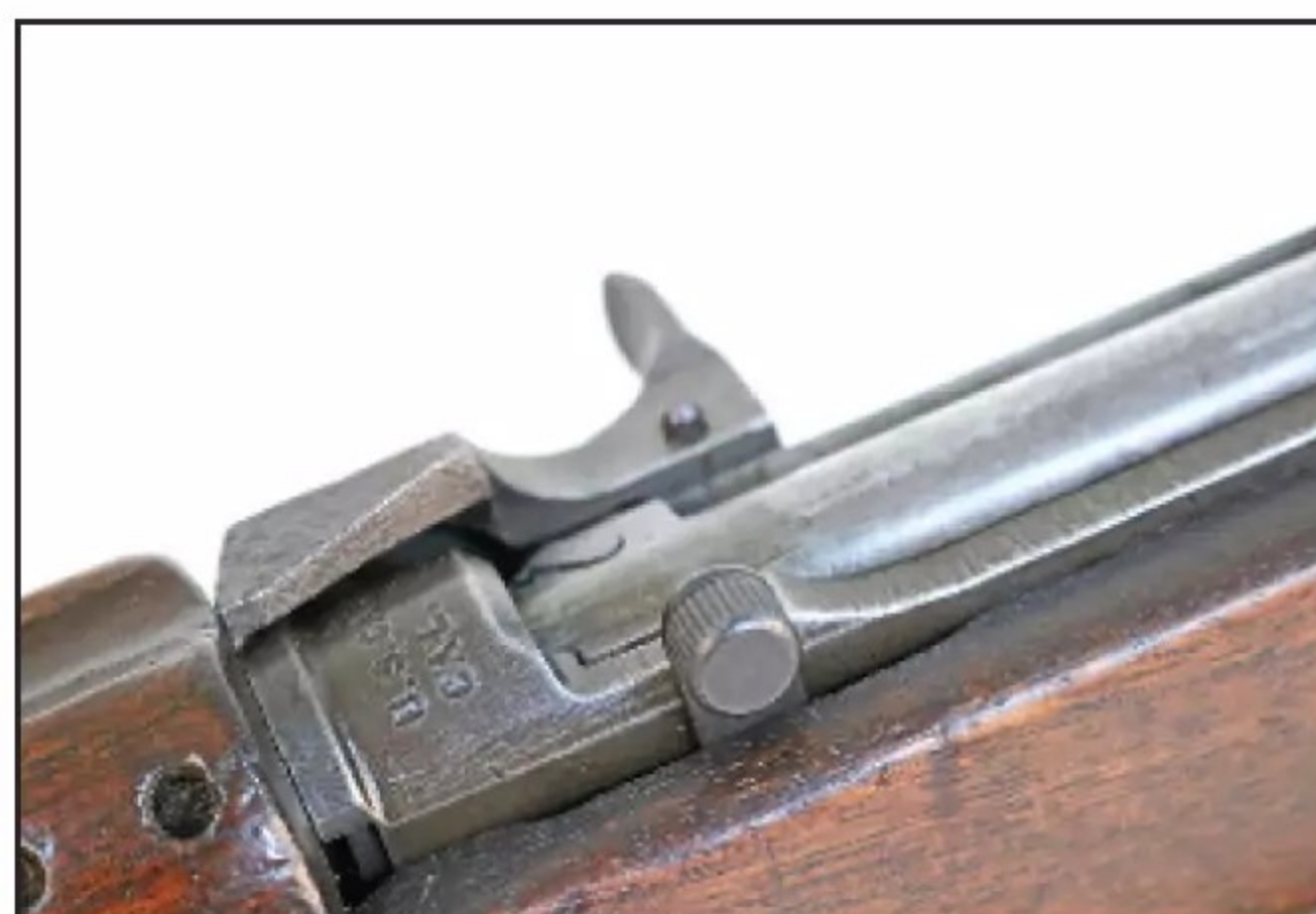
Externally, this sliding lever is really the only thing that differentiates the selective fire M2 carbine from the semiauto M1. However, that's an awfully expensive little button.
