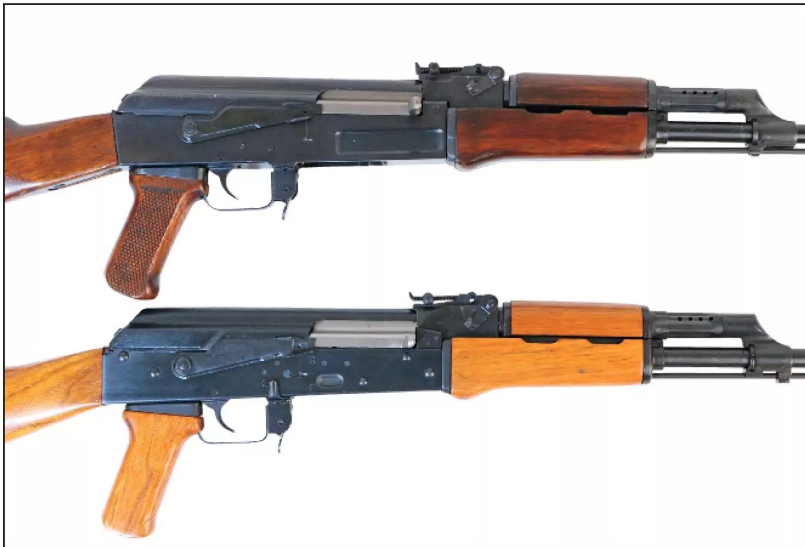
What most in the popular media call an AK-47 (top) is actually an AKM (bottom). The differences between the two receivers are obvious at a glance once you know what to look for.
