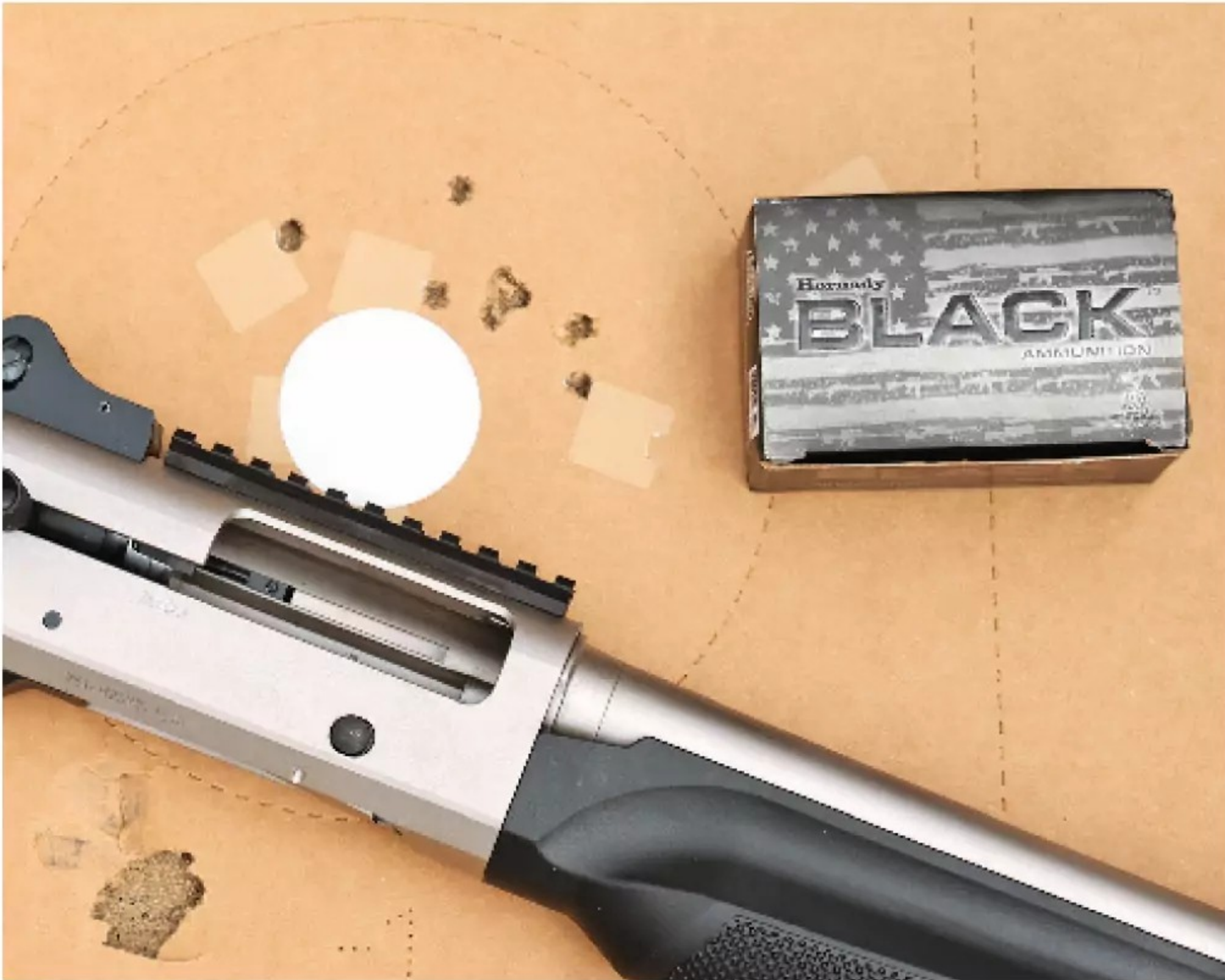
Hornady Black 00 buckshot patterns at 10 yards like it hates the cardboard. That big hole you see is the wad.
