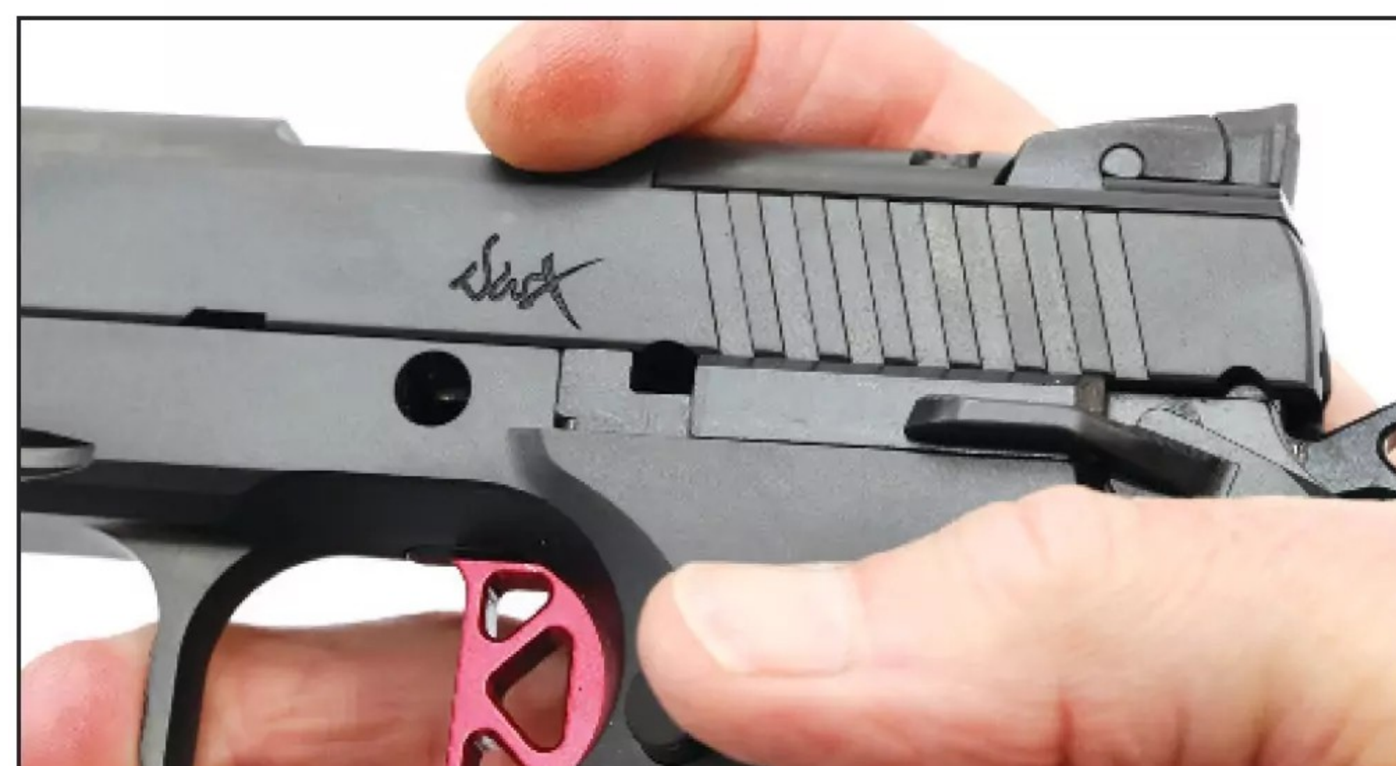
The easiest way to disassemble the DWX is by using the Vulcan-like Glock grip on it.
