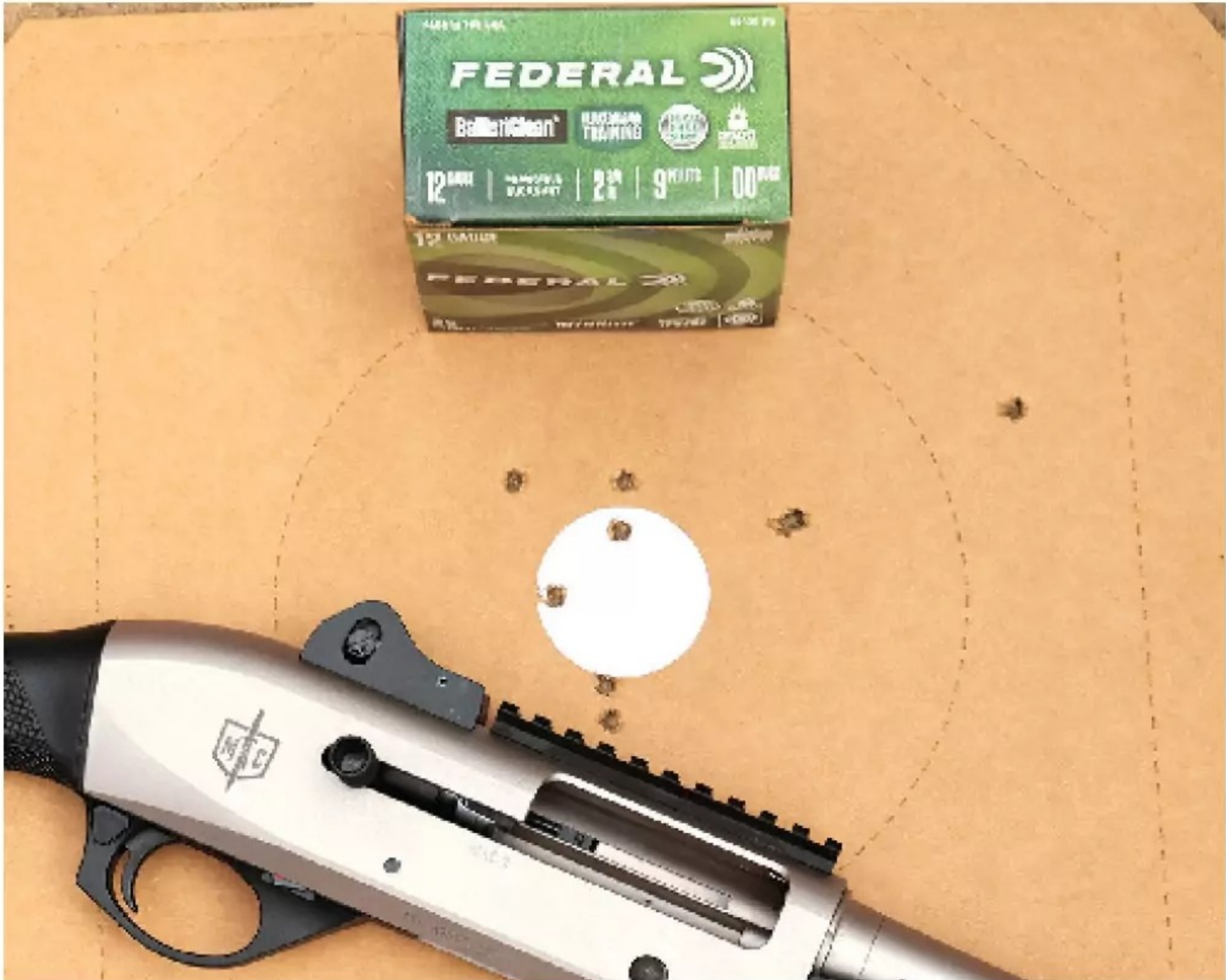
Federal no-lead buckshot (for indoor practice and indoor simulators) patterns at 10 yards as you expect buckshot to pattern.
