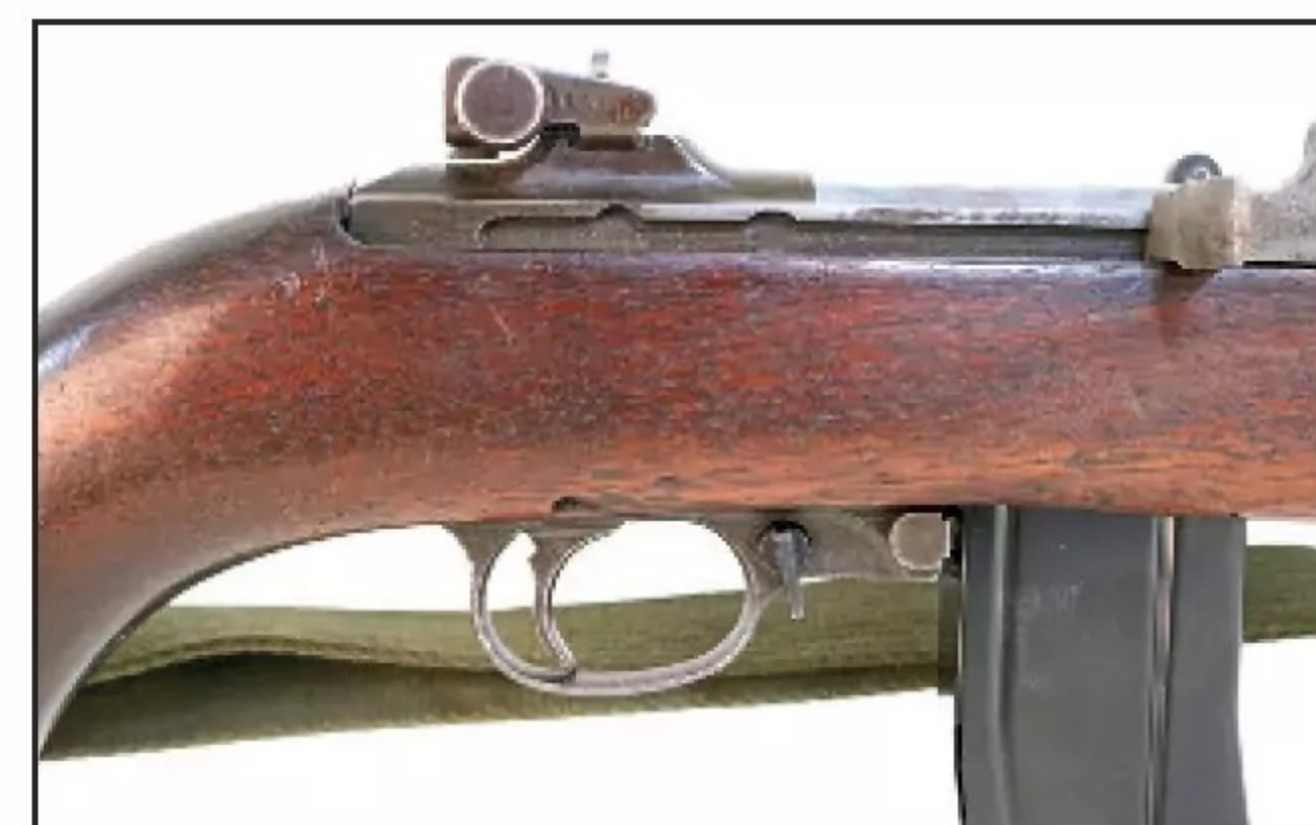
The M2 Carbine incorporated a redesigned rotating safety as well as a beefier magazine catch.
