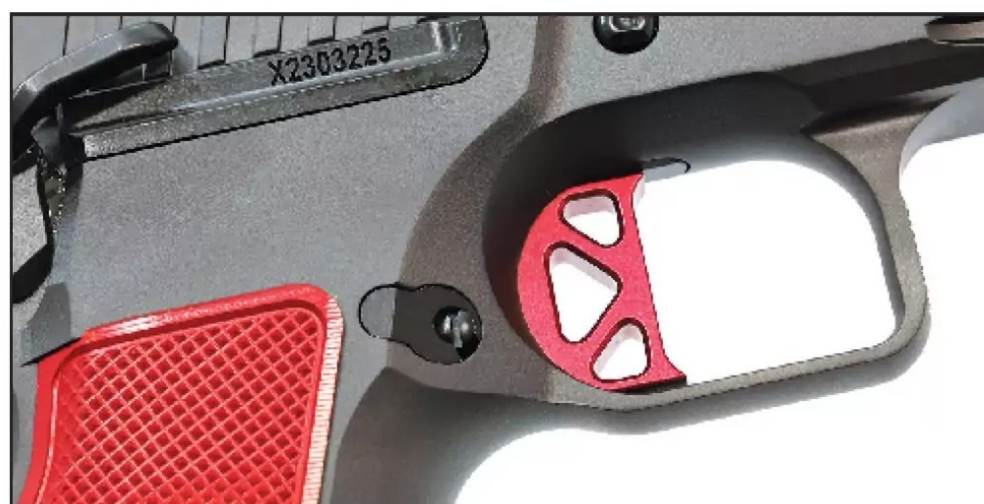
The bright part (just reflection from the lighting) is the trigger parts module, and it is the serial-numbered part, and thus the firearm. All else are only parts.
