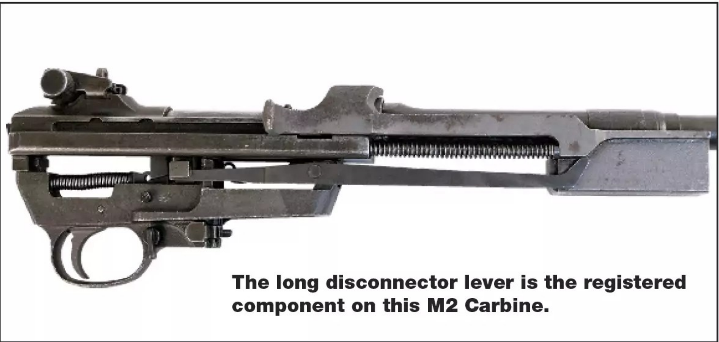
The assembled M2 Carbine action is shown here above the standard semiauto M1 sort.
