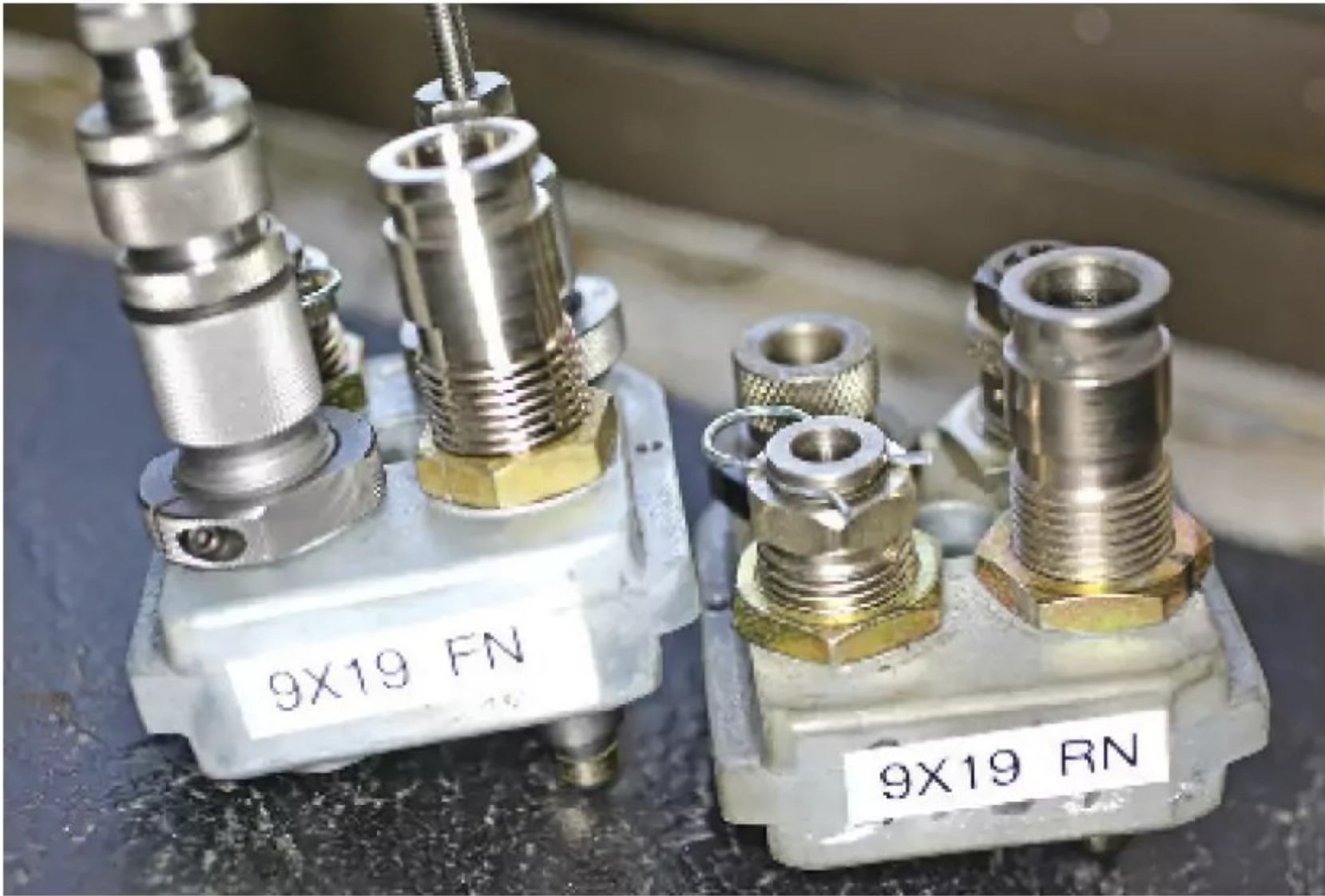
◀ One advantage of a progressive press is that you can set up different toolheads for different bullet styles.
