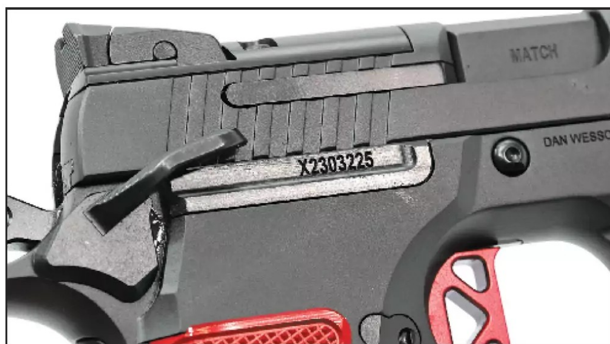
The bright part (just reflection from the lighting) is the trigger parts module, and it is the serial-numbered part, and thus the firearm. All else are only parts.
