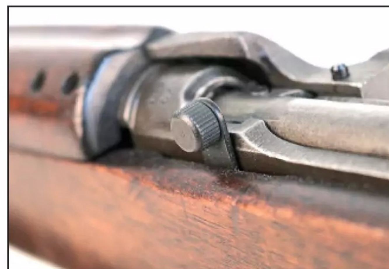
Externally, this sliding lever is really the only thing that differentiates the selective fire M2 carbine from the semiauto M1. However, that's an awfully expensive little button.
