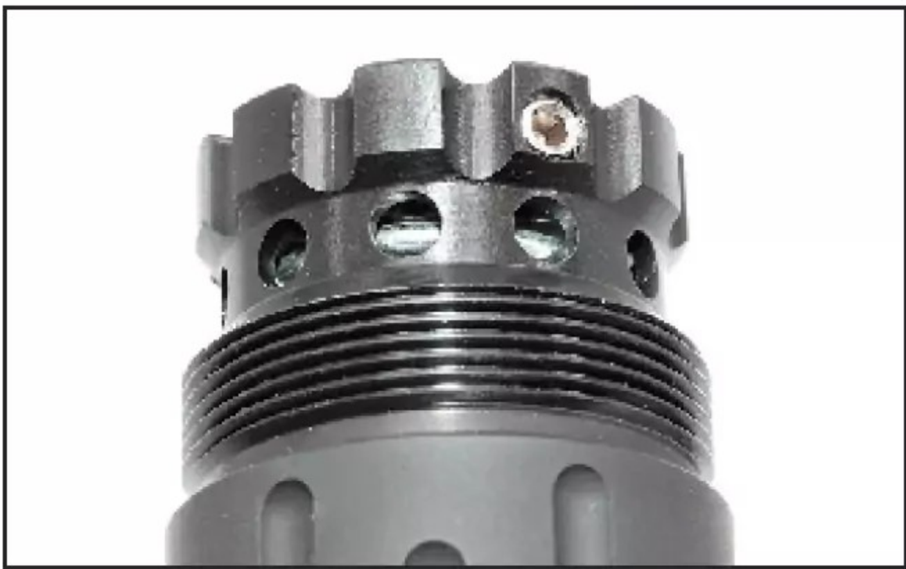
The setscrew you see is the index for the piston notches so you can shift POI if you need to.
