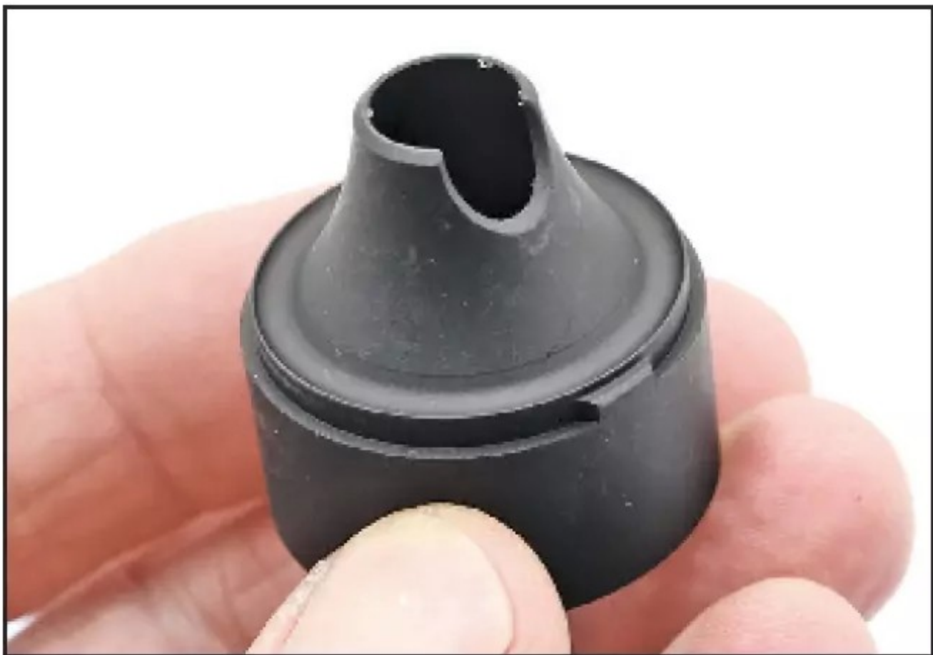
Each baffle is also notched on the entry port, to induce turbulence and thus make it quieter.
