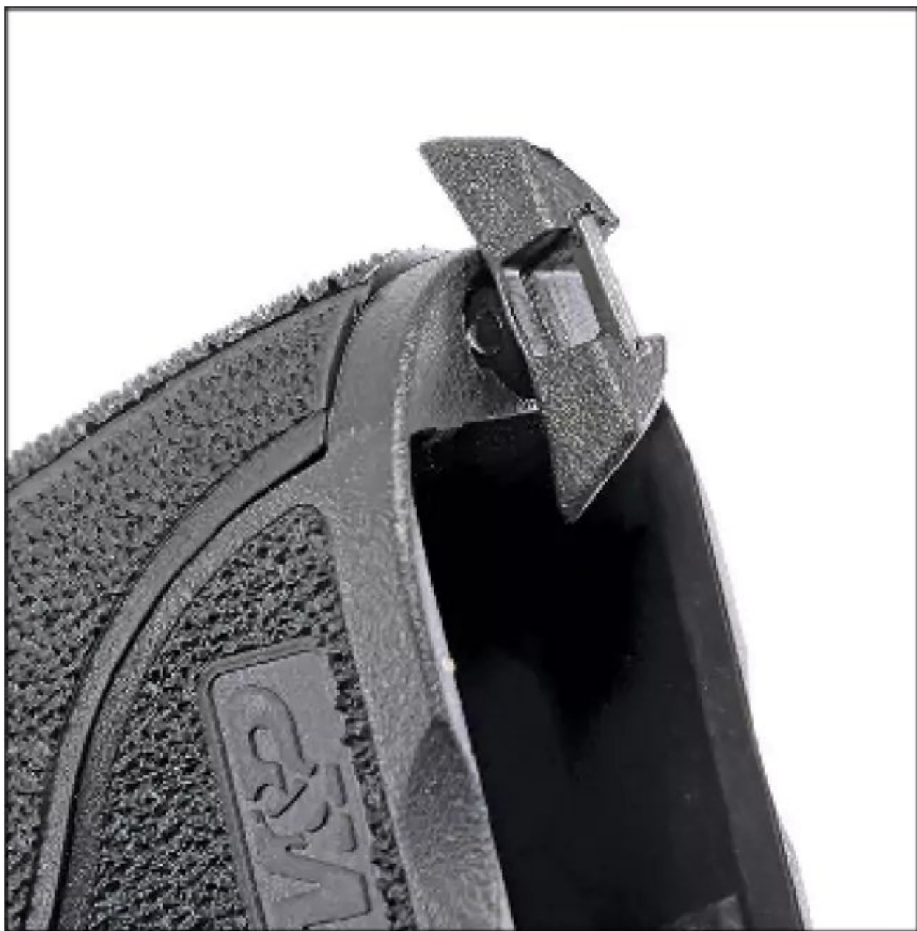
To swap backstraps, rotate the bottom ledge of the mag well opening. You can then withdraw the pin the ledge is part of. With the pin out you can hinge the old backstrap out and off, and then pivot the new one into place in its stead.
