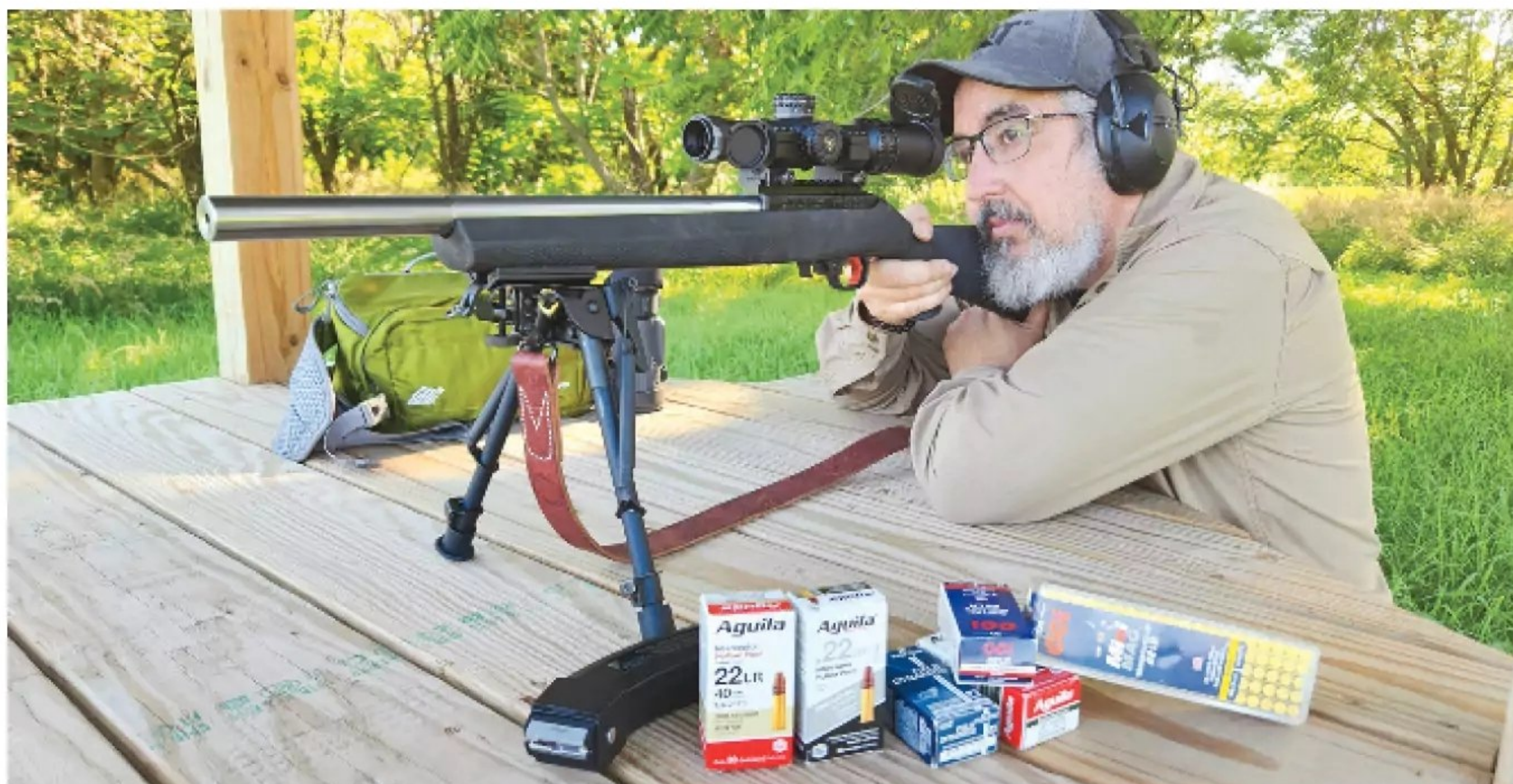
Initial testing revealed the rifle to have feeding issues with .22 LR high velocity ammunition while standard velocity and subsonic loads ran flawlessly.
