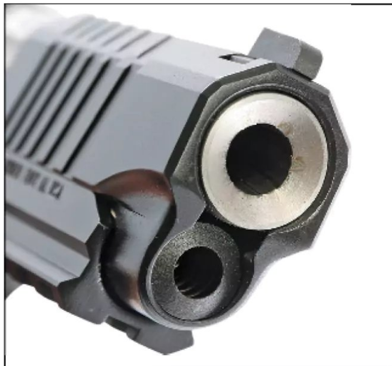
The deeply recessed crown protects the rifling, and aids accuracy. Of which there was plenty.
