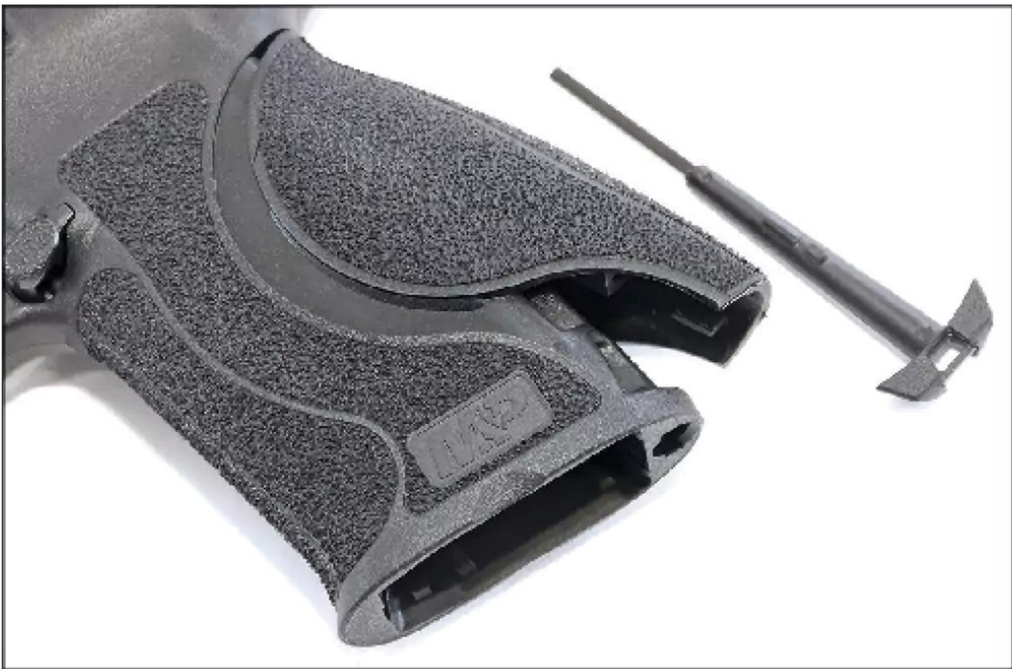
To swap backstraps, rotate the bottom ledge of the mag well opening. You can then withdraw the pin the ledge is part of. With the pin out you can hinge the old backstrap out and off, and then pivot the new one into place in its stead.
