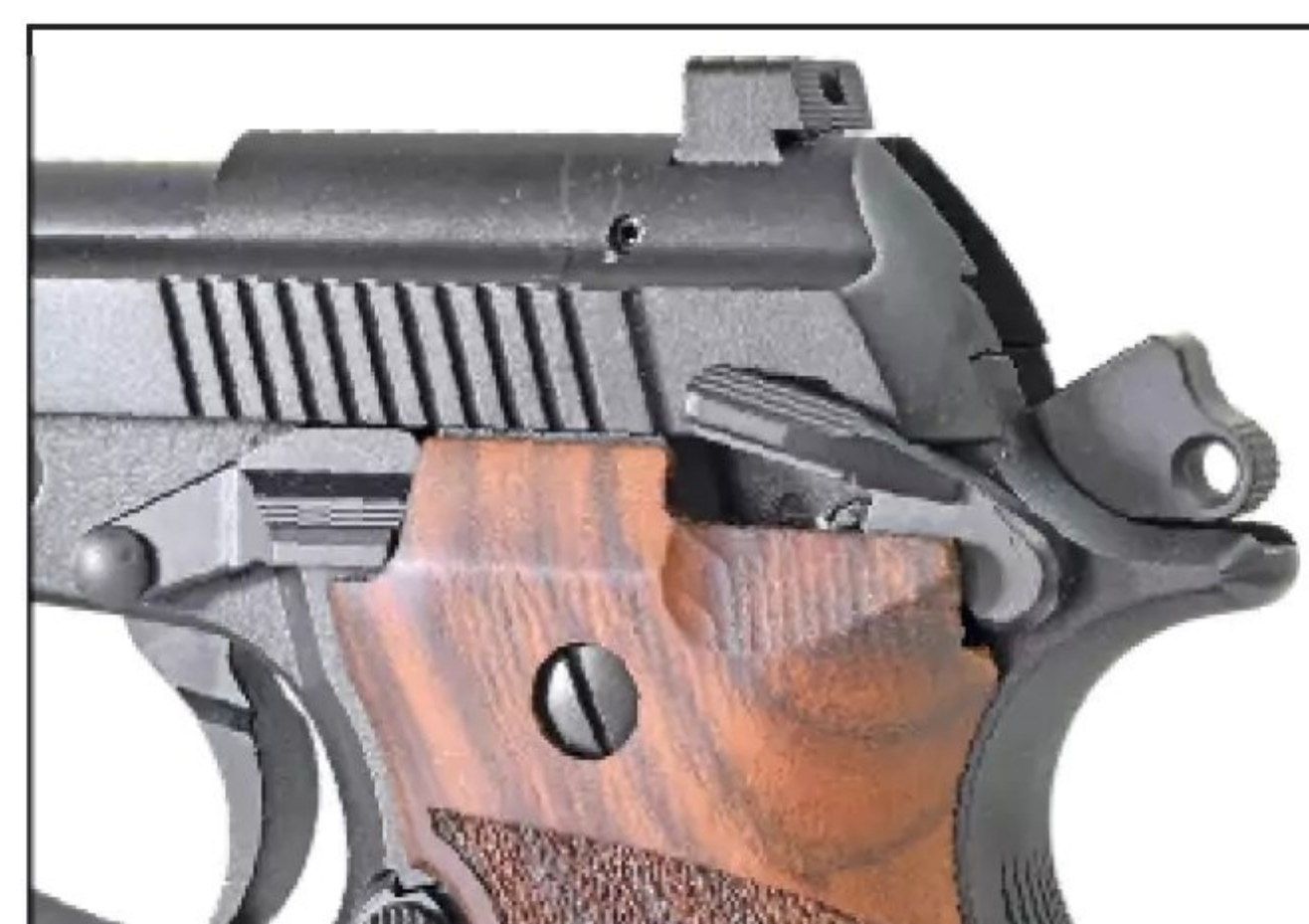
One thing Tarr really loved about the Fatih is being able to run it cocked-and-locked, the thumb safety engaged while the hammer is cocked for single-action-only operation.
