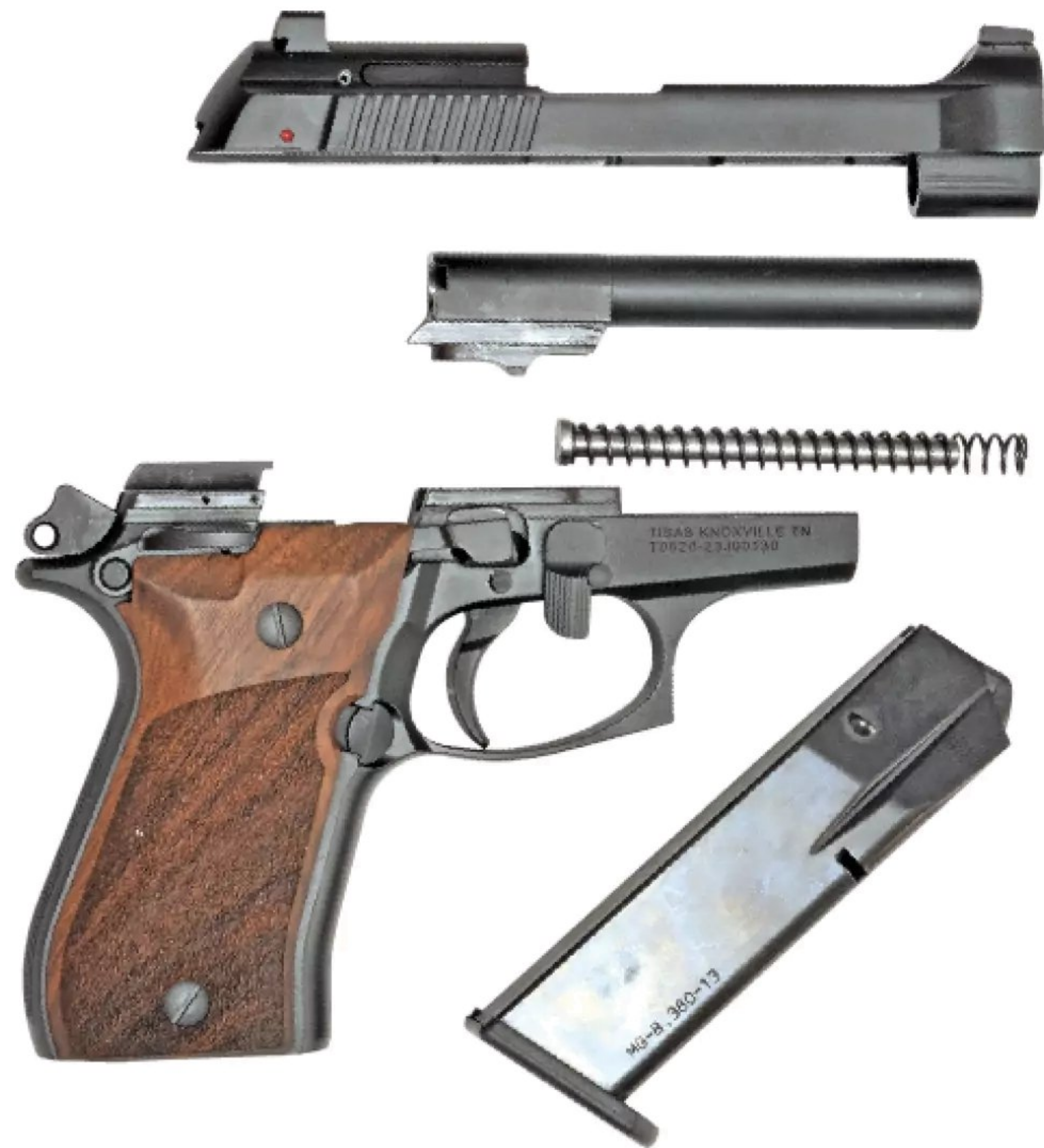
The Fatih takes down for cleaning quickly and easily. Barrel fit to frame was somewhat tight, providing good accuracy.
