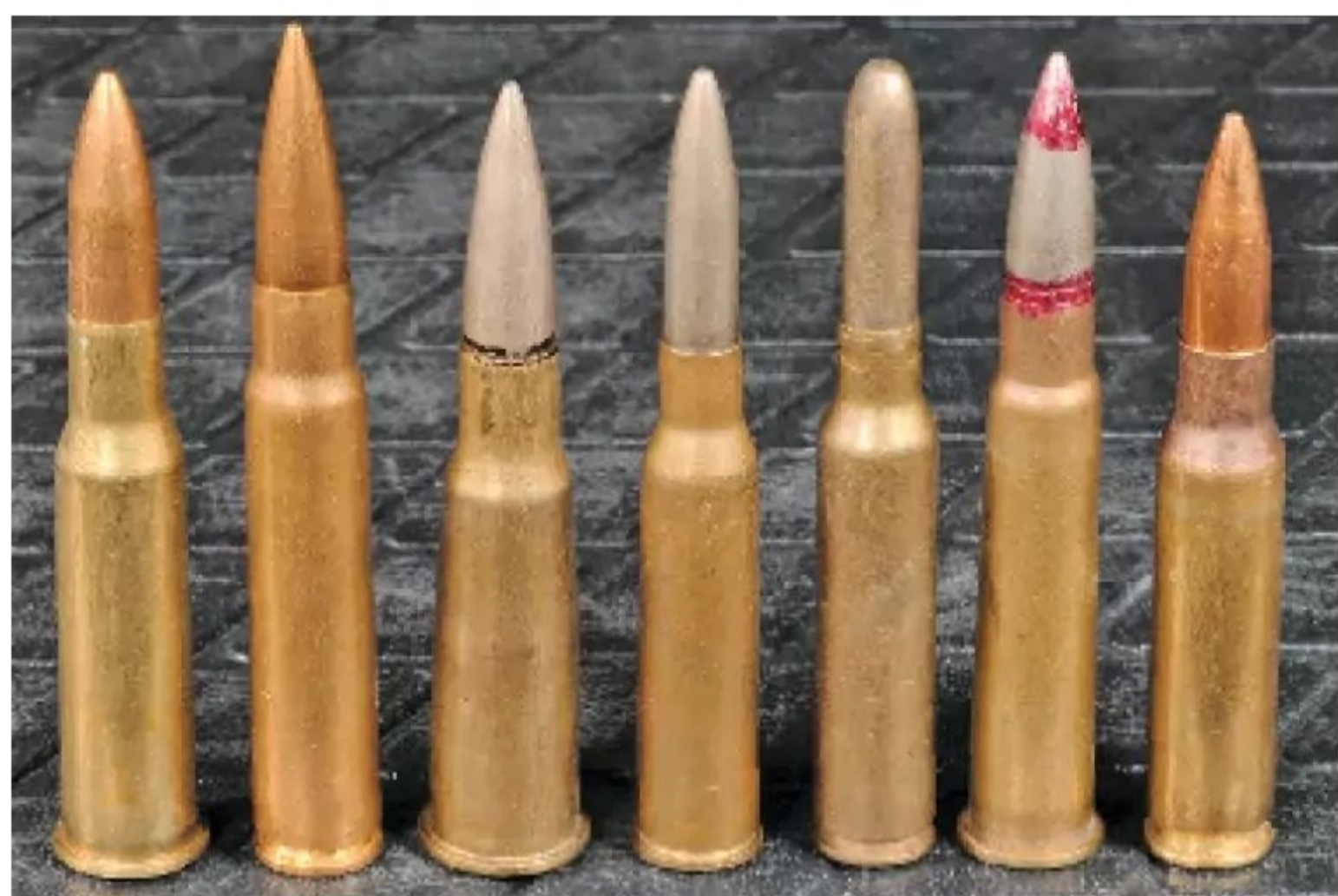
The 8mm Mauser with its peers (L to R): 7.62x54mmR, 8mm Mauser, 8mm Lebel, 6.5x50mmSR Arisaka, 6.5x52mm Carcano, .303 British and 7.62x51mm NATO.
