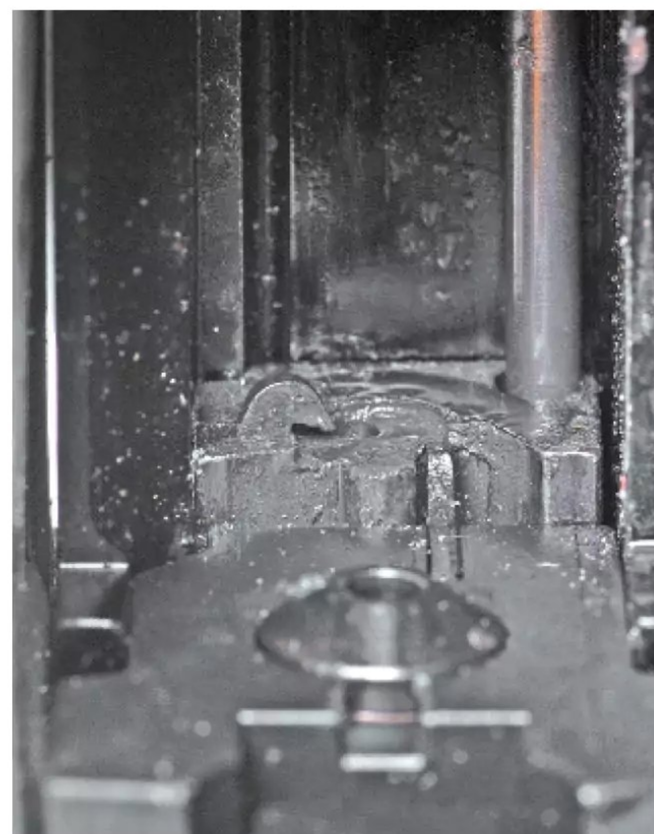
Peering inside the BC-201's action from below reveals the guide rod the bolt runs on along with the fixed ejector and claw extractor.
