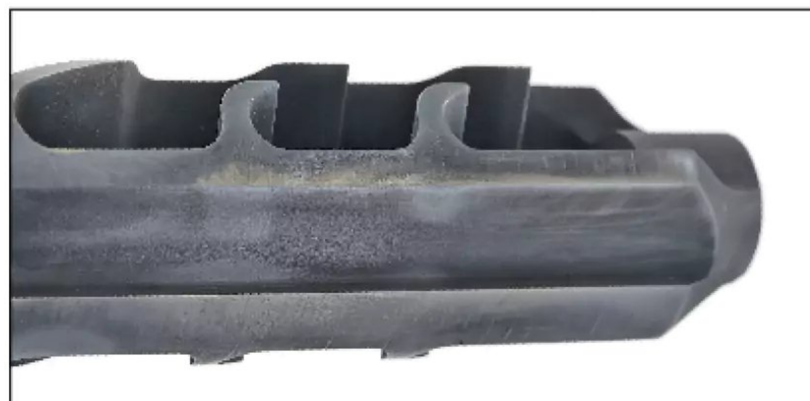
The monoco- re has scraping slots machined into the sides. They help keep it clean, but you still have to do your part.
