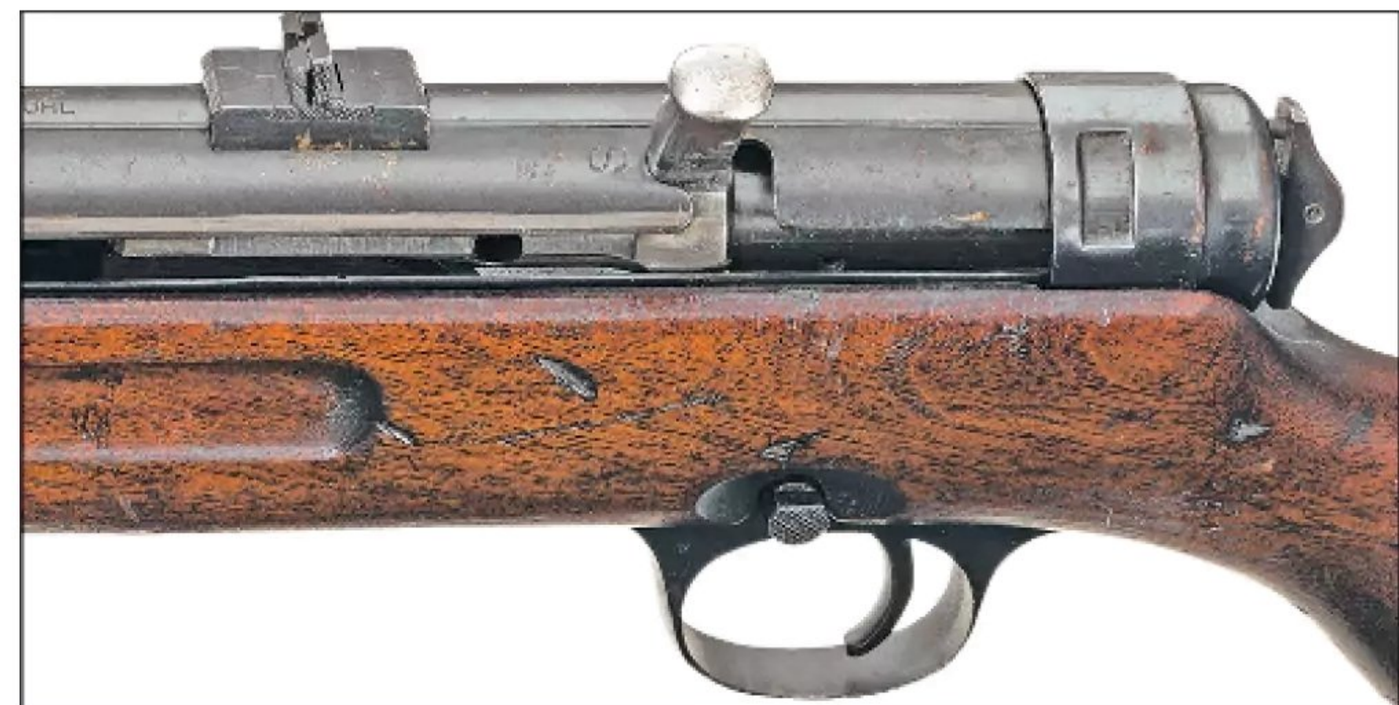
The action of the MP41 is very similar to that of the MP40 save the selective fire function built into the fire control system. (Rock Island Auctions)
