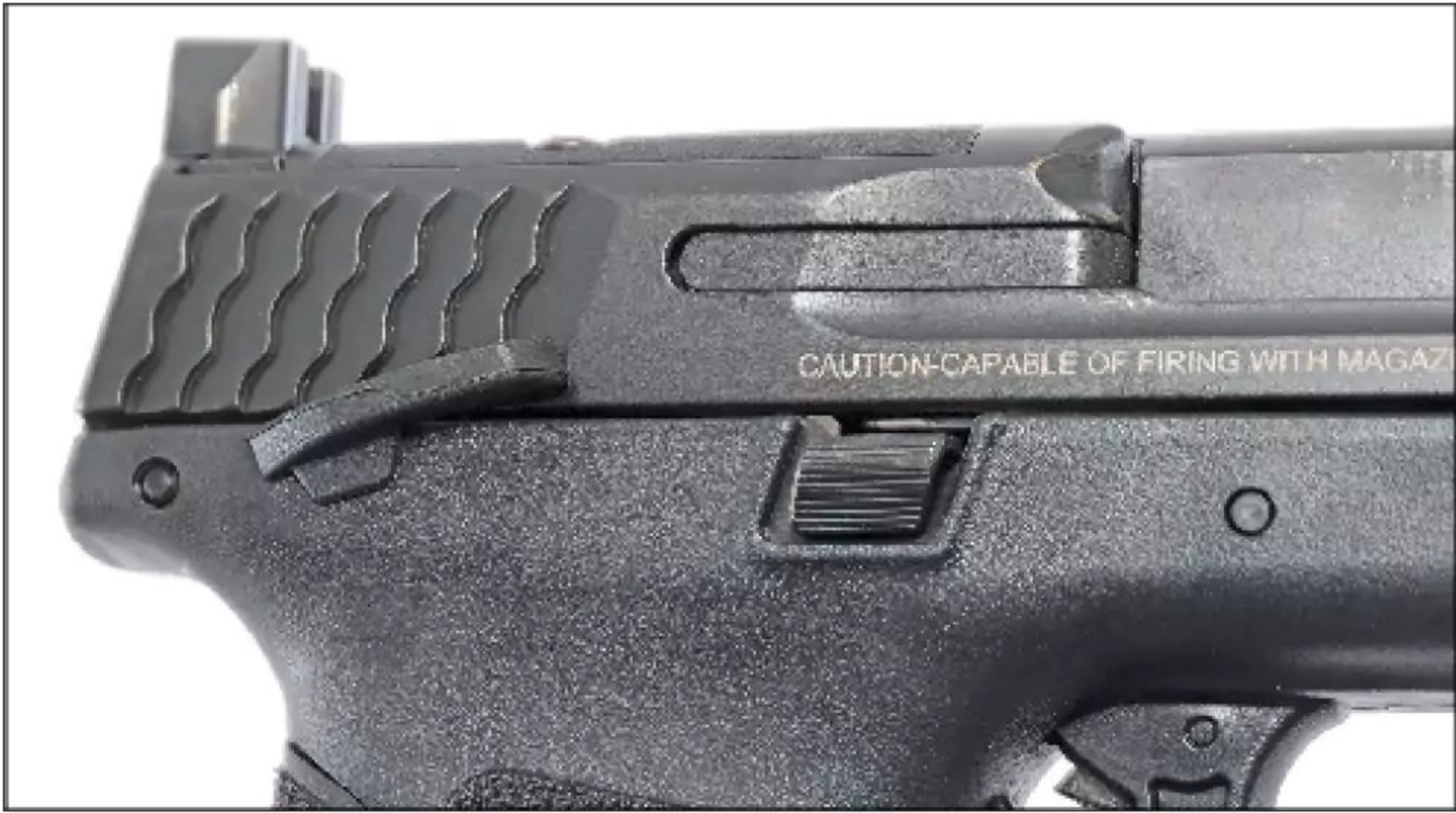
The 10mm M&P, and the hefty extractor, the ambi thumb safety and the ambi slide stop lever.
