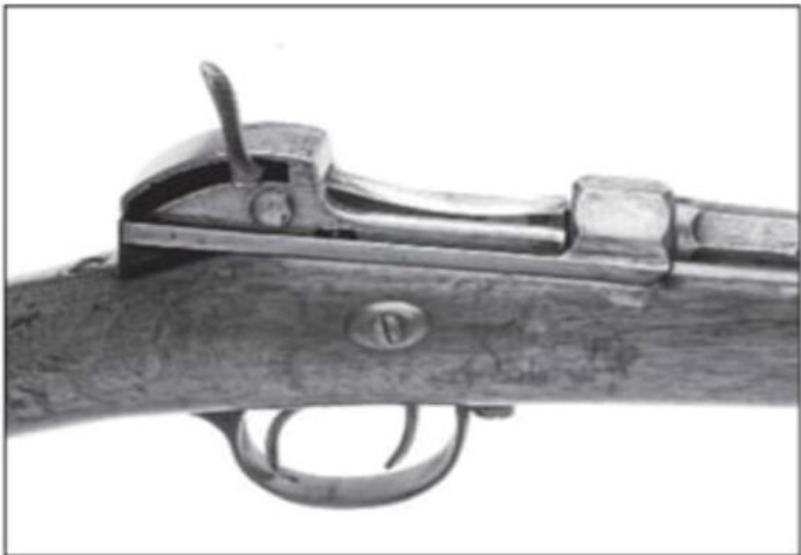
Close up of the Werder receiver. Visible here are the dual triggers and the large hammer spur projecting from the right, rear of the receiver. (James Walters photo)
