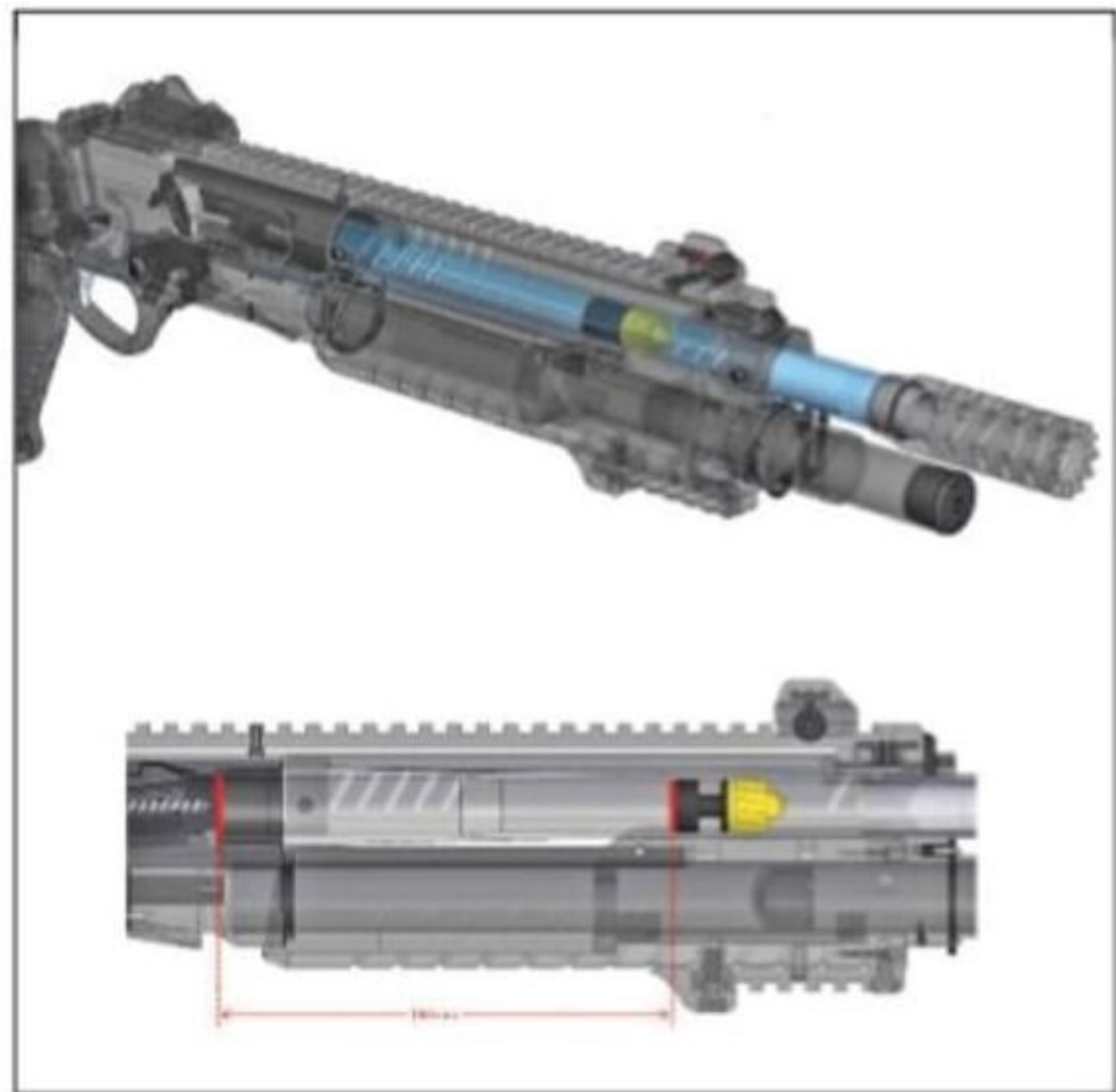
◀ A factory CAD demonstrating the obstructed bore test that the STF/12 passed with no damage to the handguard.
