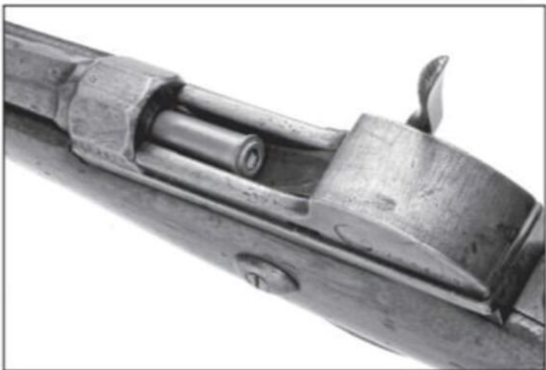
Close up of the Werder receiver. Visible here are the dual triggers and the large hammer spur projecting from the right, rear of the receiver. (James Walters photo)
