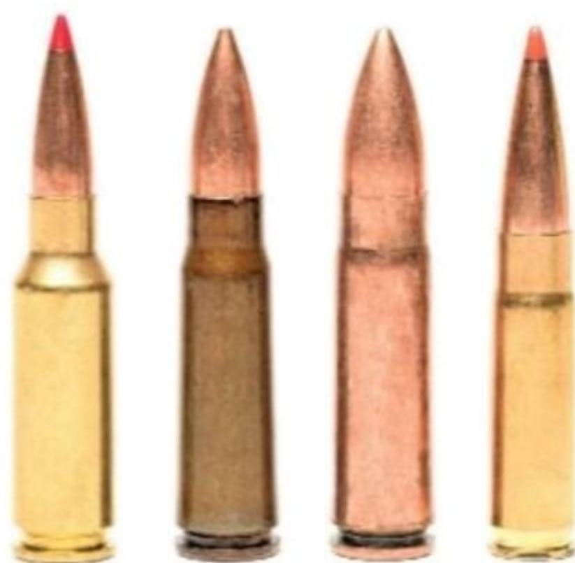
The (L to R) 6.5mm Grendel, 7.62x39mm and 9x39mm are all built on the same basic case. On right is a 300 AAC BLK. (Photo by David Fortier)
