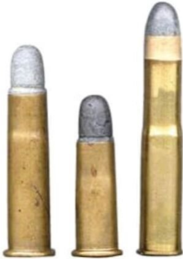
Werder rifles and carbines were chambered for the (L to R) 11mm scharfe Patrone M/69 (lang), 11mm scharfe Patrone M/69 (kurz), and the 11mm scharfe Patrone M/71. (Photo courtesy of Lou Behling)
