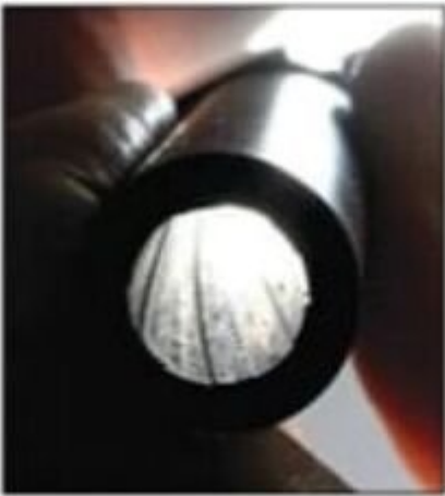
The RXM barrel uses traditionally shaped rifling, so you don't have to worry about using lead or coated bullets.
