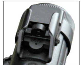
The rear peep sight is adjustable for ranging, to engage targets within 100 and 200 meters respectively.
