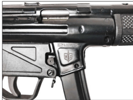
The stamped receiver design is a strong one; it also results in a lightweight firearm for its size. Note the button and paddle magazine releases. (Vincent DeNiro)
