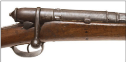
All Modello 1870 rifles and Moschetti had a sheet metal cover that could be rotated over the ejection port to keep debris out of the receiver.
