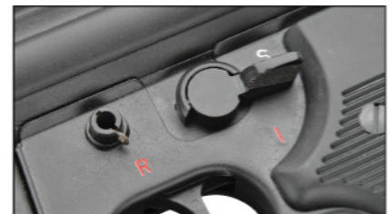
► The three-position selector is marked S for “Sicura” (safe), I for “Intermittenza” (single shots), and R for “Raffica” (full-automatic). The fire selector replaced the double push-button design in 1978, marking the transition between the PM-12 and the PM-12S.
