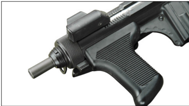
The Beretta PM-12's foregrip and reciprocating charging handle; outing this sample as a PM-12S2 is the machined bolt catch rack on the receiver, which prevents accidental discharges should the bolt be accidentally released by the gun being bumped or in case of a short stroke.
