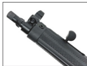
The stamped receiver design is a strong one; it also results in a lightweight firearm for its size. Note the button and paddle magazine releases. (Vincent DeNiro)
