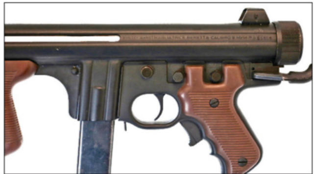
The first Beretta PM-12 incarnation featured a cross-bolt safety and a separate cross-bolt selector for single shots (“Singolo”) and full-automatic fire (“Raffica”). This solution was adopted to make familiarization easier for Italian military and police customers who were already used to the cross-bolt safety used by the Beretta M951 pistol and MAB sub-machine guns. (Photo by D&B Militaria)
