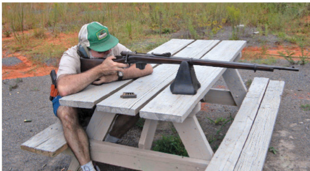
Test firing was conducted from an impromptu bench rest on my club's 75-yard range. The Modello 1870/87 fired this nicely centered group measuring 4 1/8 inches.
