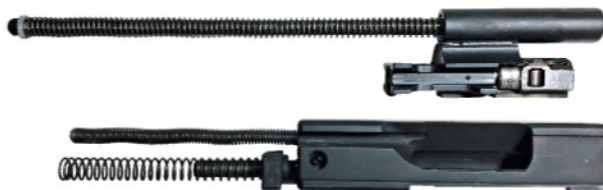
A size comparison of the 12 1/4-ounce MP5 complete bolt carrier to the 29-ounce closed-bolt UZI Carbine complete bolt assembly. (Vincent DeNiro)
