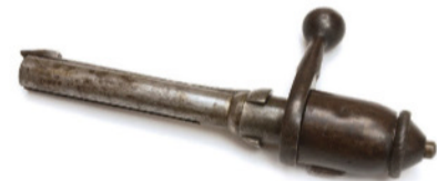
The Vetterli's bolt had dual locking lugs on the bolt handle collar. The bulbous sheet metal cap at the end of the bolt covered the mainspring.
