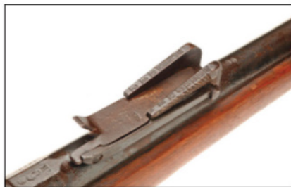
Fucili Modello 1870/87/15 were fitted with a Modello 1891 style rear sight.
