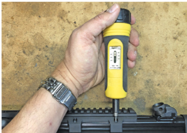
DeNiro used a Wheeler F.A.T. Wrench to tighten the bolts at 20 pounds of torque on the Midwest Industries MP5 rail mount.
