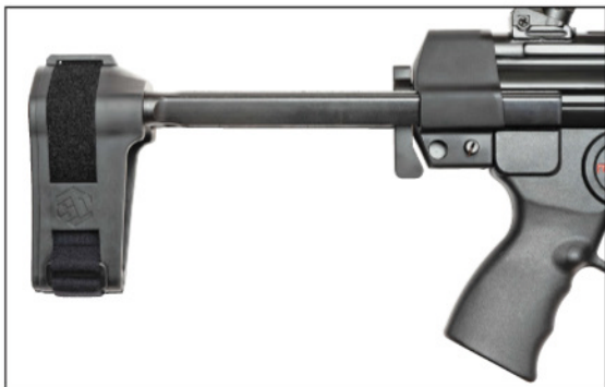
The end cap (or butt cap) of the SB Tactical brace, which includes a buffer, houses the lever-actuated mechanism which allows three brace lengths: 3.2, 5.3, and 8.0 inches fully extended. (Oleg Volk)
