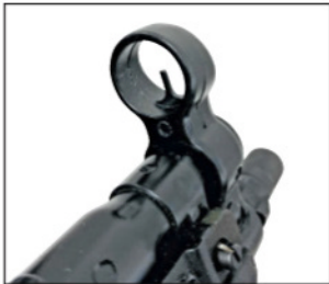
The adjustable rear sight has a four-diopter drum; this with a fully-protected blade front sight make up the “irons.” (Vincent DeNiro)
