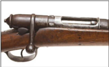
This close up of the Modello 1870 moschetto's receiver shows the safety lever behind the bolt handle and spur-less trigger guard.
