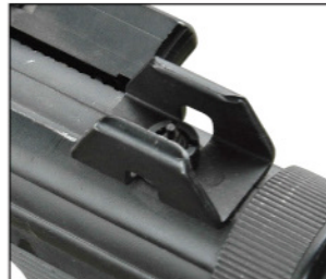
The height-adjustable front post of the PM-12S2. On the first PM-12, the sight was protected by a full hood.
