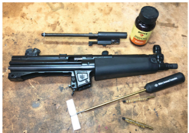
The cleaning kit includes a bore-swab tip, two bore brushes (nylon and brass), metal cleaning rod, and its case doubles as a handle. (Vincent DeNiro)
