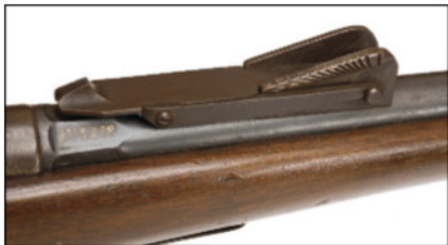
The Fucile Modello 1870/87 used a quadrant-style rear sight. This is the latter model designed for M90 smokeless powder ammunition and adjustable to 1,800 meters.
