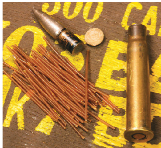
A look inside a .303-inch Mk VII round showing its “spaghetti”-like cordite propellant, flat base projectile and over powder wad.
