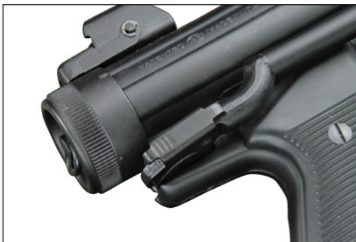
◀ A latch allows the wire metal stock to be extended or folded to the right side, cutting the overall length of the PM-12 almost in half for transport or convenient use in close quarters, from within vehicles, or under a trench coat for close protection details.
