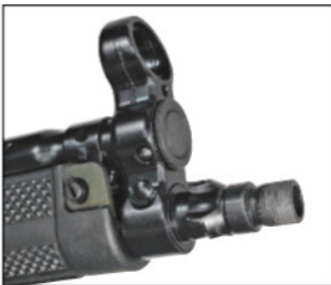
The muzzle is threaded for 1/2x28 (with thread protector), and also has the three-lug quick-attach and -detach feature for muzzle attachments. (Vincent DeNiro)
