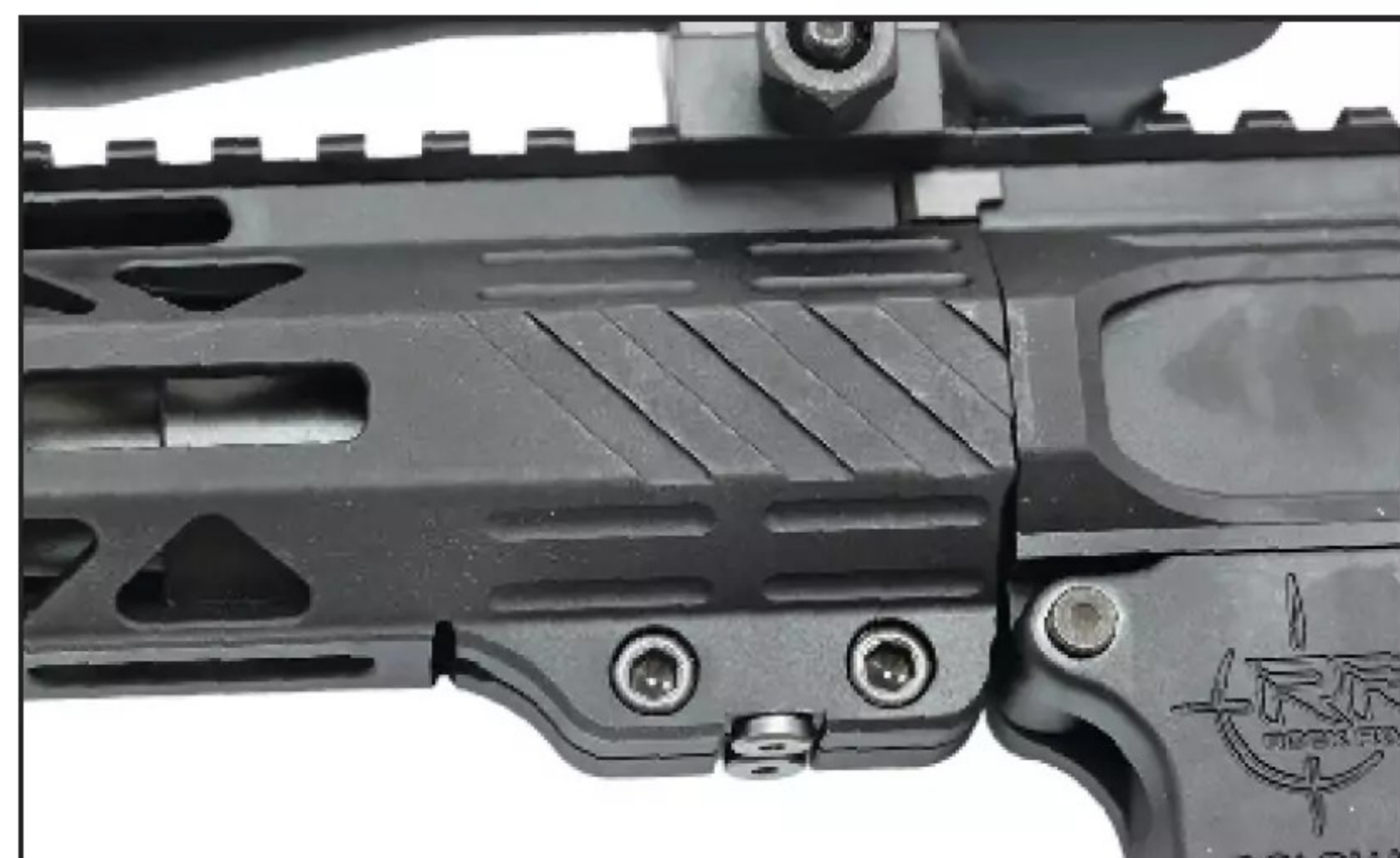
◀ The Rock River handguard has indexing tabs (steel) to keep the handguard aligned with the upper receiver. And the handguard clamps onto the barrel nut. (Patrick Sweeney)
