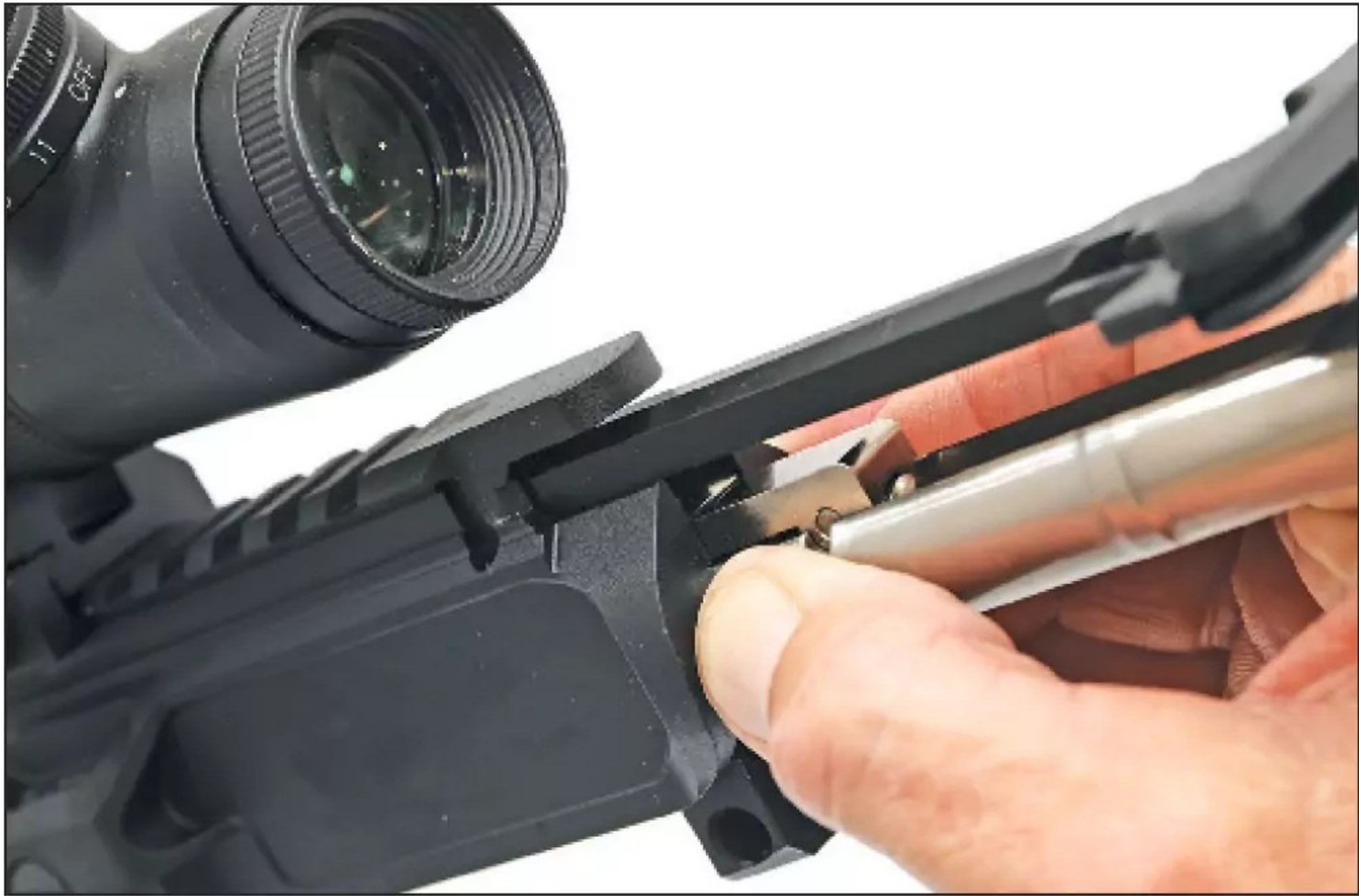
Keep the ball bearings retracted and let the rear of the upper receiver push your fingertips off of them as you install the carrier. (Patrick Sweeney)
