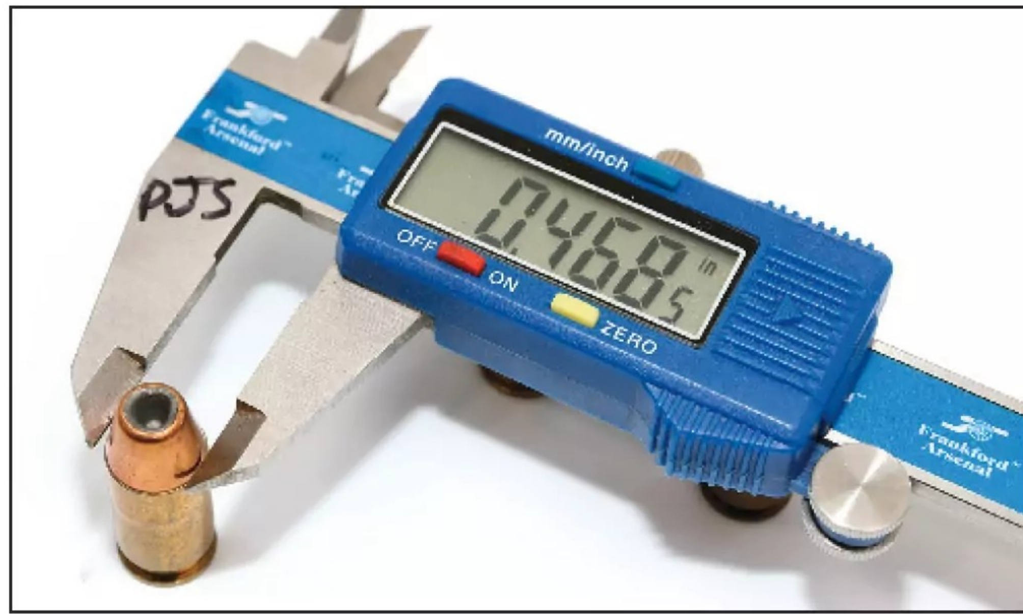
Crimp is important, and the .45 ACP gets only a taper crimp. Here, .468 of an inch is correct. (Patrick Sweeney)
