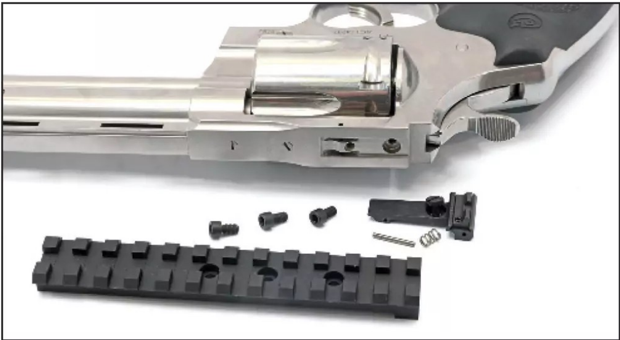
To uncover the third mount screwhole for the scope mount, you have to remove the rear sight. (Patrick Sweeney)
