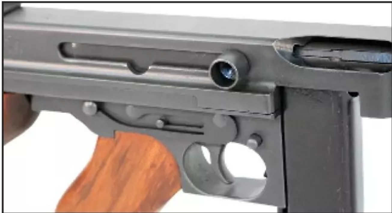
The charging handle on the M1A1 Thompson was a simple peg oriented on the right side of the gun. (Will Dabbs)
