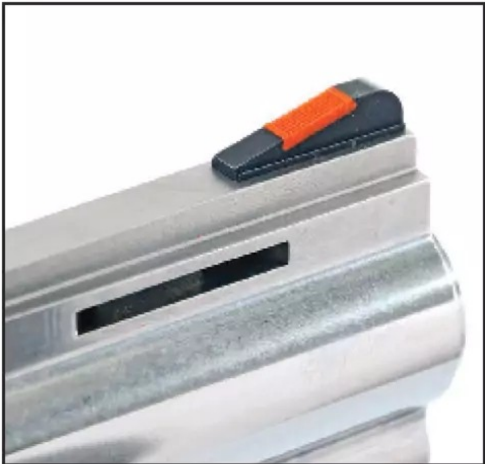
The front sight of the Anaconda is a ramp with a red insert. This is classic, and still useful. (Patrick Sweeney)
