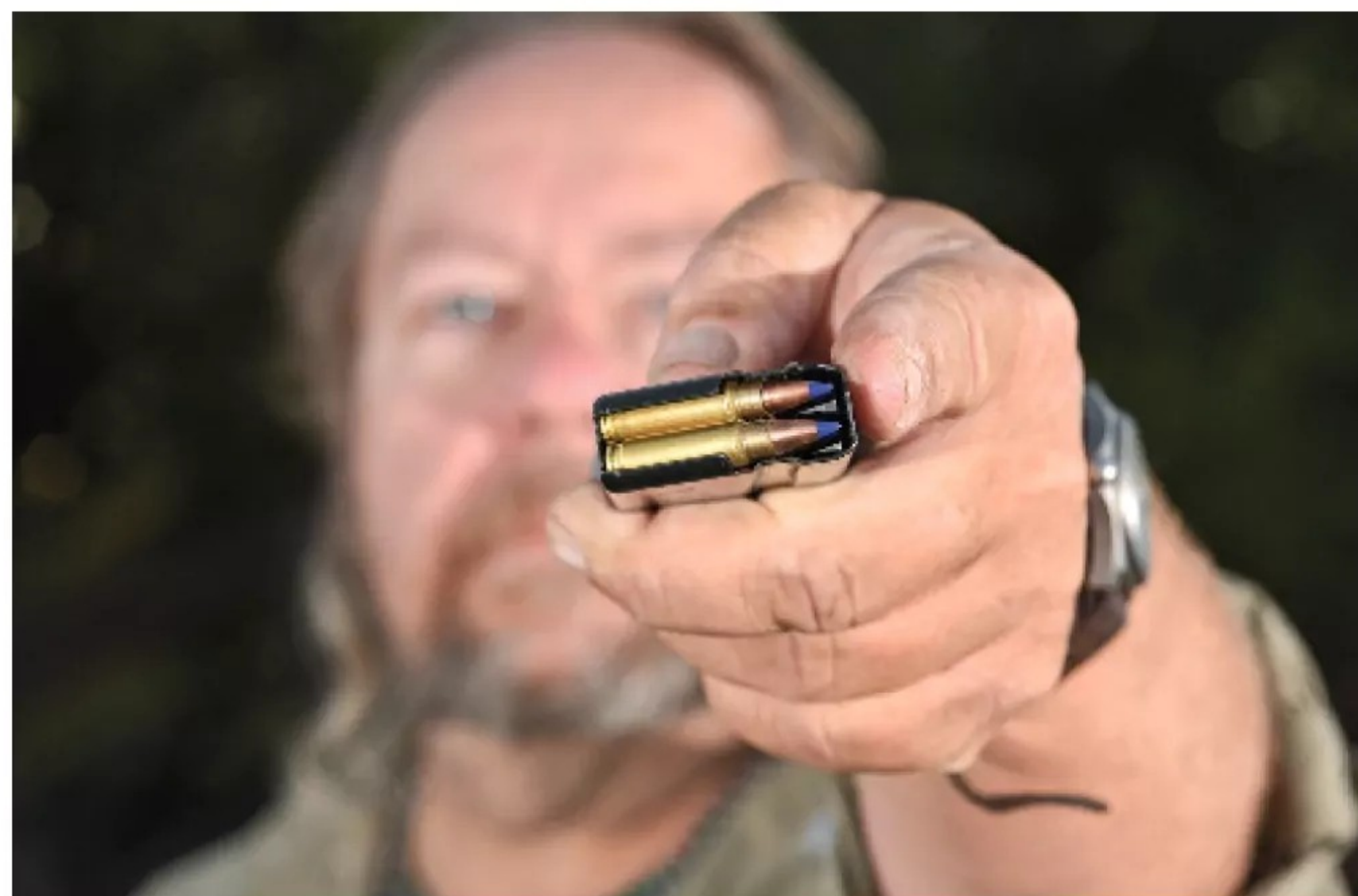
The original LC Carbine was chambered for the bottleneck high velocity small-bore 5.7x28mm cartridge seen here. (Photo by Ashley Jaderborg)
