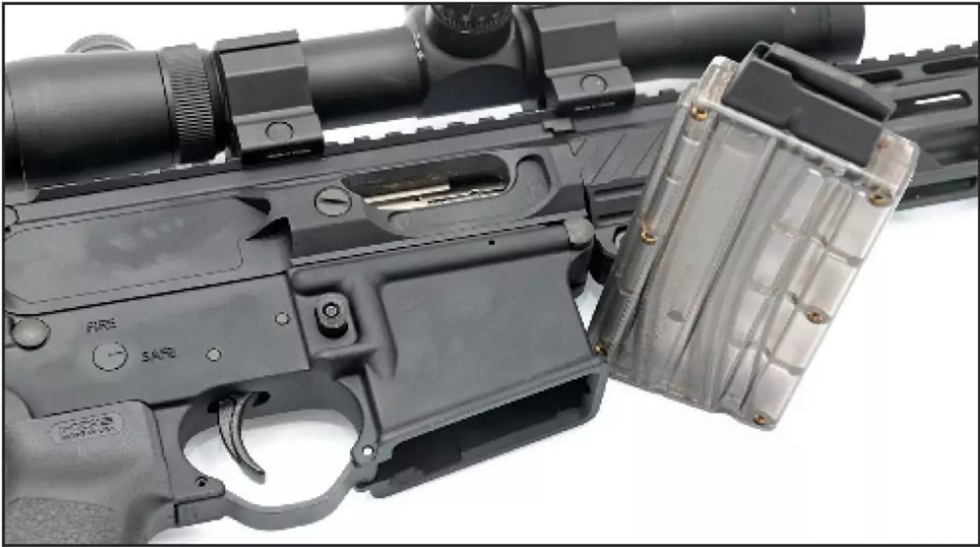
▲ The Black Dog Machine magazines fit into a regular mag well, so the Rock Chuck doesn't need a special adapter for its magazines. (Patrick Sweeney)
