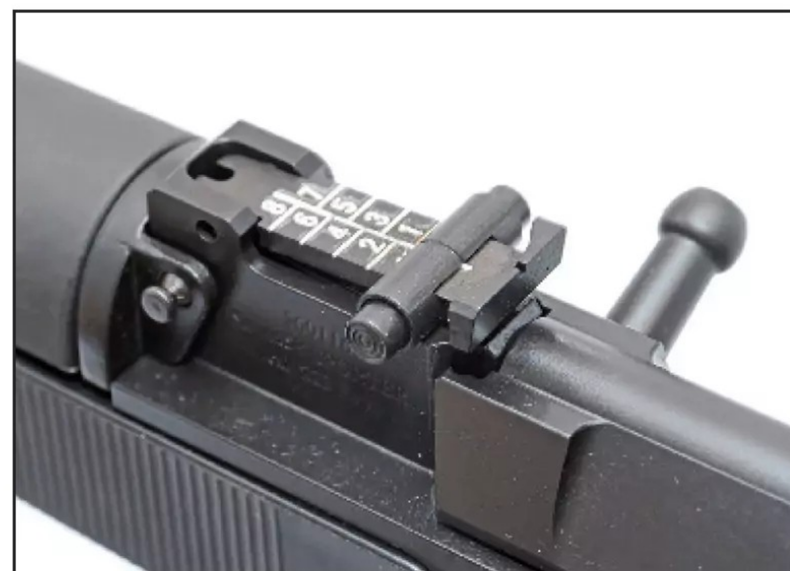
The standard Soviet sidemount scope attachment base, permanently attached to the receiver. (Patrick Sweeney)
