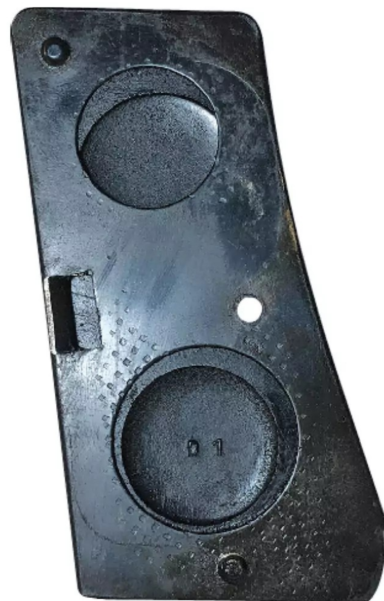
Both grip panels are reinforced with sheet steel as shown on the inside of this right grip panel. (Vincent L. DeNiro)
