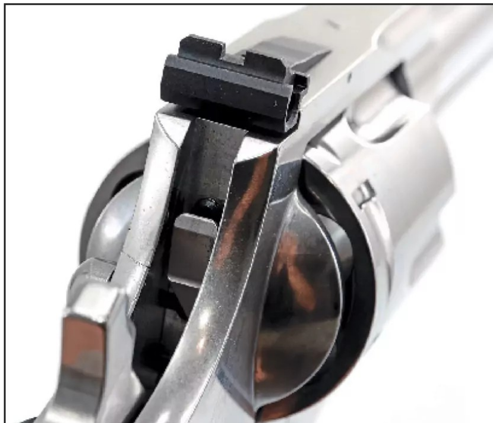
The firing system uses a transfer bar to connect the hammer to the firing pin. So the Anaconda is safe to carry fully loaded. (Patrick Sweeney)
