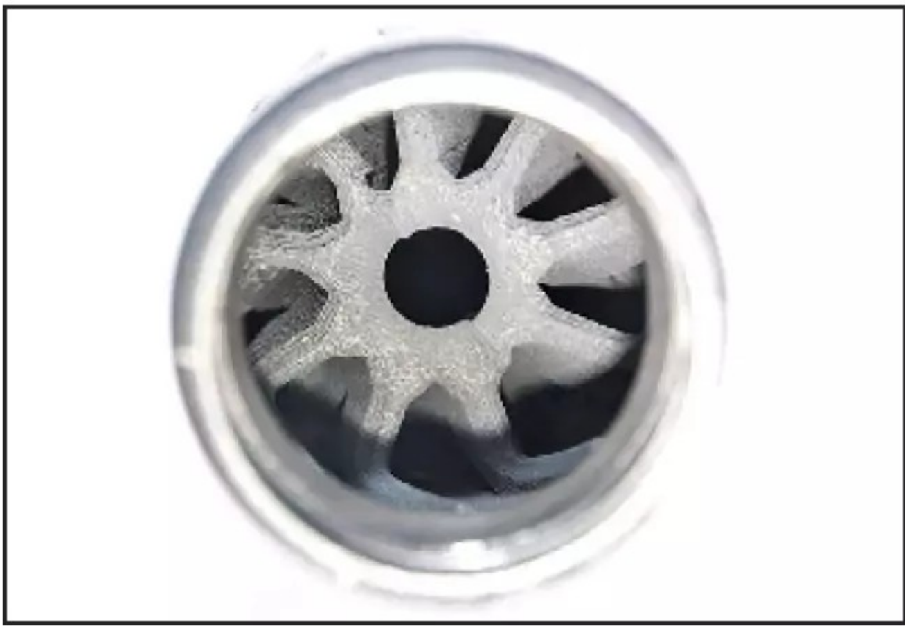
Looking into the rear of the Sandman X, at the blast chamber, you can see the kind of complex manufacture that 3D printing can accomplish, and that traditional manufacturing processes cannot. (Patrick Sweeney)
