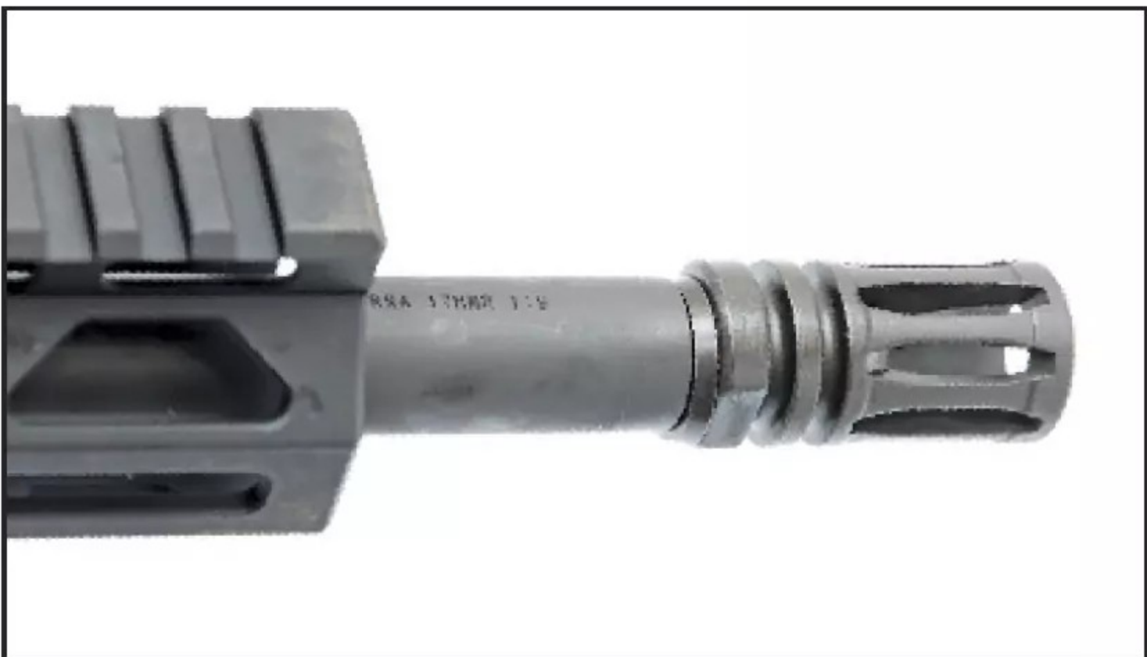
The .17 HMR Rock Chuck has a threaded barrel, so you can install a suppressor if you wish. Just be certain it is spec'd for the .17 HMR. (Patrick Sweeney)
