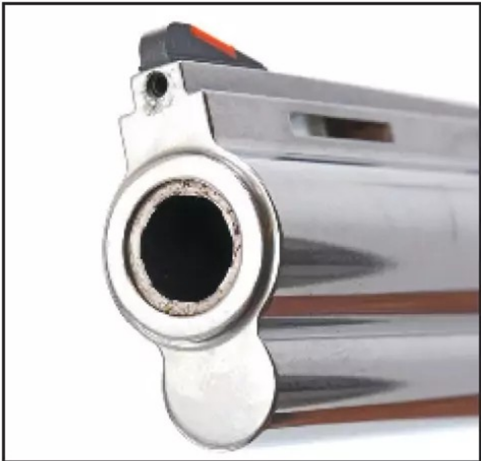
Above the recessed crown, the Anaconda sight is held in place by means of an allen screw in from the front of the rib. This holds the sight in and is easier to manage than the roll pins of yore. (Patrick Sweeney)
