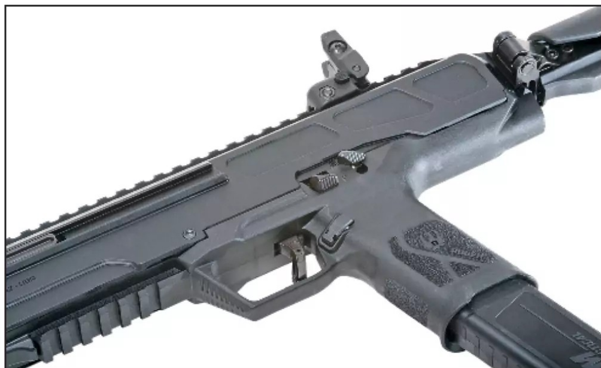
The controls are similar to the Ruger-5.7 pistol and include ambidextrous manual safety levers, a bolt release lever on the left side and a magazine release. (Photo by author)
