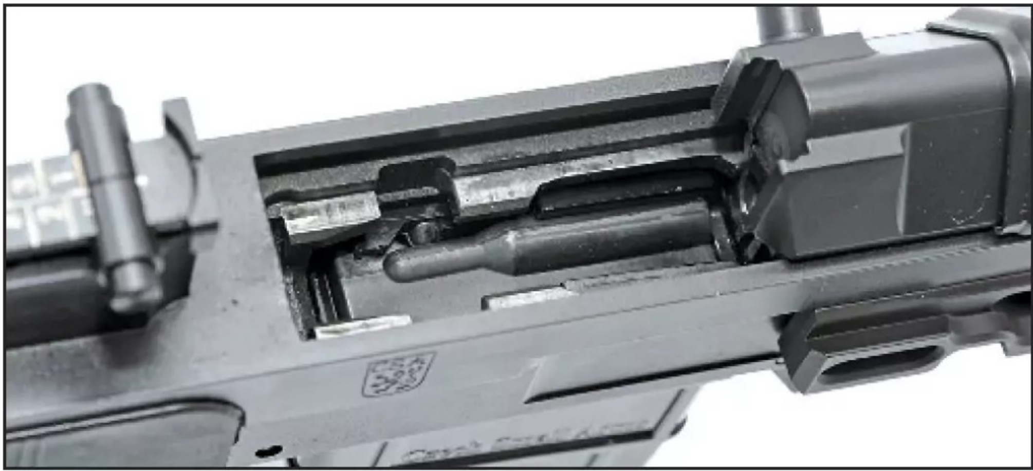
Ejection port? Really? The entire upper opens up to allow brass free exit to the rifle, its job having been done. (Patrick Sweeney)
