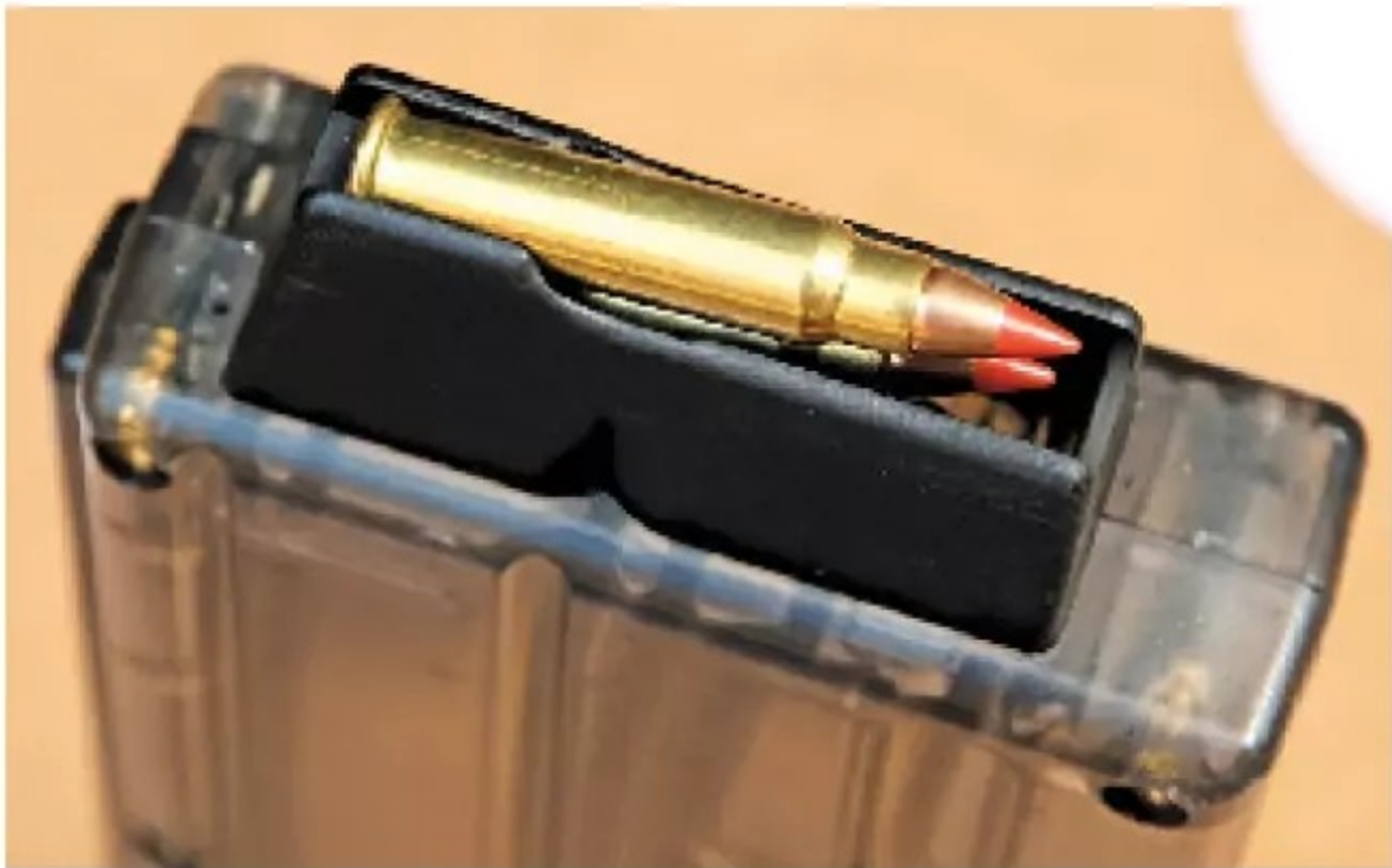
► The Black Dog magazines feed from a single point, unlike the centerfire AR-15, which feeds from alternating sides. (Patrick Sweeney)
