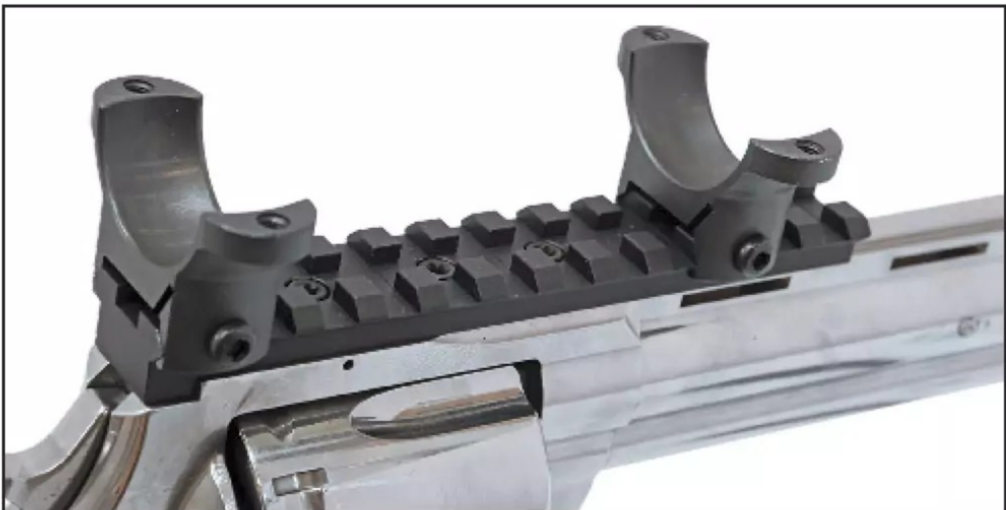
When mounting a scope, place the rings as far apart as you can while not contacting the front or rear bell of the scope. (Patrick Sweeney)
