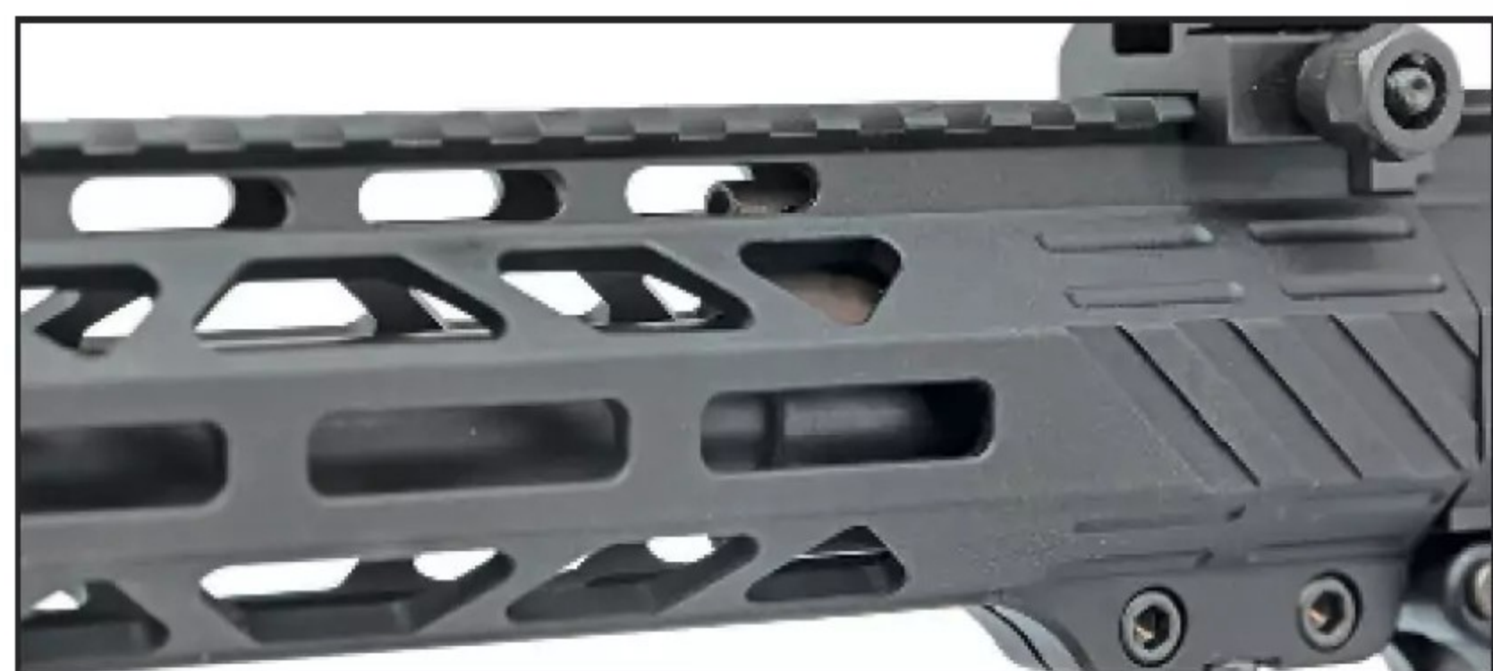
The gas block is barely visible at the rear of the handguard. Yes, a gas block, on a rimfire. (Patrick Sweeney)
