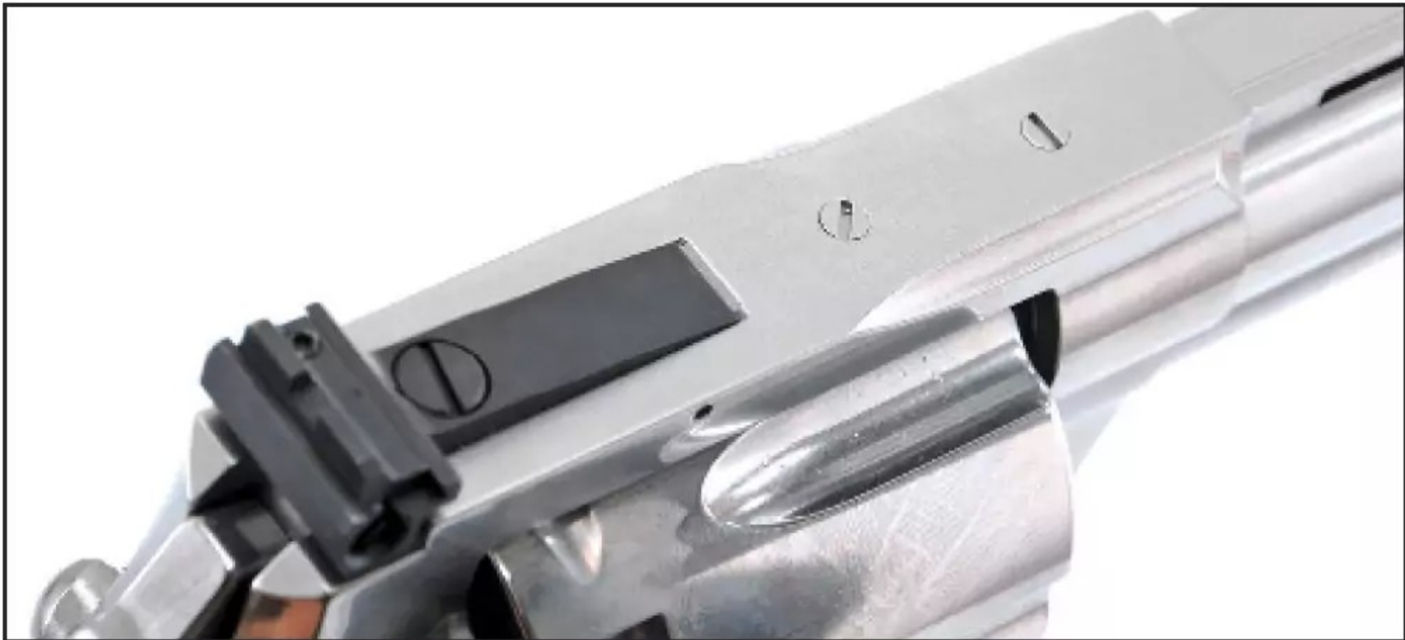
The rear sight is click-adjustable for windage and elevation. Ahead of it, you can see two of the three scope mount screws. (Patrick Sweeney)
