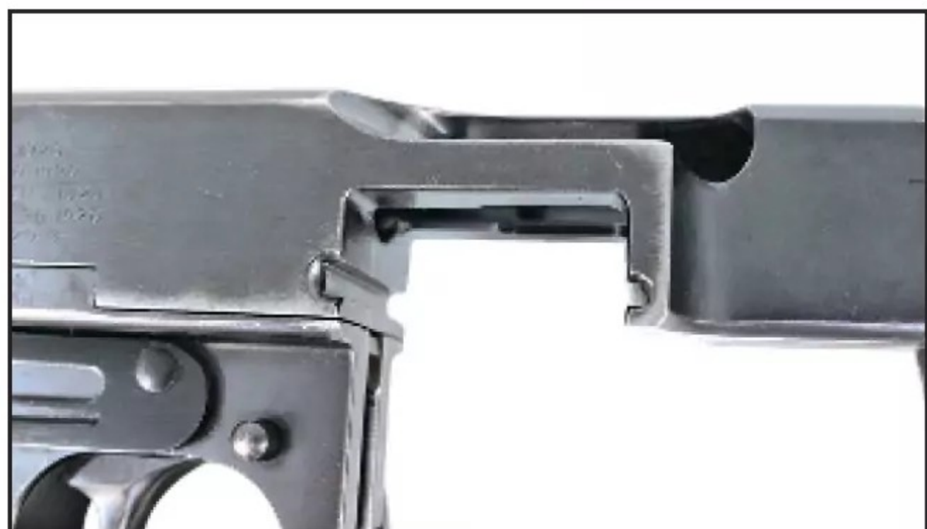
The slots cut in the receiver of early Thompsons were necessary to accommodate the 50- and 100-round drum magazines. (Will Dabbs)
