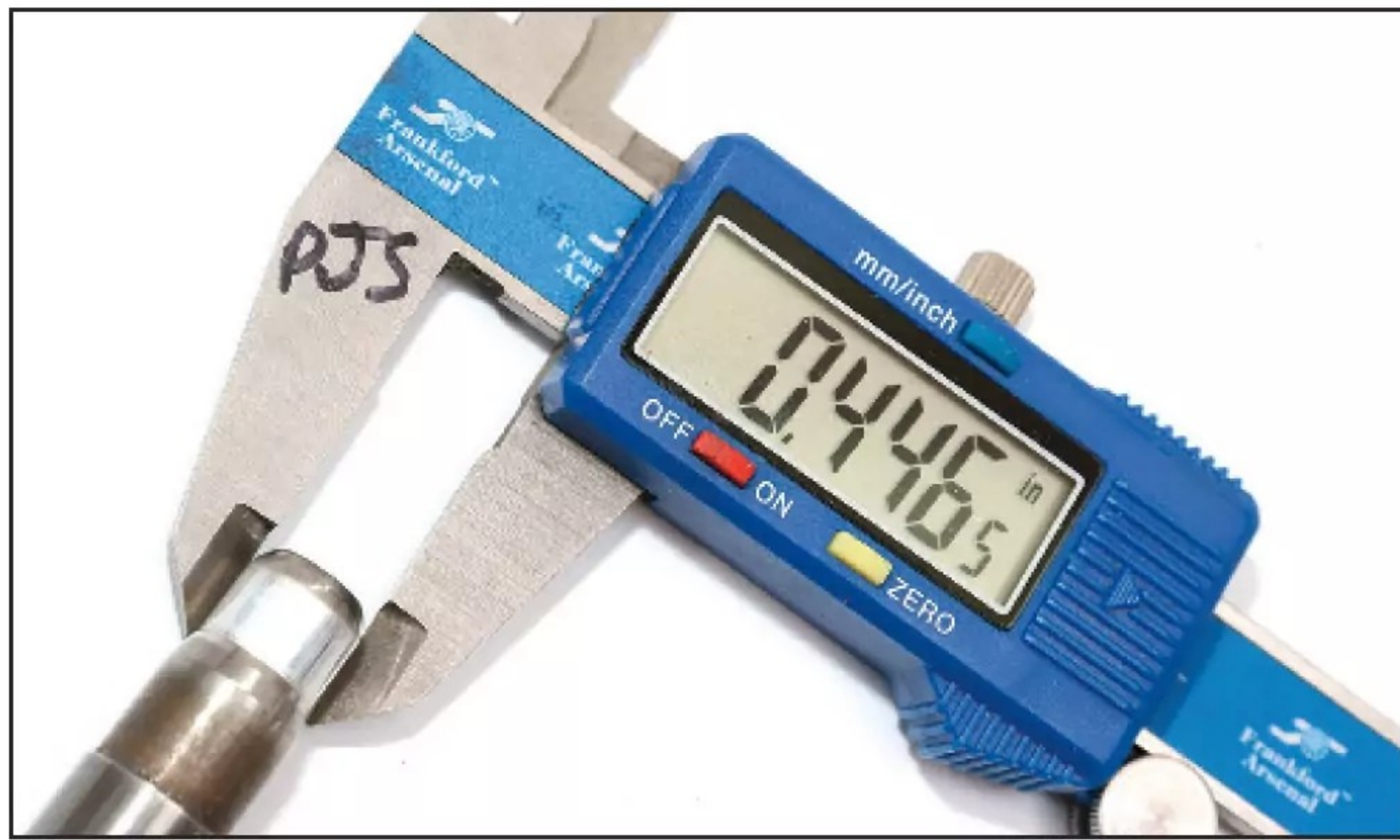
The powder drop tube, which is also the neck expander, should be .446 of an inch for the .45 ACP. (Patrick Sweeney)
