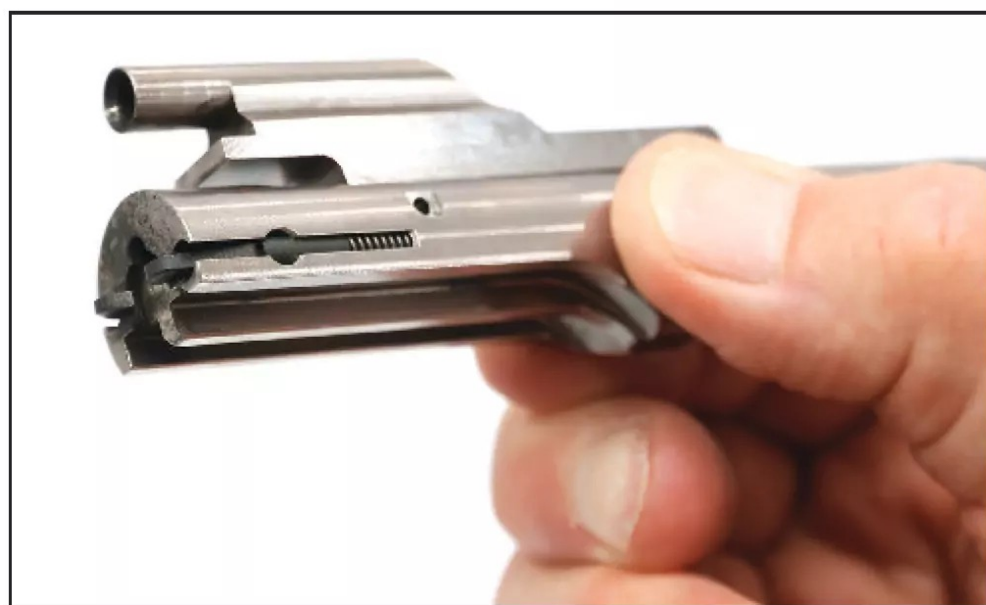
In order to insert the carrier assembly you need to keep the ball bearings retracted. Pinch them in this way once you have pushed the gas key back. (Patrick Sweeney)
