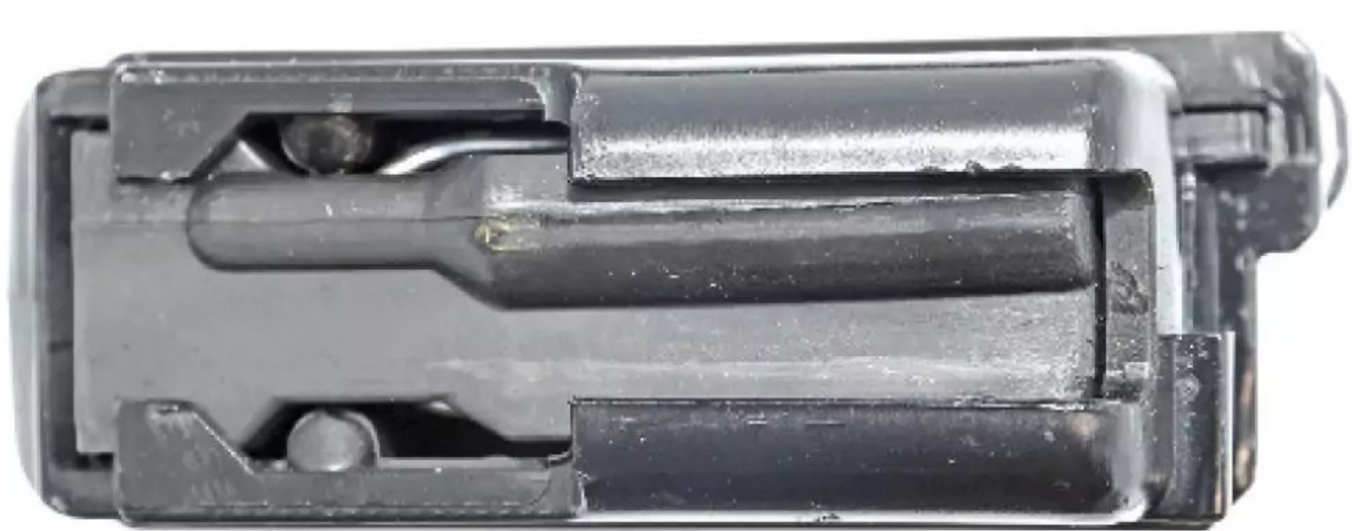
The magazines are polymer and have a bolt hold-open tab, that rides in the offset spine on the rear of the magazine as seen here. (Patrick Sweeney)
