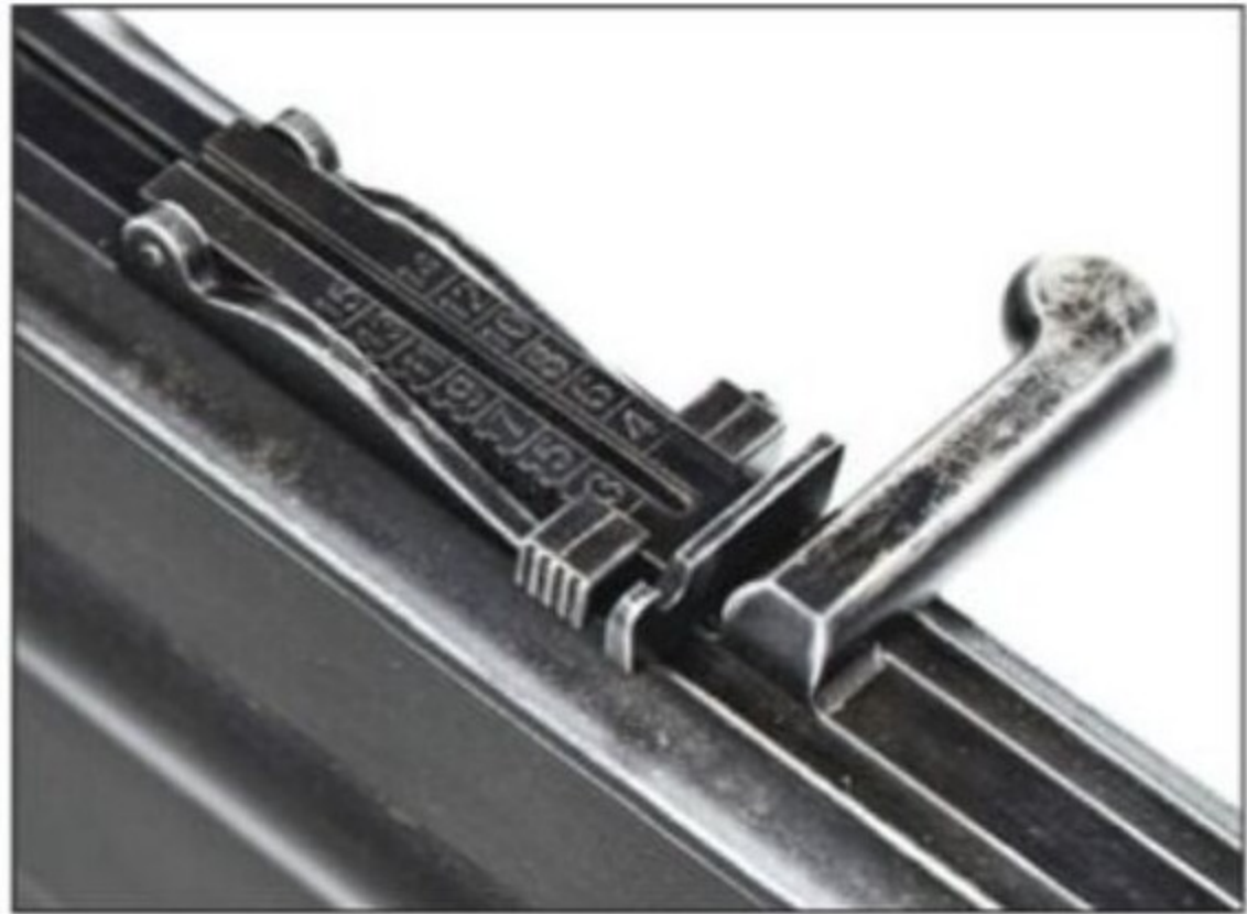
The rear sight was adjustable from 200 to 1,500 meters. Note the extended cocking handle, ejection port and takedown lever. (Courtesy of Mattias Holsti)
