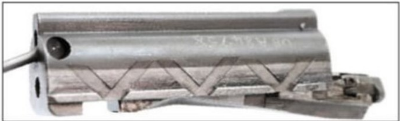
The sand cuts on the bolt carrier, to scrub gunk and crud out of the action rails. (Patrick Sweeney)
