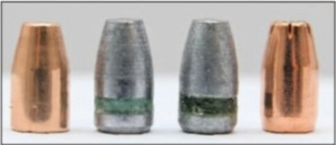
The bullets before loading, left to right: RMR, Oregon Trails, Northeast, Hornady. Notice that the RMR is shorter due to being a flat-base, not a boat-tail. This matters a lot in the 9mm. (Patrick Sweeney)
