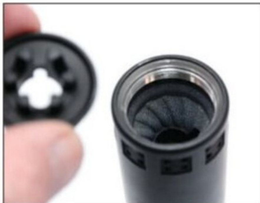
With the front cap off you can see the front end of the Triskelion baffle construct. (Patrick Sweeney)
