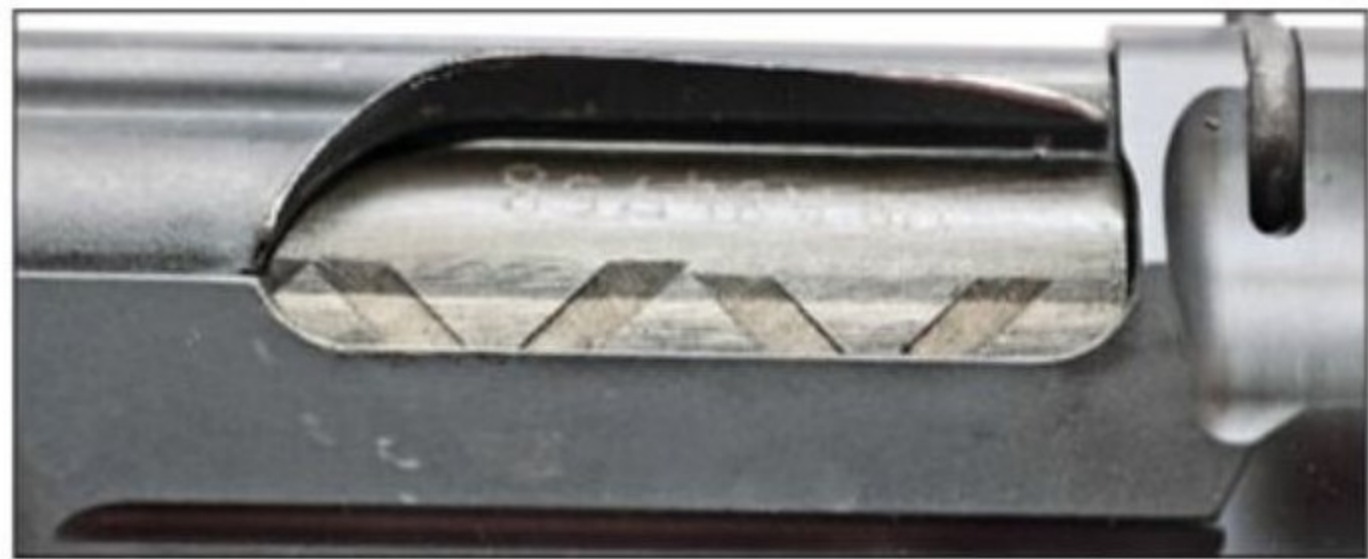
The carrier has “sand cuts” the angled grooves you see. They are there to scrape crud out when the L1A1 cycles. (Patrick Sweeney)
