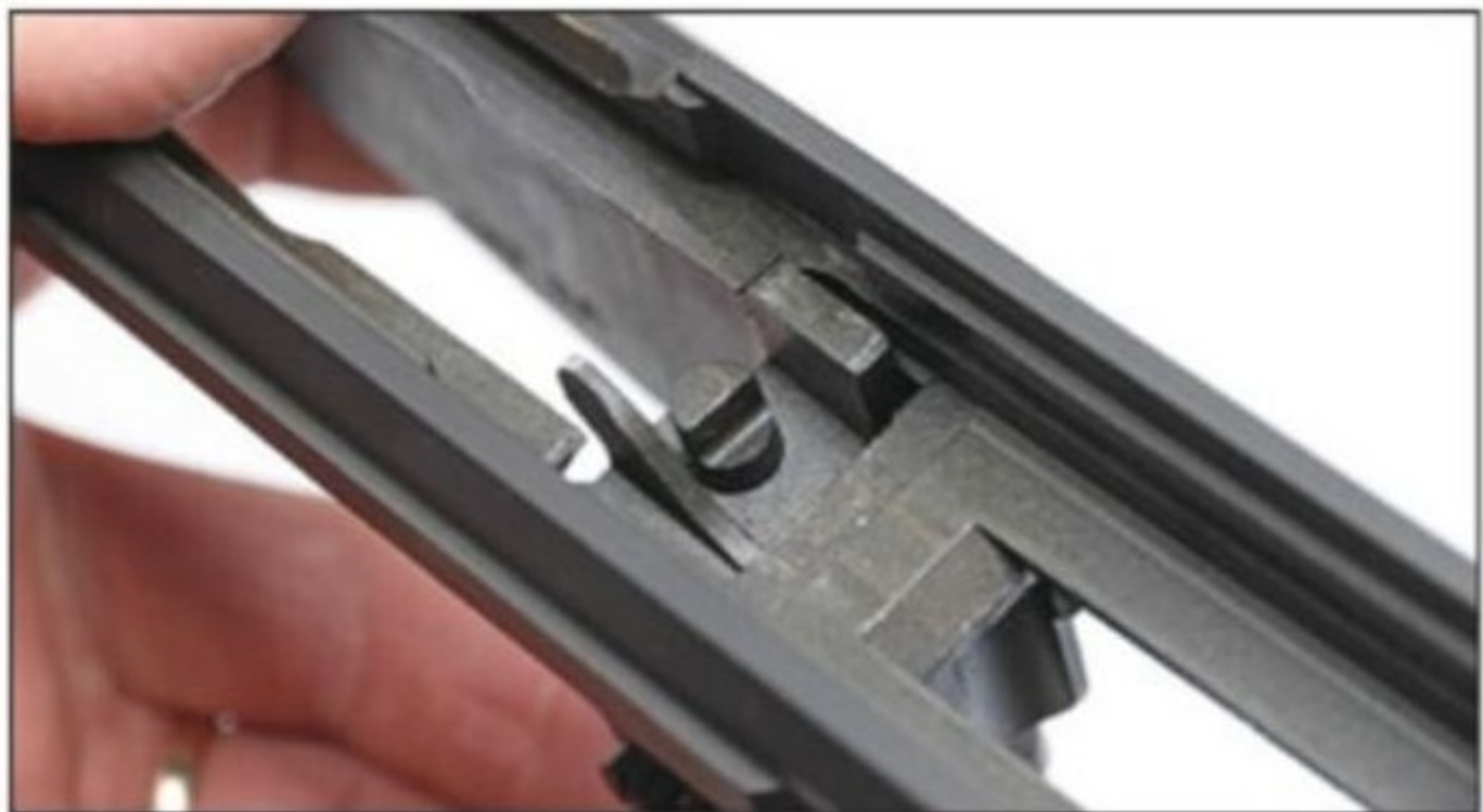
The bolt hold-open is in there, but the magazine won’t work it. You have to do it by hand. (Patrick Sweeney)
