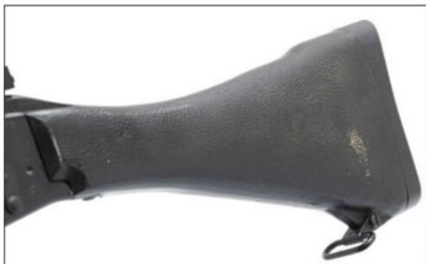
The stock also holds the recoil spring, in a long tube, and on the L1A1 made out of a tough plastic. (Patrick Sweeney)
