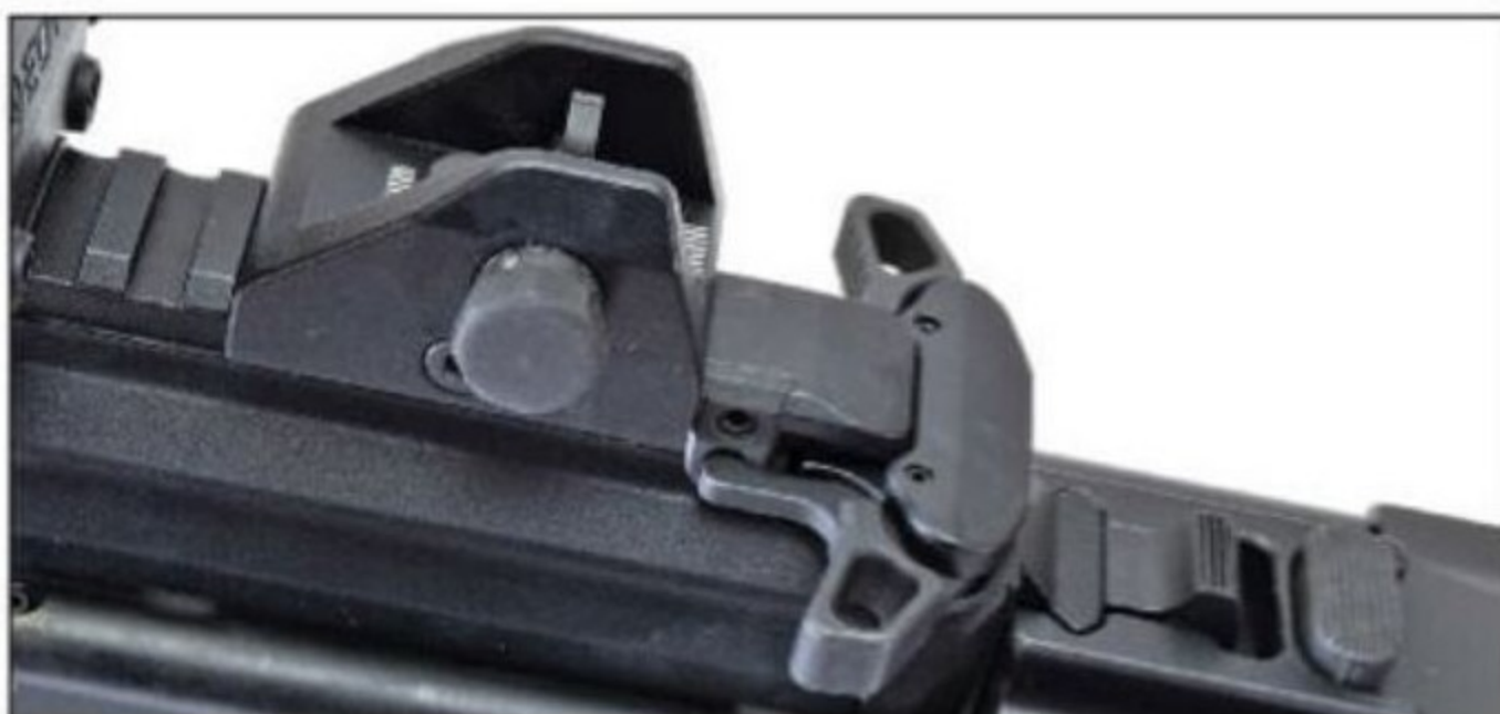
The AR-15-style charging handle has big wings. The latch hooks into a steel insert in the receiver at the back of the rail. The rear sight is click-adjustable for windage using that knob. (Photo by James Tarr)
