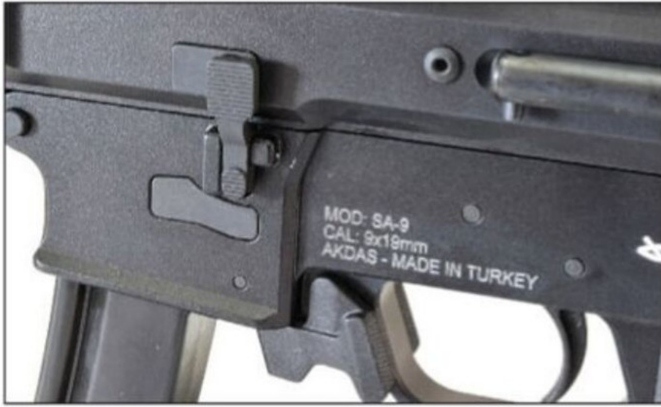
The MAC IX is a semi-auto pistol variant of the SA-9, a submachine gun made by Akdas in Turkey. You'll note many of the controls are similar to an AR-15's—that's on purpose. (Photo by James Tarr)
