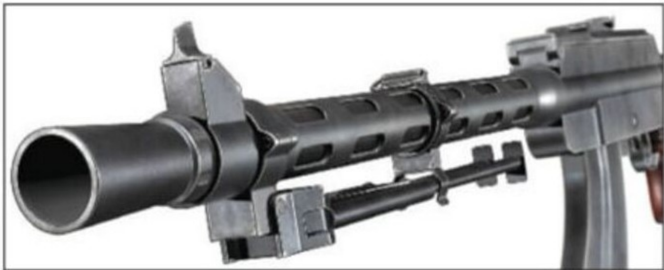
The rear sight was adjustable from 200 to 1,500 meters. Note the extended cocking handle, ejection port and takedown lever. (Courtesy of Mattias Holsti)
