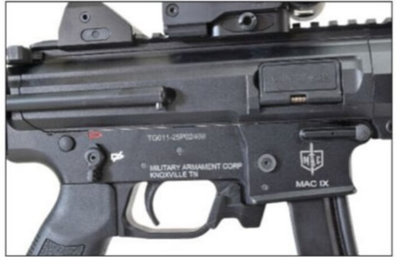
While the magazine release is different, the rest of the controls on the MAC IX are the same as on an AR-15. (Photo by James Tarr)
