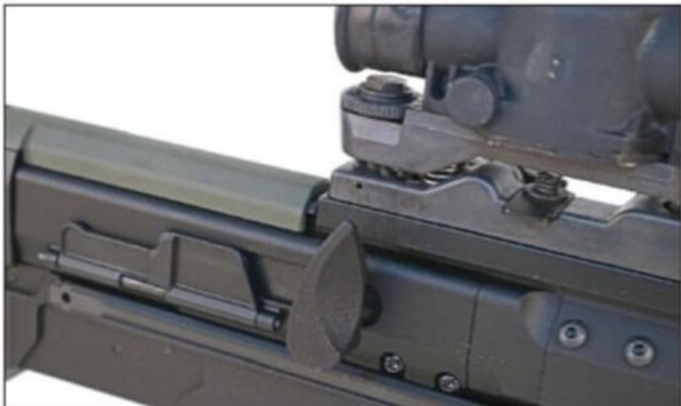
The charging handle from Aly & Kaufman mimics that of the GI SA80 and is a drop-in fit. (Will Dabbs)
