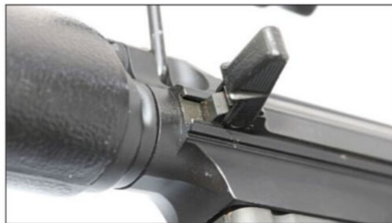
The L1A1 uses a folding charging handle, and so the end of the receiver slot has to be machined to accommodate that. (Patrick Sweeney)
