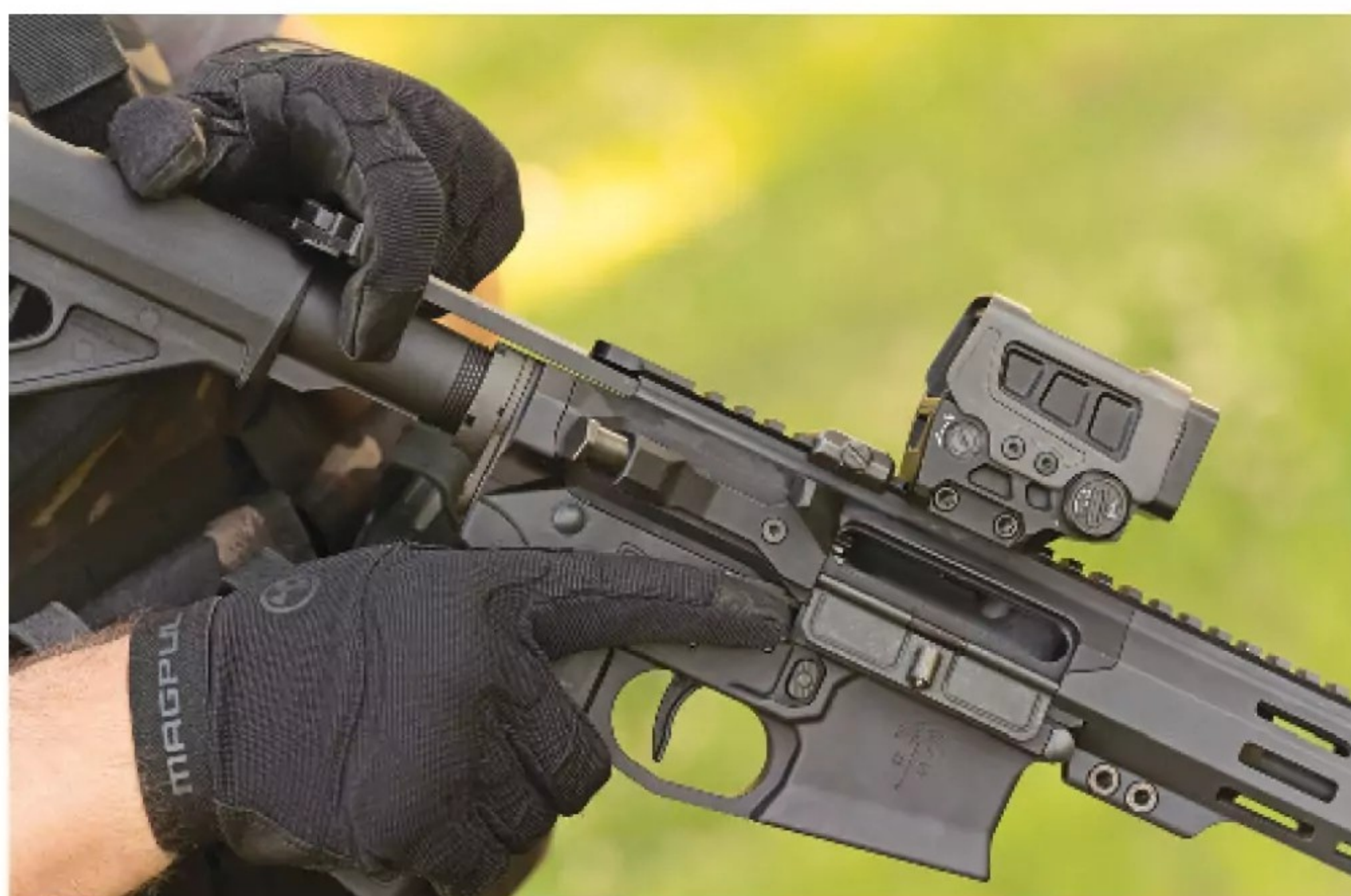
Right side bolt release lever is very helpful for locking the bolt back with the right hand staying on the pistol grip. (Oleg Volk)
