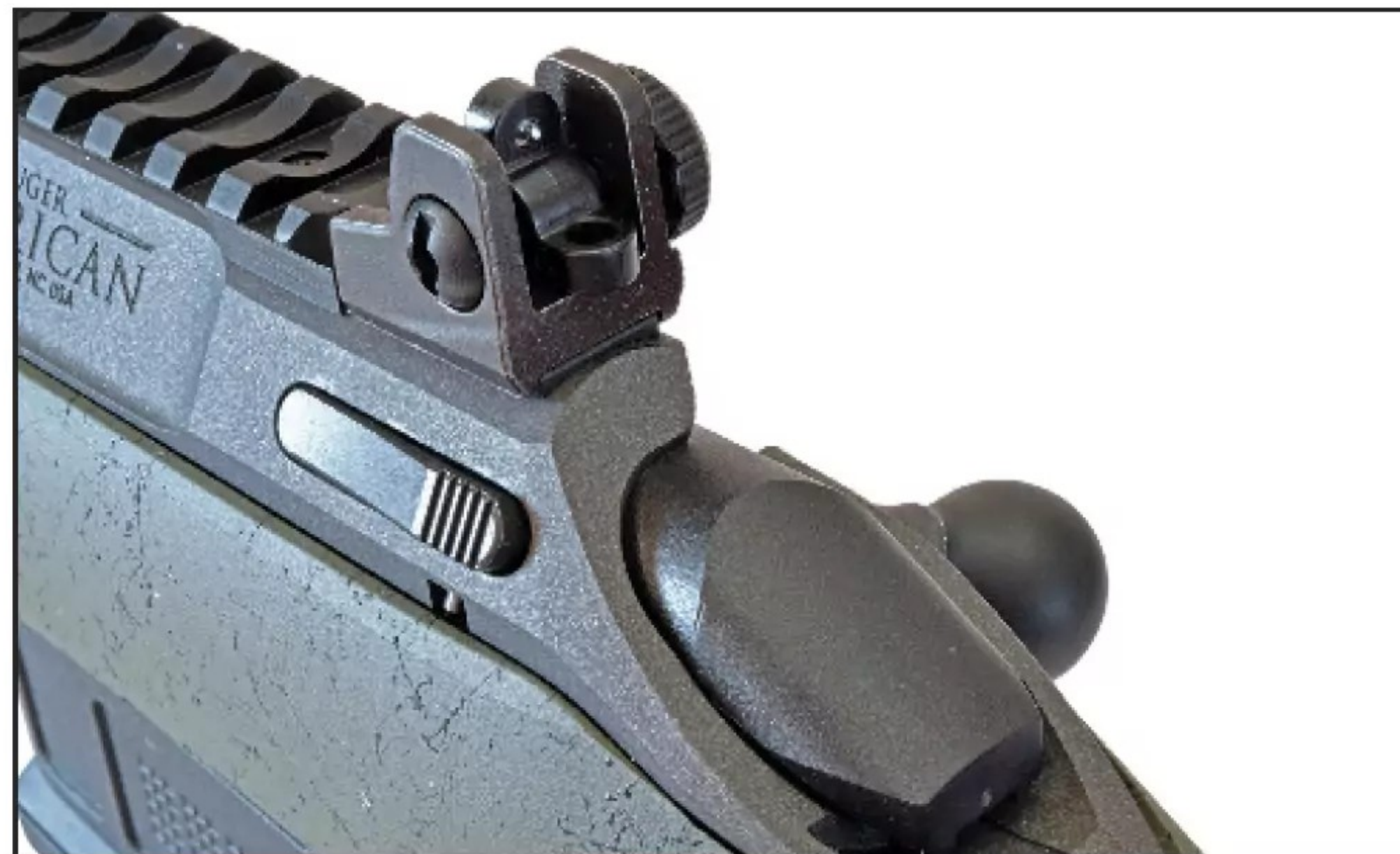
The rear sight has two protected apertures and is click adjustable for windage, at the rear of 11.25 inches of rail space. (Photo by James Tarr)
