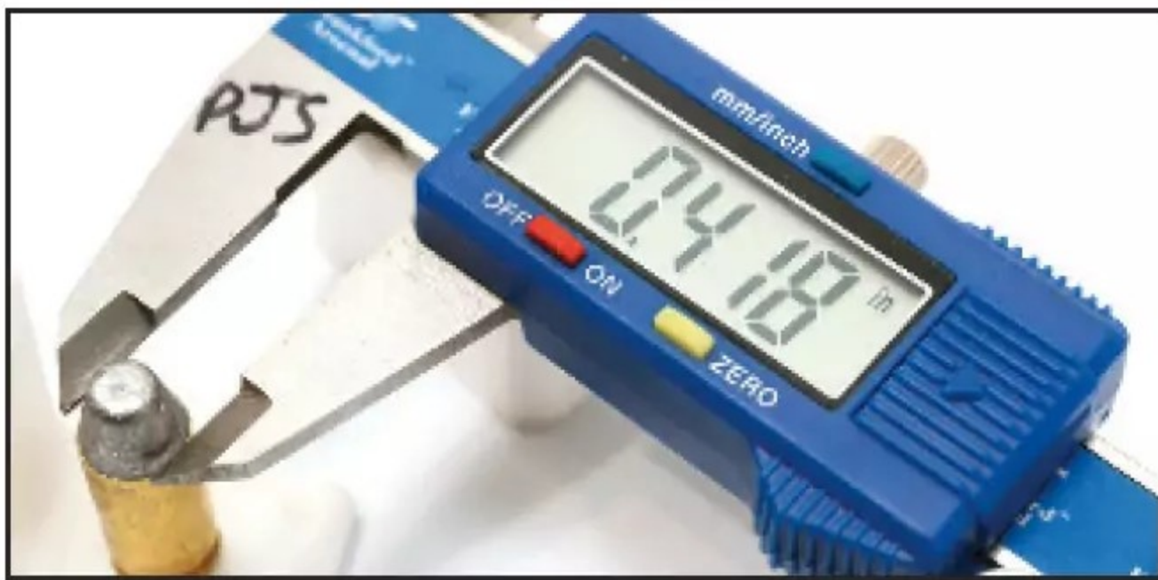
The taper crimp on the .40 is simple and not subject to much change. So, strive for .418" and you'll be in the ballpark. (Patrick Sweeney)
