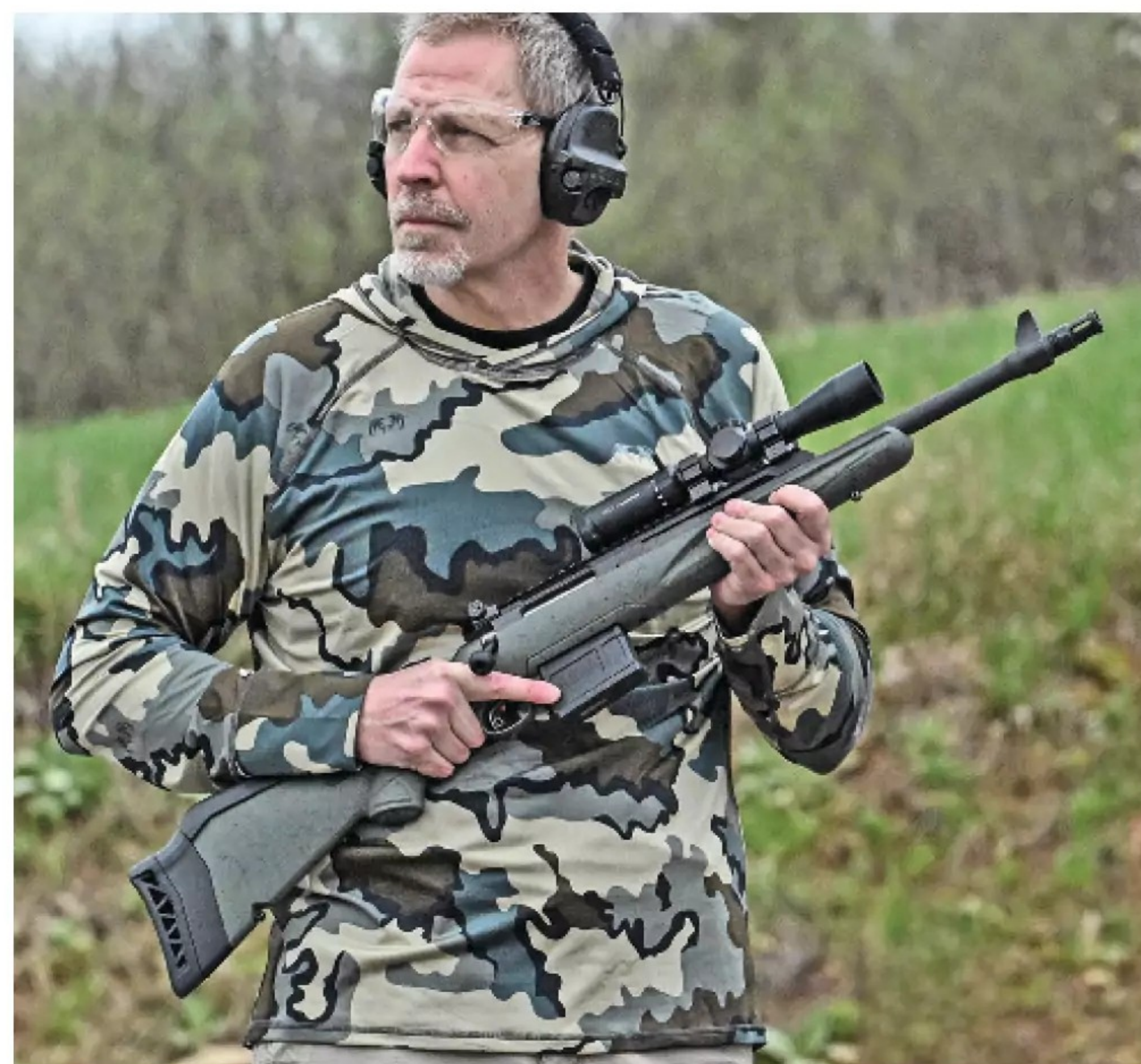
The Scout is a general-purpose rifle. Cooper’s original specs called for under a meter in length and 3 kilos in weight (including optic). The Ruger makes the length but doesn’t quite make the weight. (Photo by Andy Grossman)
