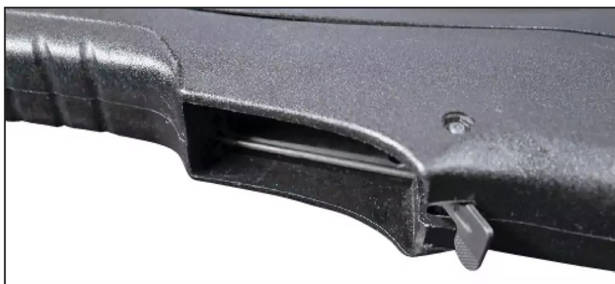
The magazine well of the Vektor CR-21 is located well behind the grip assembly; the magazine release is a standard Galil/Vektor R4-style paddle, extended to one side for easy reach. (Photo by Connor and Sarah Daine)
