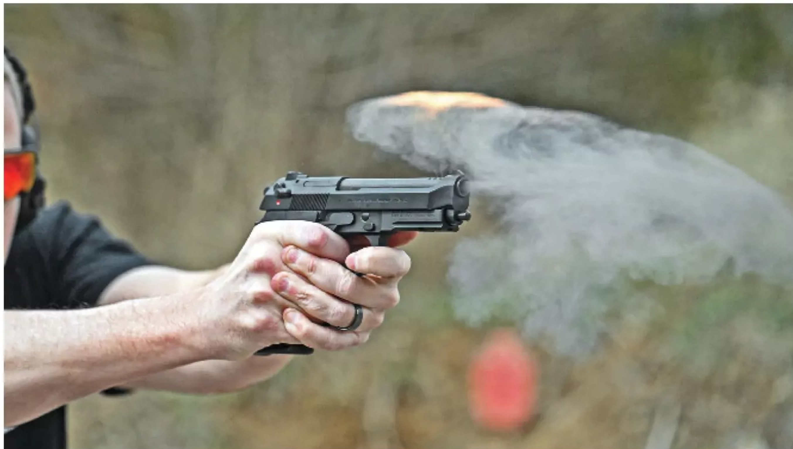
The ports in the Beretta's barrel can be seen here venting upward. They did reduce muzzle rise...but they also broasted the white dot on the front sight. (Photo by Andy Grossman)
