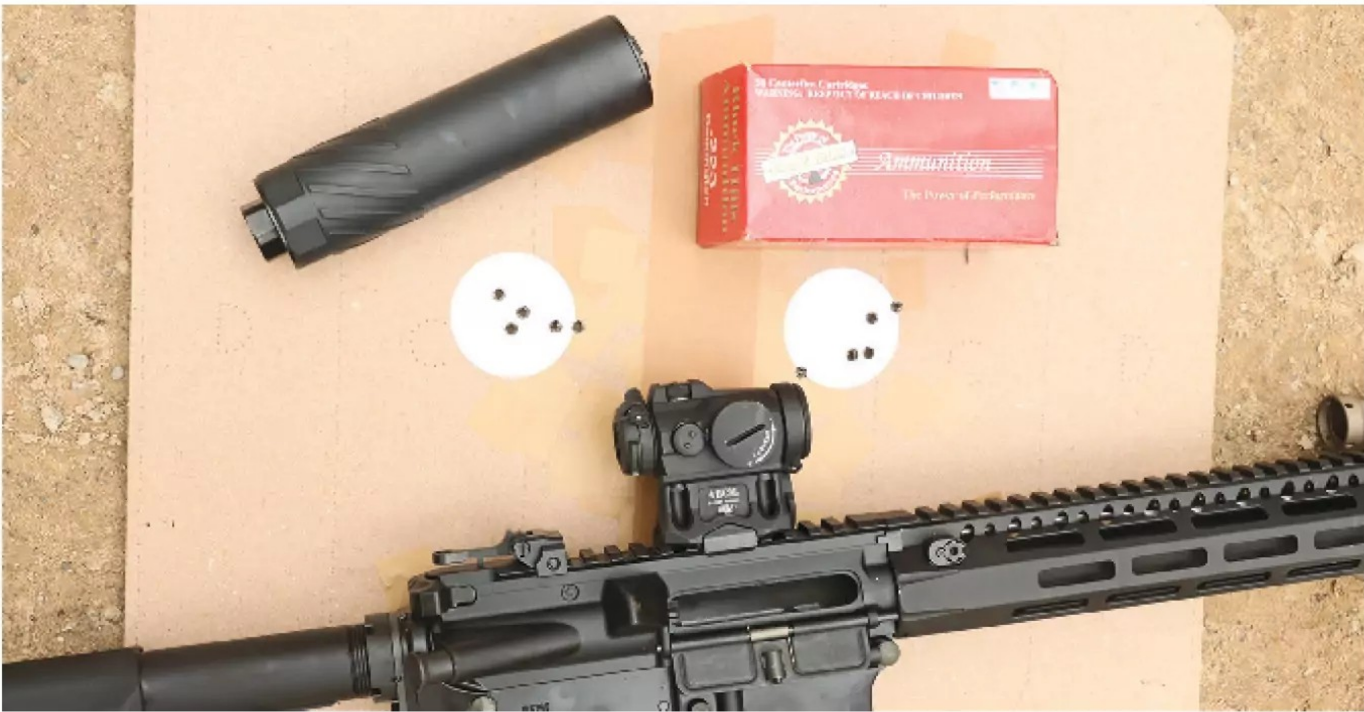
No shift in point of impact between suppressed and un-suppressed, always a good sign. (Patrick Sweeney)
