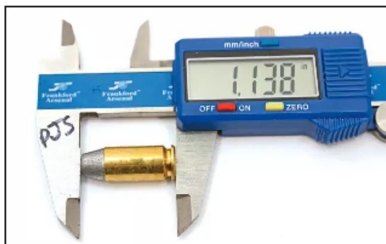
The OAL of the .40 is severely limited, with this one right in the limited range. (Patrick Sweeney)
