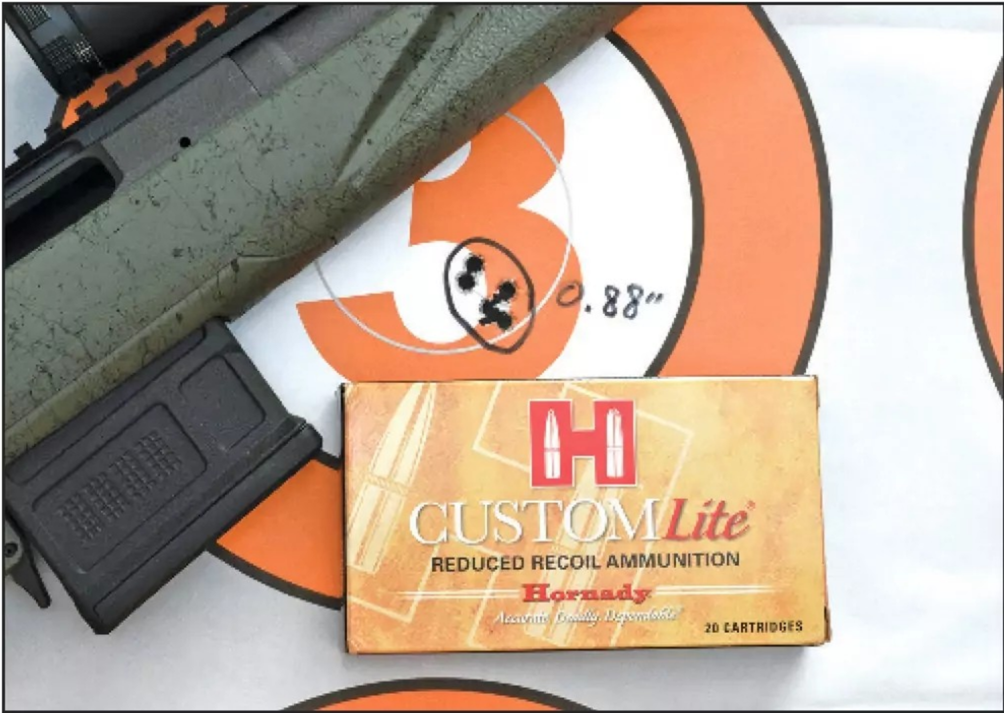
The best group from the scout was this .88 of an inch group fired with Hornady’s reduced recoil load. The rifle averaged 1 to 2 MOA, which is solid performance. (Photo by James Tarr)
