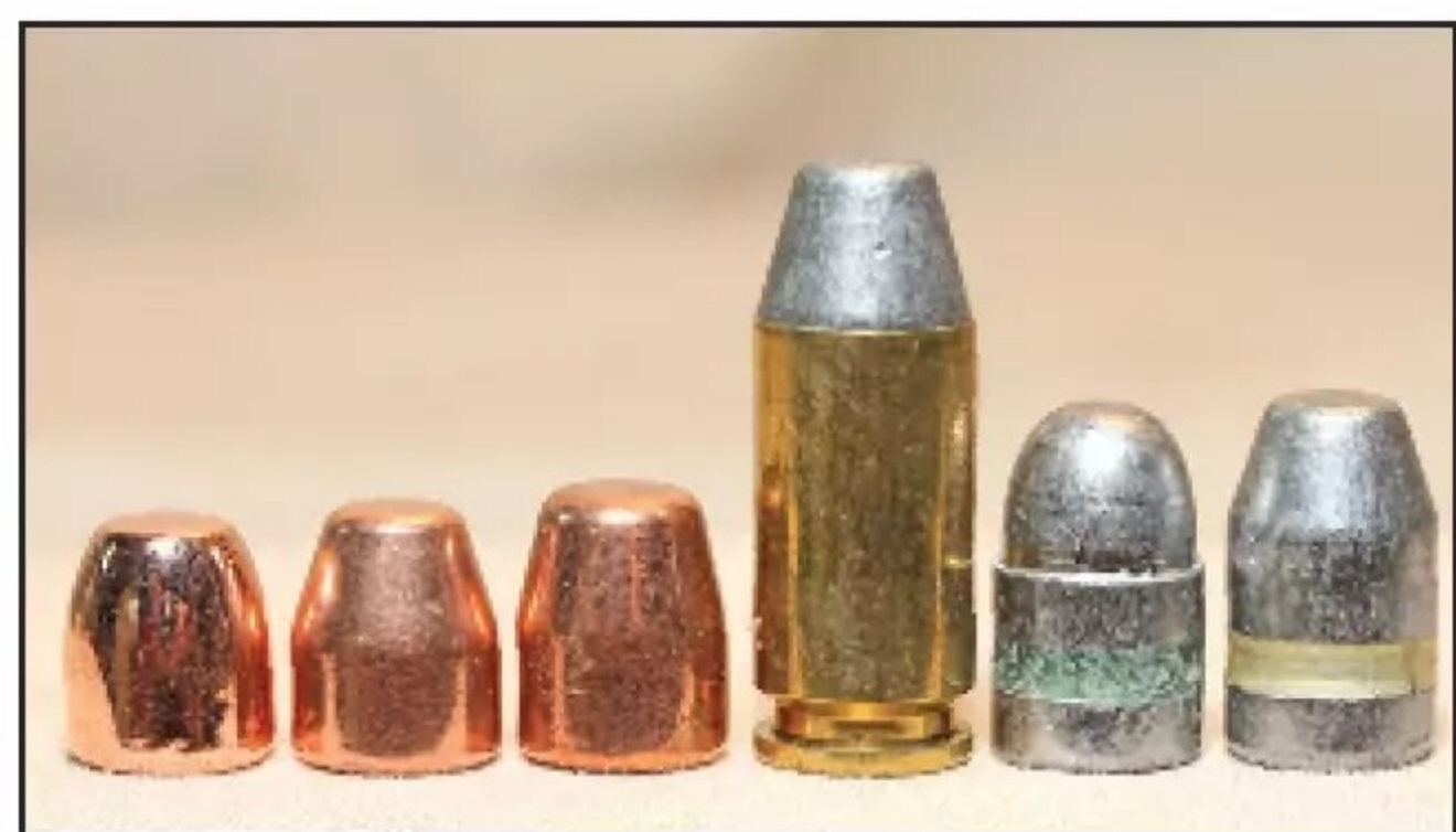
The weight range for the .40 is from 135- to 180-grain projectiles. Lead, plated, coated, they all work. (Patrick Sweeney)
