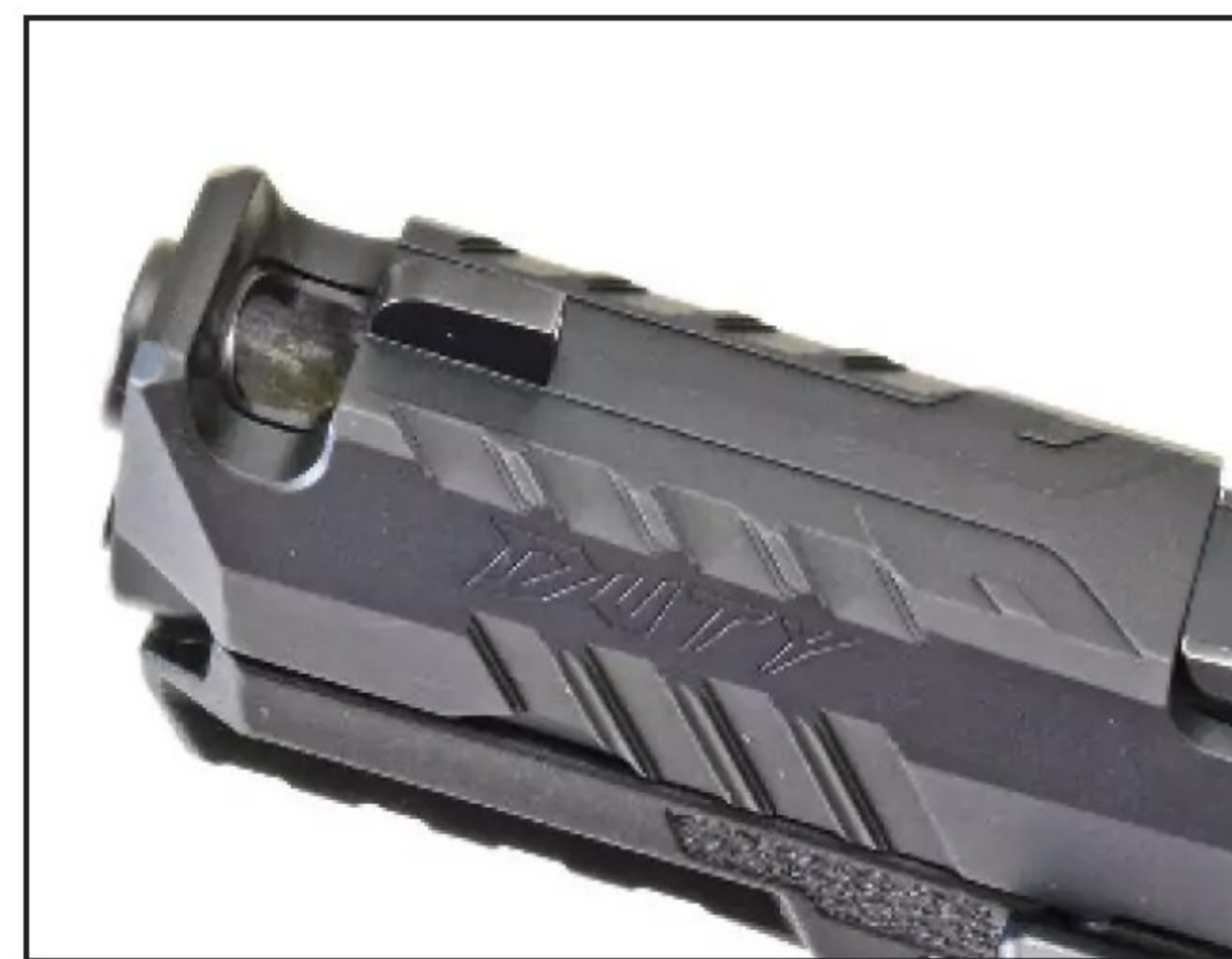
Some ports, like what's seen here on the TISAS PX-9 Duty, can also work as a compensator. The front of the cut in the slide works as a baffle, helping to redirect gases. (Photo by James Tarr)
