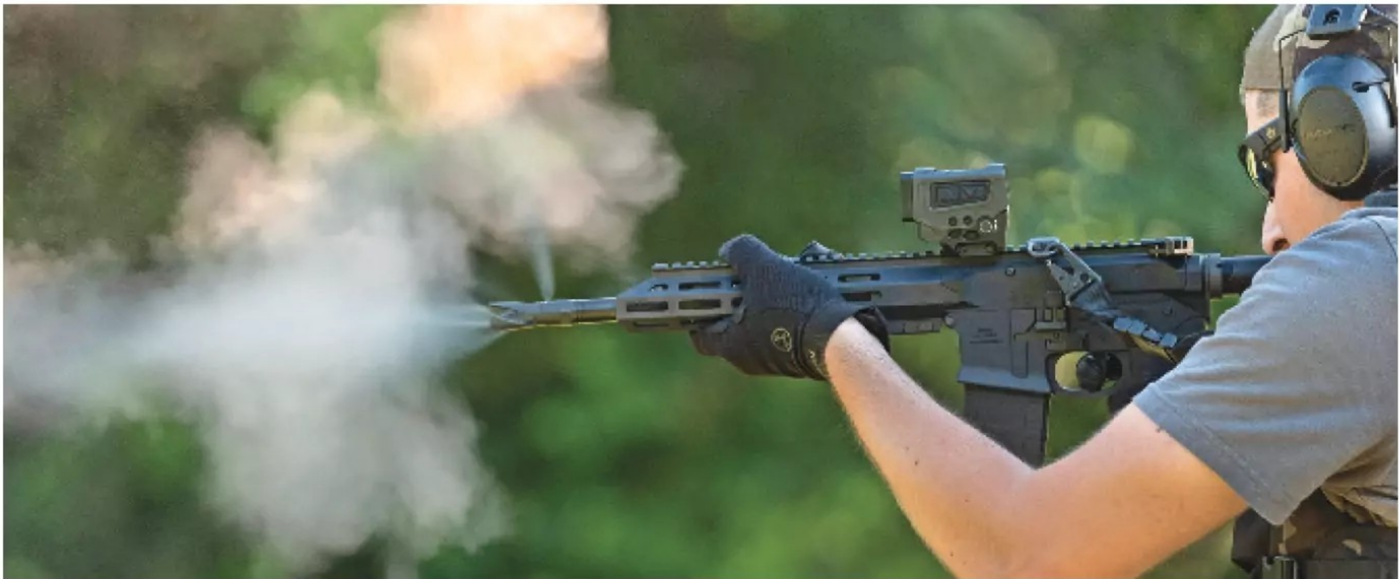
Well-defined jet streams dissipate flash while stopping muzzle climb. (Oleg Volk)
