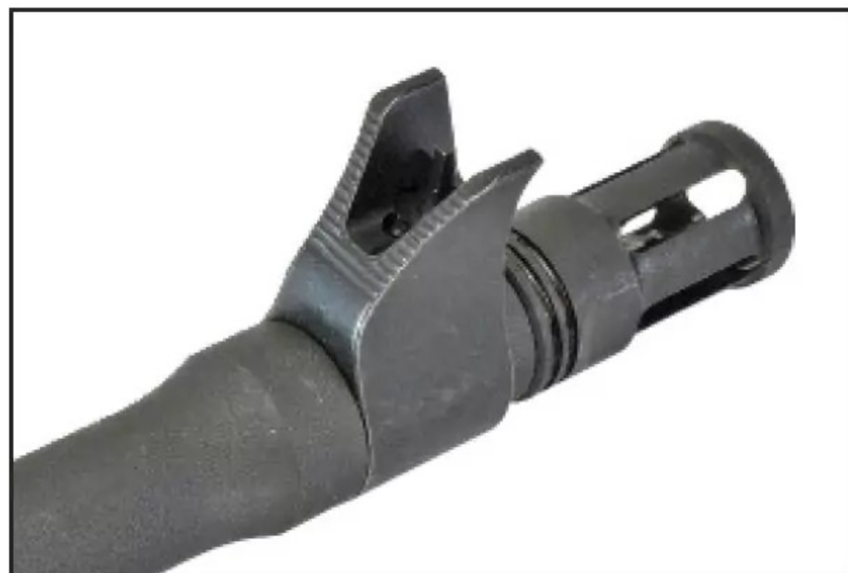
◀ The AR-style post front sight (adjustable for elevation) is protected by beefy steel wings, serrated to reduce glare. (Photo by James Tarr)
