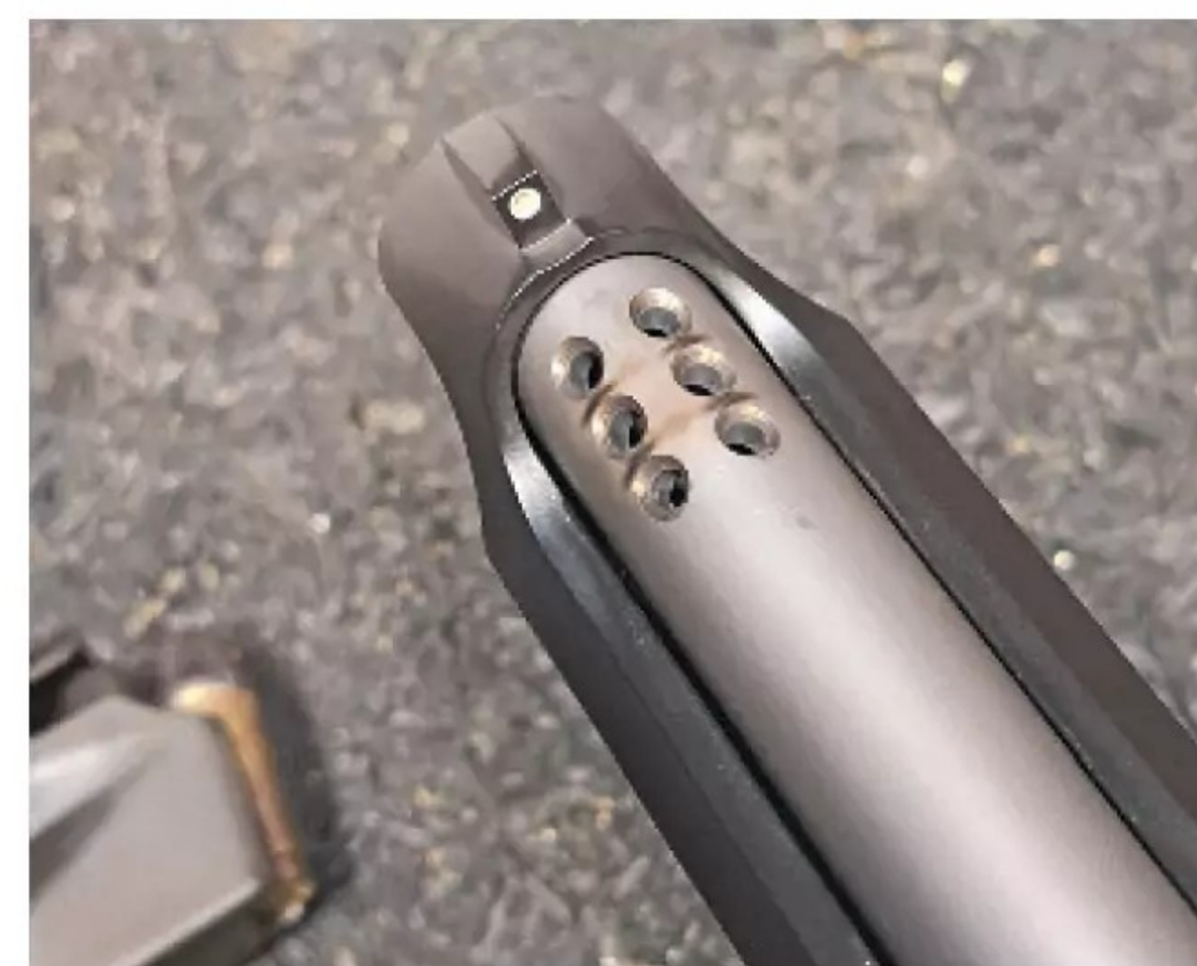
Ports, like those seen here in a Beretta 92, are simply holes put into the top of a barrel to vent some of the gases upward. (Photo by James Tarr)
