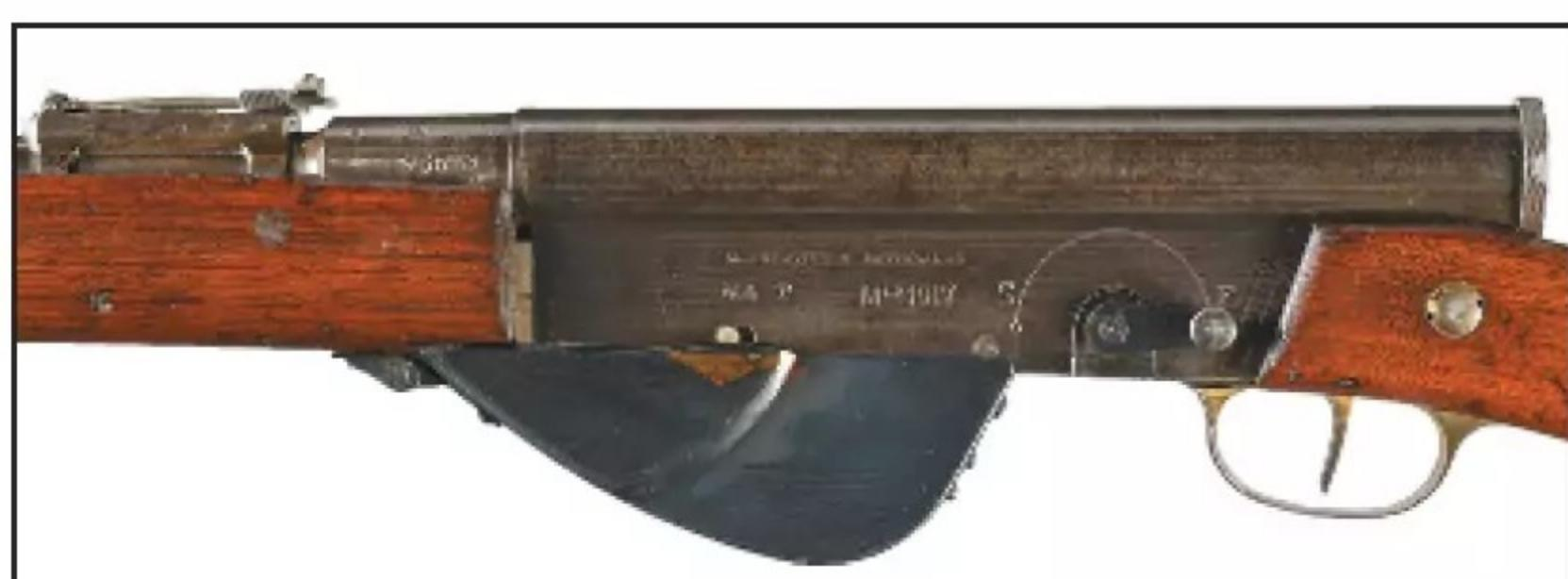
**A rotating safety catch was located on the left side of the receiver. (Courtesy of Rock Island Auction Co.)**
