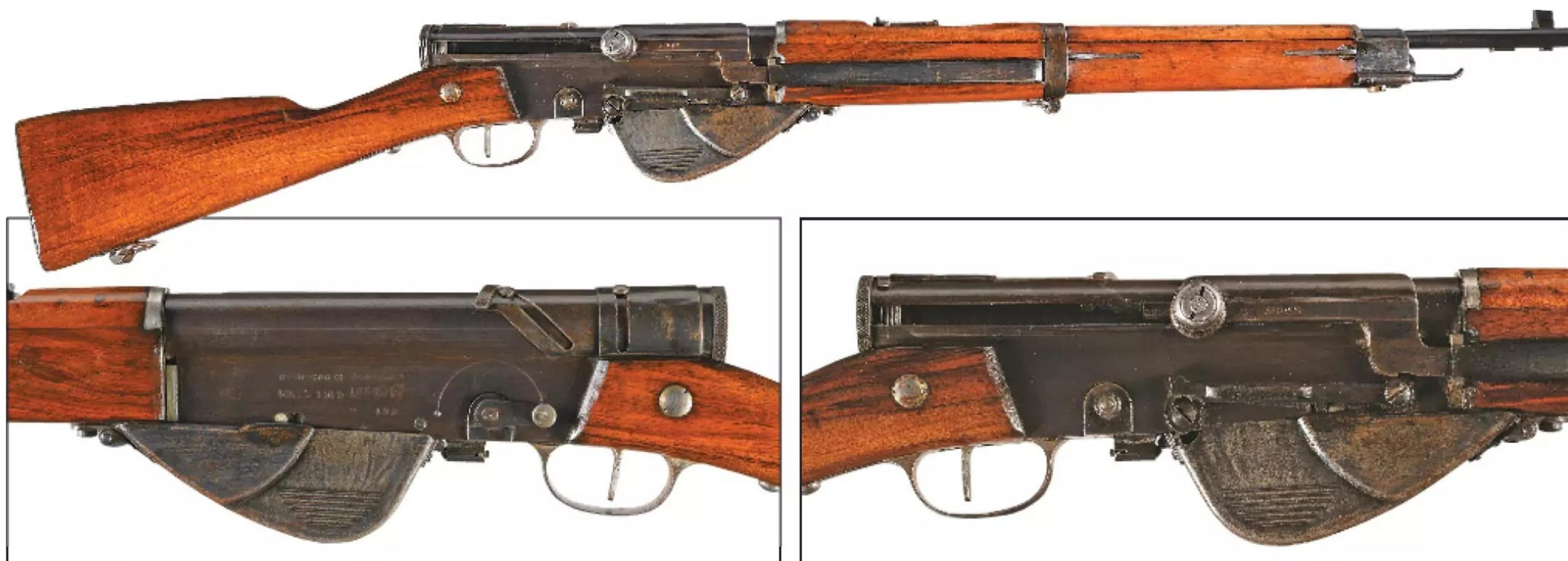
**The Mousqueton automatique Modèle 1918 was shorter than the Modèle 1917, it featured a sheet metal dust cover that could be rotated over the bolt slot, plunger type magazine catch and used the widely available Modèle 1916 Berthier clip. (Courtesy Rock Island Auction Co.)**
