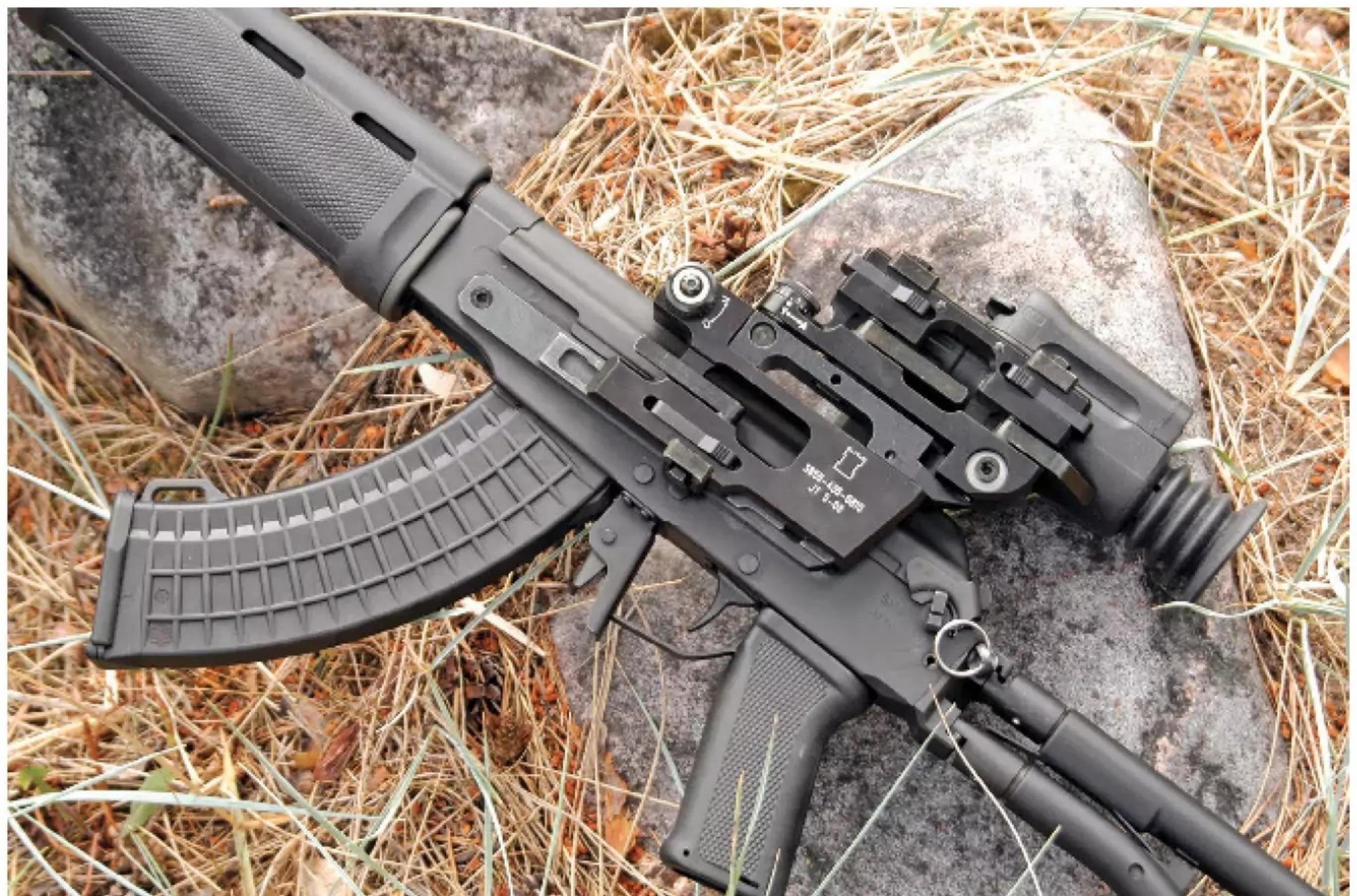
**A rail allows day/night optics to be easily mounted. Also note the top cover retainer. (David M. Fortier)**
