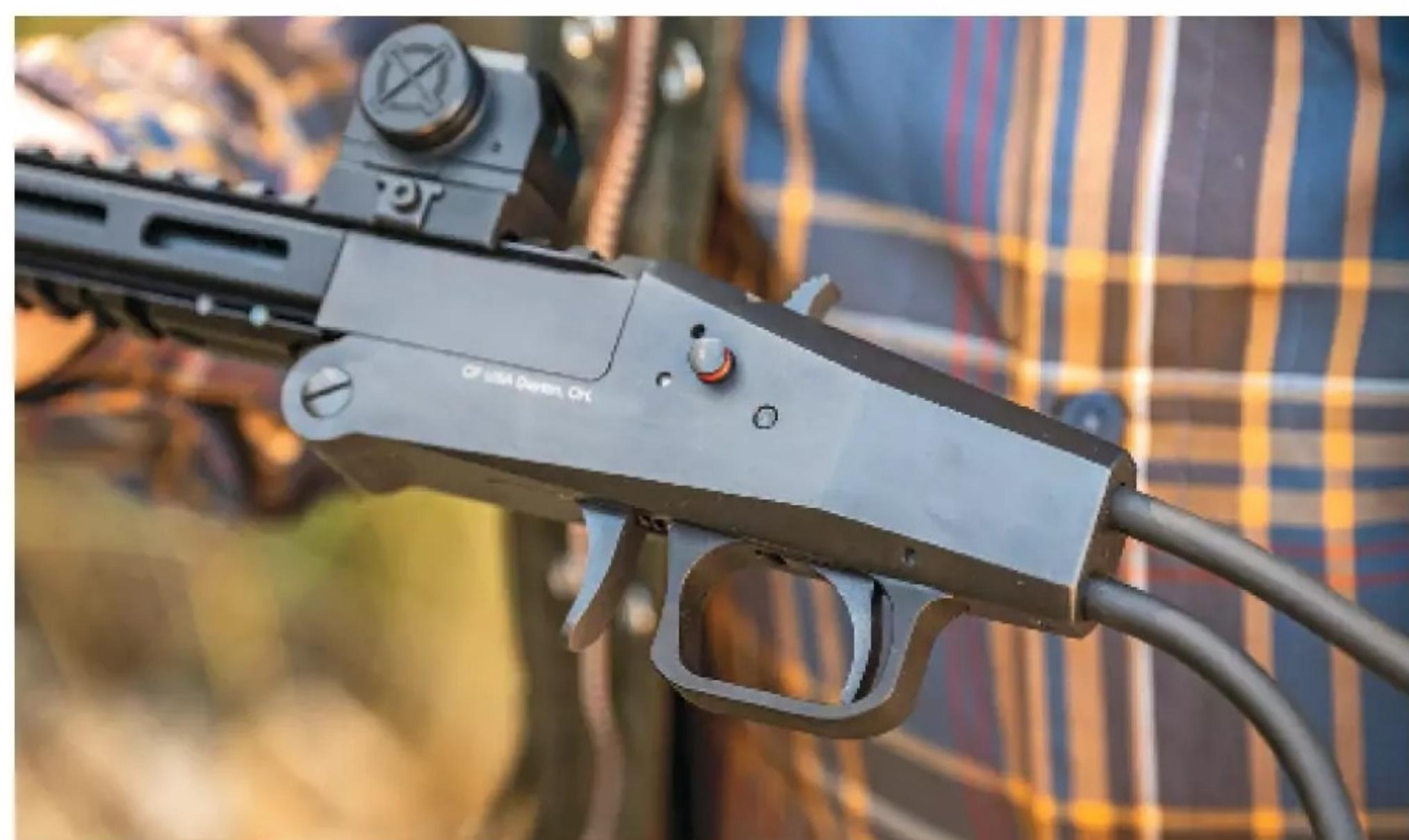
**The Chiappa Firearms Big Badger, in all its variants, features an external hammer that must be manually cocked before firing; the hammer can also be manually set to a half-cock position to dub as a safety, but all versions also come with a crossbolt manual safety for good measure. (Pierangelo Tendas)**
