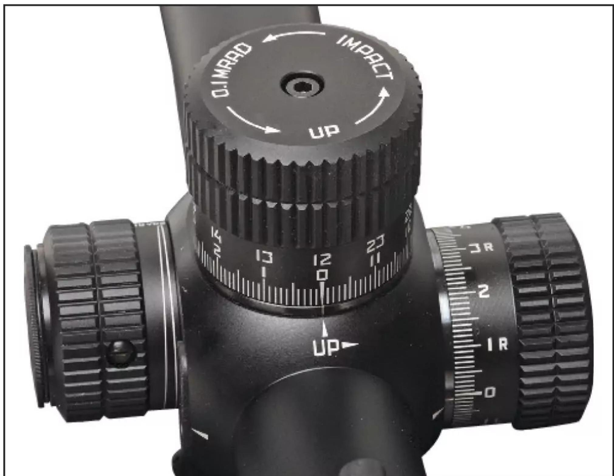
**The adjustment turrets are very large, feature a zero stop, and positive audible and tactile 0.1 MRAD adjustment clicks. Internal elevation adjustment range is 32 mils. (David Fortier)**
