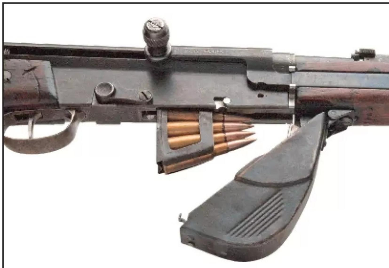
**The Modèle 1917's magazine housing was opened, a five-round clip inserted into the bottom of the receiver and the housing closed. (Nathan Reynolds photo)**
