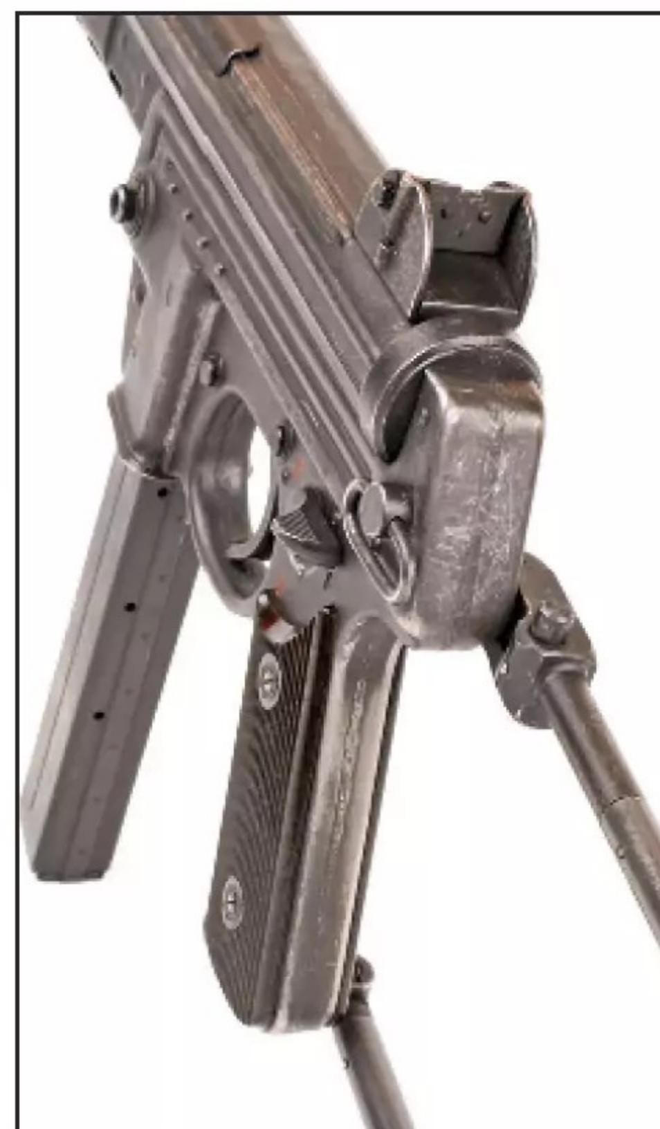
**The heavy wire stock folds to the right when not in use. Strangely, the stock strut runs across the bottom portion of the ejection port and can adversely affect reliability. (Will Dabbs)**
