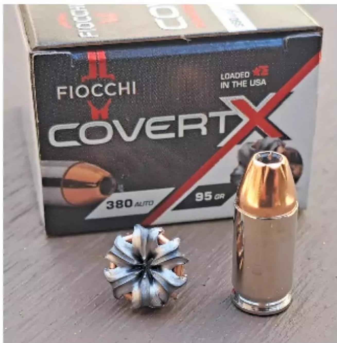
**Fiocchi's new CovertX line features a .380 load that performs even out of short barrels. Tarr fired this bullet out of the 2.75-inch barrel of the S&W Bodyguard 2.0 and it penetrated the gel block 11.5 inches and showed this perfect expansion. (James Tarr)**
