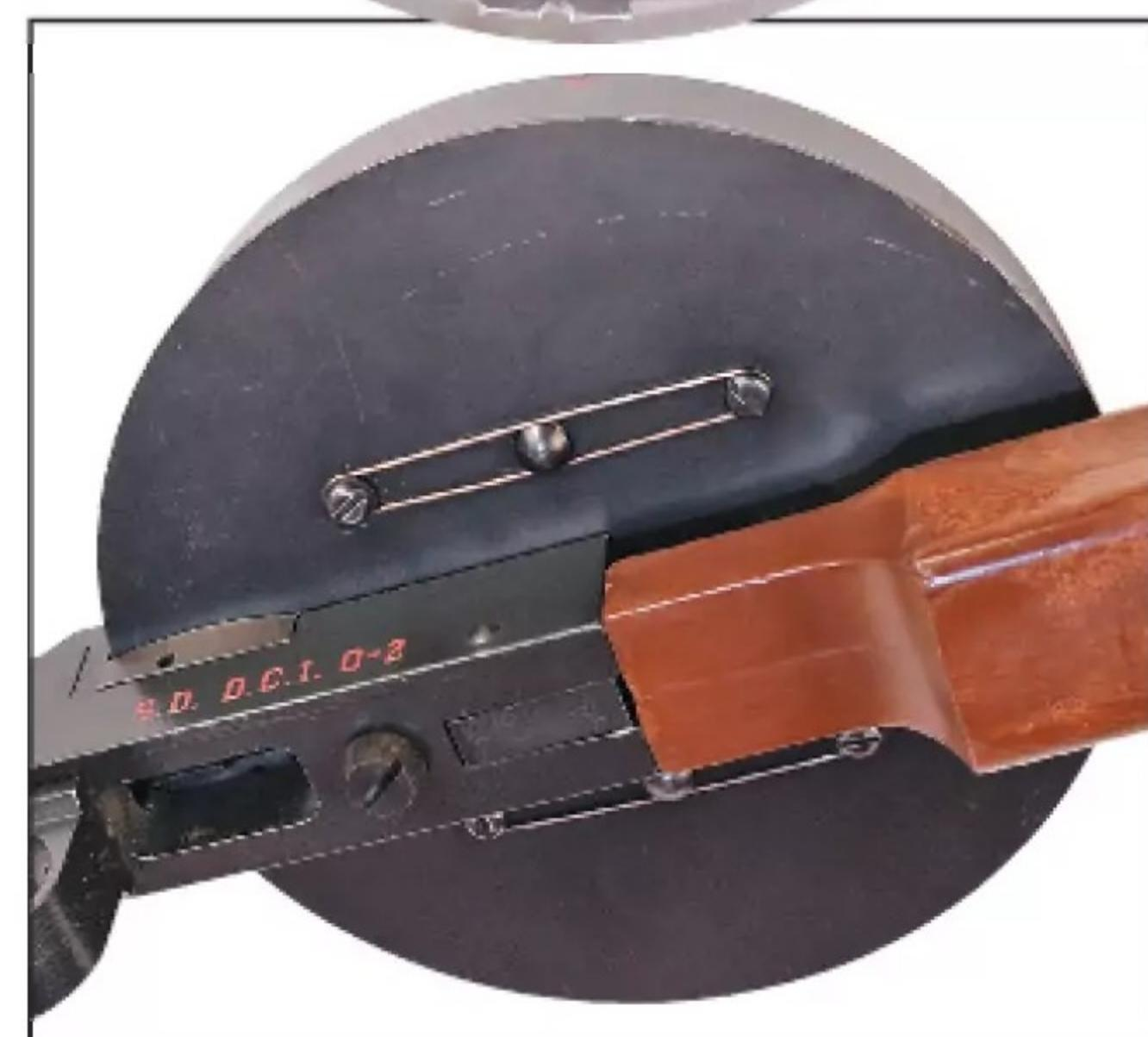
**The top-mounted drum magazine is the American 180's most distinctive feature. This original steel version packs 177 rounds of .22LR onboard. (Will Dabbs)**
