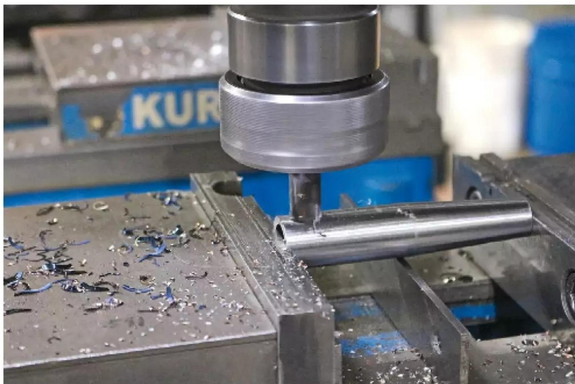
**We used an end mill to cut the slot to accommodate the existing front sight. (Will Dabbs)**
