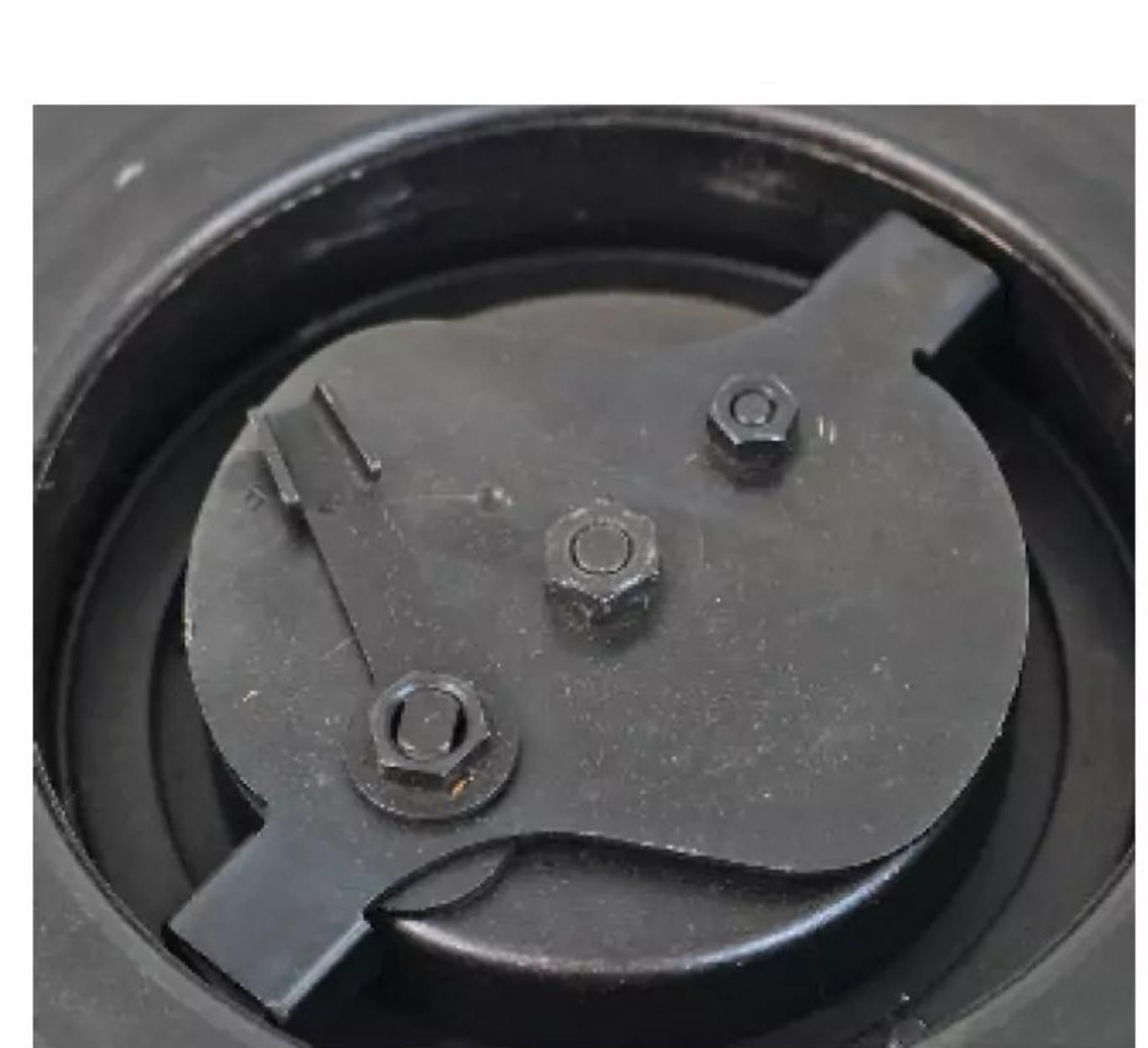
**That lever on the winder motor controls a clutch that keeps things locked in place until you are ready to shoot. (Will Dabbs)**
