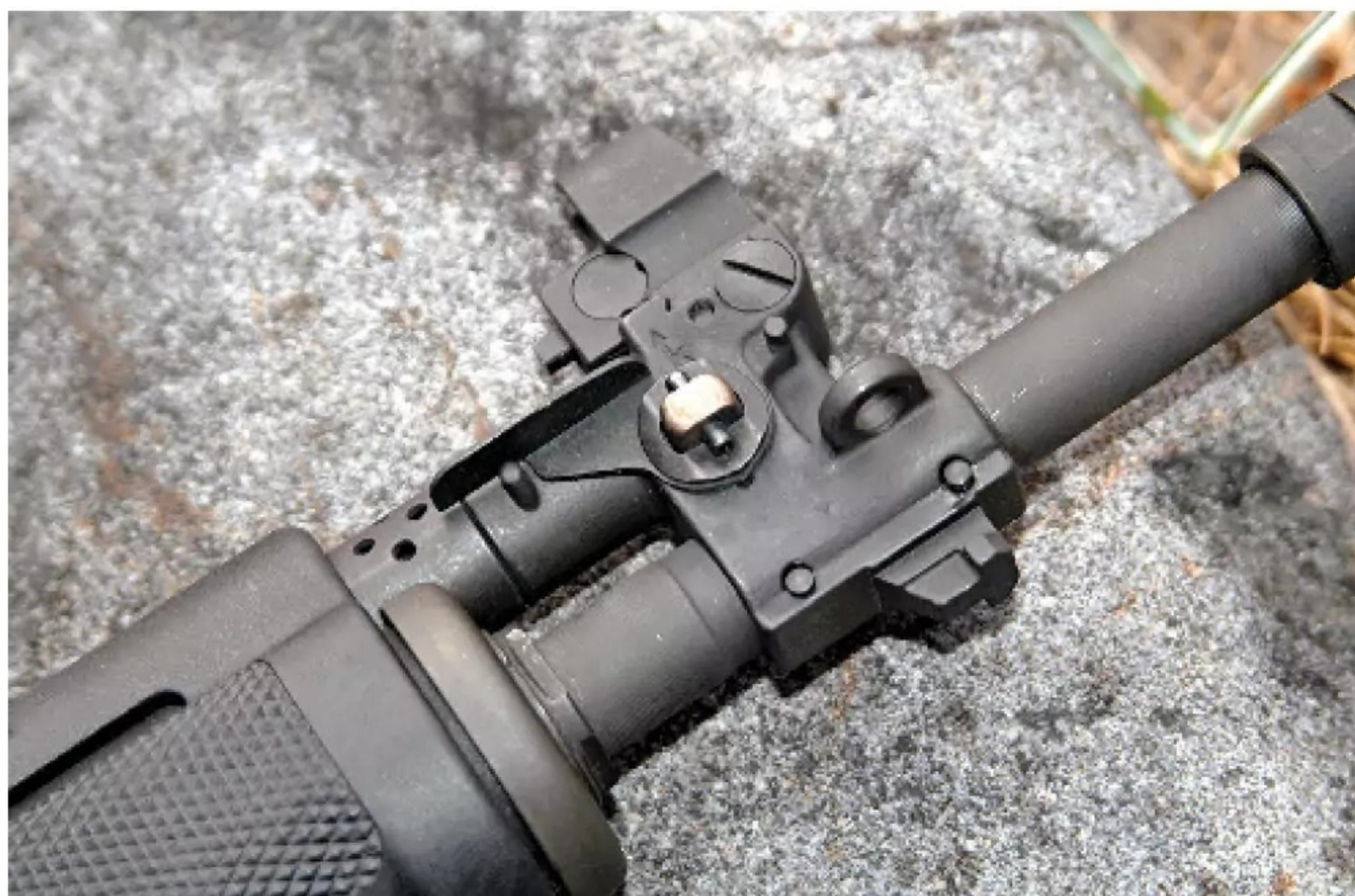
**The RK 95 TP's gas block features a two-position valve allowing the gas flow to be shut off. (David M. Fortier)**
