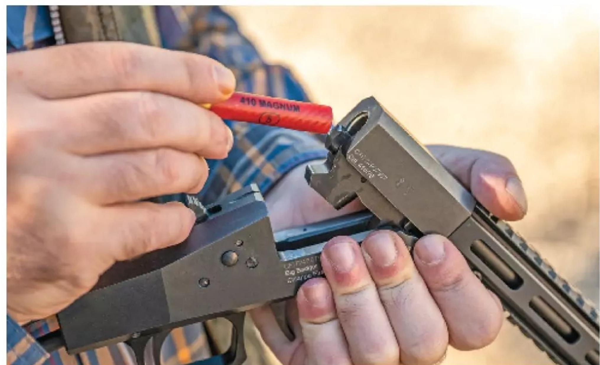
**A large extractor extends automatically when the barrel breaks open, speeding up the process of manually removing spent cases for reloading. (Pierangelo Tendas)**
