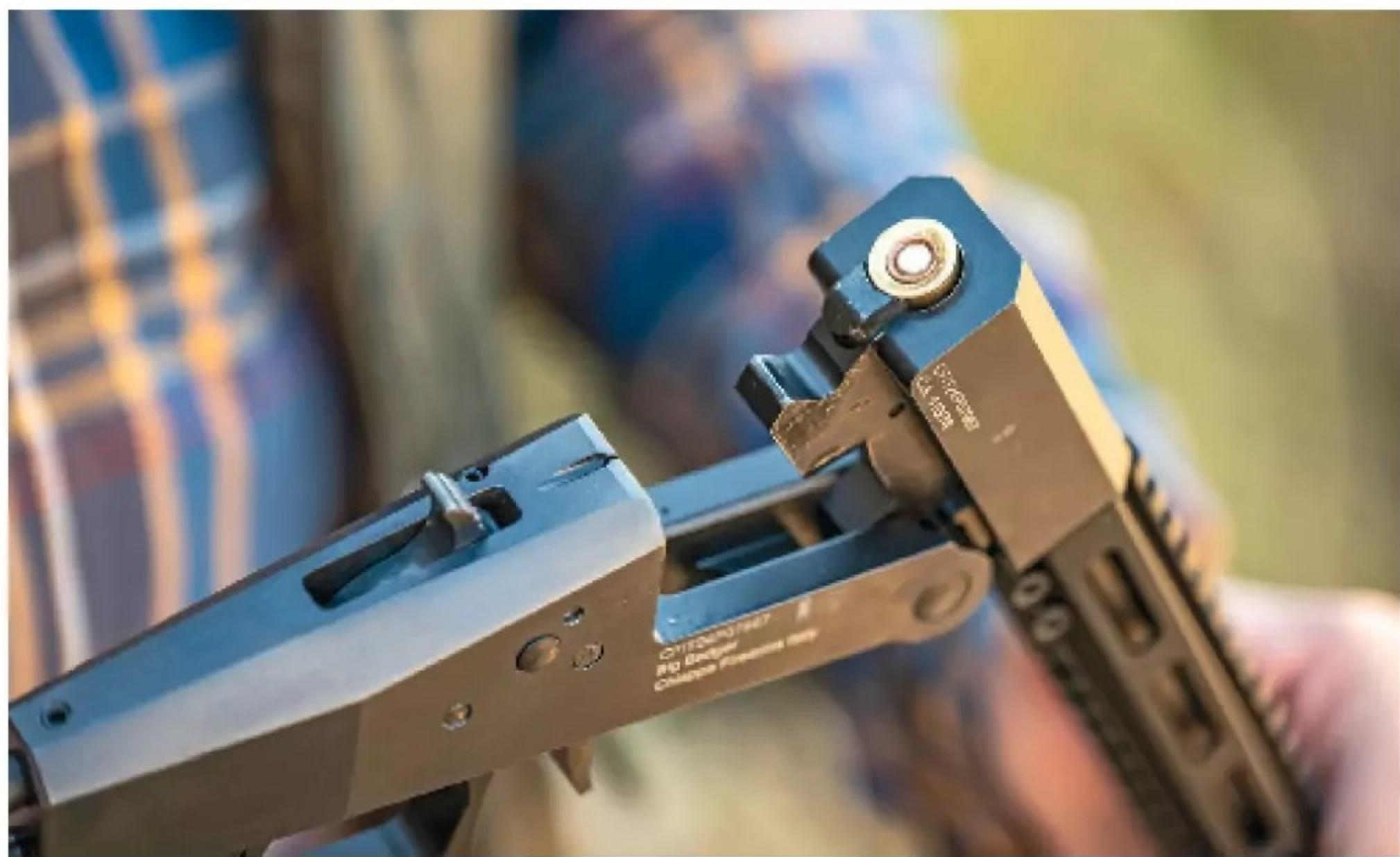
**On the 350 Legend and .30-30 Winchester versions of the Chiappa Firearms Big Badger, the rear portion of the top Picatinny rail extends all the way back to the top of the chamber to accommodate any sort of optical sights. The same can't be said for the .410 variant, so that the rear portion of the handguard does not get in the way of the rear sighting notch cut on top of the receiver and the red fiber optic front sight. (Pierangelo Tendas)**
