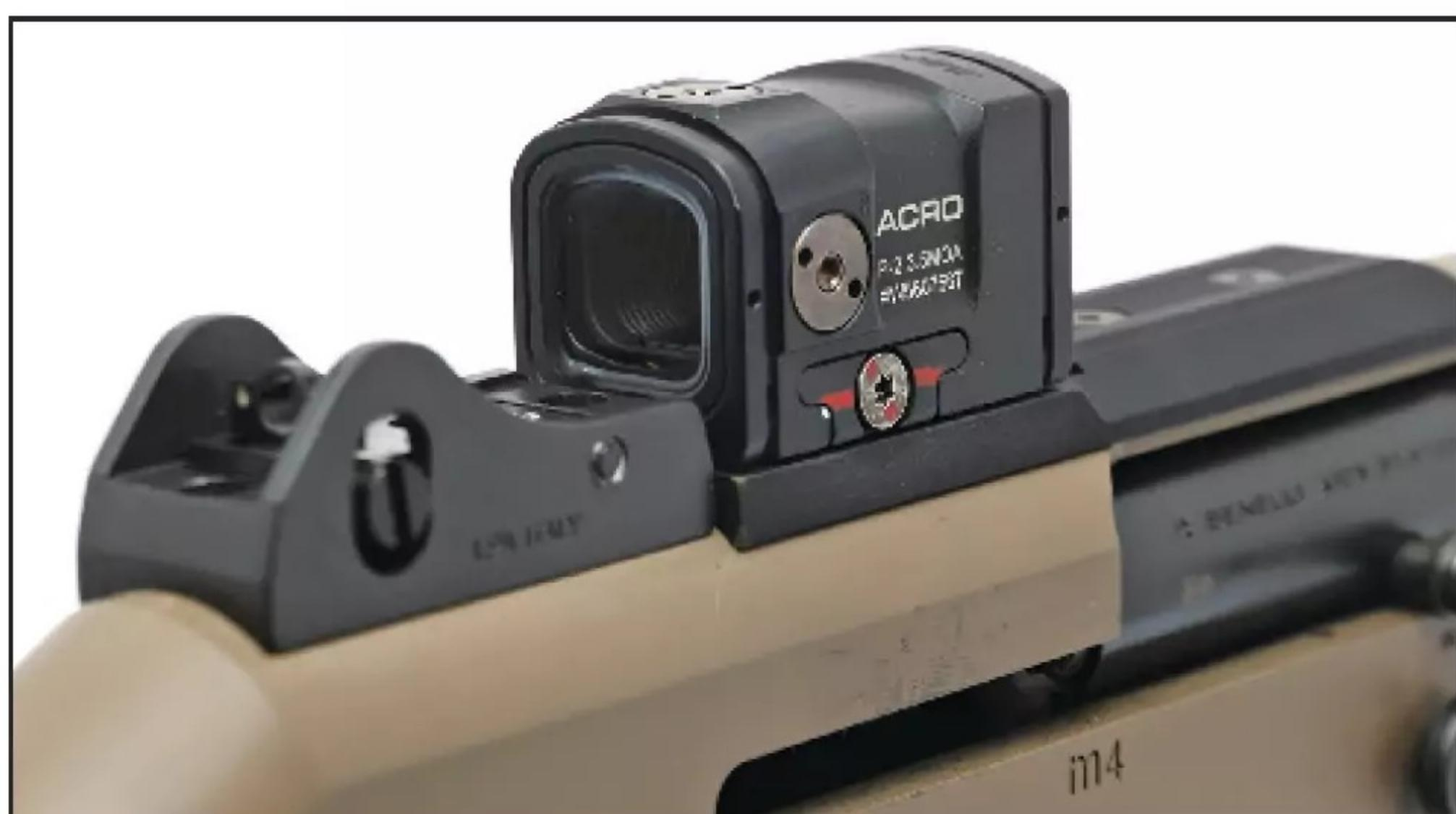
◀ The drilled and tapped receiver means you can install a mounting plate like this one, and then a red dot optic. Mesa Tactical and Aimpoint for the win. (Patrick Sweeney)
