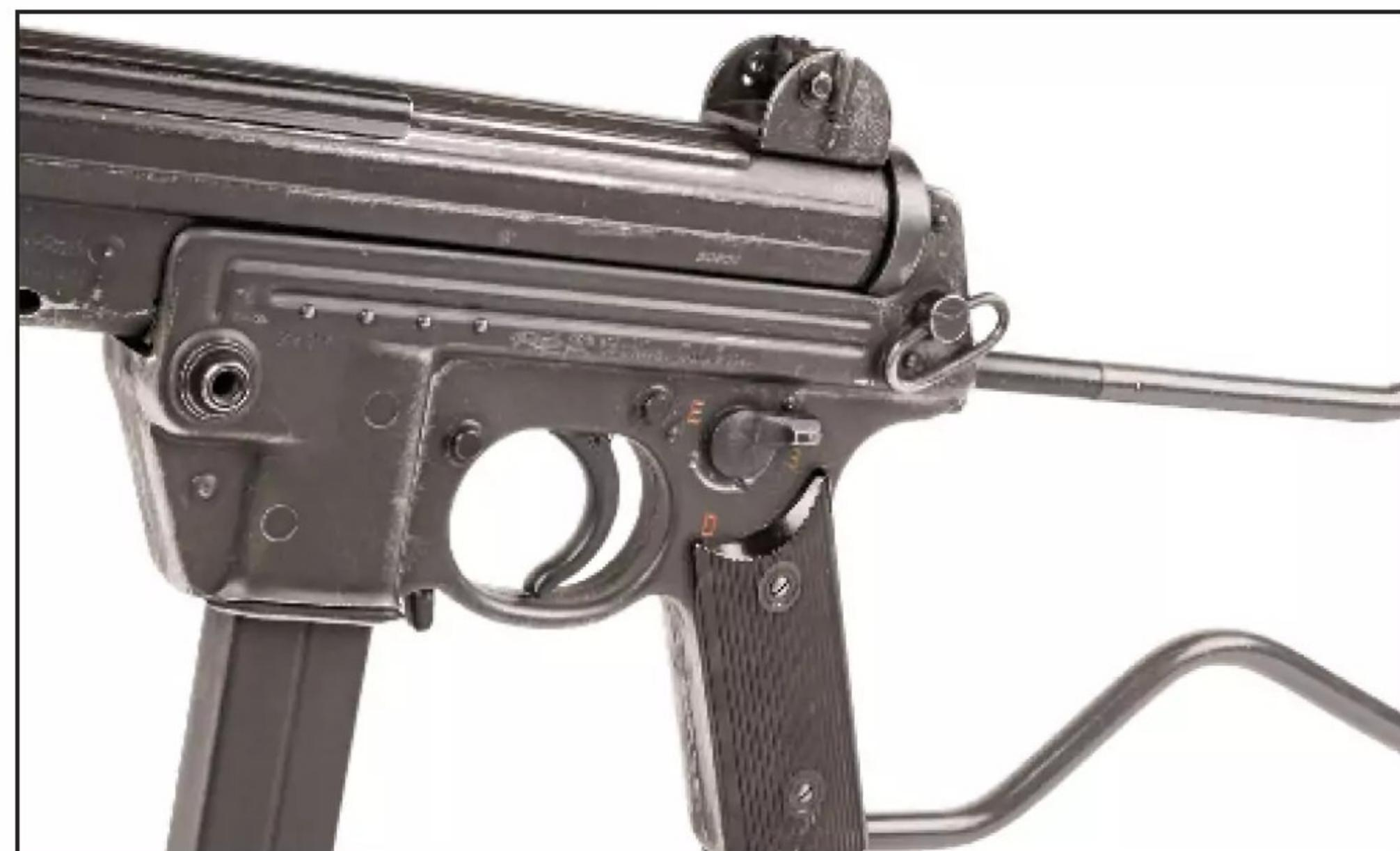
**The Walther MPL's safety selector has three positions. Pointing backwards is safe, downward is full auto, and pointing forward is semi-auto. Also note the plastic grip and sling swivel. (Will Dabbs)**
