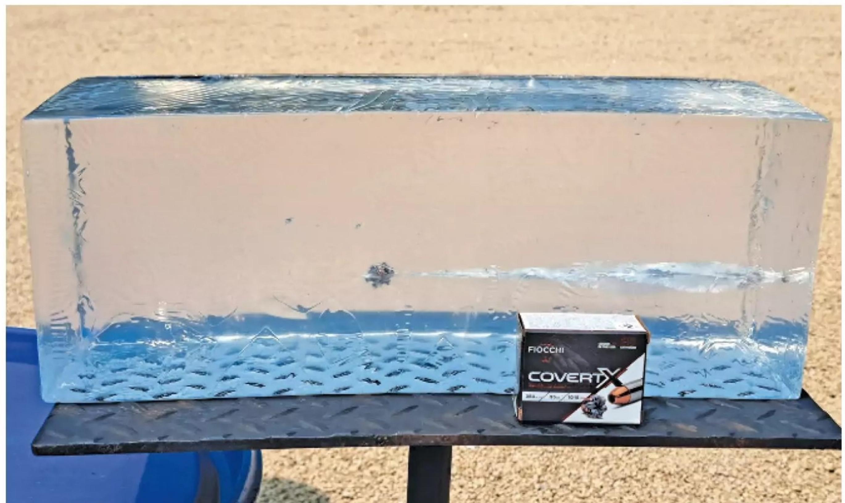
**A gel test of Fiocchi's 95-grain .380 ACP CovertX. It penetrated the block ten inches and expanded significantly. (James Tarr)**
