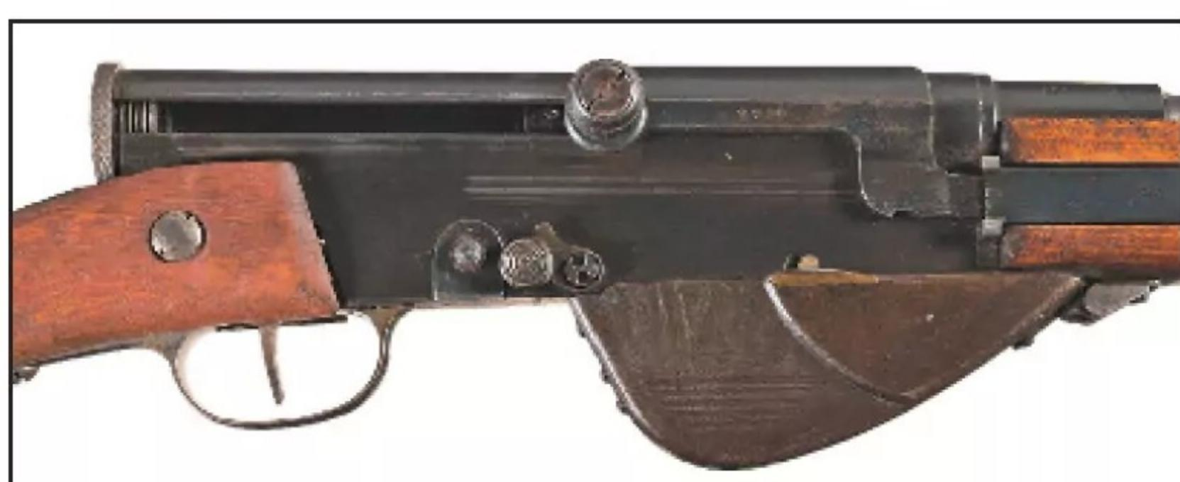
**Close up of the Modèle 1917's receiver shows the large bolt handle, full-length opening in the receiver, the bolt hold open catch, exposed operating rod and bulbous magazine housing. (Courtesy of Rock Island Auction Co.)**
