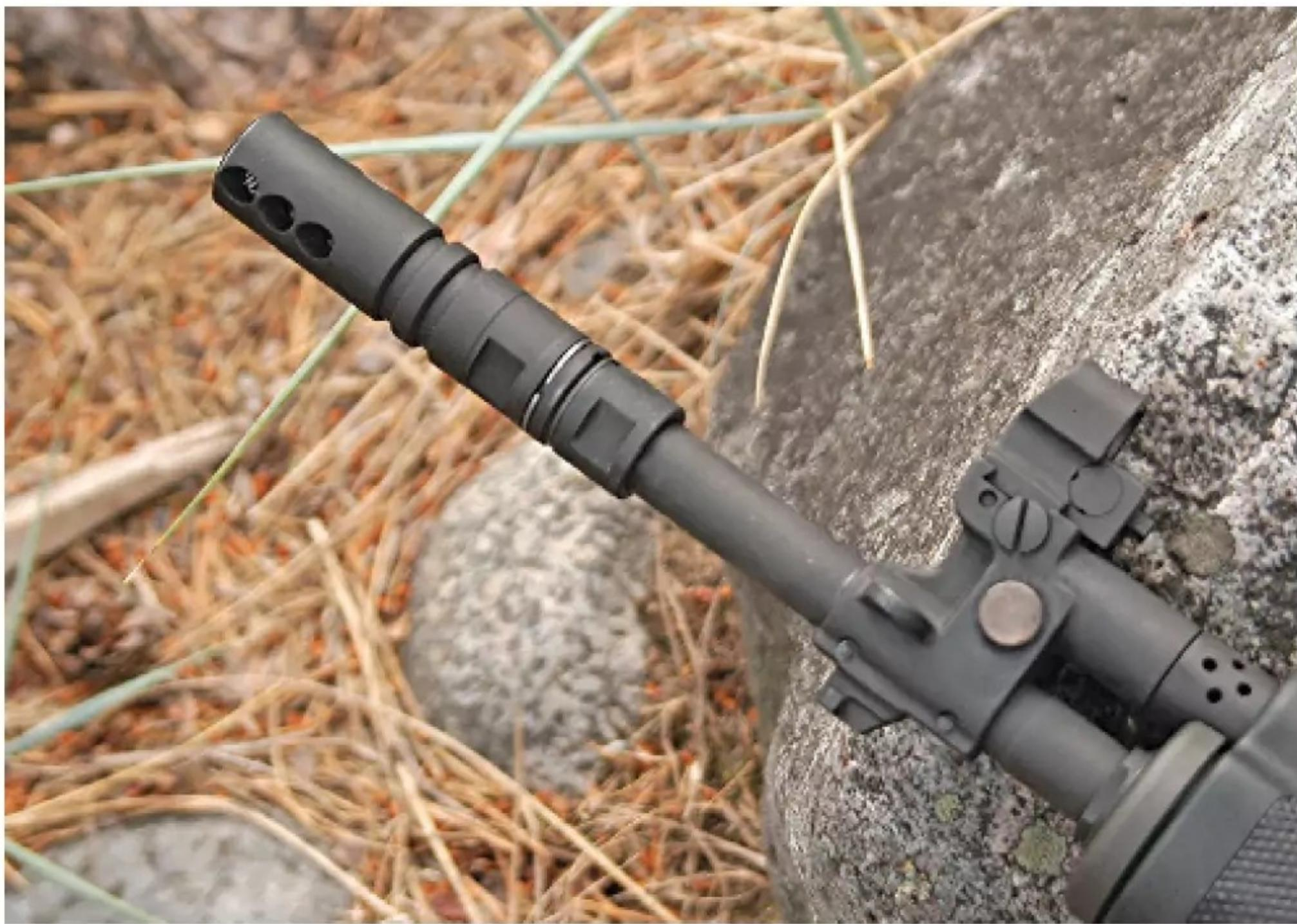
**The RK 95 TP features a combination muzzle brake/flash suppressor, which doubles as a spigot grenade launcher.**
