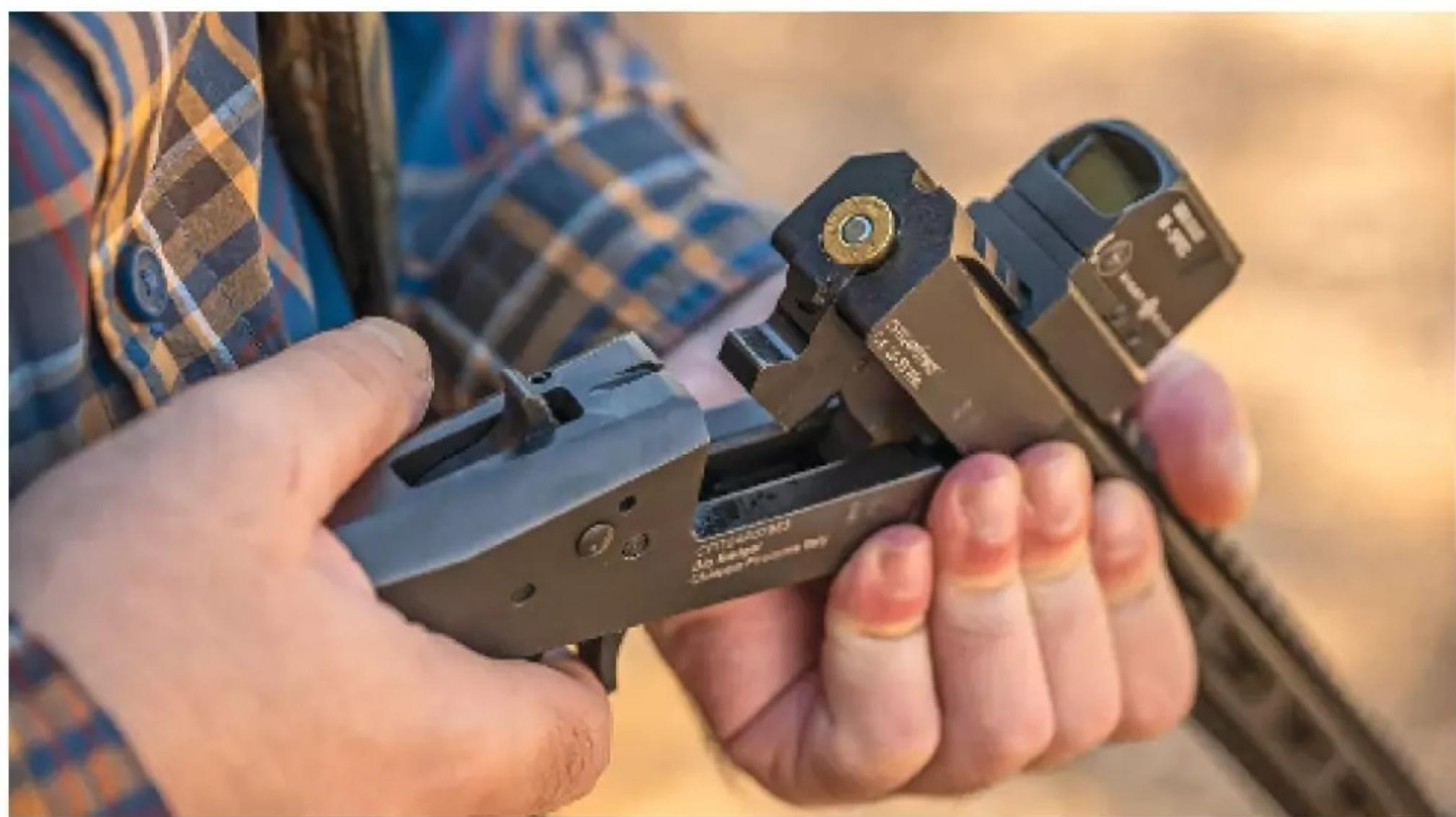
**When the Big Badger is closed, the barrel assembly and receiver are held together by a single, massive locking lug manufactured out of steel. It's sturdy enough to withstand even the highest levels of pressure that .30-30 Winchester, 350 Legend or .410 can develop. (Pierangelo Tendas)**
