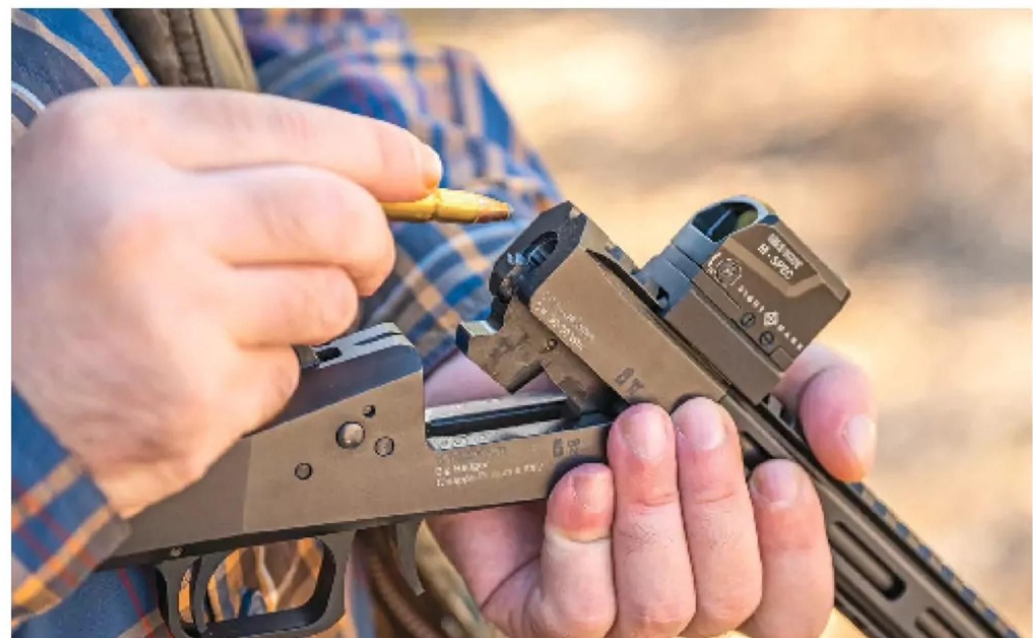
**The Chiappa Firearms Big Badger must be loaded and unloaded manually after each shot; the chamber is fluted to prevent cases to stick to the walls in case of pressure spikes. (Pierangelo Tendas)**
