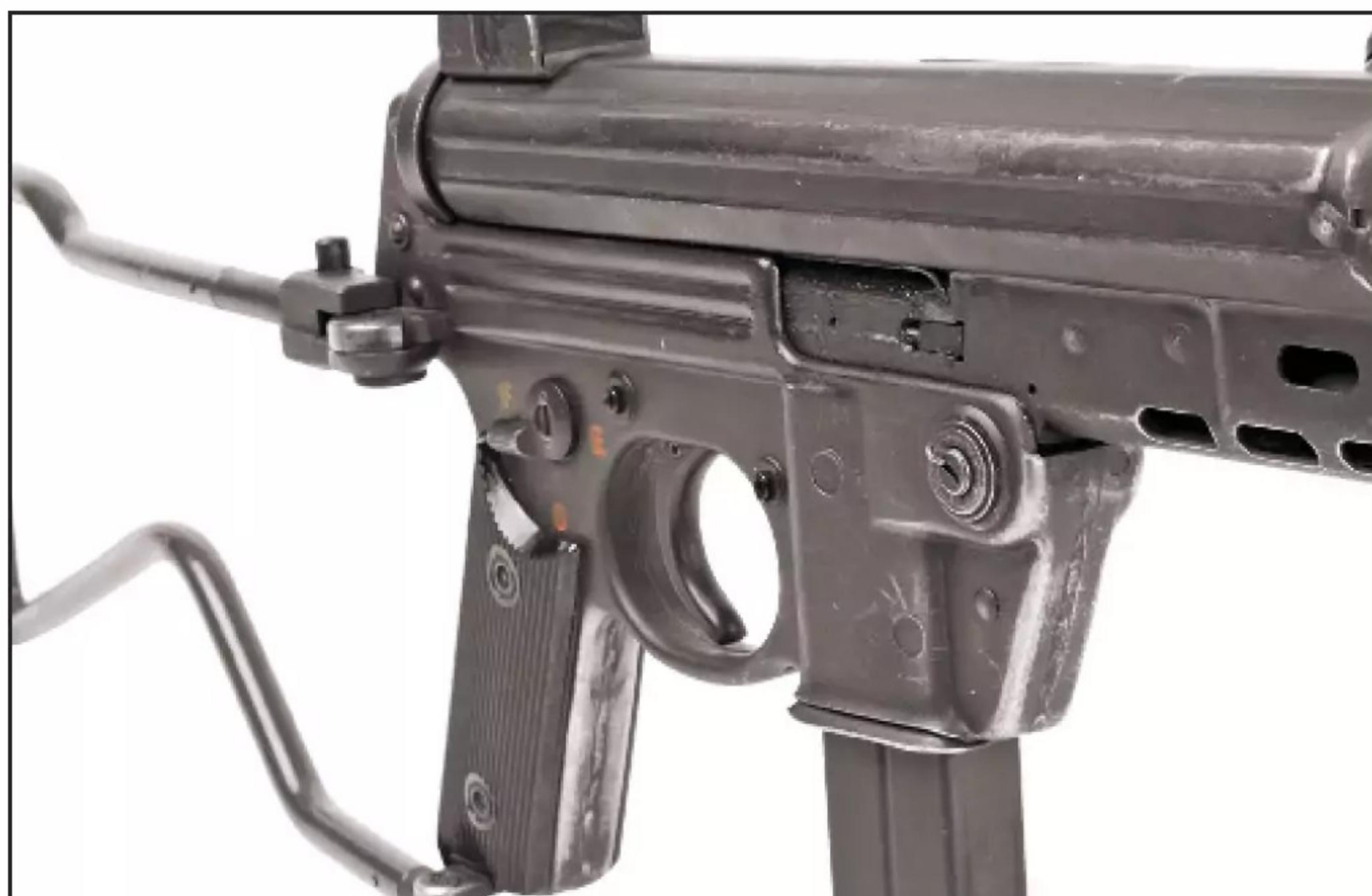
**The MPL's selector is ambidextrous and the takedown pin is of the same type as the MP5 SMG. The hinge of the folding stock is adequate. (Will Dabbs)**
