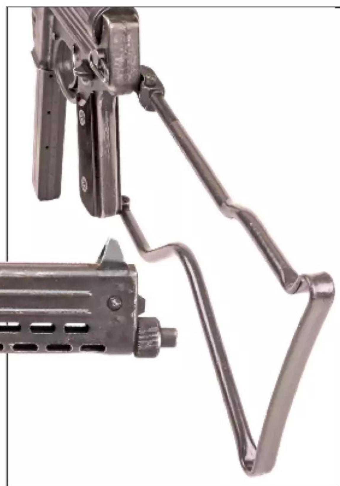
both the MPK and MPL and folds to the right when not in use. Oddly, the stock partially occludes the ejection port when closed and adversely affects reliability as a result.
