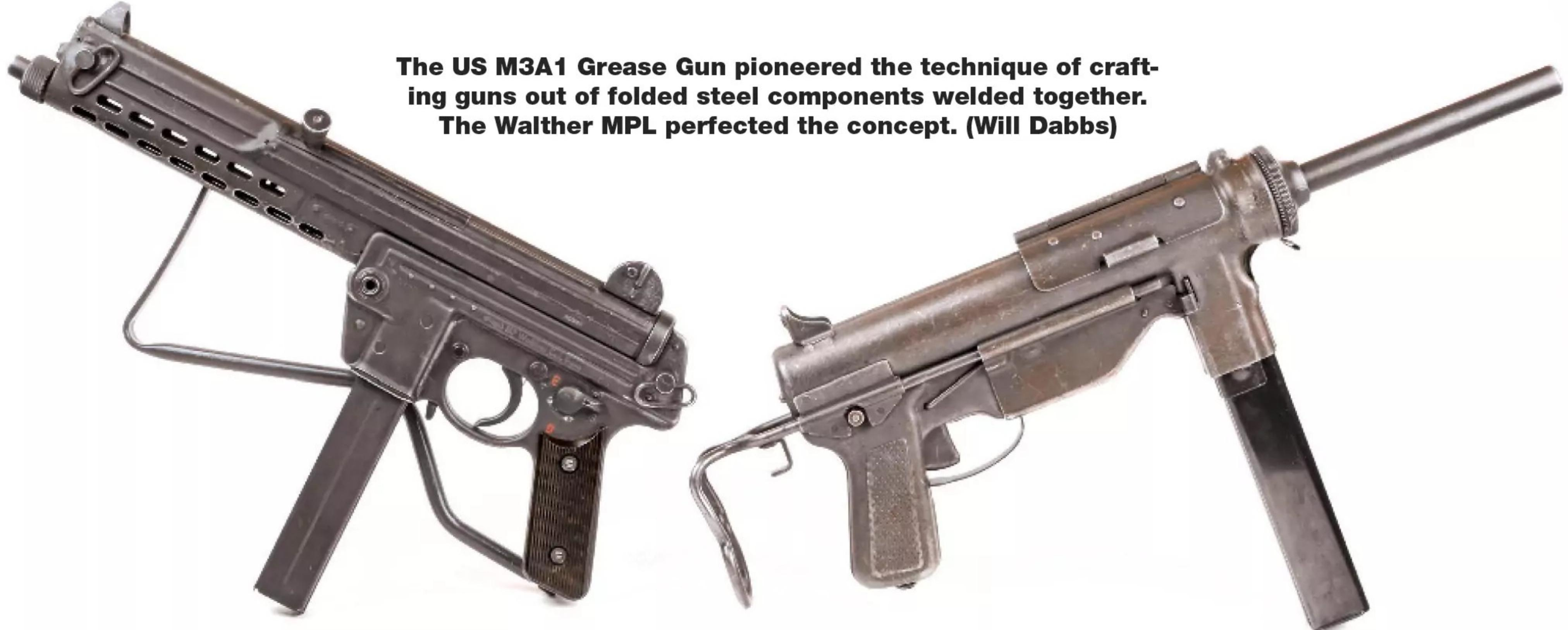
**The US M3A1 Grease Gun pioneered the technique of crafting guns out of folded steel components welded together. The Walther MPL perfected the concept. (Will Dabbs)**
