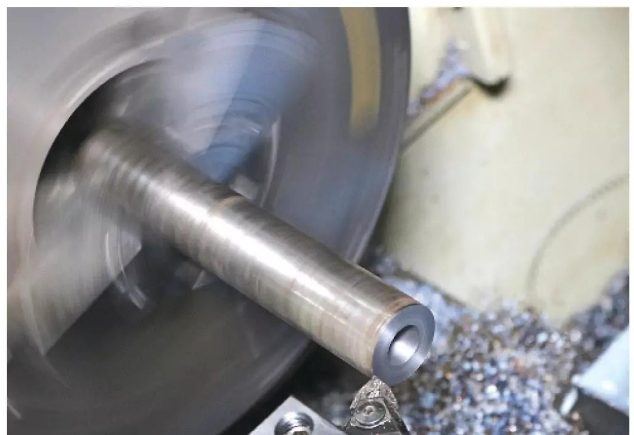
**The custom M1907 compensator began life as a piece of cylindrical steel scrap bored out and turned to shape. (Will Dabbs)**
