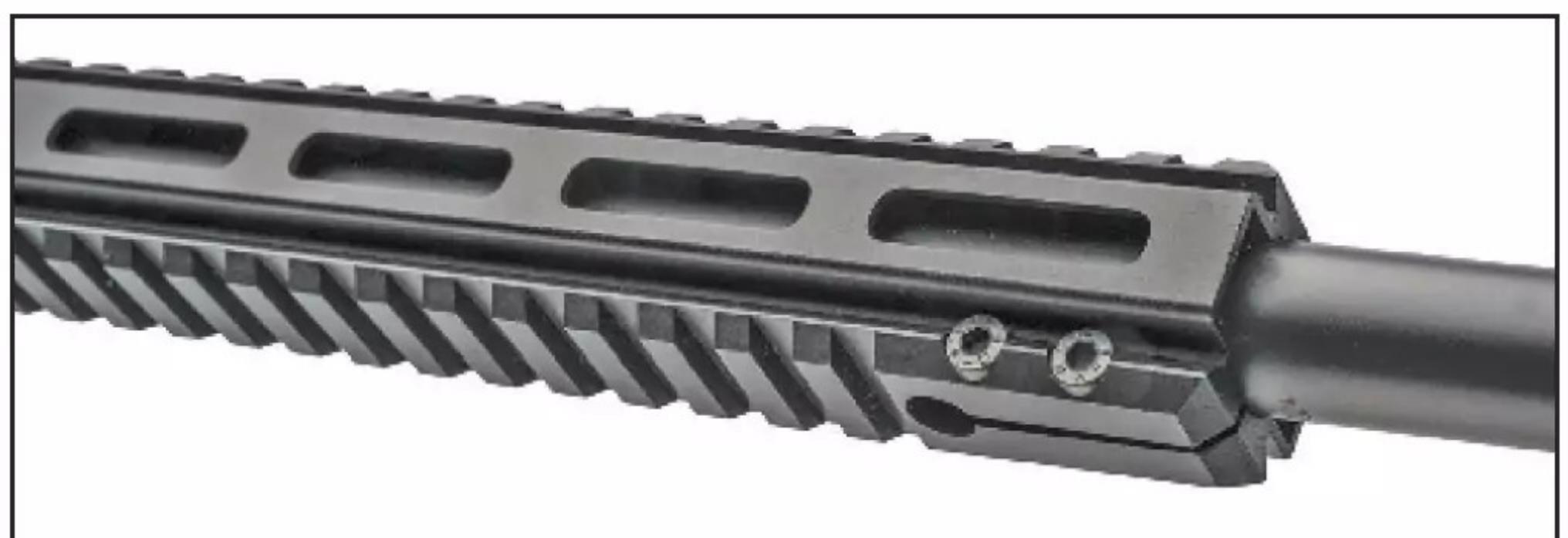
**The black polymer handguard of the Chiappa Firearms Big Badger is clamped by four screws, two at the front and two at the back. It comes with full-length top and bottom Picatinny rails and two sets of M-LOK slots on the sides. (Photo provided by Chiappa Firearms)**
