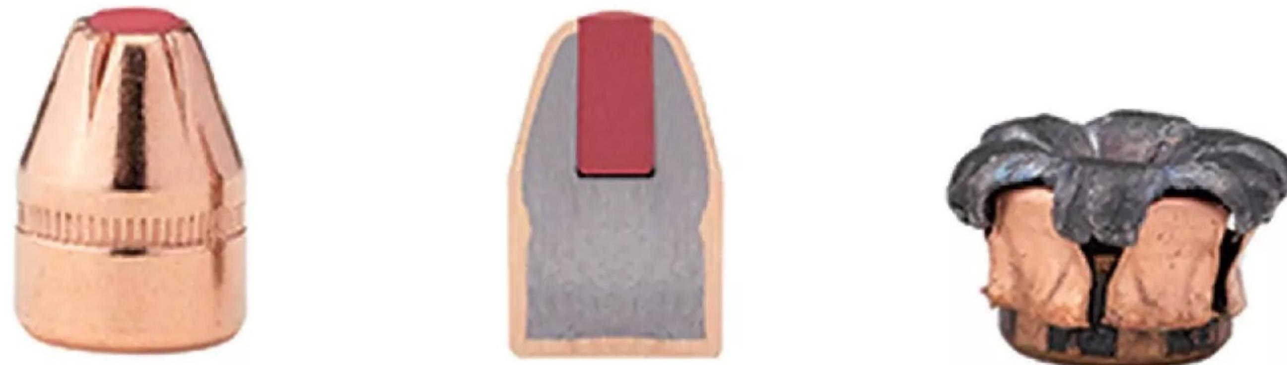
**Manufacturers use different methods to get their bullets to perform. Hornady stuffs the cavity in their Critical Defense bullets with polymer to initiate expansion. This is their 90-grain .380 bullet. (Hornady)**
