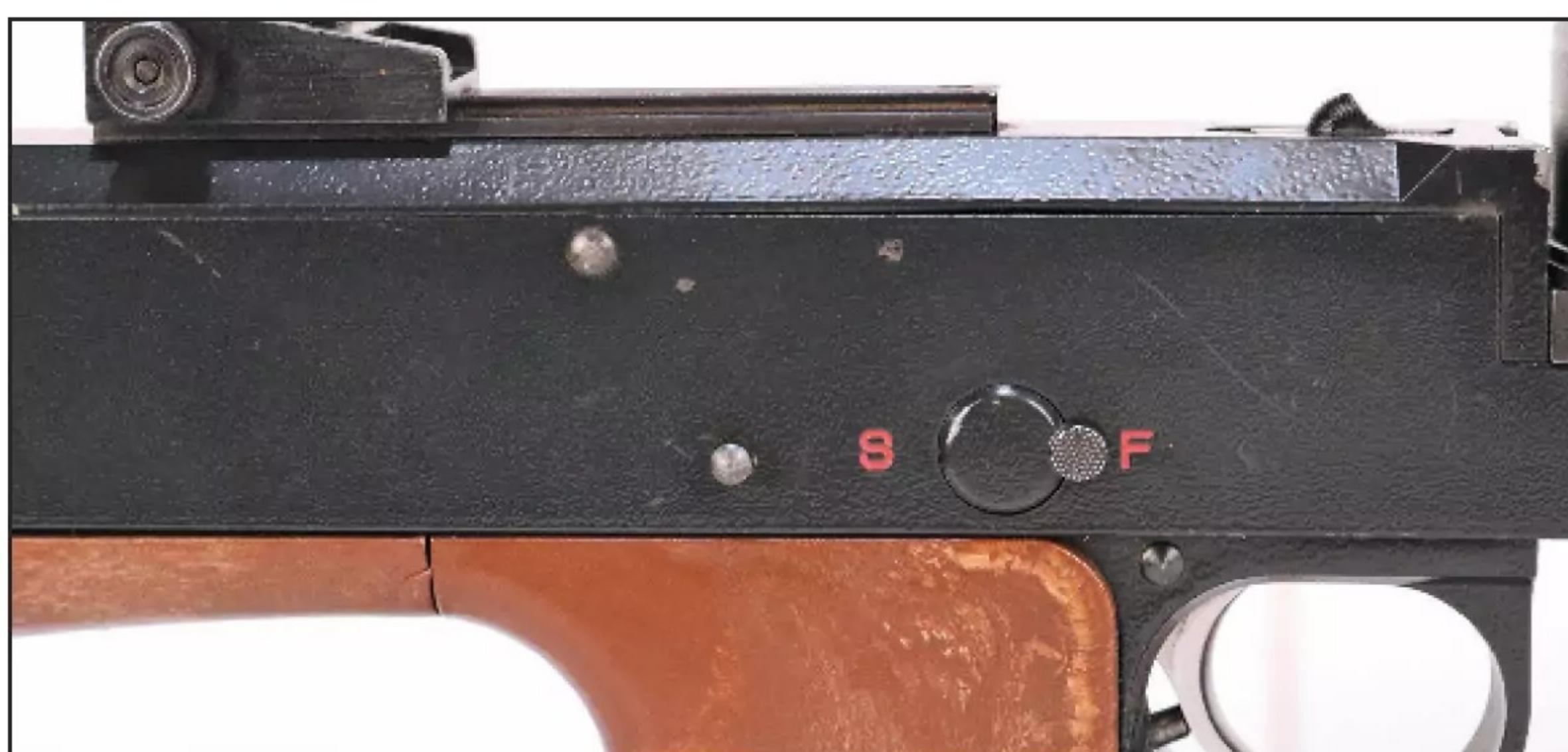
**The controls are easily mastered, but the ergonomics are suboptimal. The safety is located on the right side of the receiver. The nubbin behind the safety is the crossbolt fire selector. (Will Dabbs)**
