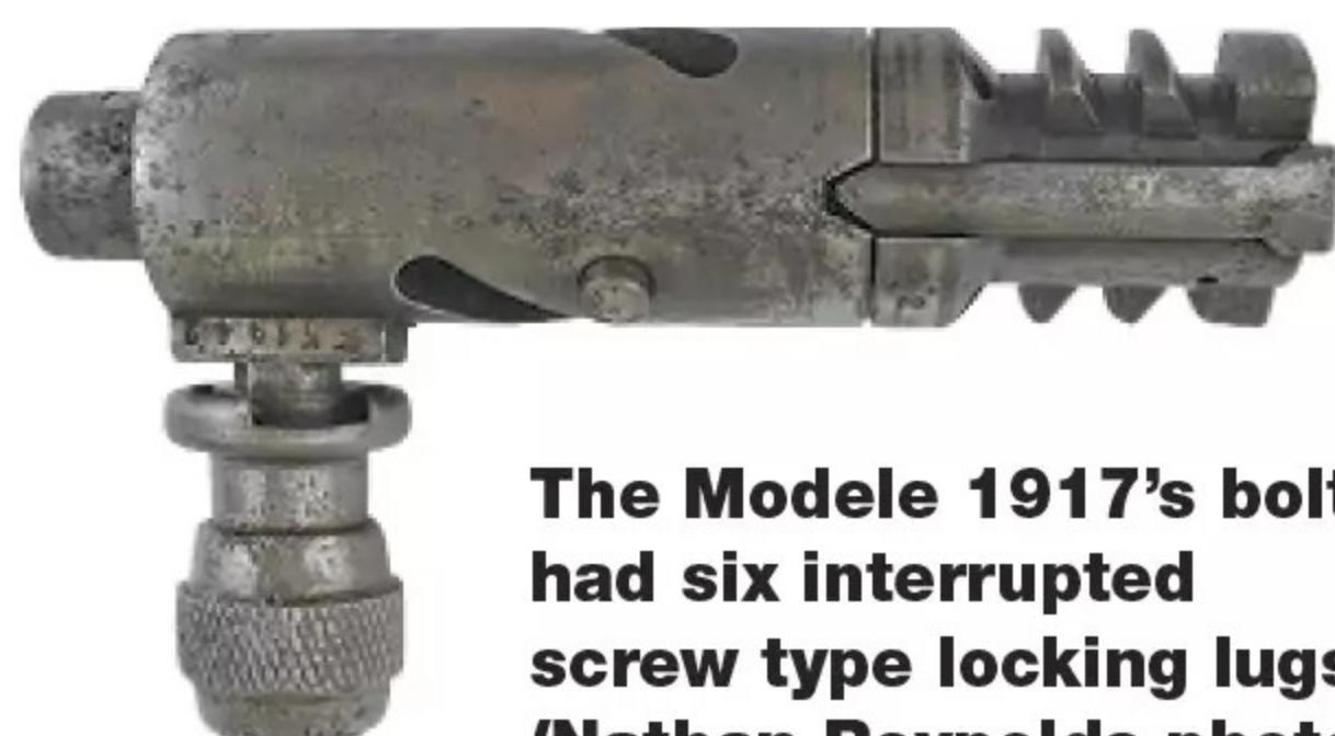
**The Modèle 1917's bolt had six interrupted screw type locking lugs. (Nathan Reynolds photo)**
