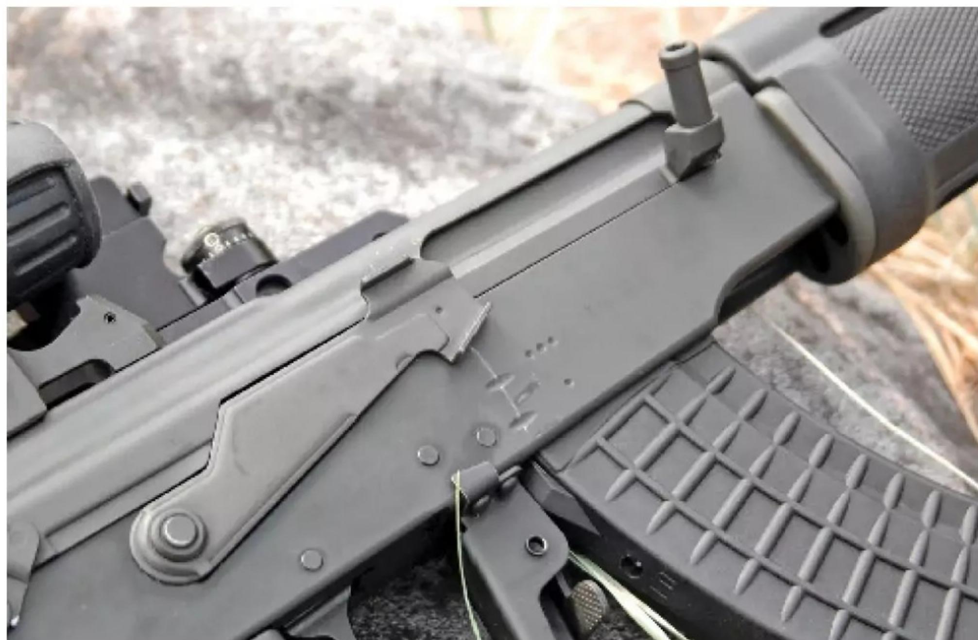
**Although the Finn's tested a thumb operated selector, in the end, they stuck with the standard Remington/Kalashnikov selector lever design. (David M. Fortier)**
