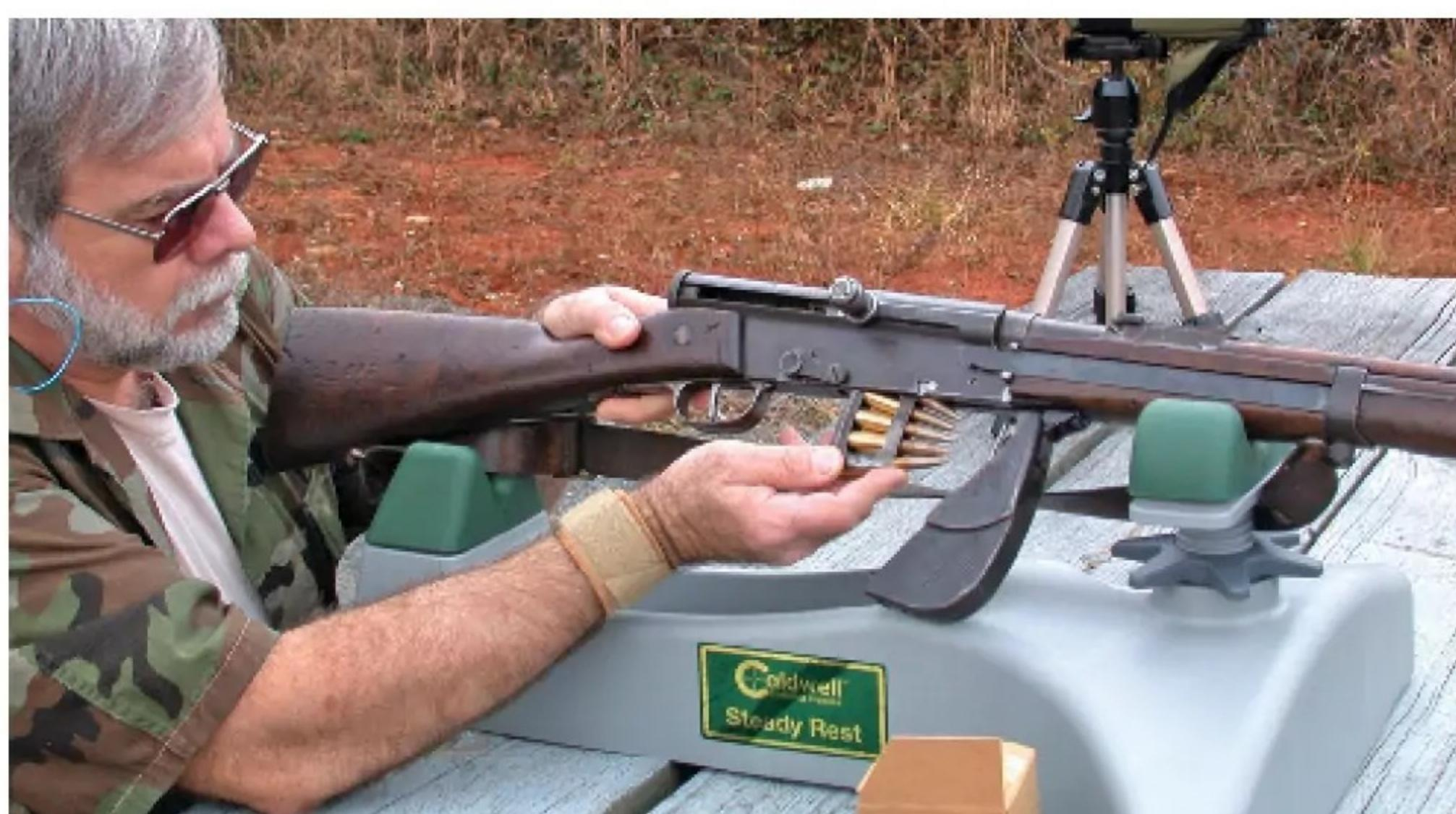
**Loading was fairly easy but would have allowed dirt and debris to enter the rifle's receiver and magazine housing. (Becky Scarlata photo)**
