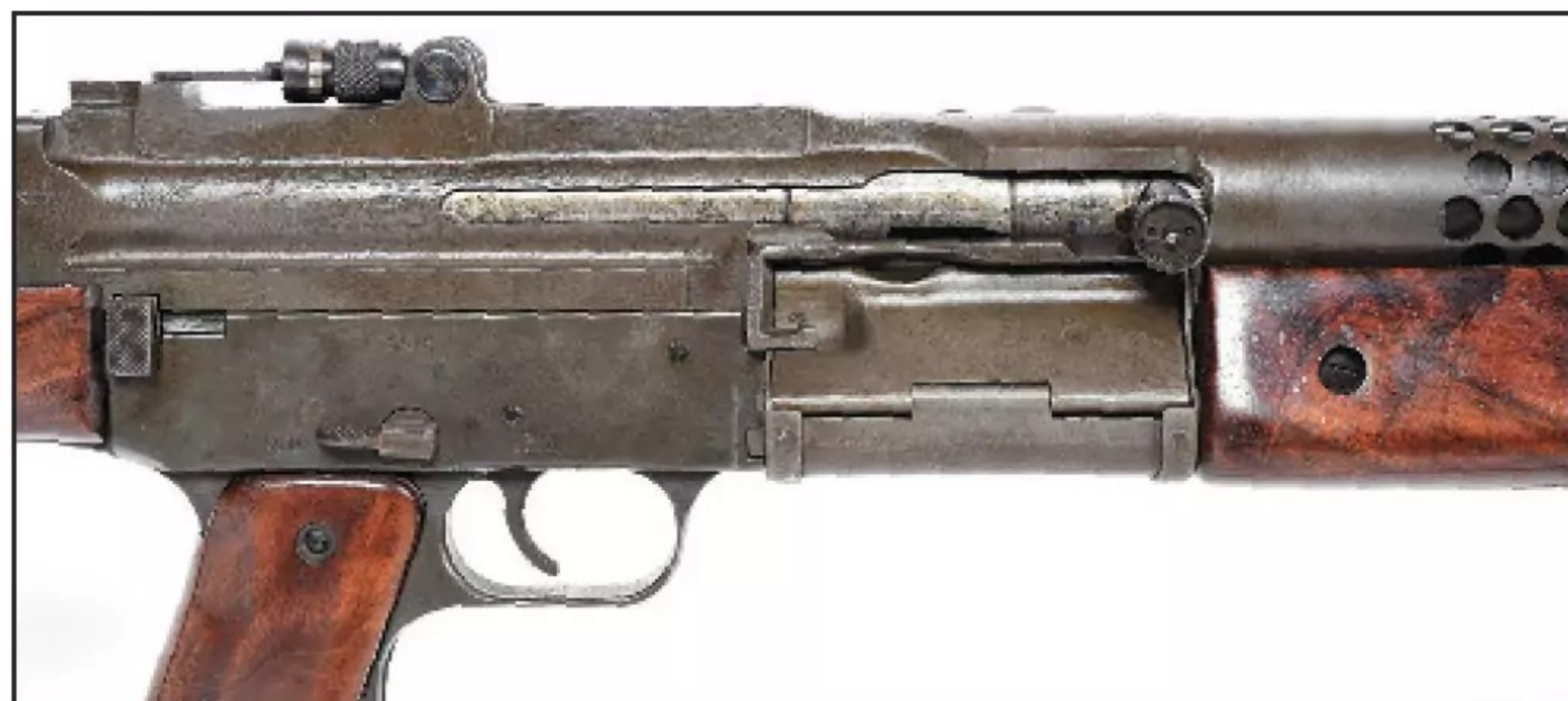
Right hand view of the receiver shows the charger guides on the magazine, and the safety lever. (Morphy Auctions)
