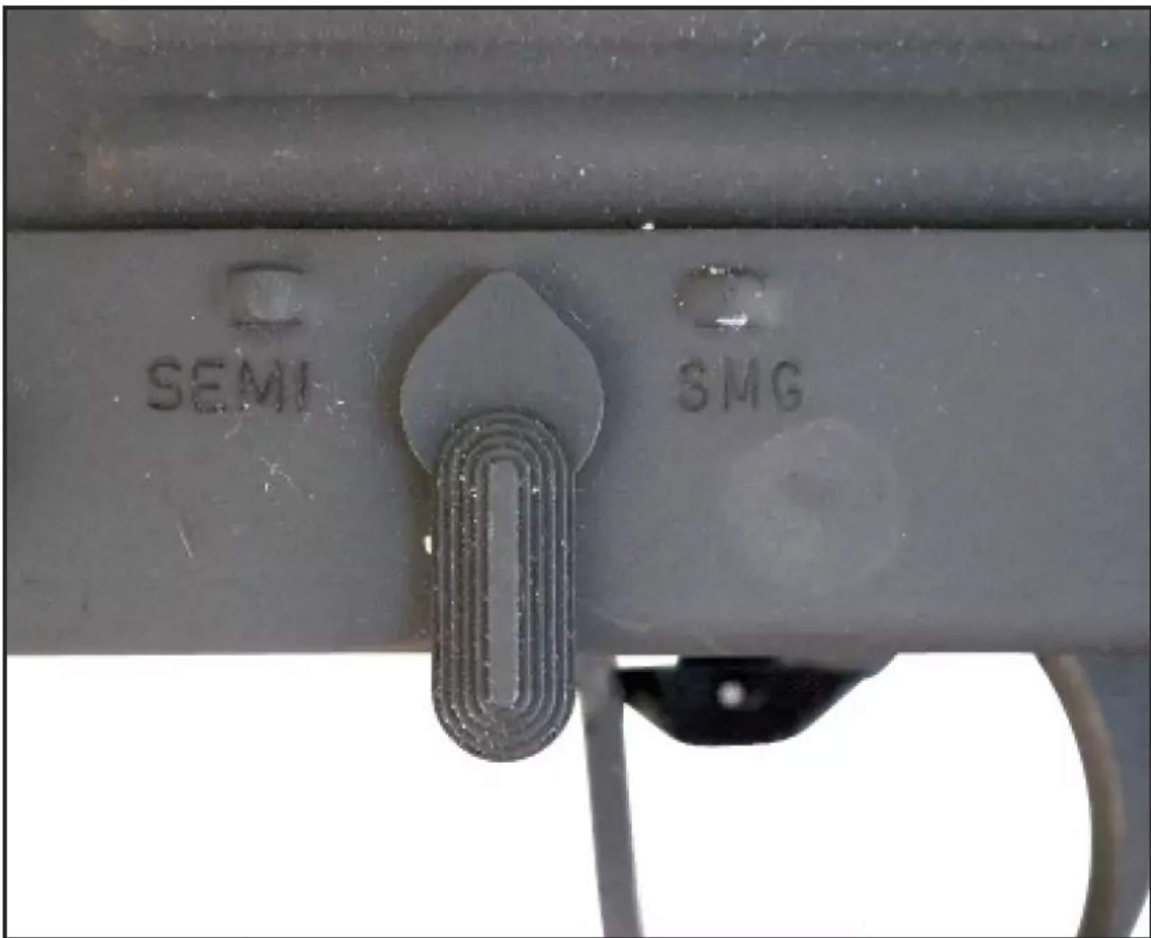
If you look closely, you can see the scant discoloration just behind the selector on the left. This means that this gun was most likely converted from a semiauto pistol prior to the 1986 machine gun ban. (Will Dabbs)
