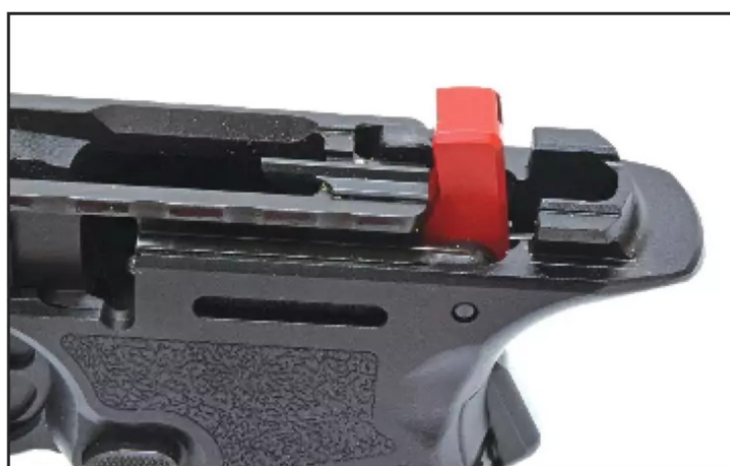
The Bulwark isn't a striker-fired pistol, but rather a semi-auto-only, with an internal hammer. The hammer, red, can be seen cocked and then released. (Photo by James Tarr)
