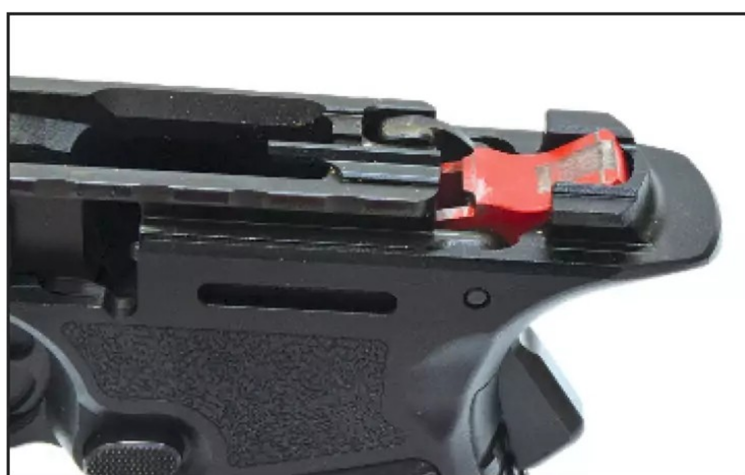
The Bulwark isn't a striker-fired pistol, but rather a semi-auto-only, with an internal hammer. The hammer, red, can be seen cocked and then released. (Photo by James Tarr)
