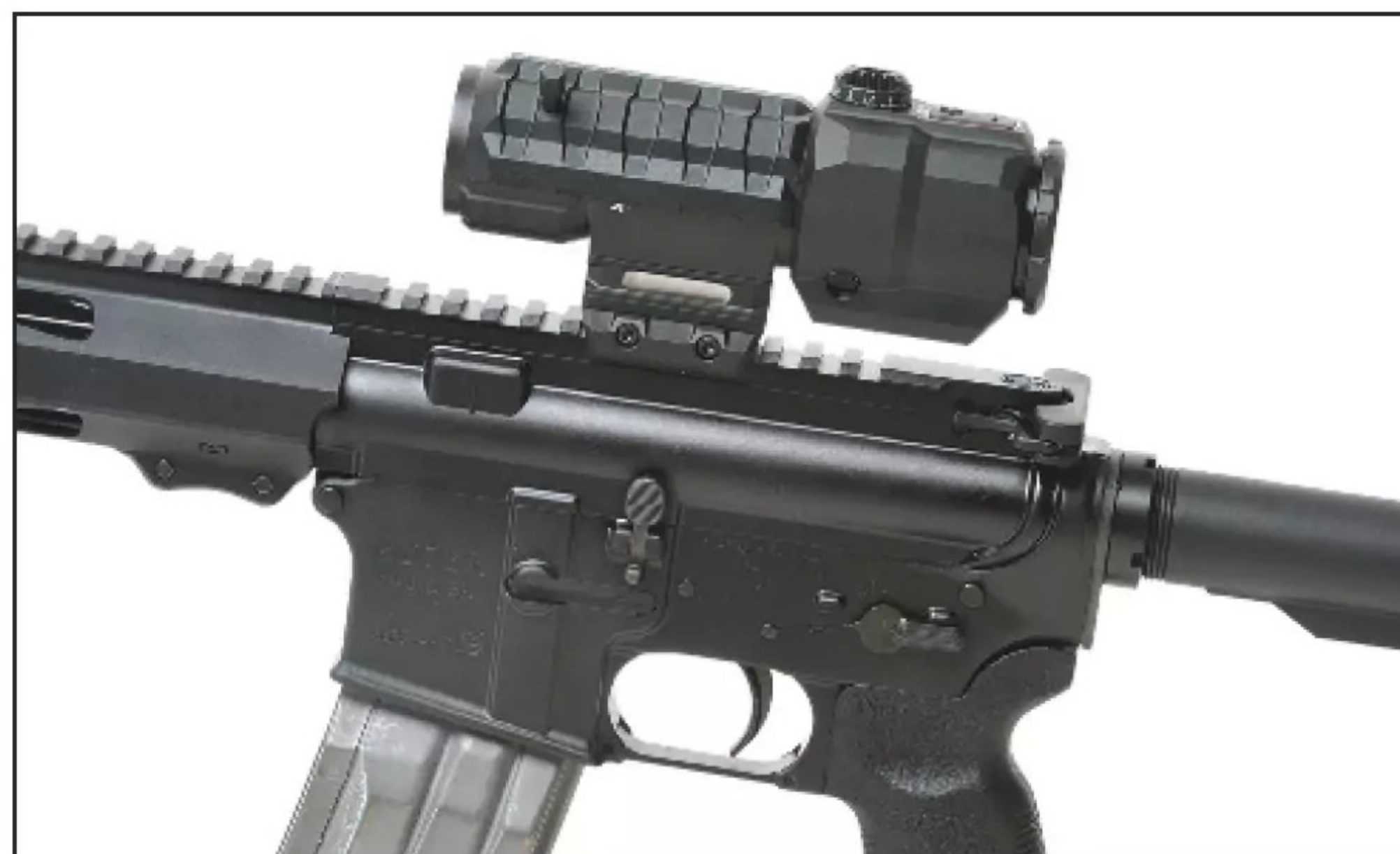
Upper and lower receivers are forged from 7075 aluminum alloy and feature a Type III hard coat finish for durability and corrosion resistance. (Photo by David M. Fortier)
