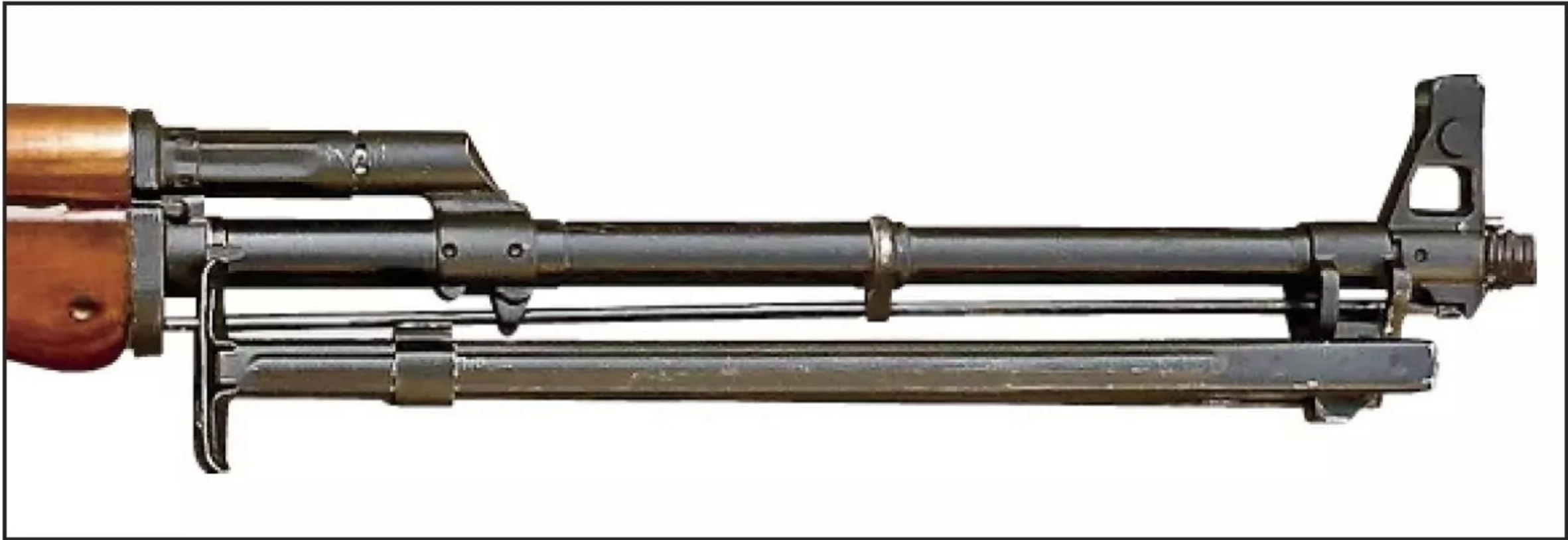
A longer barrel on the RPK improves ballistics of the 7.62x39mm cartridge; the folding bipod gives more stability when firing prone. (Leroy Thompson)
