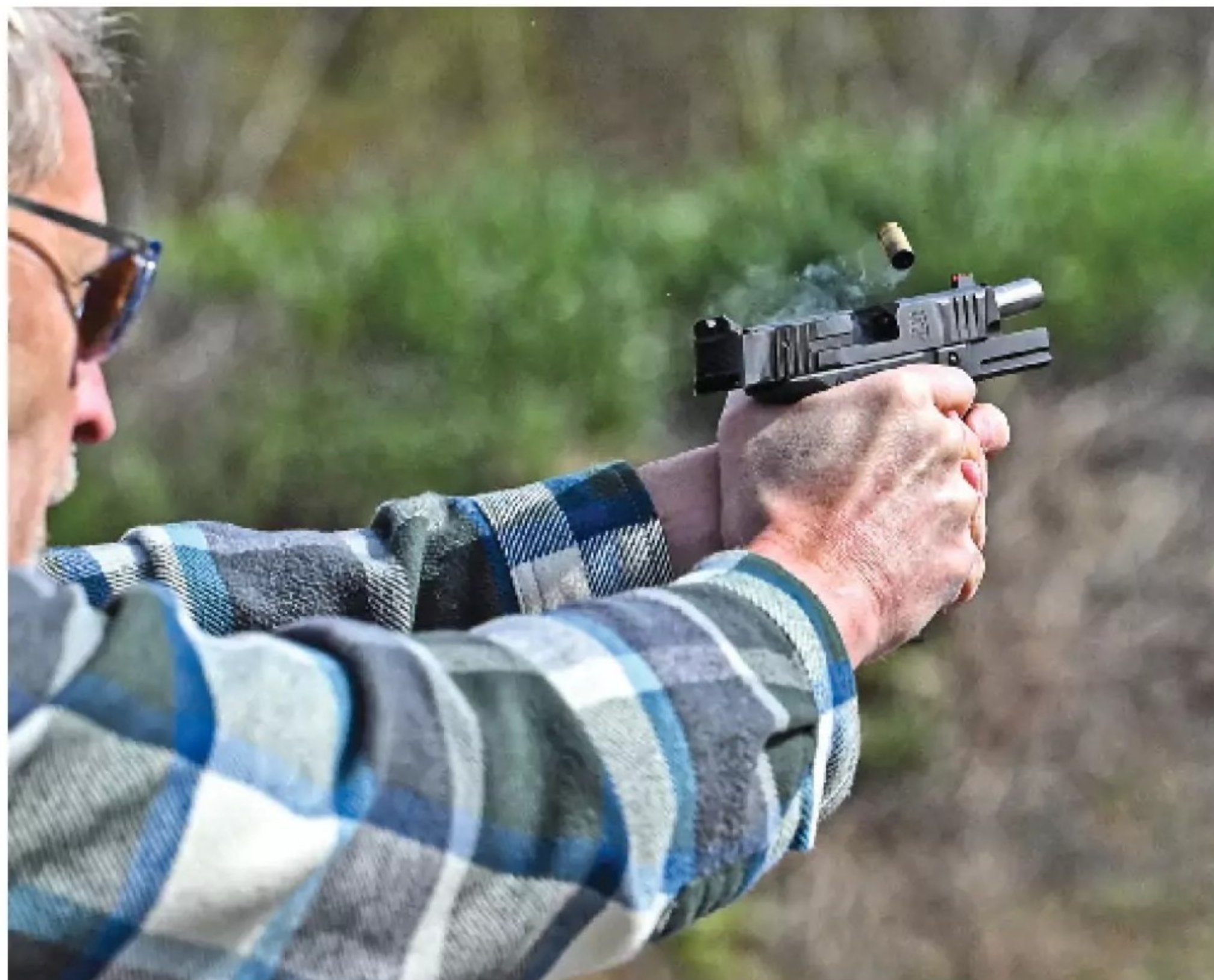
The Bulwark has the low bore of a striker-fired pistol, but with an aluminum frame it weighs more, so it was very controllable. (Photo by Andy Grossman)
