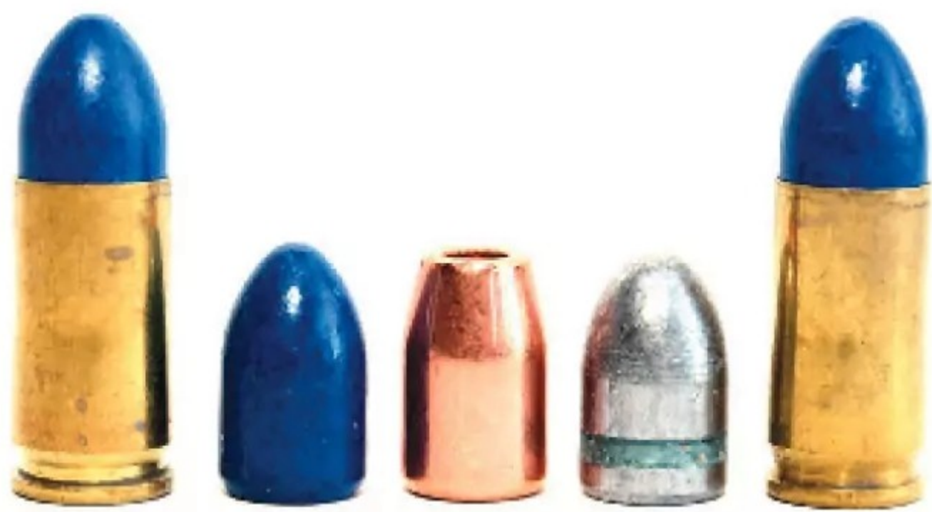
The charge of 3.6 grains of Vihtavouri N330 works pretty much regardless of what 125-grain 9mm bullet you use. Here, a Blue Bullet loaded round flanks a Blue Bullet, a Berry's plated hollow point, and a hard-cast 125-grain round nose. (Patrick Sweeney)
