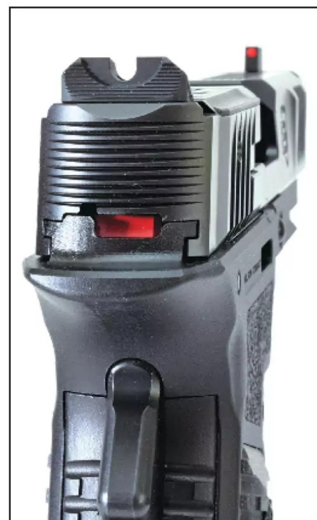
The Bulwark isn't a striker-fired pistol, but rather a semi-auto-only, with an internal hammer. The hammer, red, can be seen cocked and then released. (Photo by James Tarr)
