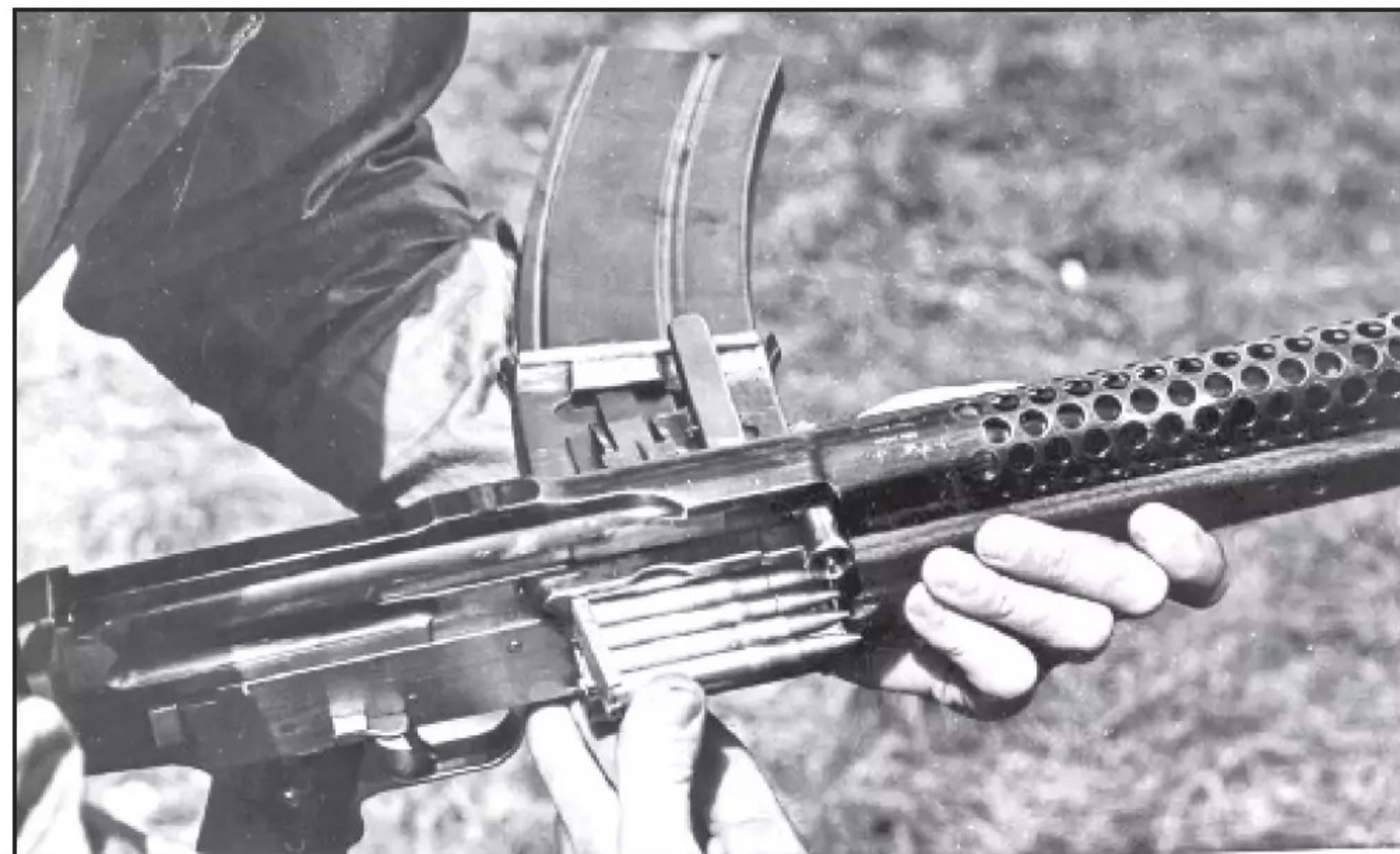
Like the Johnson rifle the LMG's magazine could be loaded with five round chargers. (Photo provided by James Walters)
