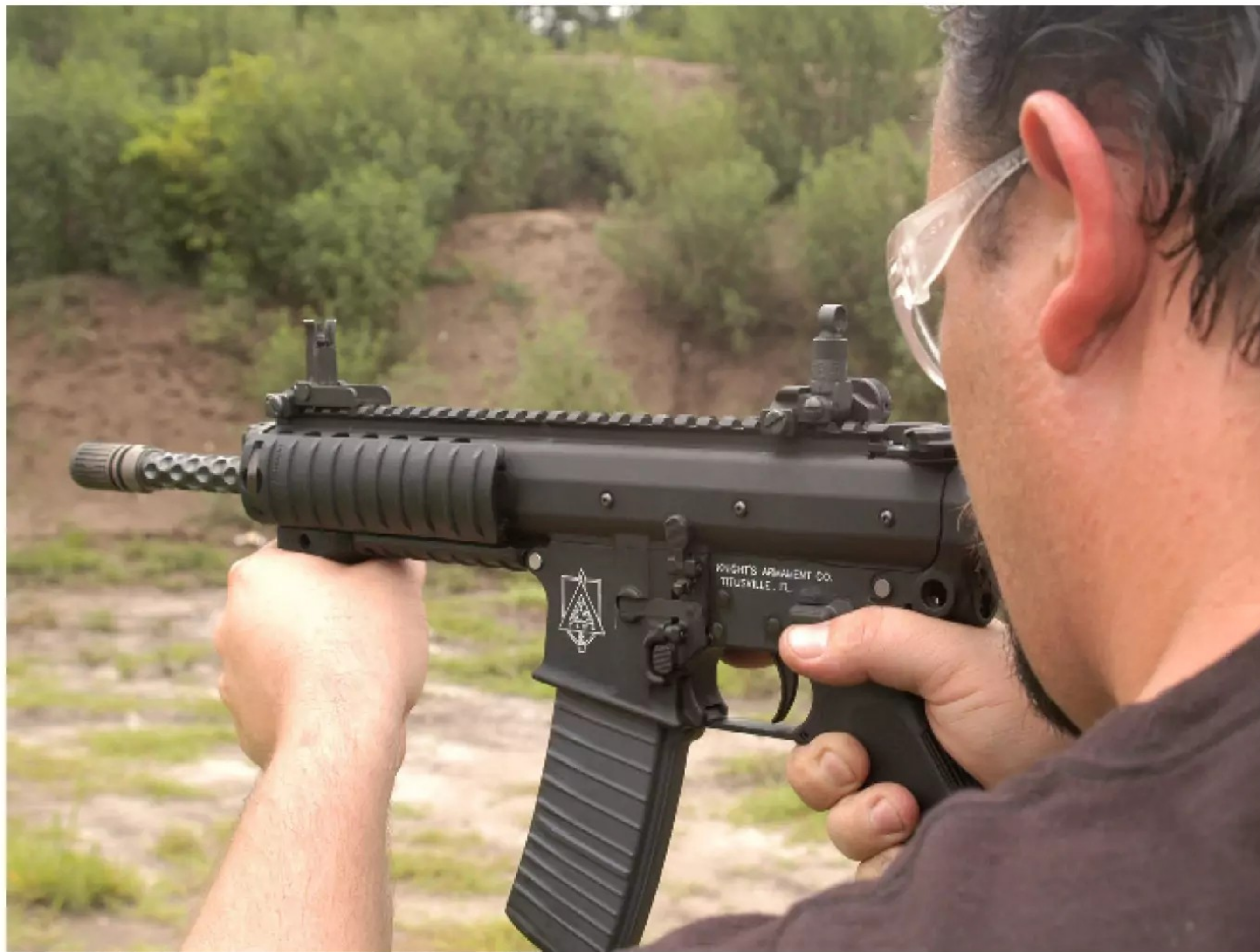
KAC's 6x35mm TSWG cartridge was designed to perform well from eight and 10-inch barrels reducing muzzle flash, blast and noise compared to a short barrel 5.56x45mm. (Photo by David M. Fortier)
