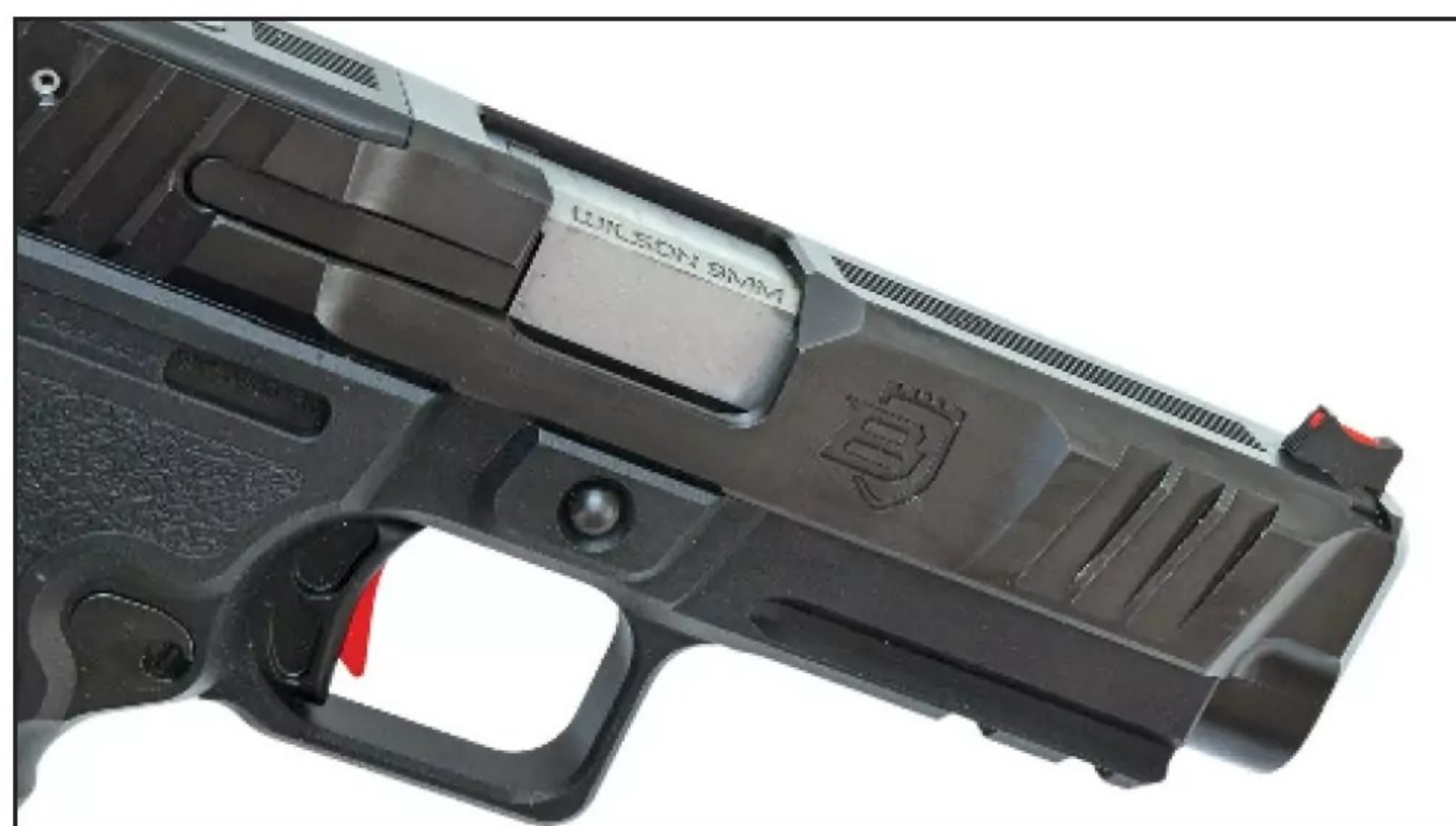
The Bulwark uses an external spring-powered extractor. The Bulwark logo is on the slide just forward of the ejection port. (Photo by James Tarr)
