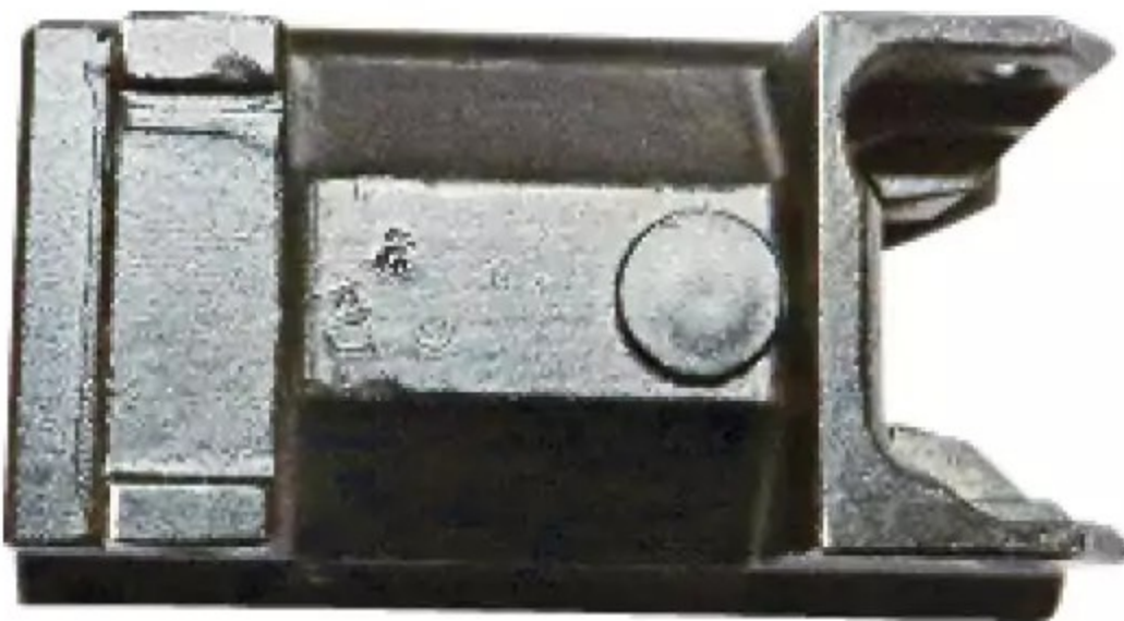
◀ The RPK has a reinforced barrel trunnion to handle the longer bursts likely to be fired from it. (Leroy Thompson)
