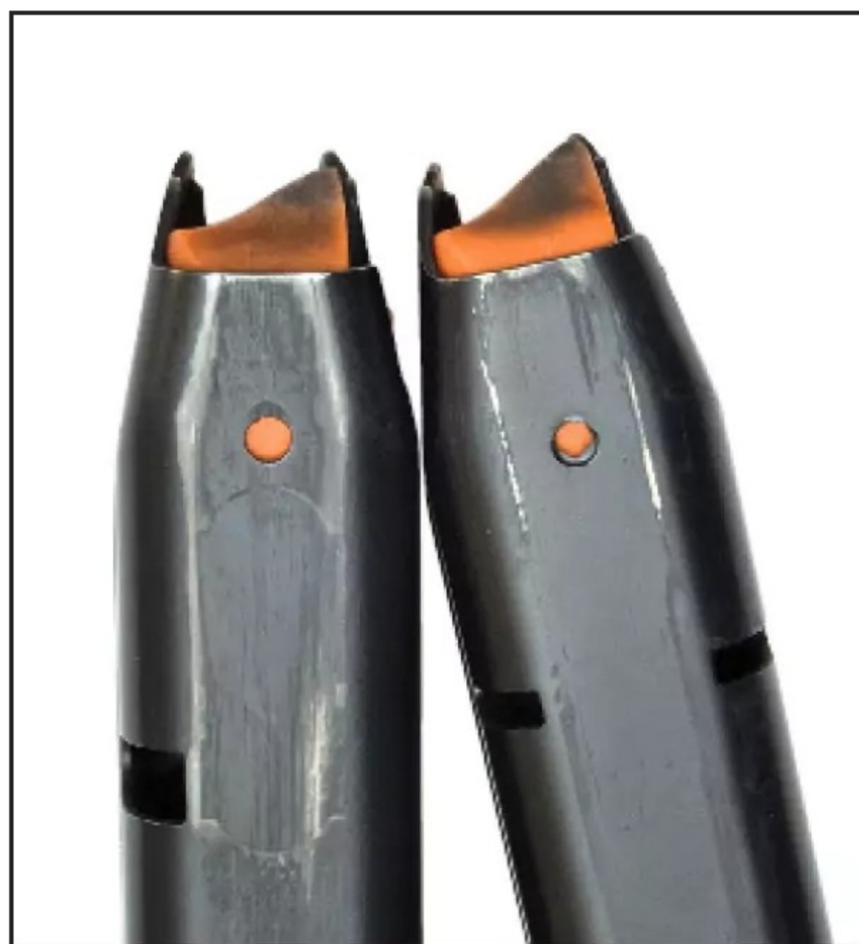
◀ The Bulwark magazine (right) uses the same body and follower as Wilson's EDC X9 magazine (left), but it has a different magazine release notch. (Photo by James Tarr)
