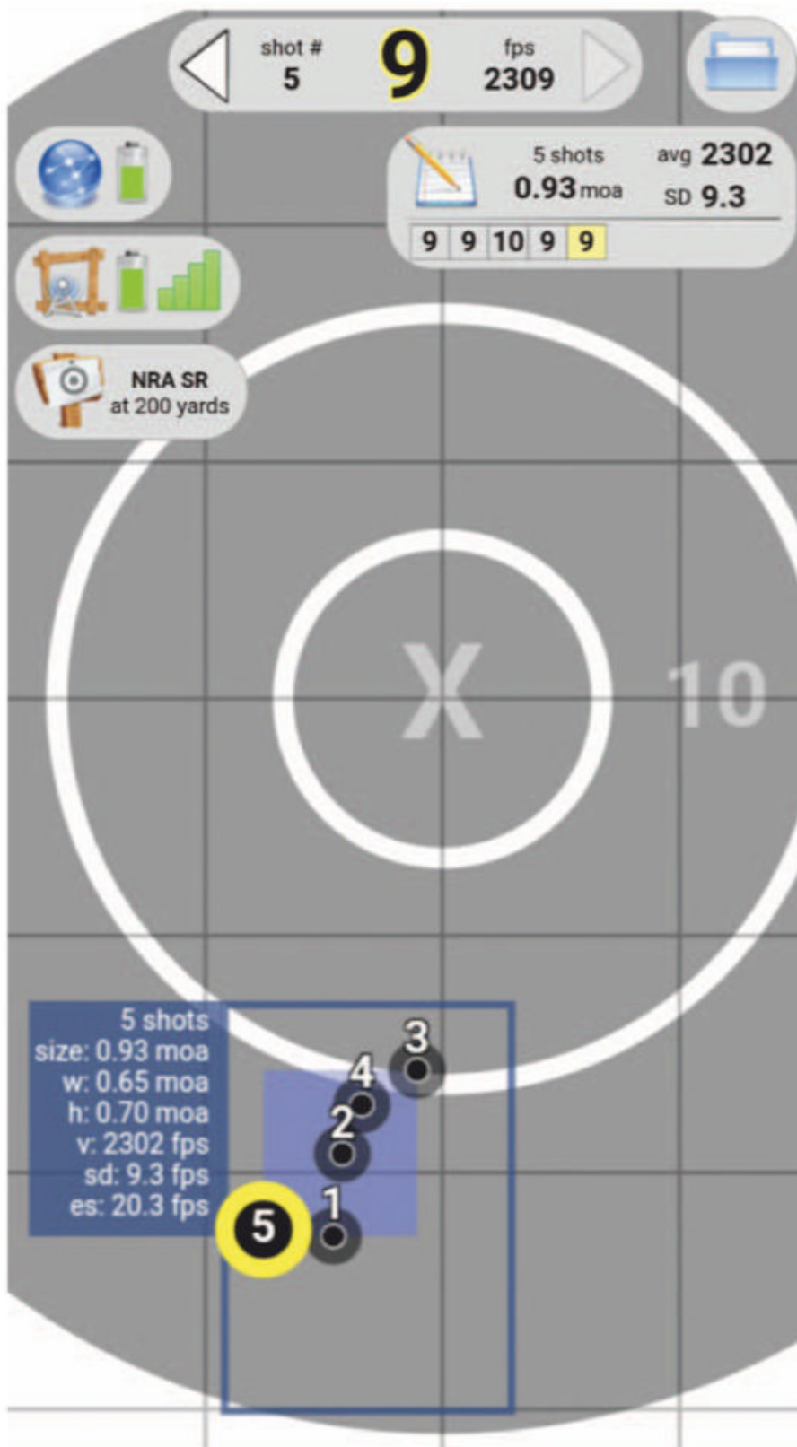
Below: A ShotMarker Electronic Target showing that the CZ's five-shot group with 165-gr. Sierra Gamechanger ammunition at 200 yards measured 0.93 MOA.
