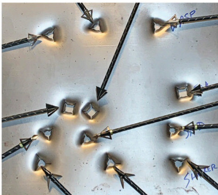
These photos show the various shapes and sizes of holes our test broadheads left in the .03-inch thick sheet metal used in our Hard-Impact Test.
