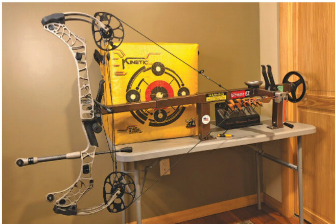
It is easy to check cam timing using a draw board and make adjustments if necessary. In this case, the Mathews V3X being checked displayed perfect cam synchronization, with both top and bottom draw stops contacting the cables simultaneously.
