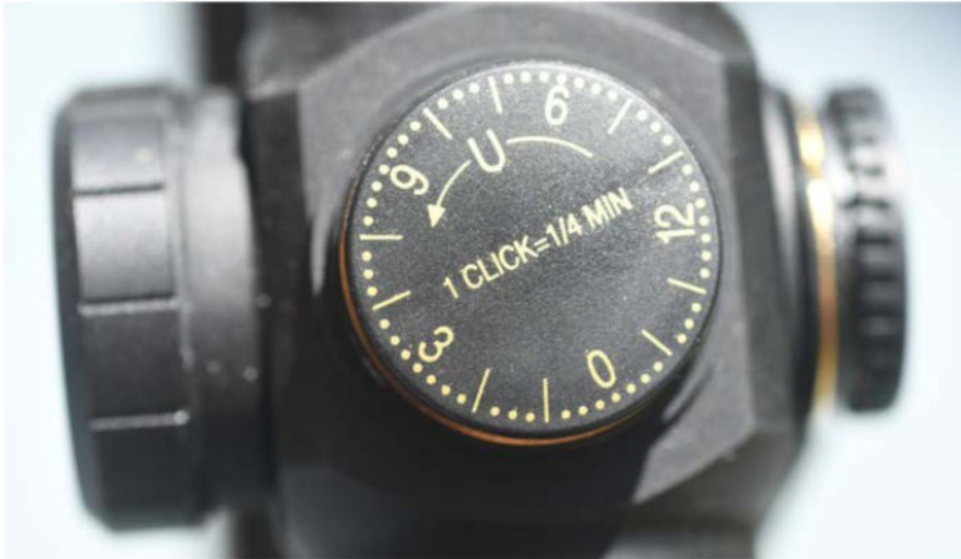
The turret adjustments on low-powered scopes are positive, simple and easy to follow.
