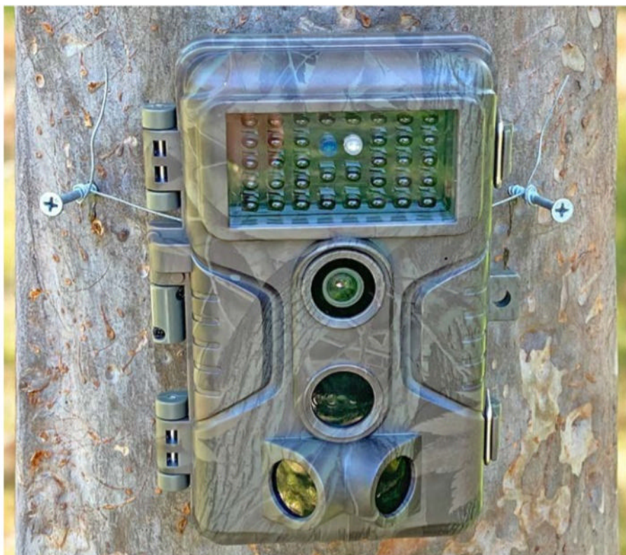
Don uses self-tapping galvo screws and fine galvo wire to mount trail cameras.
