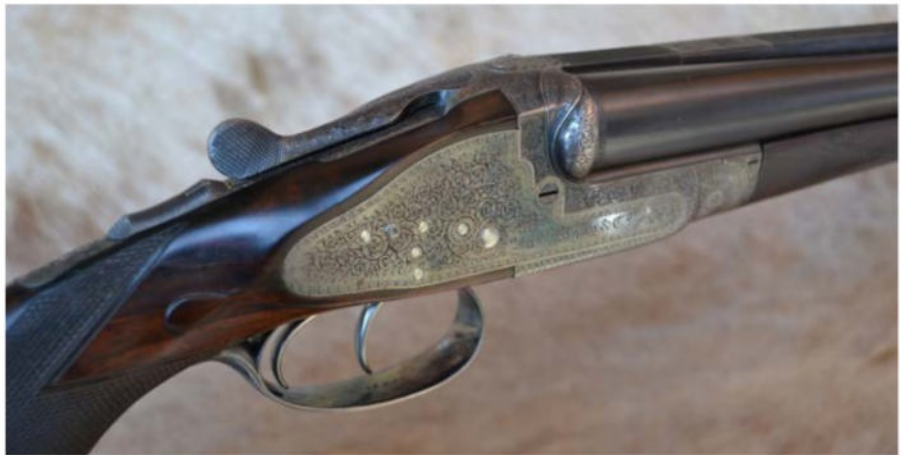
The recently resurrected Rigby/Bissell-patent rising-bite action was initially used from 1879 to 1912. Pictured is a .303 double rifle from 1898.
