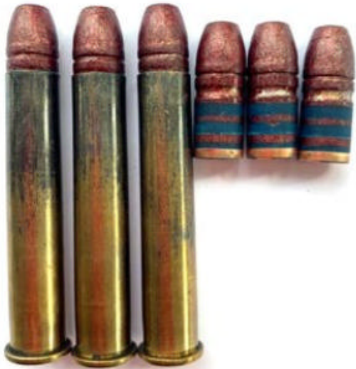
.38-55 Win loaded with 265-grain WW metal cast bullets, Hi-Tek coated, GC.
