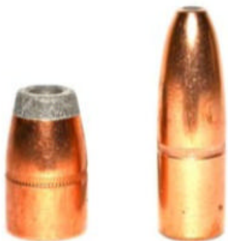
Although not the same shape or construction, this photograph serves to illustrate the difference in SD between a 300-grain .458 (left) and a 300-grain .375 bullet.
