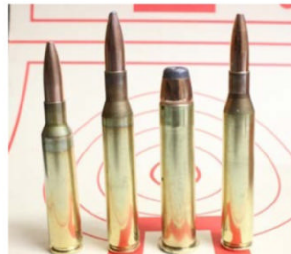
The two cases on the left are properly annealed.
