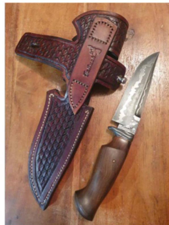
A 4.5" trailing clip point with large dagger-style swedge boasts a nine-layer San Mai blade with 1095 steel as the core, 15N20 pure nickel and 1074 cladding with Damascus half hand guard featuring a copper spacer and inland rosewood handle, with a left-hand sheath.
