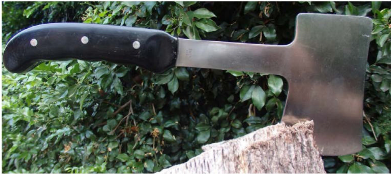
Softer steels have their place, especially on tools which see hard direct force impact use where stiffer steels may shatter.
