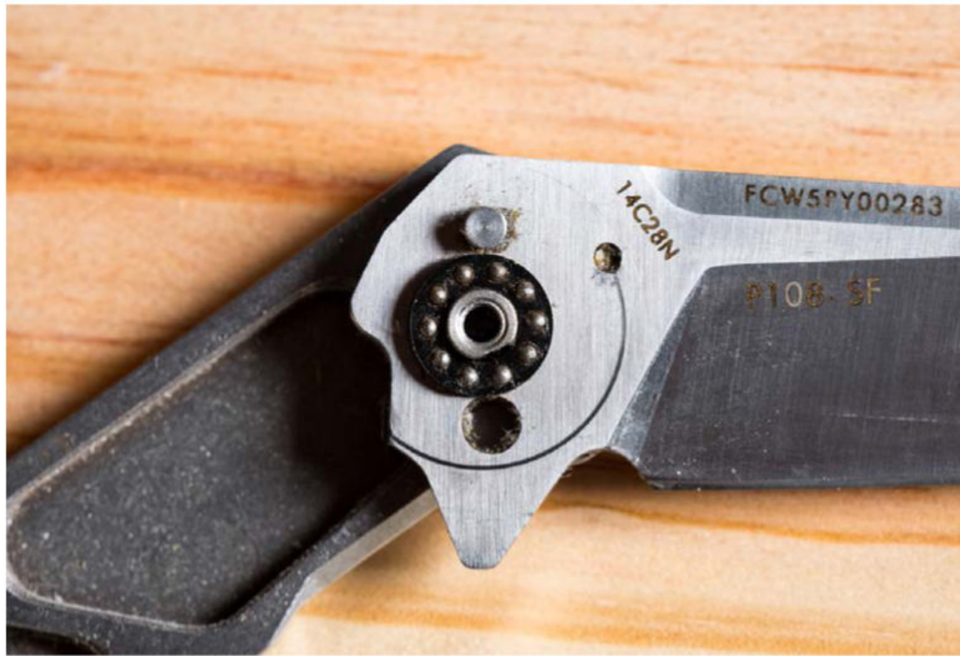
The ball bearing washer after spending half a year lost in the mud.
