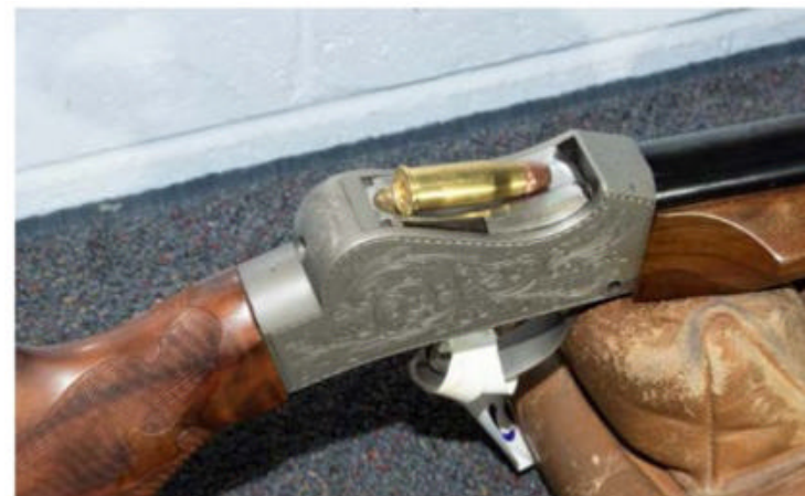
The body of the action of this Martini rook rifle has been engraved then treated with nitrates to cause the metal to remain as in the raw.
