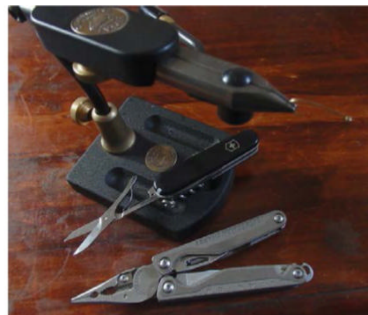
Steel for vices, scissors, blades and multi-tools all require different compositions and treatments depending on their intended use.
