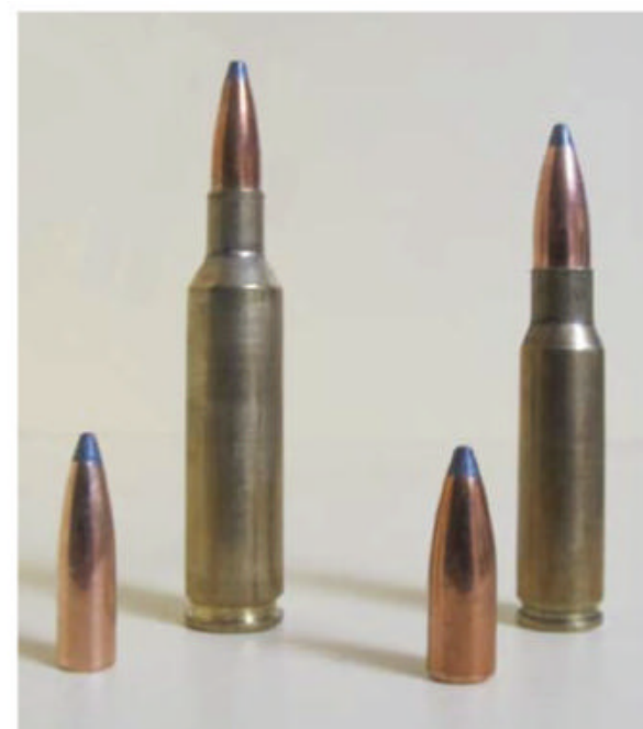
The 90gr 6mm projectile at 3120fps (left) and 110gr 6.8 projectile at 2822fps have the same energy, but the 110gr projectile has more momentum and cross-sectional area.
