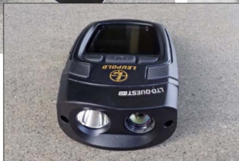
Leupold's LTO Quest HD compact, handheld thermal scanner.
