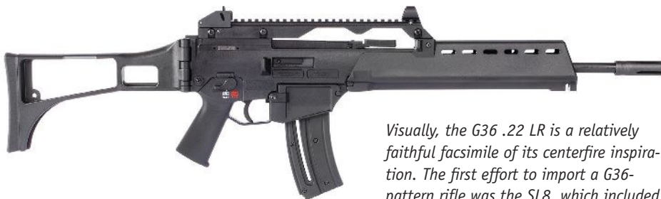
The hooded front post is typical of H&K rifles, but a departure from the original G36. The flippable rear sight consists of an aperture for speed and a notch for greater precision.
