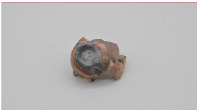
Left: A Precision Hunter bullet recovered from the wetpack. It retained more weight than the Match bullet.
