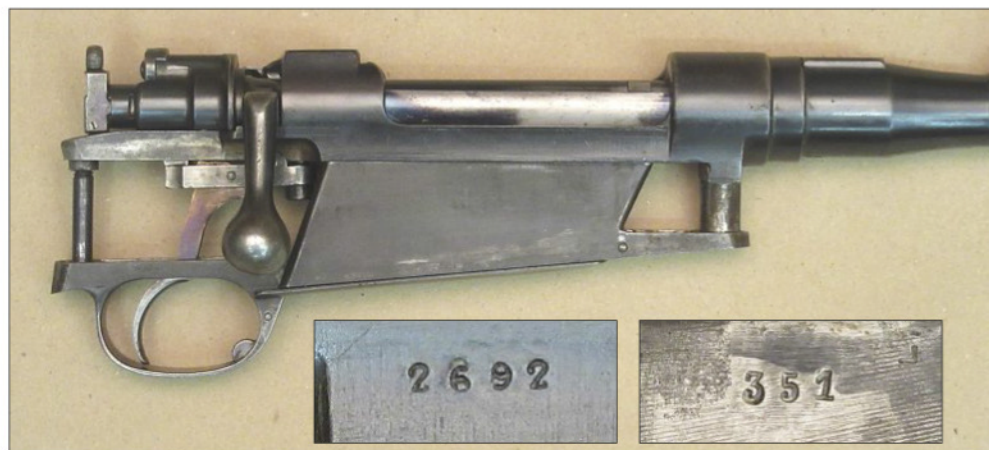
Rifle no. 1 action with slanted magazine box and step-down receiver ring. Rigby number 2692 and Mauser number 351.
