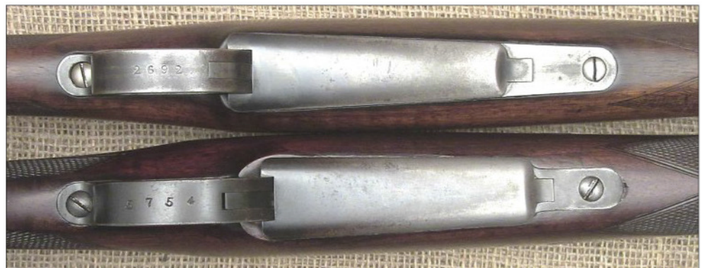
Bottom view showing the difference between a slanted-magazine-box Magnum action (top) and a normal Magnum action (bottom). Both floorplates are of the straddle type and the slanted magazine box is significantly tapered to its front to accommodate the .400/.350 NE cartridge.
