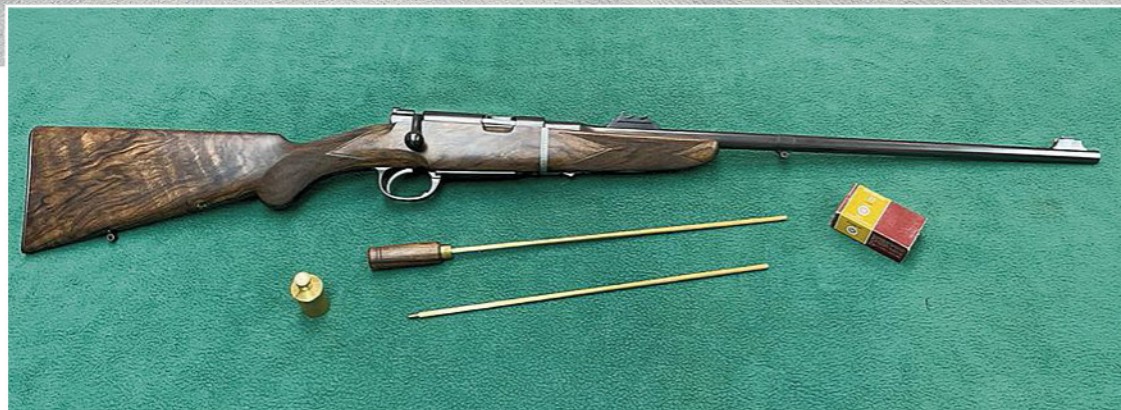
TOP AND BOTTOM: Johan converted the Mauser .22 LR into a take-down rifle – a copy of the owner's .275 Rigby rifle. The result is a creation that will stand tall among custom rifles from around the world.
