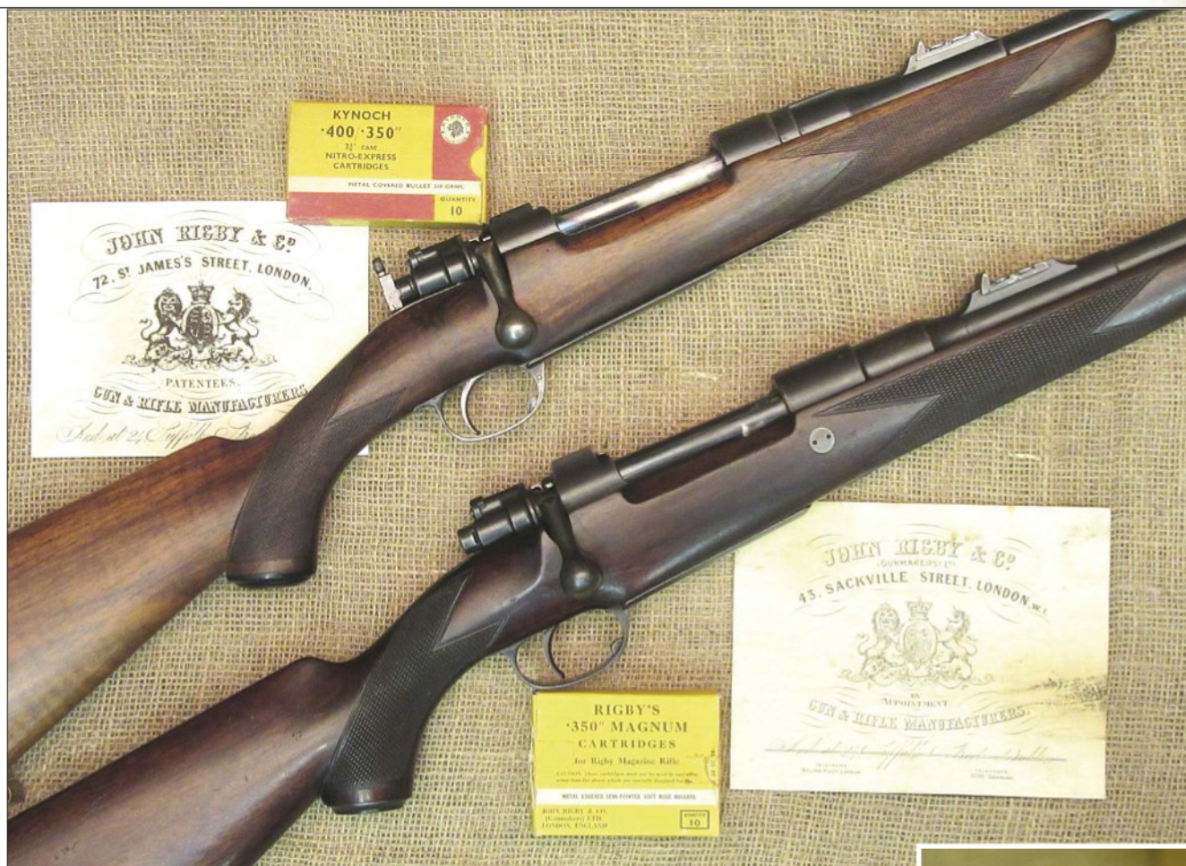
TOP: Early (1906) Rigby in calibre .400/.350 NE, built on a slanted-magazine-box Magnum action with step-down receiver ring. BOTTOM: Late (1947) Rigby .350 Magnum built on a normal Magnum action.
