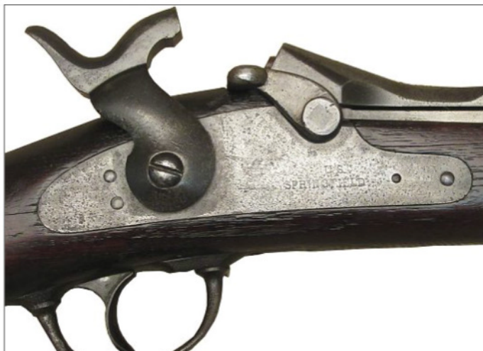
"U.S. SPRINGFIELD" stamped on the lock. Note the large, external, exposed hammer and the thumb latch for unlocking the breechblock.
