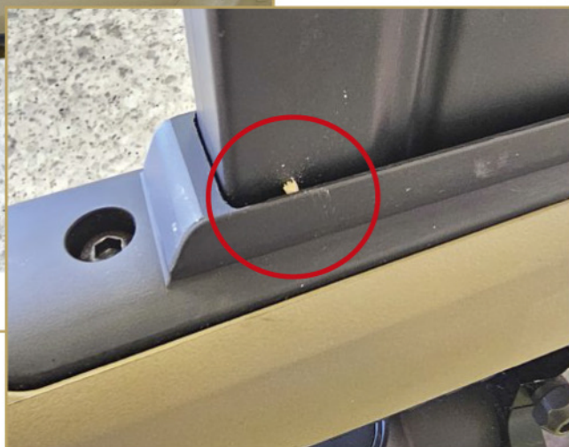
To stop the factory magazine from rattling, push a toothpick into the gap between the magazine wall and the well. Unconventional, but it works...
