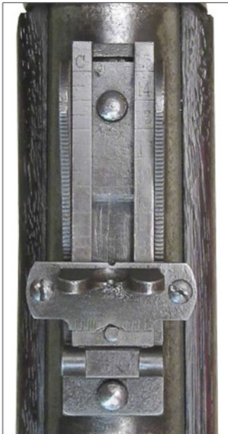
LEFT AND ABOVE: The early rear sight found on the carbine. Note the “C” stamped into the top left of the ladder and on the left side.
