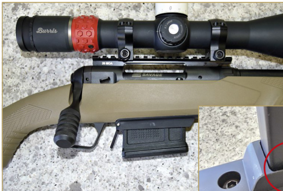
The rifle fitted with the replacement Magpul five-shot magazine. To me, this is the answer for taking the Savage to the bush.
