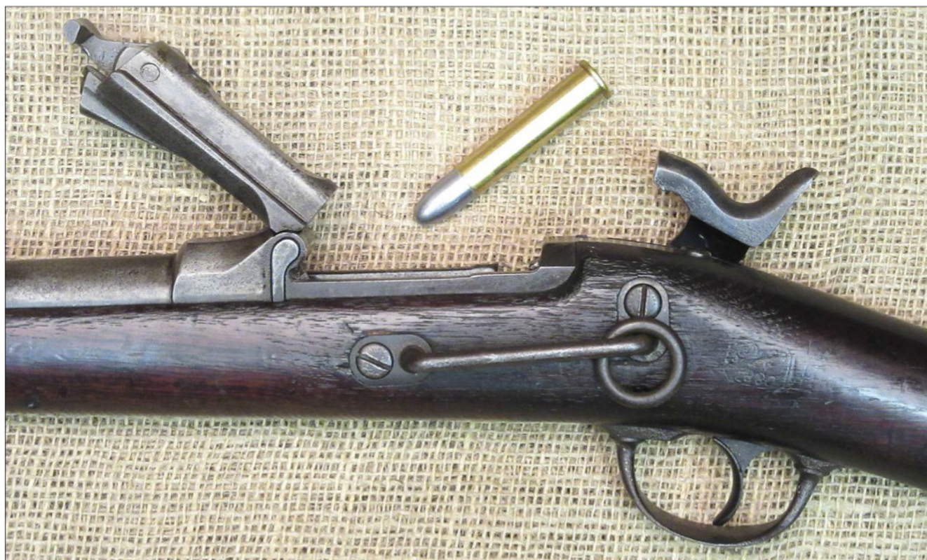
Loading the Trapdoor action. Once a single cartridge is inserted, the breech is closed and the rifle is ready to fire.
