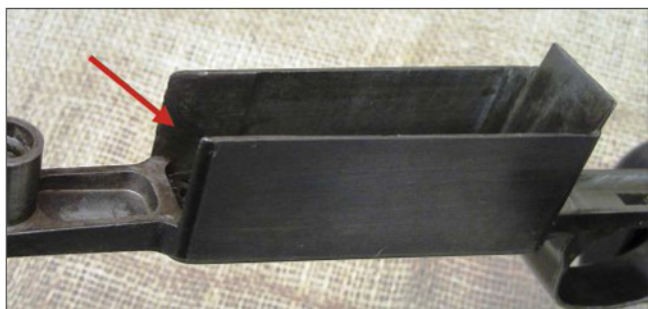
Magazine box with front wall completely cut away.
