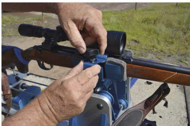
Kobus adjusting the clamps that secure the forend.
