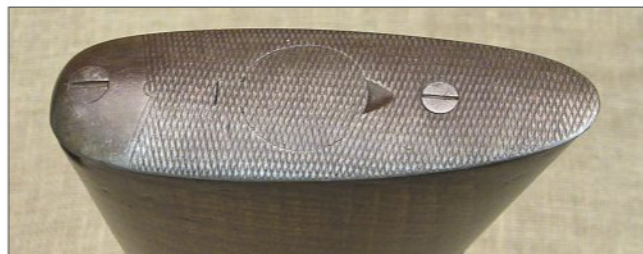
Original steel butt plate with trap as fitted to both rifles.
