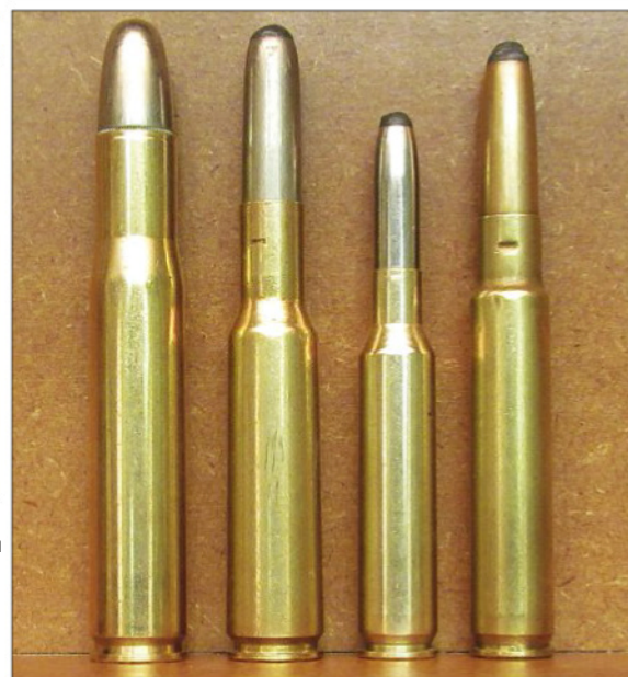
FROM THE LEFT: .404 Jeffery, .333 Jeffery, 6.5x54mm Mannlicher-Schönauer and .318 Westley Richards cartridges. Note that the .333 has almost the same overall length as the .404.
