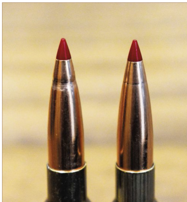
LEFT: A soft-cone bullet seated into an unprepared new case. RIGHT: A soft-cone bullet seated into a prepared new case.
