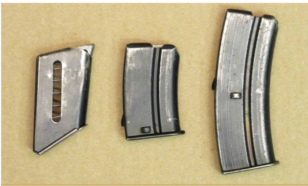
LEFT TO RIGHT: First-series slanted, five-shot magazine, B-series curved, five-shot magazine, B-series curved, ten-shot magazine. Original B-series magazines have a small Mauser banner on the base plate.
