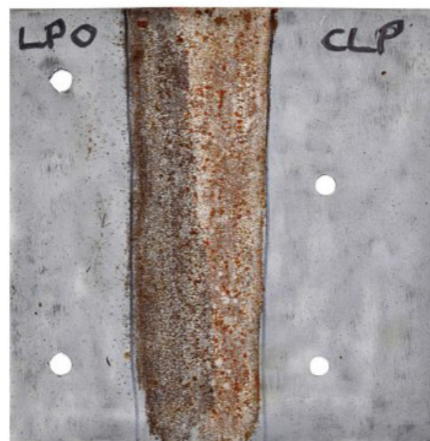
The metal plate treated with LPO (left) and CLP (right). The middle section was left untreated.
