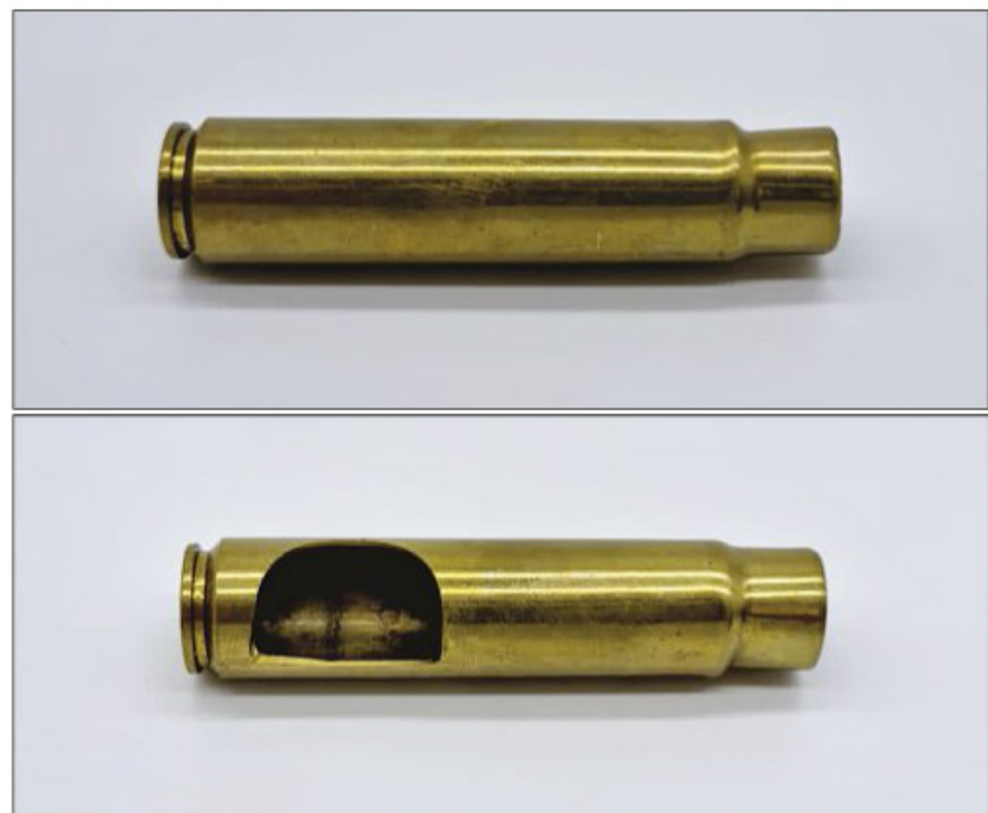
TOP: A .500 Jeffery case with a distorted shoulder, but seemingly without case head separation.
