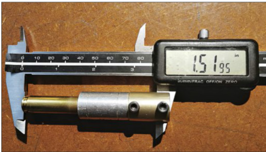
The head-to-shoulder dimension of a new, unfired Lapua 6,5 Creedmoor case.
