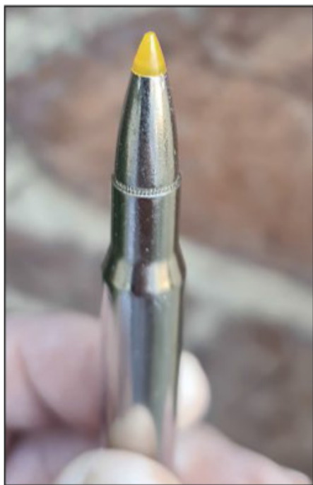
The Trophy Bonded Tip bullets have a plastic cap to protect them against deformation in the rifle's magazine during recoil.
