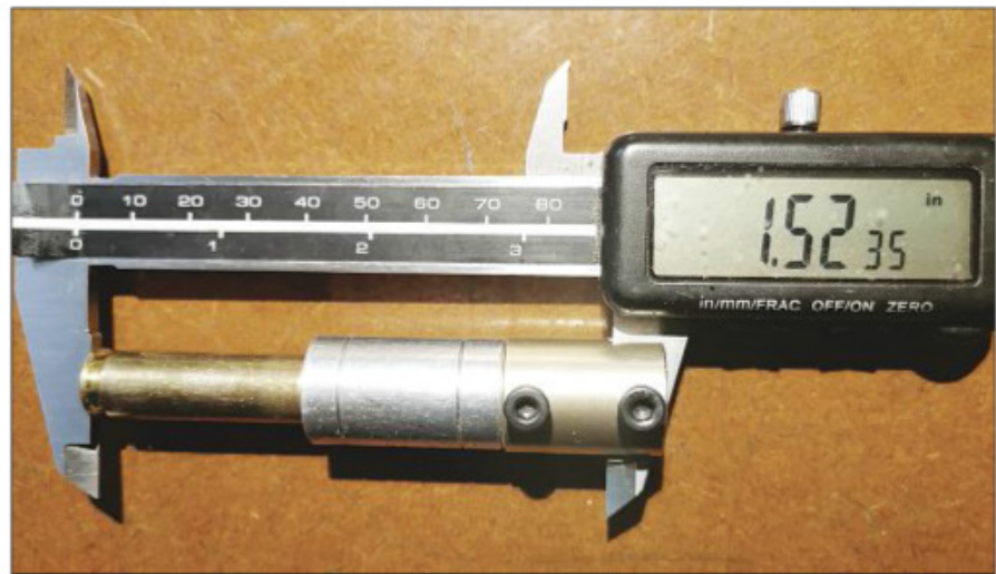
The head-to-shoulder dimension of the same case after being fired in the Tikka UPR rifle.
