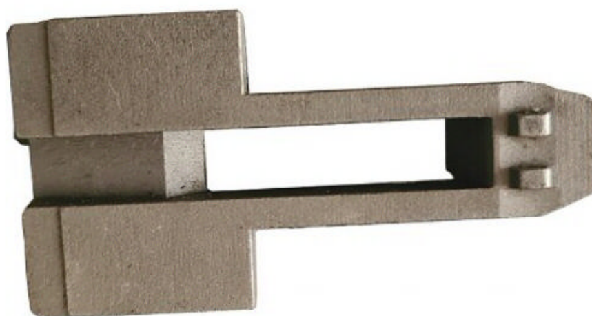
A view from the top of a "key", or sliding-bolt, of a B25. Manufacturing a new one is a job for the brave!
