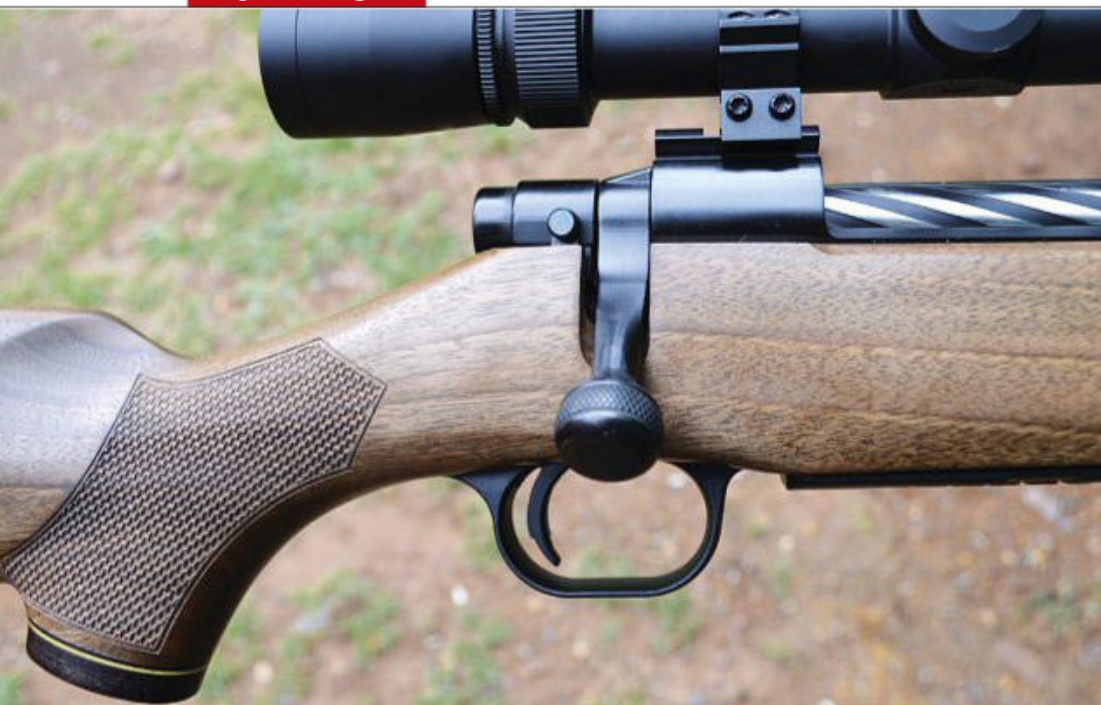
The Mossberg features two-panel chequering on the pistol grip. Note the safety catch on the right side of the bolt shroud.
