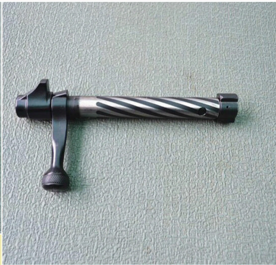
The bolt is fluted to save weight and ensure smooth travel.
