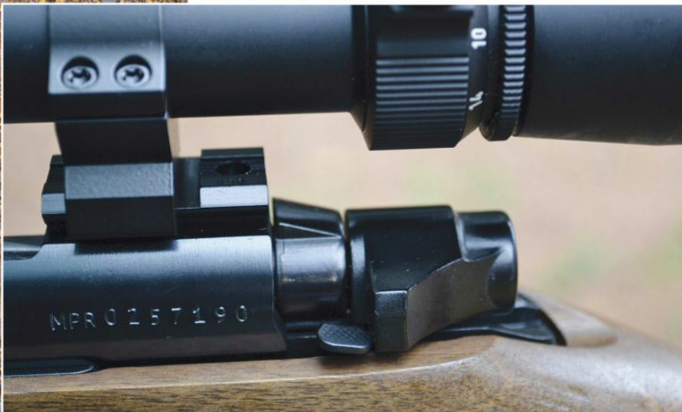
The bolt release button is situated on the left side of the bolt shroud.
