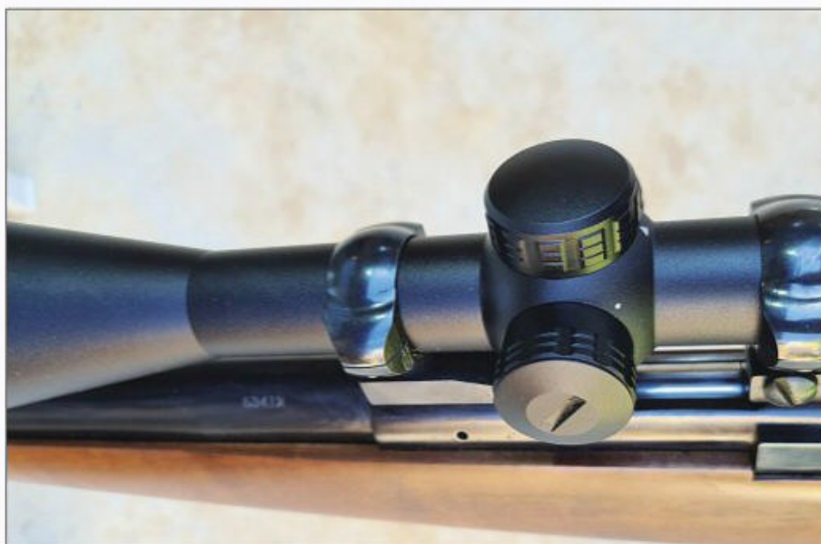
The illuminated reticle's adjustment knob is situated on the left side of the turret housing.
