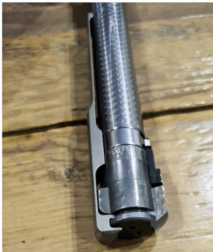
The Model 70's broad, Mauser-style claw extractor ensures control-feeding and positive extraction and is a very desirable feature on a rifle intended for dangerous game.
