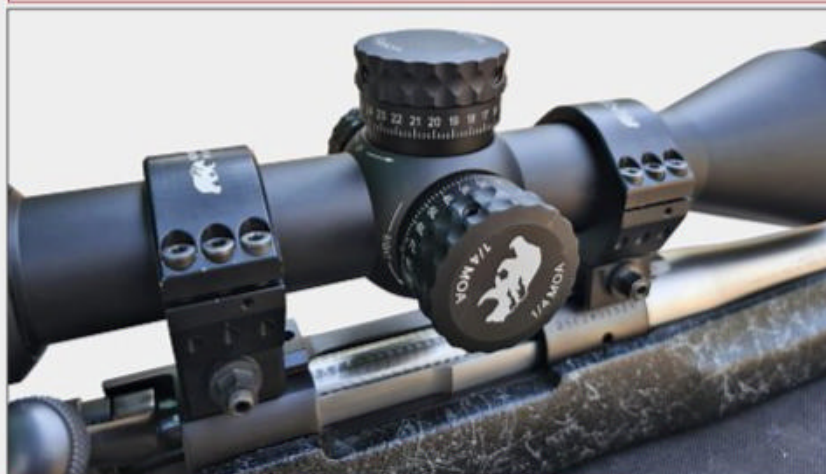
The Nordiske's turrets are stout affairs and adjustments were easy to make and positive.
