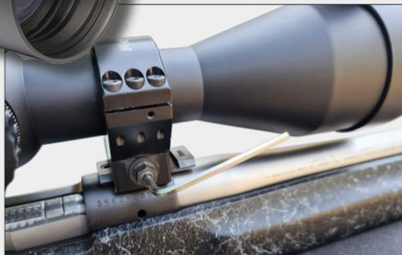
Windage-adjustable Nordiske rings were used to mount the scope on the rifle. They performed very well.
