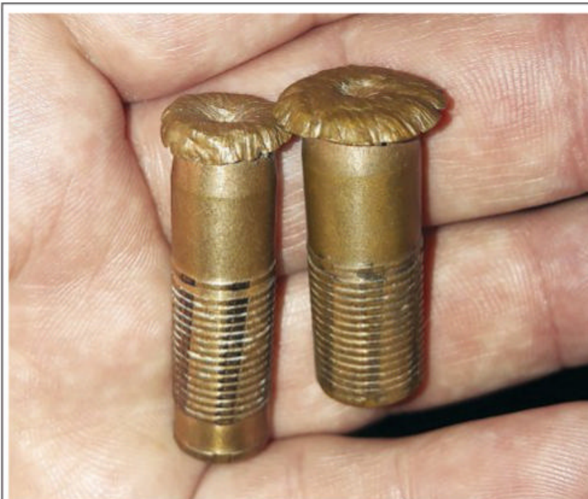
Two expanded North Fork Cup-Nose solids. Both were recovered from buffalo. On the left is a 400-grain .416 fired from a .416 Rigby. The bullet on the right is a 500-grain .458 fired from a .450 NE. The Cup-Nose is typical of the latest generation of bullets for dangerous game.
