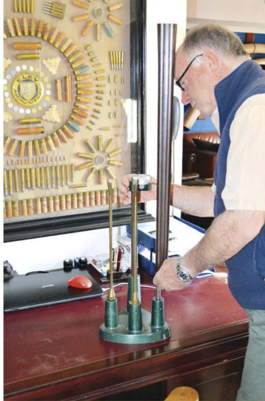
Gun dealer Andrew Tonkin measuring the barrels of a vintage Damascus-barrelled 12-bore gun. A barrel thickness gauge such as this is an essential piece of kit for the dealer who wants to make a living selling old guns and is the prime hedge against disaster in the form of dangerously thin barrels.
