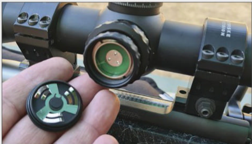
The battery housing for the illuminated reticle on the left side of the scope, located next to the parallax adjustment and illuminated reticle adjustment wheels.
