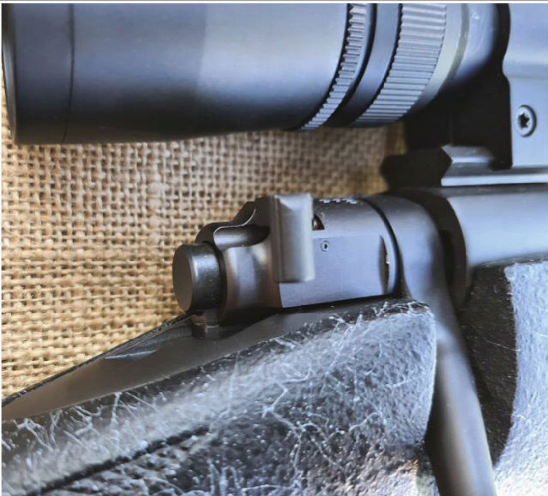
The Winchester three-position safety is one of the best in the business and has been copied by many.
