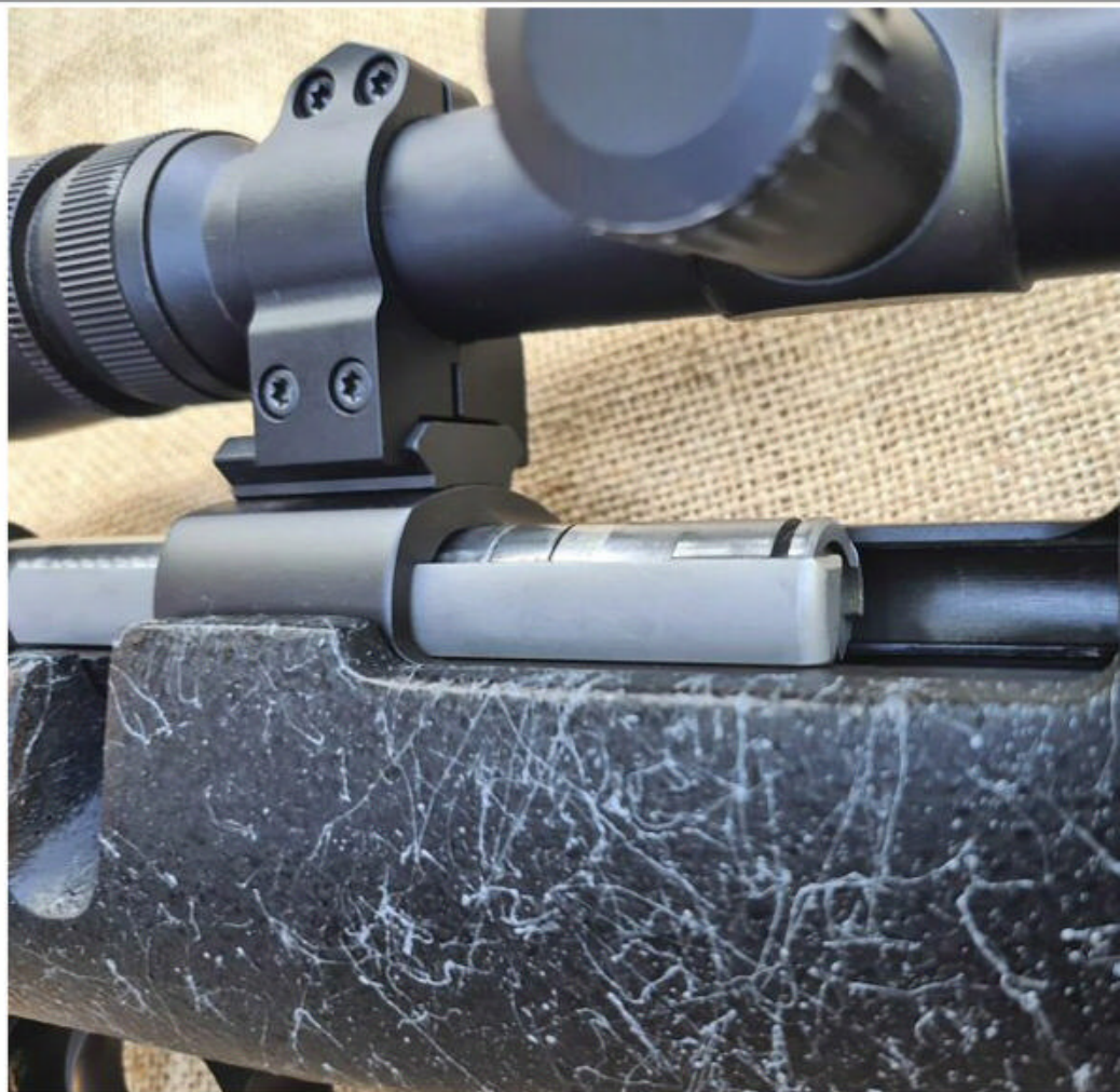
The Mauser-type claw extractor has been one of the redeeming features of the original Model 70. It is a standard feature on the latest Model 70s as well and is seemingly here to stay for good.
