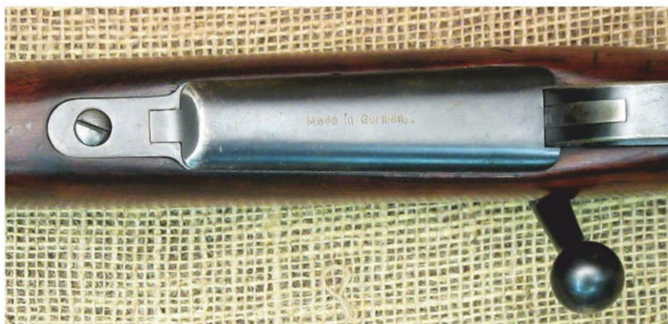
Mauser .318 straddle-type magazine floorplate.
