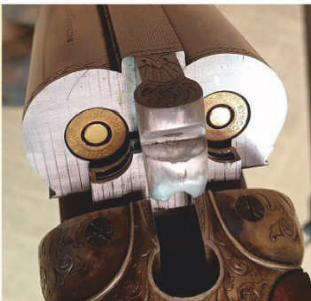
Rifle with cartridges loaded. Notice how the cartridges have dropped all the way into the chambers, past the extractors that are in the lowered position.
