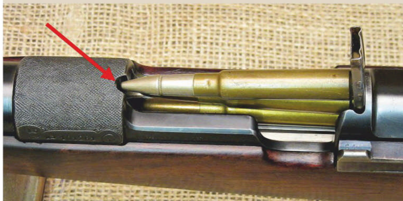
The Mauser receiver cut-out to allow loading of cartridge with LT capped-pointed bullet using a 5-round stripper clip.
