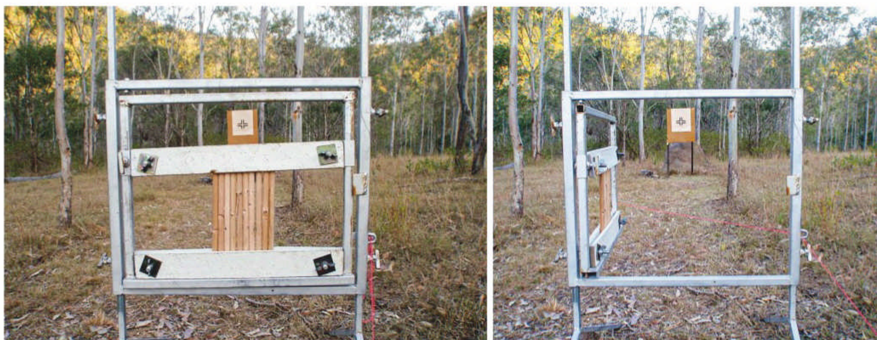
LEFT: The frame with the window closed and the target in the background. RIGHT: The frame with the window open and the target in the background.
