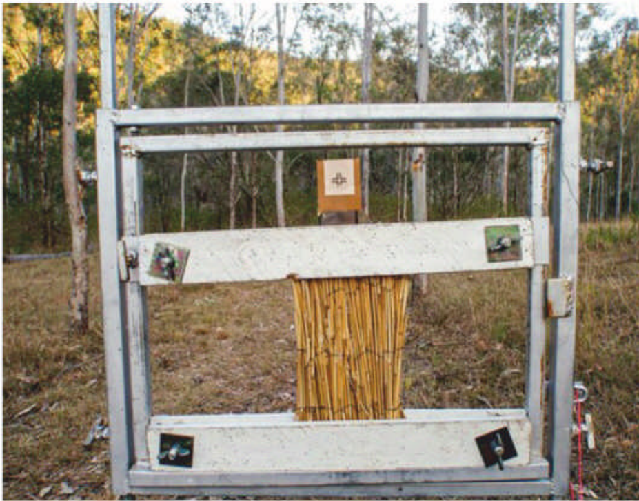
The cane media clamped in the frame with the target in the background.
