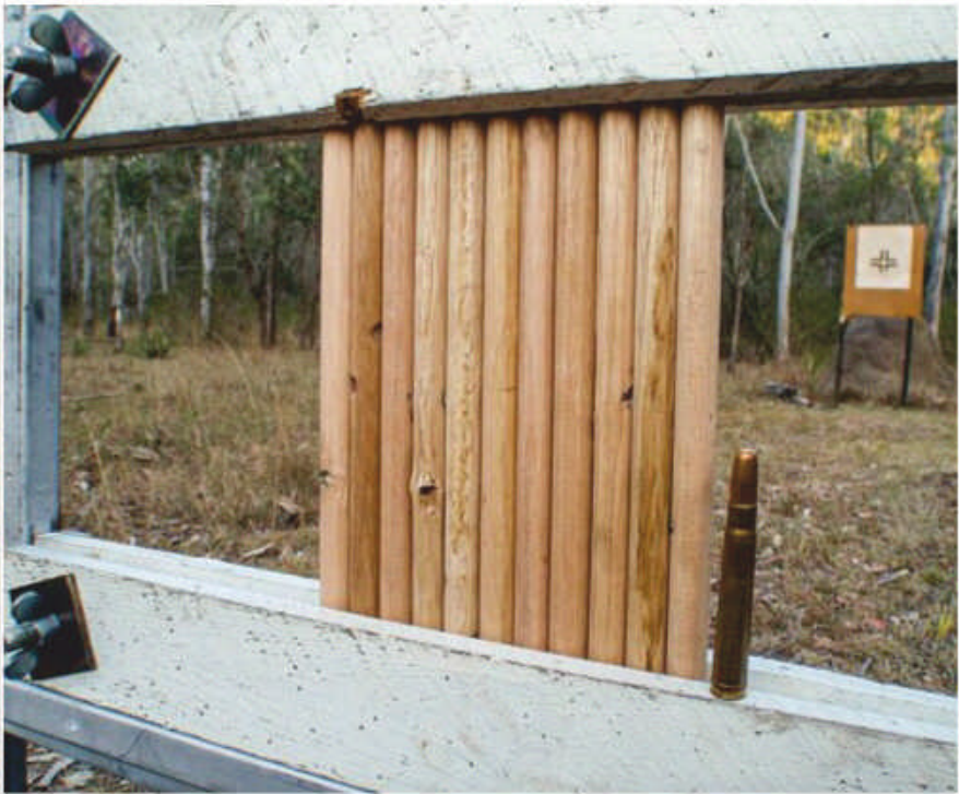
The 16mm dowel clamped in the frame with a .375 H&H cartridge for comparison.
