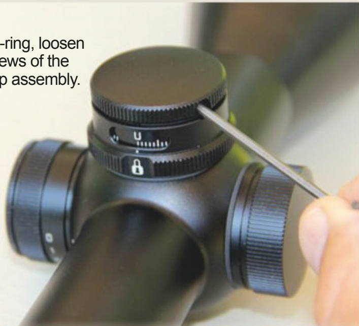
TOP LEFT AND RIGHT: Notice the lock-ring (bottom half of the turret) in unlocked and locked position. The latter prevents accidental adjustment when in the locked position. Also notice the “window” through which the index marks are visible.
