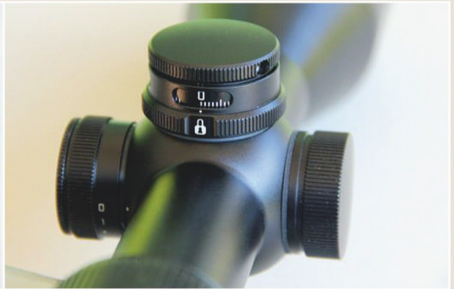
TOP LEFT AND RIGHT: Notice the lock-ring (bottom half of the turret) in unlocked and locked position. The latter prevents accidental adjustment when in the locked position. Also notice the “window” through which the index marks are visible.
