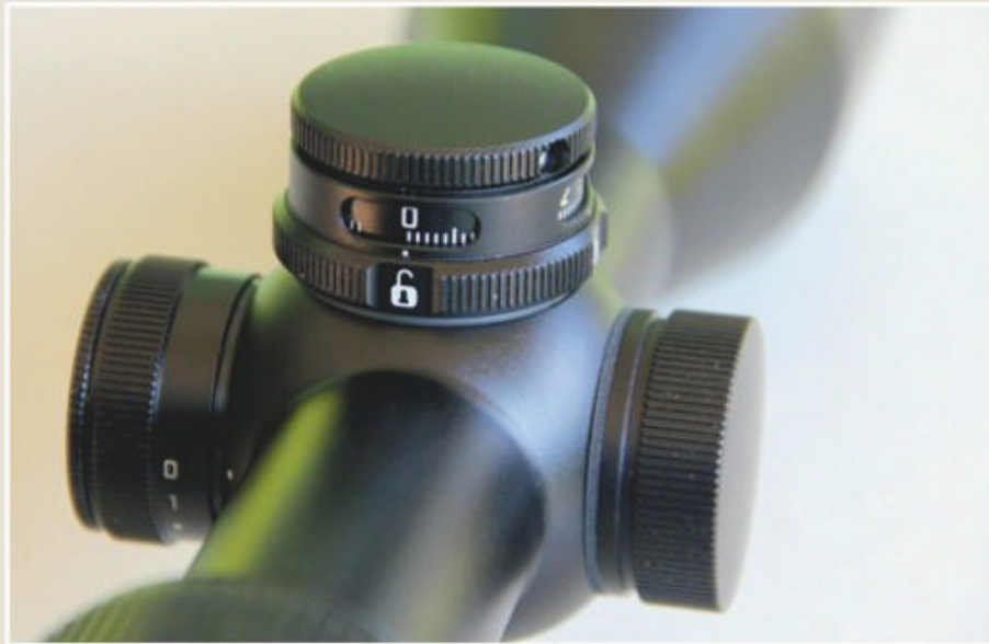
TOP LEFT AND RIGHT: Notice the lock-ring (bottom half of the turret) in unlocked and locked position. The latter prevents accidental adjustment when in the locked position. Also notice the “window” through which the index marks are visible.
